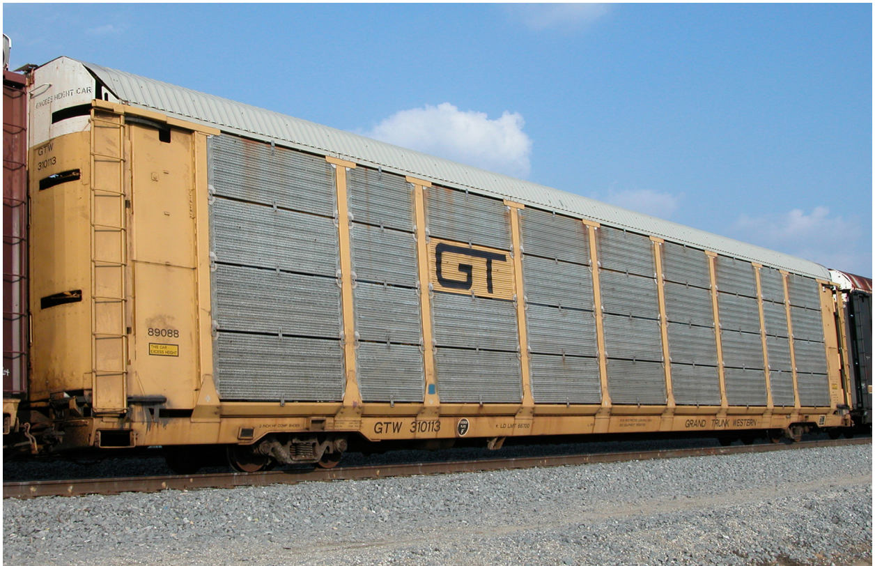
Tri-level, low-level, ExH 18'10", Radial doors. GTW 310113.
