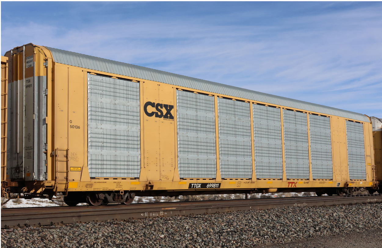
Bi-level, low-level, ExH 19'0", Tri-Fold doors. TTGX 699811.
