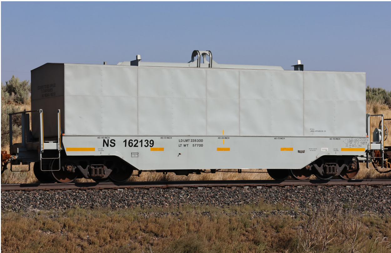
NS 162139. Built 8-23. From AOKX 100000-100149. H 14-6. Light weight 57,700 lbs. Photographed August 30, 2024. Summit County, Utah.
