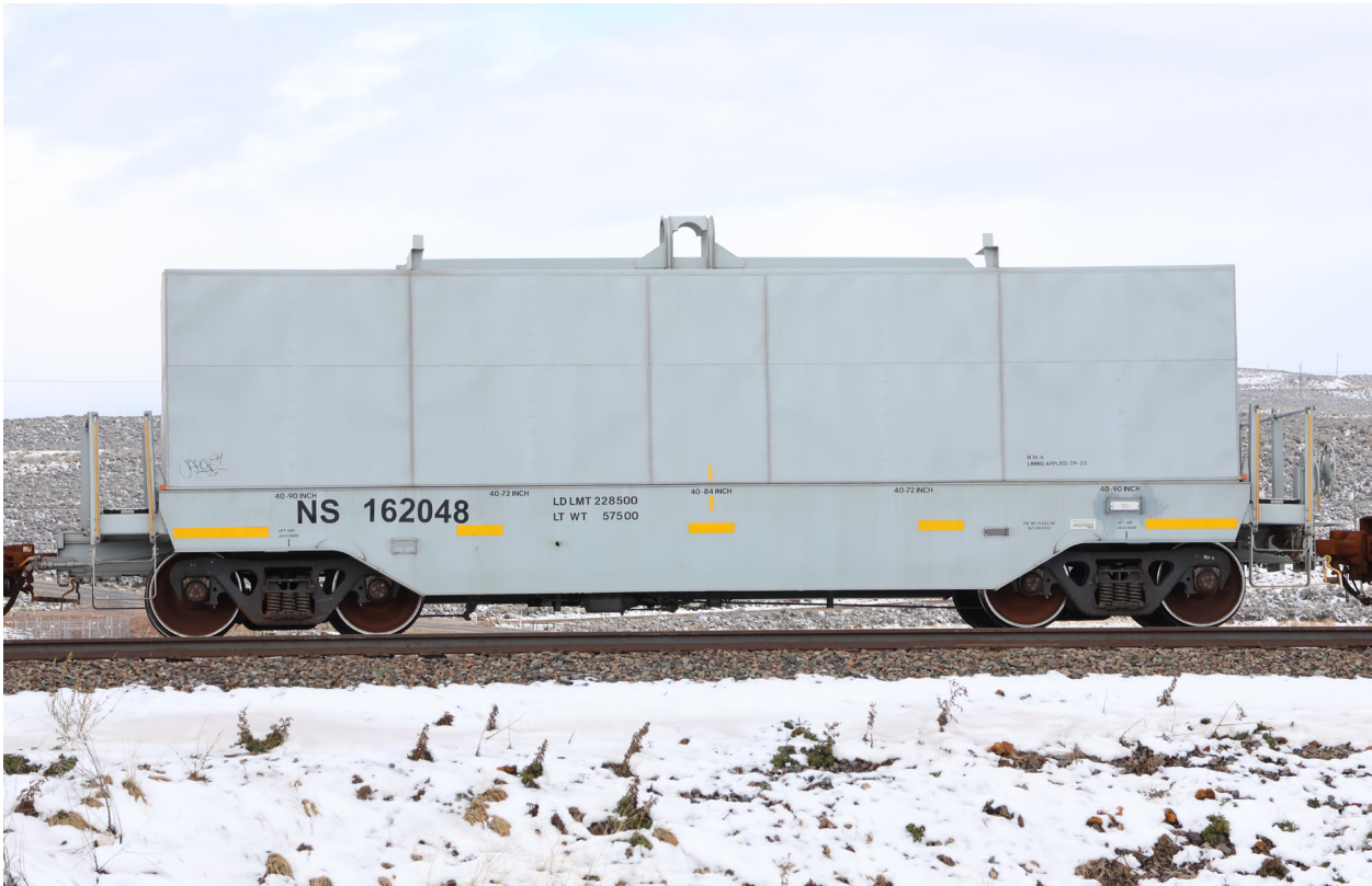
NS 162048. Built 9-23. Cover lining applied 9-23. This car is from the AOKX 100000-100149 series. H 14-6. Light weight 57,500 lbs. Photographed October 31, 2024. Summit County, Utah.
