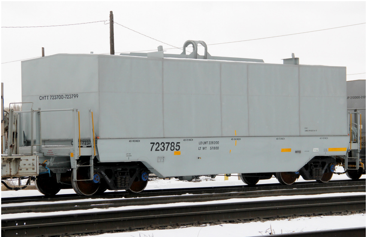
CHTT 723785. Built 6-22. Cover lining applied 6-22. H 14-1. Light weight 57,800 lbs. Missing side reporting mark. Photographed May 9, 2025. Uinta County, Wyoming.
