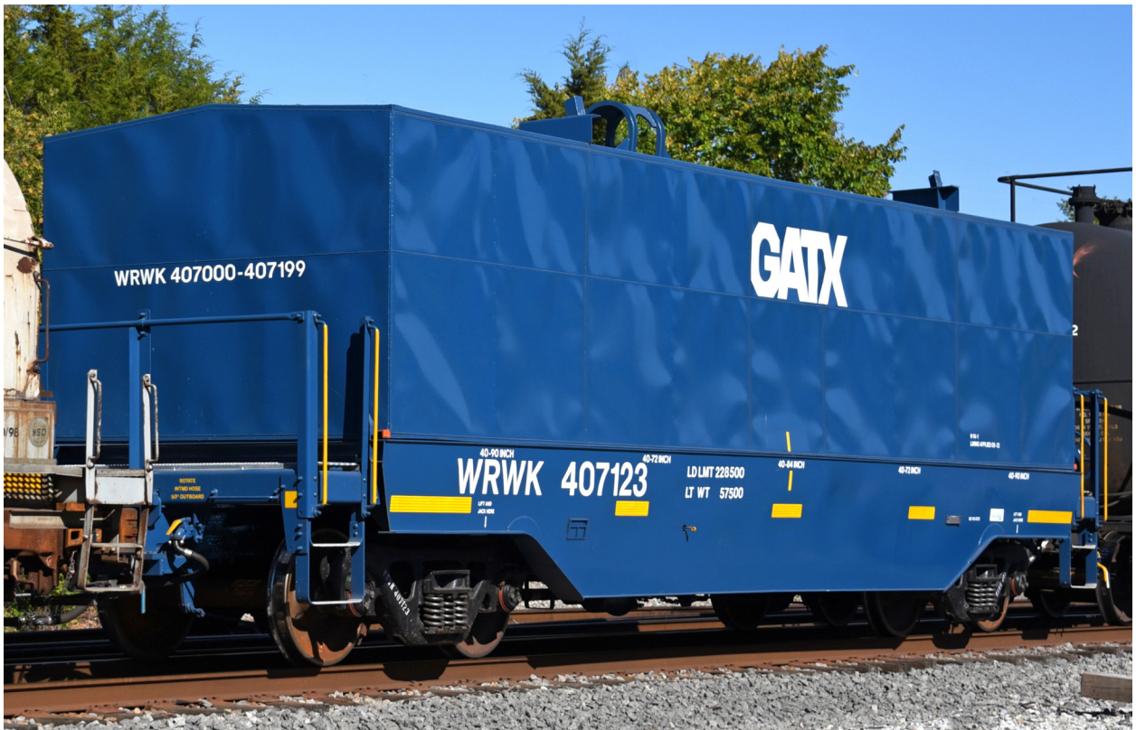
WRWK 407123. Built 8-22. Cover lining applied 7-22. H 14-1. Light weight 57,500 lbs. Photographed October 7, 2022. CSX Lewisburg, TN. Patrick Harris photo.
