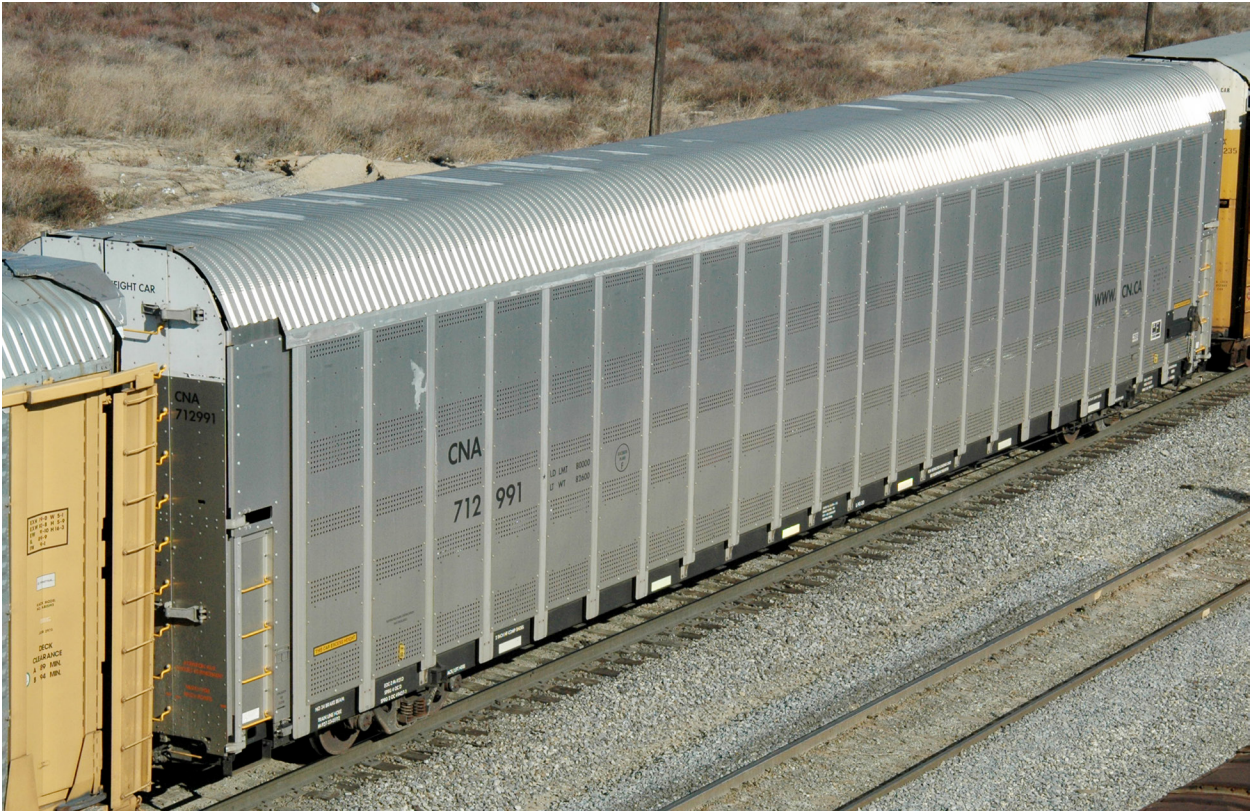
Bi-level, high-level, ExH 19'0", Bi-Fold doors. CNA 712991. This is Johnstown America's AVC, a steel integrated car and aluminum superstructure.
