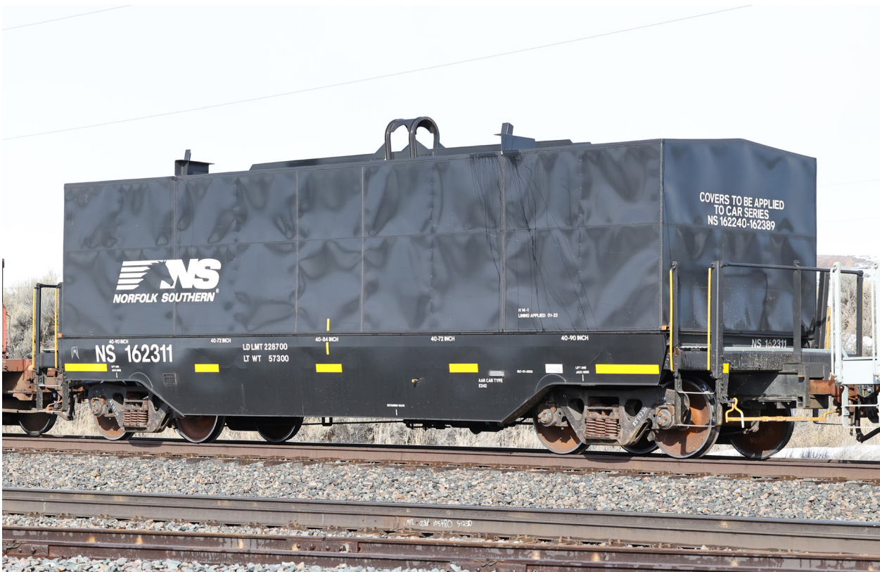
NS 162311. Built 1-23. Cover lining applied 1-23 H 14-1. Light weight 57,300 lbs. Photographed April 1, 2024. Summit County, Utah.
