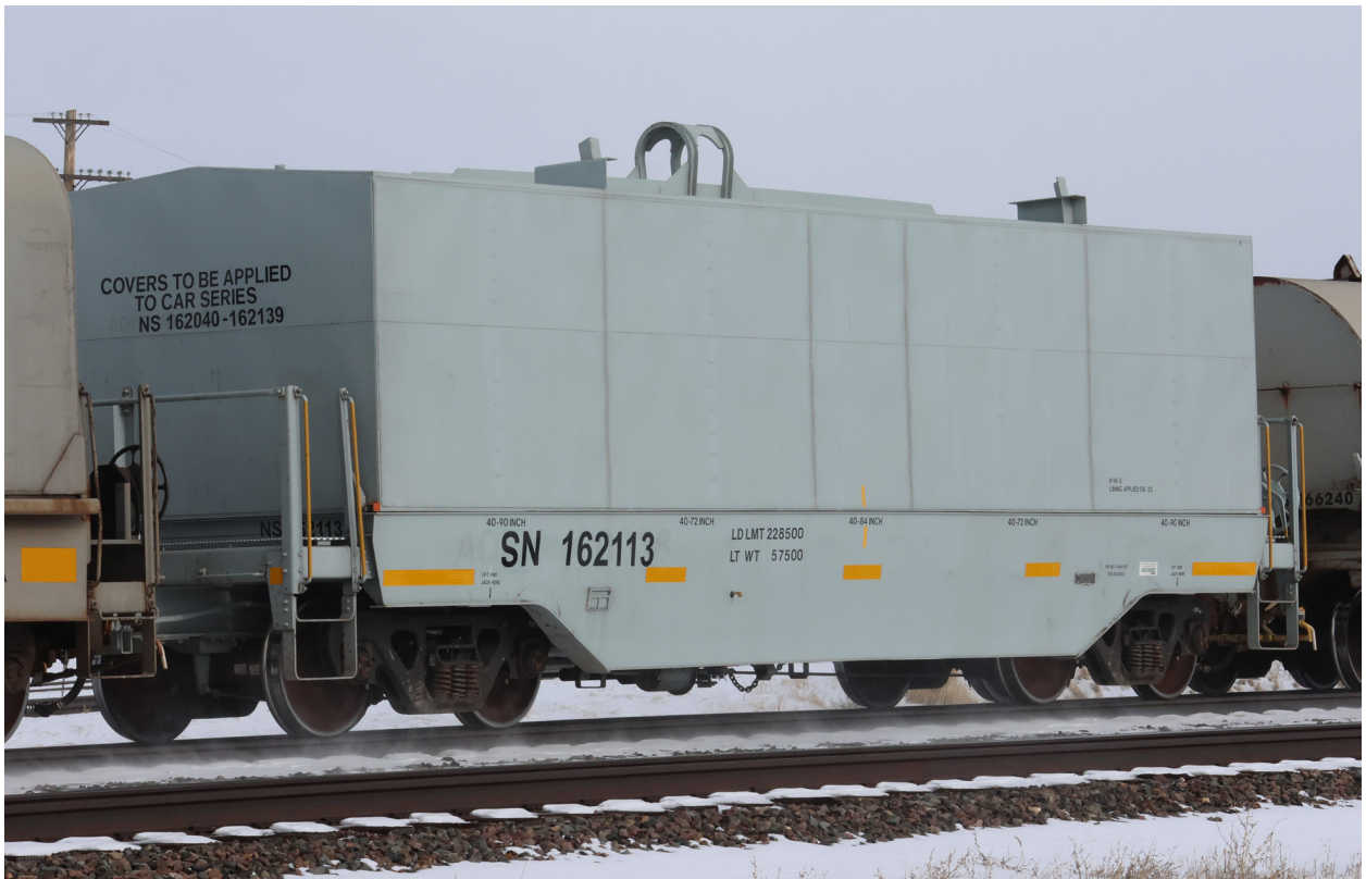
NS 162113. Built 9-23. Note the incorrectly applied reporting marks "SN". From AOKX 100000-100149. H 14-5. Light weight 57,500 lbs. Photographed February 15, 2025. Summit County, Utah.
