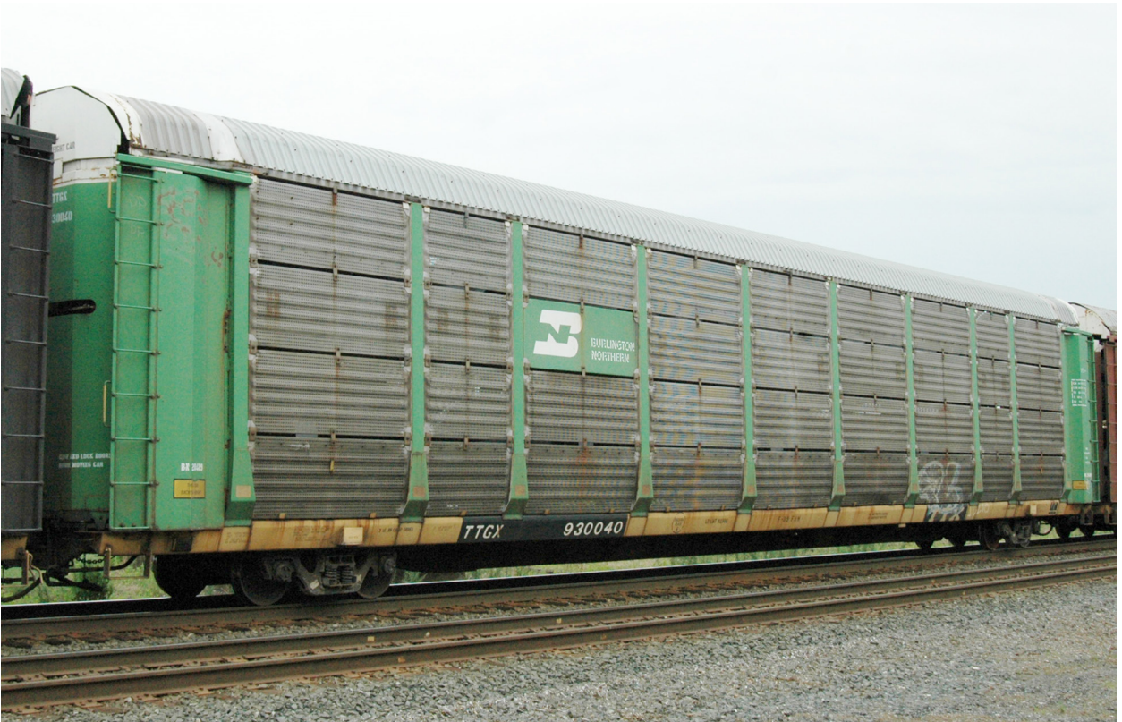
Bi-level, high-level, ExH 19'0", Tri-Arc doors . TTGX 930040.
