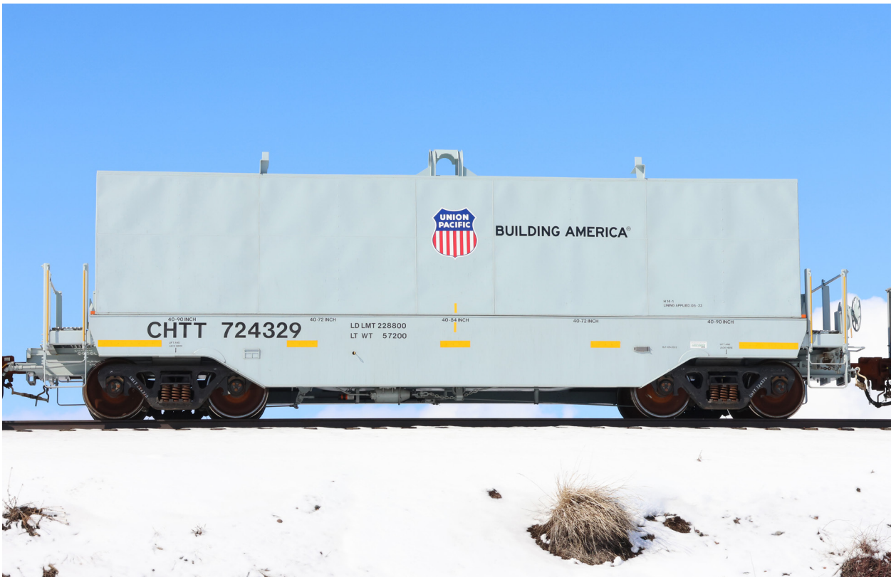
CHTT 724329. Built 5-22. Cover lining applied 5-22. H 14-1. Light weight 57,200 lbs. Photographed February 22, 2024. Uinta County, Wyoming.
