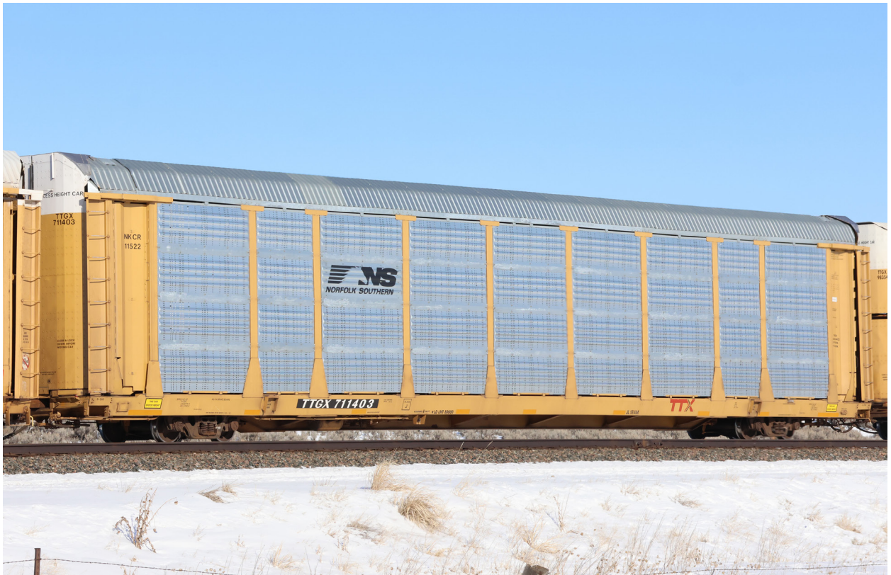
Bi-level, low-level, ExH 19'0", SealSafe doors . TTGX 711403.
