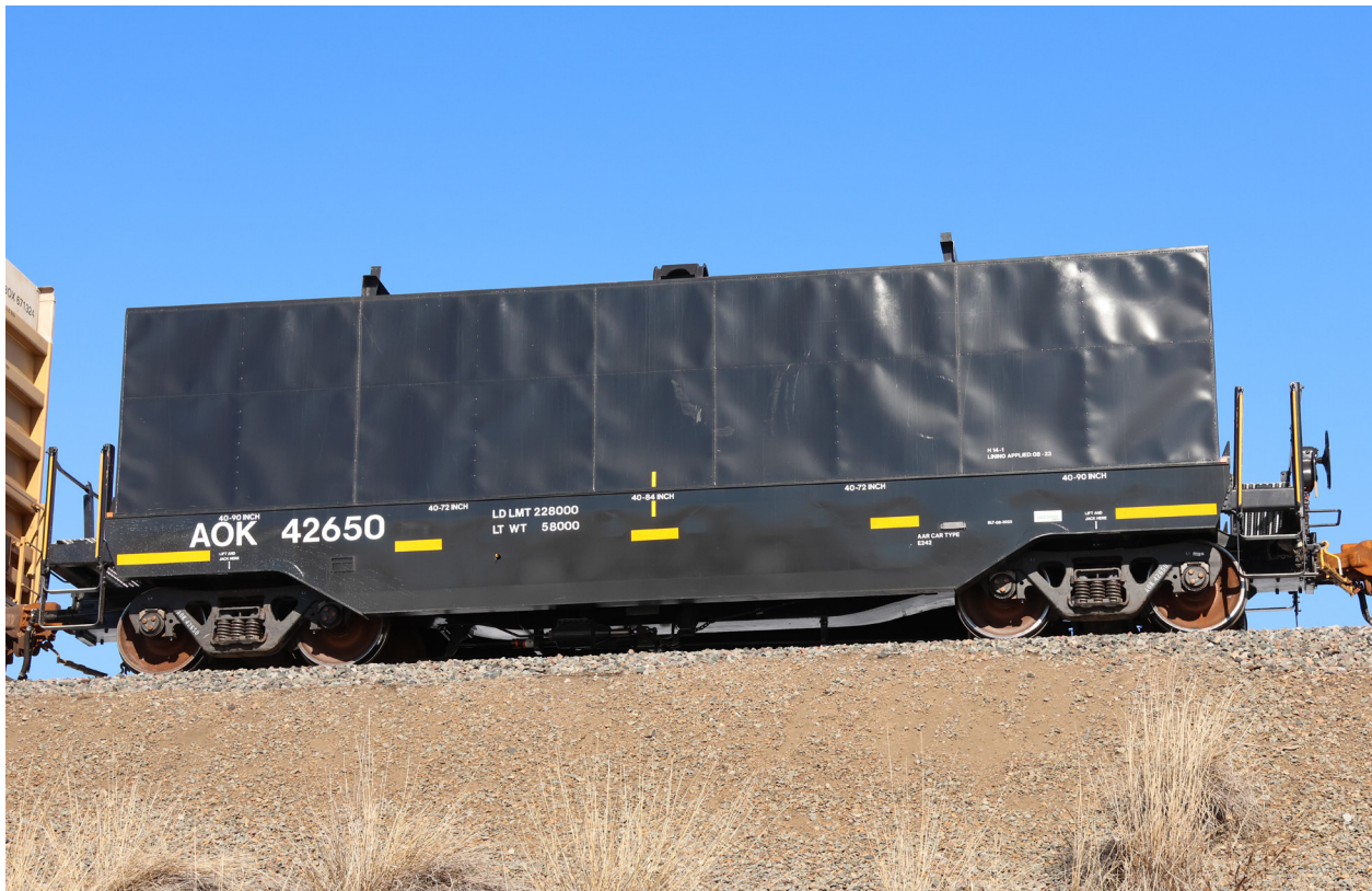
AOK 42650. Built 8-23. Cover lining applied 8-23. H 14-1. Light weight 58,800 lbs. Photographed January 30, 2024. Uinta County, Wyoming.
