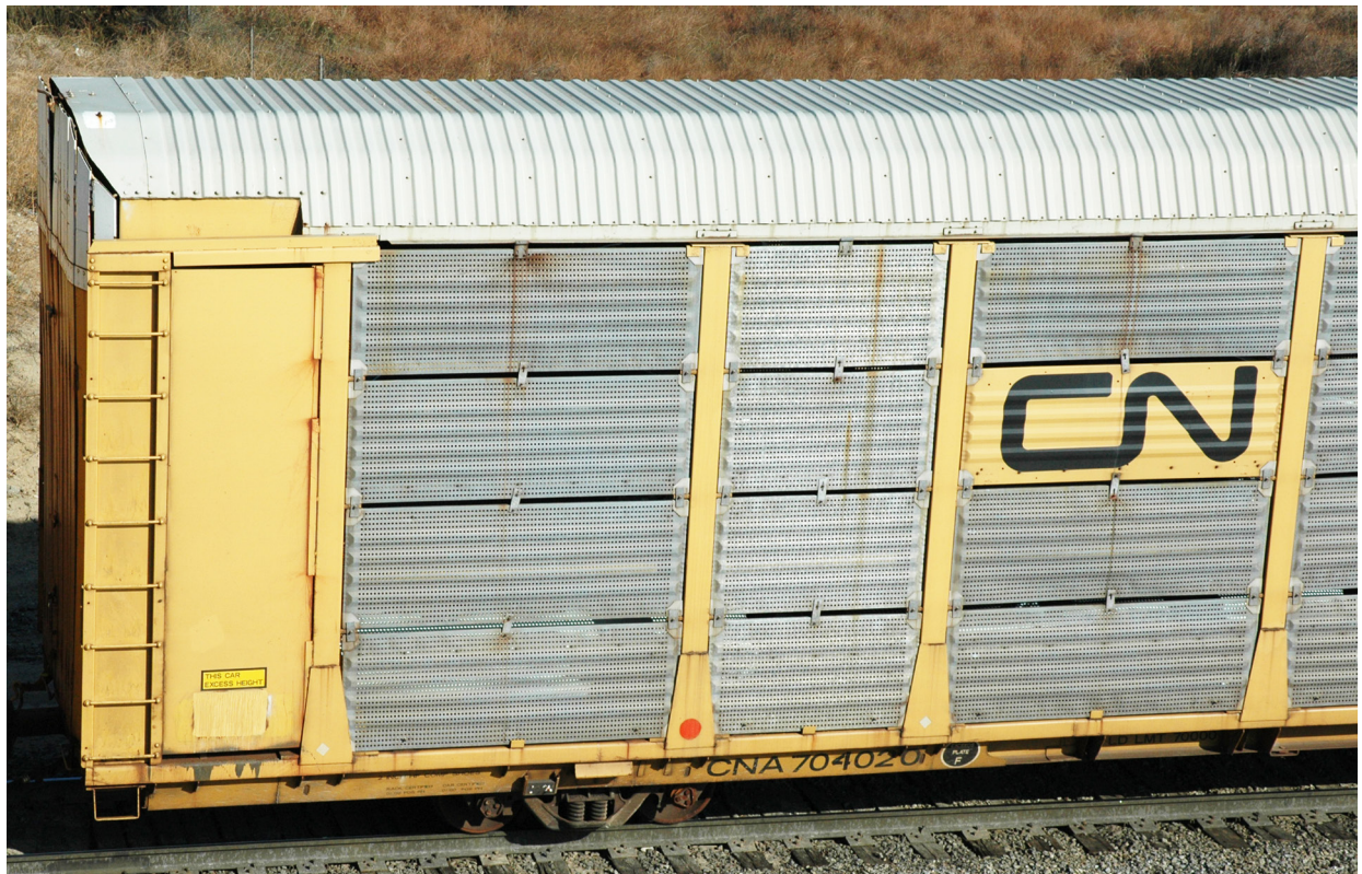
Tri-level, mid-level, ExH 18'11", Portec-RAVE doors. CNA 704020.
