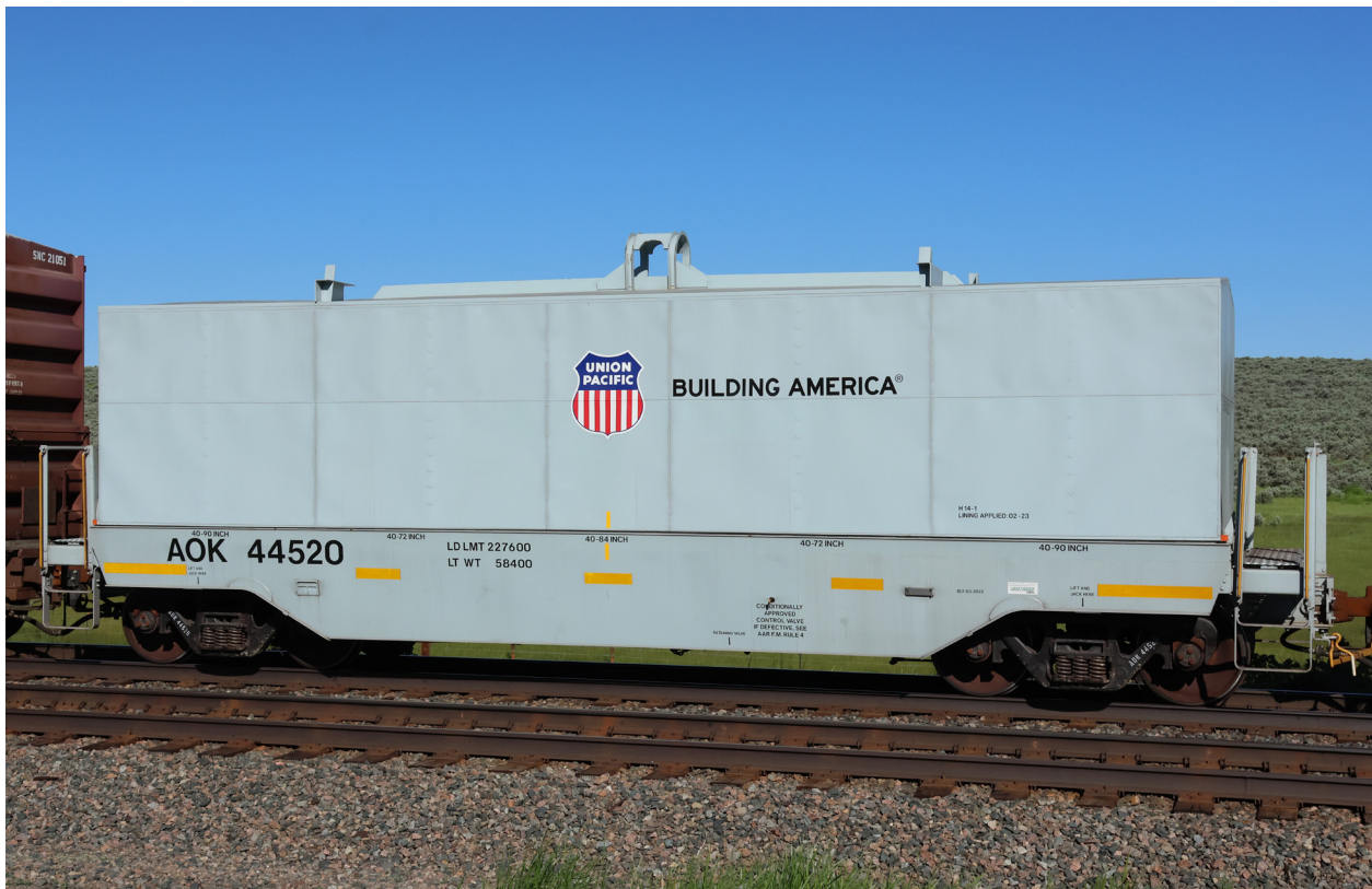
AOK 44520. Built 3-22. Cover lining applied 2-22. H 14-1. Light weight 58,400 lbs. Photographed May 9, 2025. Uinta County, Wyoming.
