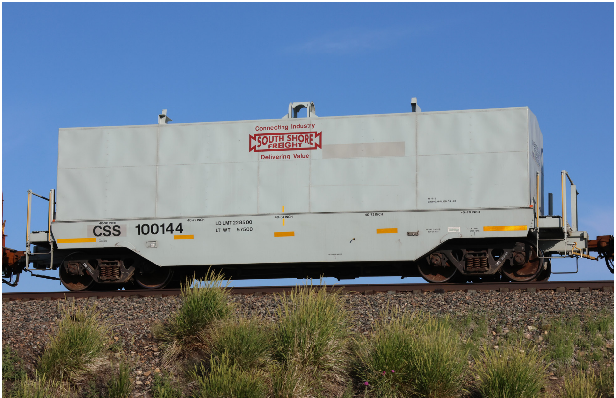
CSS 100144. Built 9-23. Cover lining applied 9-23. This car is former AOKX 100144. H 14-6. Light weight 57,500 lbs. Photographed July 2, 2025. Uinta County, Wyoming.
