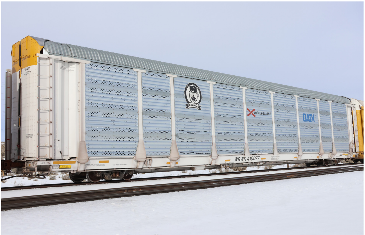
Bi-level, low-level, ExH 19'0", SealSafe doors . WRWK 410077.
