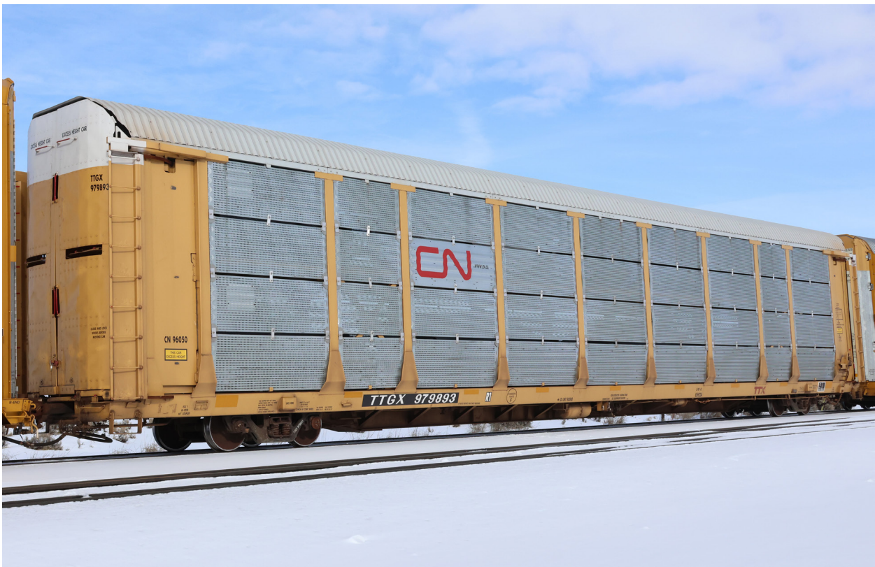
Bi-level, high-level, ExH 19'0", Radial doors . TTGX 979893.
