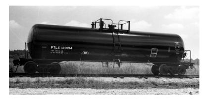
**PTLX 120194.** This non-insulated general-service tank car was built in June 1974 by Richmond Tank Car, Houston, Texas (builder's reference 1072). Capacity 21,034 gallons. DOT 111A100W1. AAR car type code T105.
