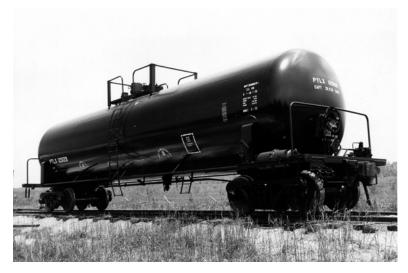
**PTLX 120128**. Built in May 1973 by Richmond Tank Car, Houston, Tx (builder's reference 1064). Capacity 20,938 gallons. DOT class 111A100W1. This is a non-insulated tank car. AAR car type code T105.
