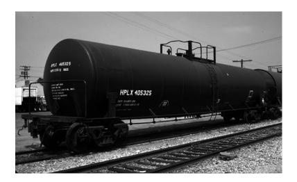
Two views of **HPLX 405325**. This car was built in August 1979 by Richmond Tank Car. Insulated and coiled. DOT 111A100W3. Its believed that the tank was actually fabricated by Trinity Industries (before they became the mega railcar builder today) as evidenced by the "T.I. Inc" on the tank's day fabrication date (8-9-79).
