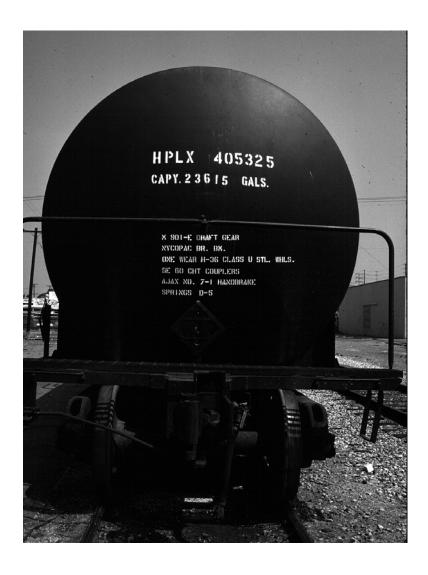
A full "head" on end view of **HPLX 405325** shows the simple Richmond style insulated jacketing. Lettering details the type of draft gear, brake wheels, couplers etc.
