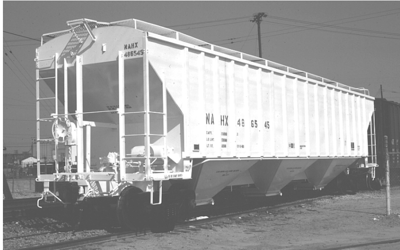
NAHX 486545. An example of a 4750-cubic-foot covered hopper - still the most commonly seen grain & potash covered hopper on GERSCO's roster.
