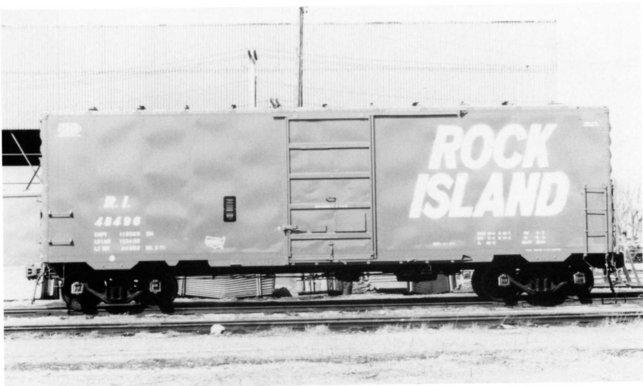
TOP Rock Island 48268 is from lot 995. Rebuilt in November 1970, it is one of 100 ex-New Haven cars sent into a new lease to the RI. Originally built by Pressed Steel in August 1941 it is green with white markings. This car, fitted with an eight foot door and rated at 3715 cuft. went into the series 48200-48299.
