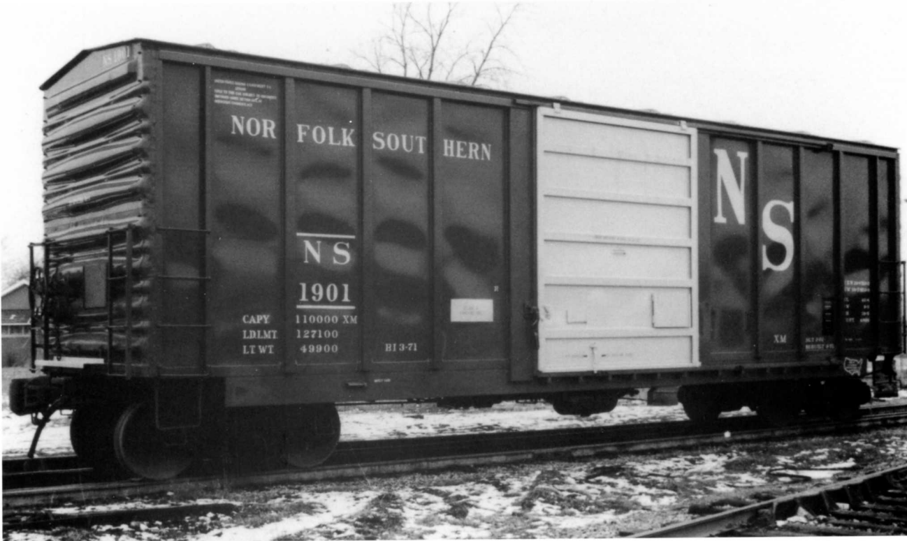
BOTTOM Under lot 596 Evans leased to the NYC 500 box cars in the series 207500-207999. Rebuilt in April 1967, there were two sets of cars; those with 3842 cuft. rating and cars similar to this one, which was rated at 3687 cuft. This car, originally built in April 1942 as lot 703-B, was given the NYC lot 118-B upon the rebuilding.
