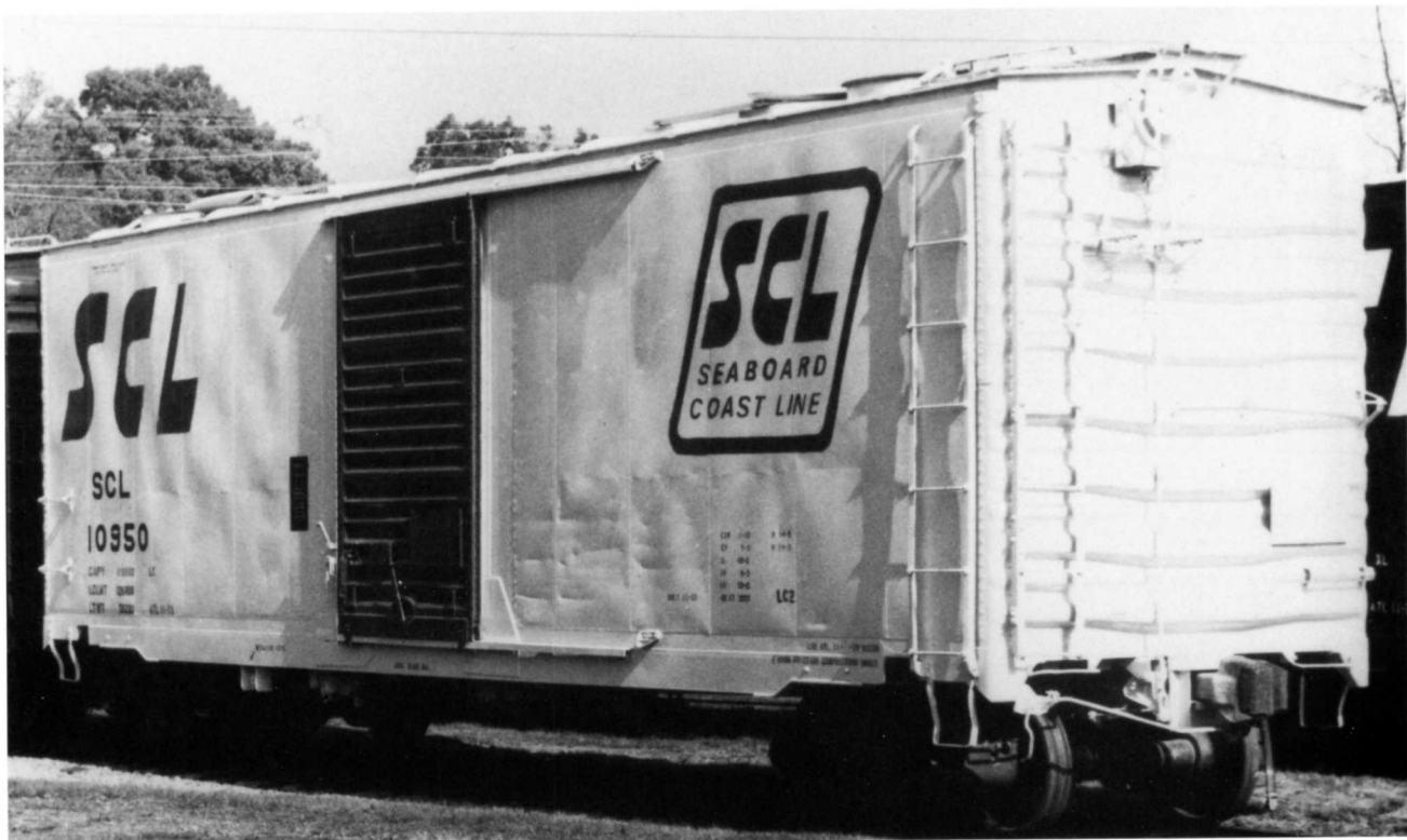
BOTTOM The Seaboard Coast Line picked up 100 of these "LC" design cars in November 1970 under lot 1076. Assigned class LC-2, these cars featured 4 roof hatches and were rated at 3933 cuft. It was part of the 10950-11049 series (from ACL's O-26 22230-23595 series) and had 30" roof hatches and 6' doors.
