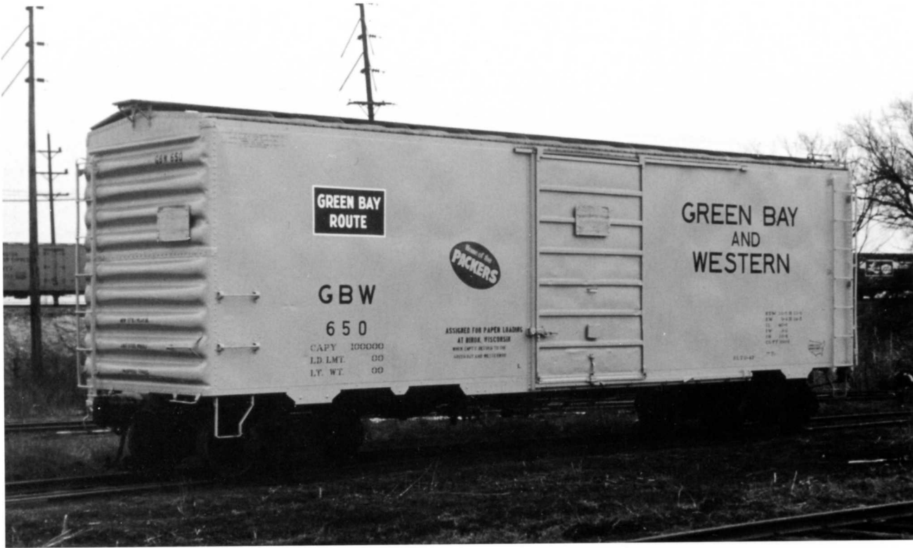
TOP The Green Bay and Western leased this smart looking car from USEX. It was one of 42 cars rebuilt under lot 324 that it went into the GB&W as part of the series 650-691. These cars were in roll paper service. This particular car is in assigned service to Biron, WI. Originally built in December 1947 it is yellow with black stencilling. The logo
