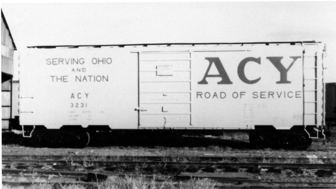
Akron, Canton and Youngstown received this good looking car under lease from USEX. We do not know anything about this car other than it was rated at 3717 cuft. and originally built in March 1948. The small repack data is nearly unreadable, but indicates a 1962 date. This car did become part of the ACY series 3200-3346, presumably all from USEX. It was bright yellow with red stenciling. Though tough to see, the roofwalk is unpainted except at the ends.
