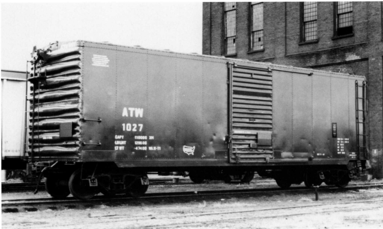
TOP Atlantic and Western 1027 is one of 30 cars out of lot 1102. Rebuilt in October and November 1971, it is a part of the series 1001-1030. Rated at 3903 cuft., this car was originally built in May 1947. Official Railway Equipment Register information shows numerous individual cars with varying dimensions including cubic capacity, supported by the roster notes of "miscellaneous boxcars." This car was deep blue with white stenciling.
