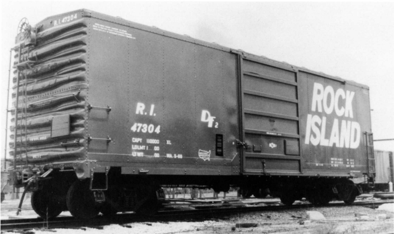
BOTTOM The Rock Island was a good customer of USEX rebuild equipment. Here RI 47304 shows off her green and white markings in May 1969. While we do not have any lot information on this series, it was a part of the 102 cars series 47300-47401. These cars had four DF-2 belts and was built in November 1945.
