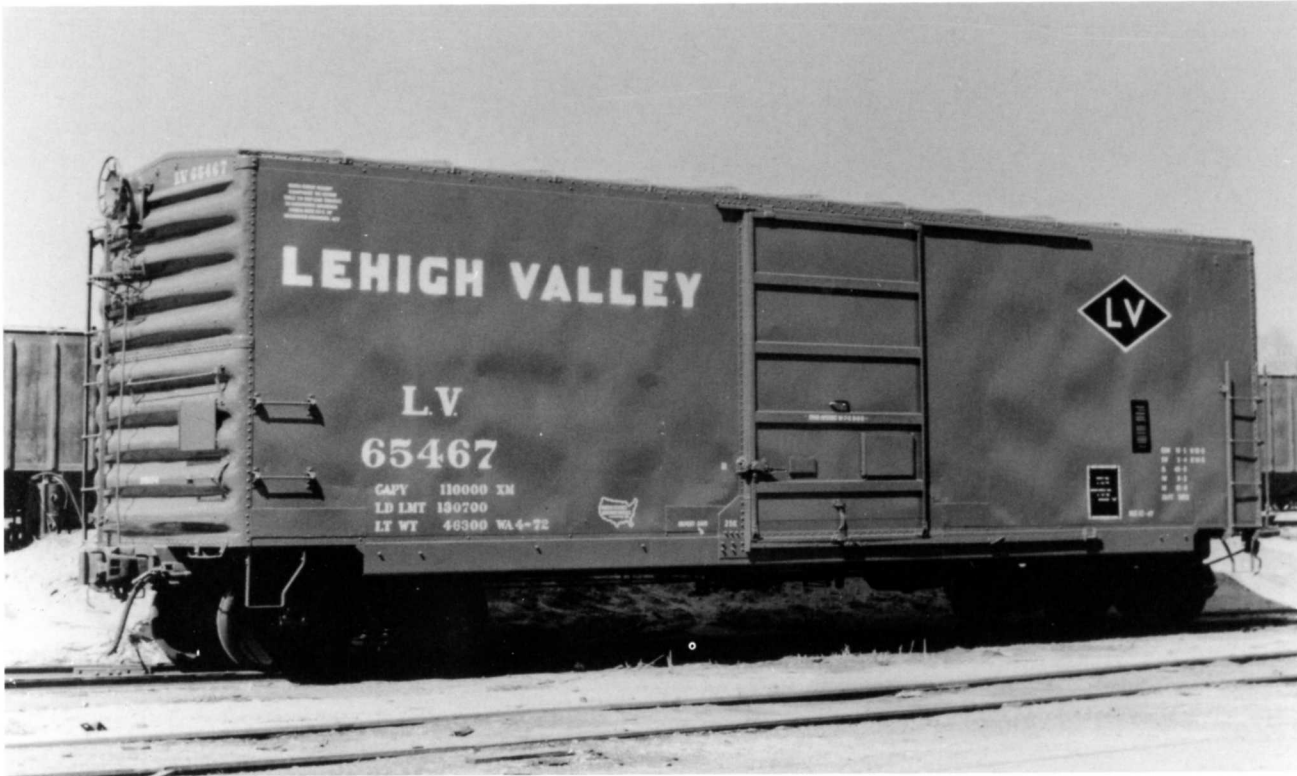
TOP Lehigh Valley 65467 is a part of a 100 car order from lot 1109. The records indicate 41 of these cars were taken from old New Haven box cars. Washington worked this order from December 1971 to April 1972. These cars were placed into the LV series 65400-65499. They were rated at 3903 cuft. and were equipped with 7-foot doors. This particular car was built in December 1947 and is green with white sten-
