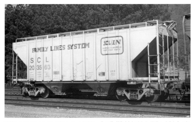
**PS 3000 cf design** (above). SCL 203563 is part of the SCL 203500-series built for cement and phosphate service. This car was built in August 1981 at Bessemer AL.
