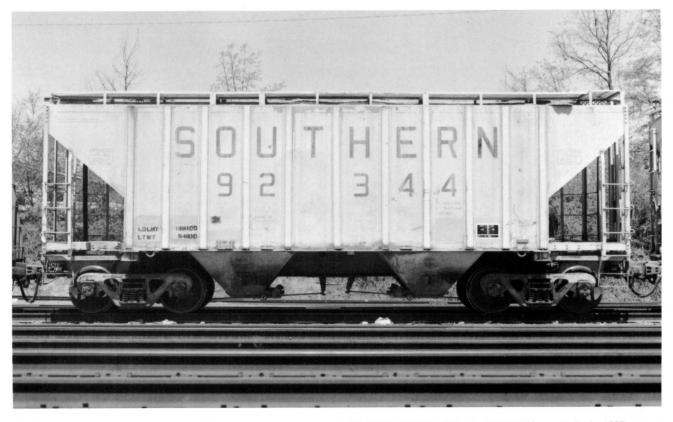
**PS 3000 cf design** (above). Southern 92344 was built in January 1981 as part of the series 92100-92399 (300 cars). Outside length, 41'11". The standard PS 3000 design has eleven side stakes, clerestory roof, and a straight side sill.
