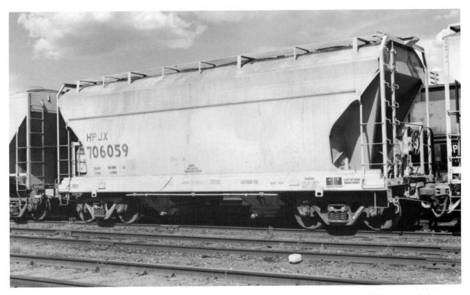
ACF 2970 cf design (above). HPJX 706059 is a former Missouri Pacific car. Originally from the TP 706000-706099 series. Built in March 1967 at Milton. Outside length, 39'8". Equipped with four 30" hatches and gravity outlets. HPJX is a reporting mark of HELM-Pacific Leasing.
