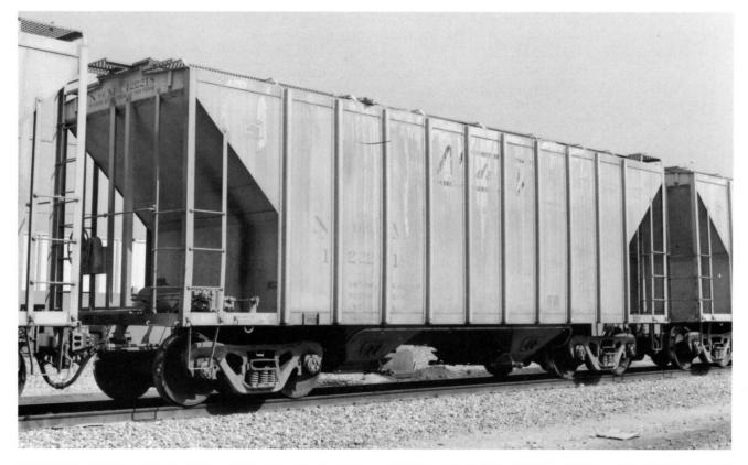
**CNCF 3000 cf design** (above). NdeM 122218 was built in 1986 as part of the NdeM 122000-122299 series. Though it looks a little like the PS design with the clerestory roof there are a number of differences including only ten ribs and a much different end platform arrangement.
