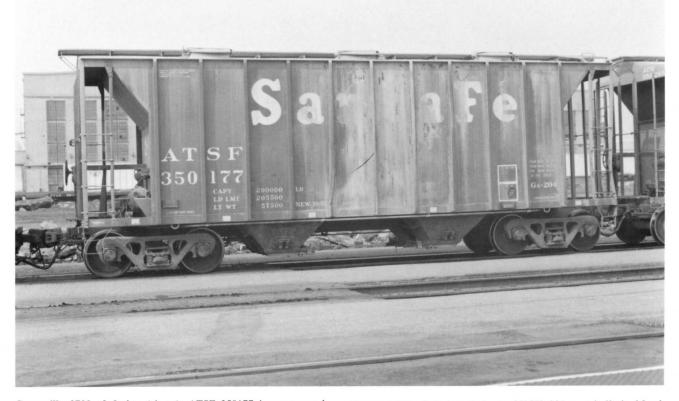
**Greenville 2700 cf design** (above). ATSF 350177 is pretty much the same design as the ANAX/NAHX 2917 cf car on the previous page. Both cars have almost the same features. Note that on this car the top end of the hopper falls just inside the ladder. On the ANAX car the top hopper ends go past the inner ladder stile. Outside length is 41'11".
