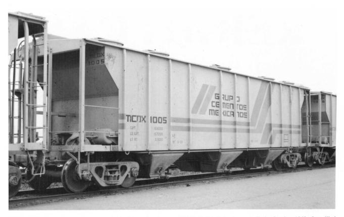
MCDX 1005 (above) is part of a series of fifty 70-ton three-bay covered hoppers being operated by Grupo Cementos Mexicanos (MCDX is a reporting mark of Sunbelt Cement). Number series, MCDX 1000-1049. Built in 1958. This car has a stencilled cubic-foot capacity of 2,927. Outside length, 49'11".
