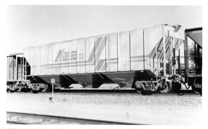
**CEMX 1107** (above). Not originally built as cement car - this three bay hopper was originally built for grain service. This is a PS 4427 design that is being used for cement service.
