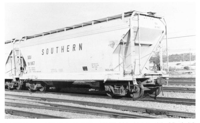
ACF 3300 cf design (above). SOU 91967 was built in 1976 as part of the SOU 91800-92099 series (300 cars). The 3300 cf design was a longer version of the 2980 cf design. These are primarily used for phosphate service. Outside length, 44'0". Painted here in the NS "Southern" scheme in October 1987.
