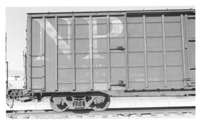
NP 2918. (Above). Left side detail showing stenciling indicating a cushioned underframe. Load limit on this car is  $181,200 \, \text{lbs} \, (263,000 \, \text{GRL} \, / \, a.k.a \, "100-ton" \, \text{car}).$
