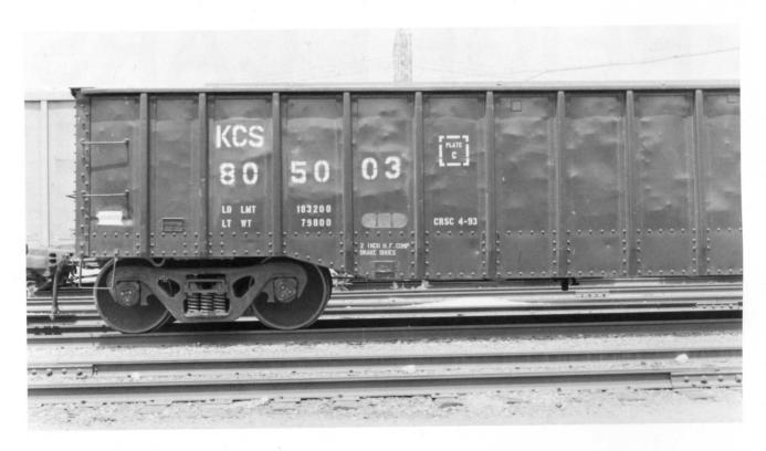
KCS 805003 (Above). Photo section 1 left side detail showing side posts numbers 1-9. Note the rivets at the floor line, bottom, and on side posts below floor line.
