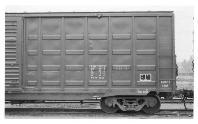
BPRR 1222 (Above). Right side detail. Each of the cars have a 5,050 cubic-foot capacity. These are 50'6" IL Plate B box cars.
