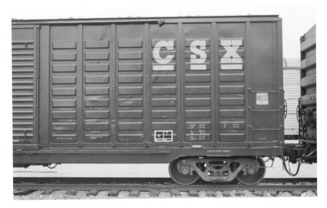
CSXT 507273 (Above). Right side detail. Note the stencilled capacity is 5,277 cubic-foot. The car was repaired as the Nashville shop in June 1994, then sent to ALRC for painting in August 1994.
