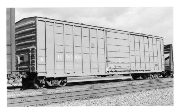
IC 563026 (Above) was built in September 1969. Again, four rows of waffles plus two in each of the upper corners (but, shifted over one panel). Note the recessed stamped corrugation end.
