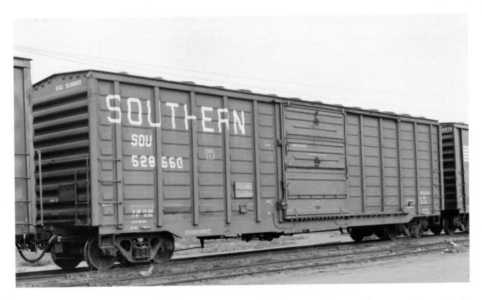
$\bf SOU~528660~(Above)$  was built by Pullman-Standard a part of the SOU 528300-529099 (800 cars). The car is a 50'6" IL Plate C box car. Note the door has been rebuilt with a new bottom replacing the original PS style corrugated door.
