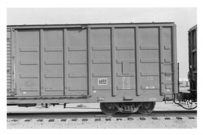
ATSF 611409. (Above). Detail of right side. Cubic-foot capacity is stencilled as 6,348. Note the large jack pad on the side sill just above the truck.
