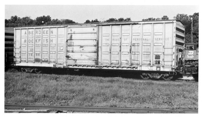
**AR 1599** (Above) is the last car of the series AR 1500-1599 (100 cars). It was built by SIECO's Ashland City plant in 1979. Note the four widely spaced rows of waffles. The ends are non-terminating (recessed) riveted to the sides (instead of welded). *Mike Foley* photo.
