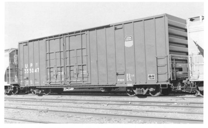
**UP 355047.** (Above). This is a 50'7" IL Plate F box car. FMC built 100 of these for the UP in 1974. Note the slightly recessed trucks, offset double plug doors, eleven post side, and 2/2/3 corrugated end. Capacity 6,189 cubic-foot. UP class BF-100-15. Series is UP 355000-355099.
