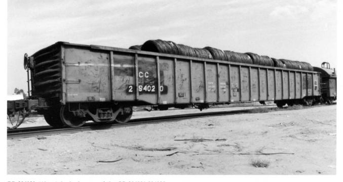
**CC 294020** (Above) is the last car of the CC 294001-294020 series. The car has a 65'6" IL. Inside height is 5'0". Inside width is 8'11". Note the top reinforcement angle and nineteen side posts. The middle 15 side posts are tapered at the bottom. The outer two side posts on each end have squared bottoms. All welded design.
