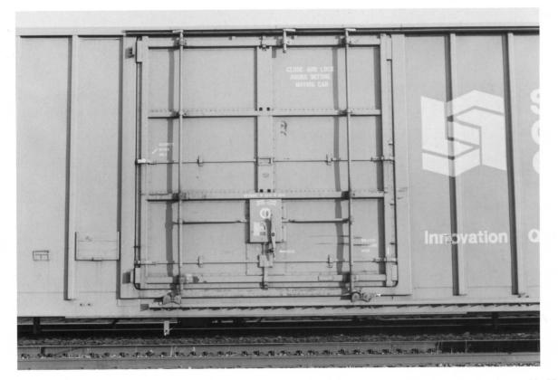
AG 1018. (Above). Detail of plug door and door area. This is a Youngstown (YSD) door. Note the frame surrounding the door goes just below the floor line. The bottom of the door itself is at the floor level.
