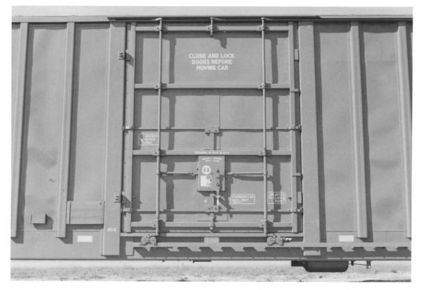
**BN 286157.** (Above). Detail of door area. Note how narrow the door looks especially with the massive door frame.
