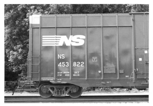
**NS 453822** (Above). Left side detail. Note the 286K GRL stencil and the load limit is correctly matched at 204,700 lbs (the load limit plus the light weight will total 286,000 lbs).
