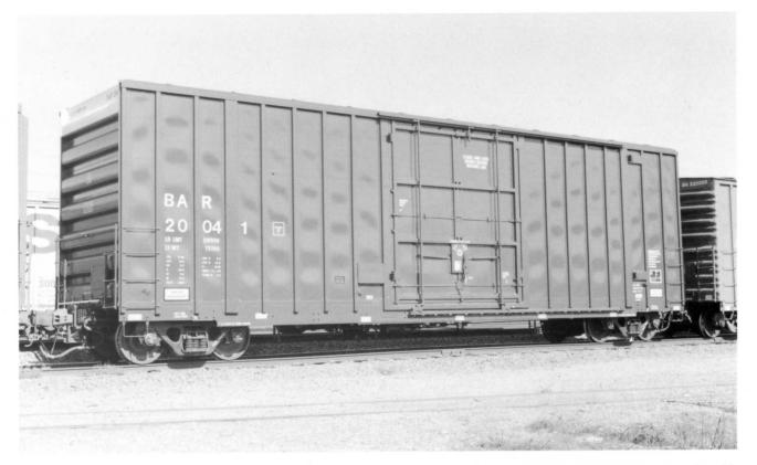
**BAR 20041.** (Above). Gunderson built this car in December 1994. Series, BAR 20000-20078 (79 cars). Livery is brown and white. These are 50'6" Plate F box cars. Door opening,  $10'0" \times 12'4"$  (WxH). Note the 2/2/3 end, fourteen side posts, and flat roof. Photographed in Colton, CA.
