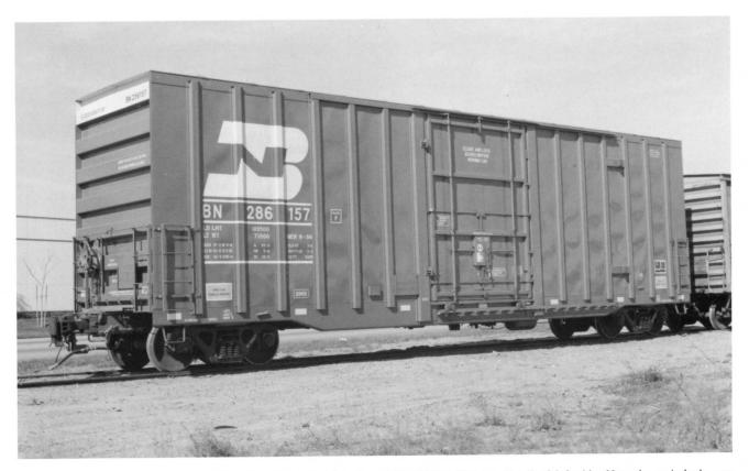
**BN 286157.** (Above). National Steel Car (Canada) built 150 of these for the BN in 1994. These are 50'6" IL Plate F box cars. Note the relatively narrow 10'0" x 12'4" (WxH) plug door. Note the 1/2/2/2 corrugated end, flat roof and twelve post side.
