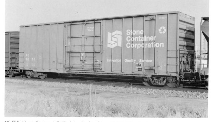
AG 1018. (Above) Gunderson built 50 of these for the A&G Railroad (Alabama) in 1990. Series, AG 1000-1049. Correct stencilled capacity is 5,757 cubic-foot (Registers show 5,505). Door opening,  $12'0" \times 12'0"$  (WxH). This car was built before Gunderson went to a wide side post. Note the 2/2/3 corrugated end, flat roof and twelve side posts.
