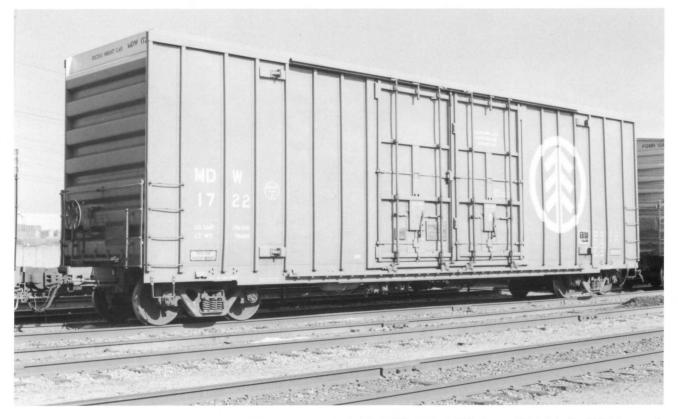
**MDW 1722.** (Above). This is a 50'6" IL Plate F box car. Door opening is  $16'0" \times 12'0"$  (WxH). Series MDW 1700-1799. The correct stencilled cubic-foot capacity is 6,241 (Registers list it as 6,246). This car was built in July 1976. Note flat roof, 2/2/3 corrugated ends and twelve post sides.
