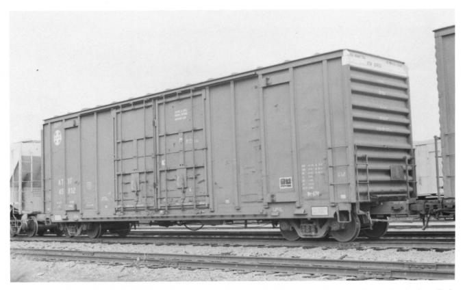
**ATSF 45932.** (Above). Pullman-Standard built 100 of these in 1974. These are 50'6" IL Plate F box cars. Door opening, 16'0" x 12'0" (WxH). Santa Fe class, Bx-170. Series, ATSF 45900-45999. Note the four wide side posts (ribs) to either side of doors. Pullman-standard rolled 3/3/5 ends. Flat roof. Cubic-foot capacity, 6196.
