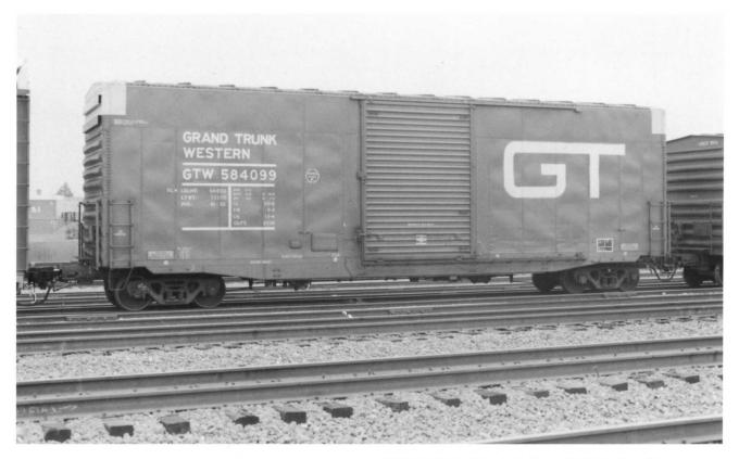
**GTW 584099** (Above) is a rebuilt box car that has had its roof raised to Plate F clearance height. GTW's Port Huron Shops (PHS) rebuilt 159 of these in 1992 from the GTW 309000-309299 series (Pullman-Standard 1970). Capacity 6,635 cubic-foot with a starred load limit of 54,000 lbs!
