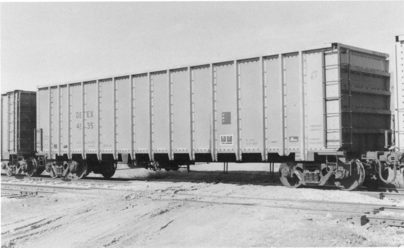
DEEX 4935. (Above). Built in January 1991. Cubic-foot capacity remains 4,325. Photographed in the Powder River Basin of Wyoming during August 1995.
