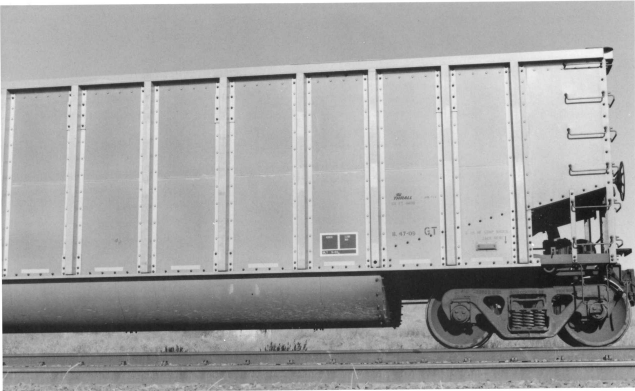
SATX 9065. (Above). The two photos on this page show the different slope sheet versions. This one has an angle slope sheet. Built in 1992. Capacity is 4,400 cubic-feet.
