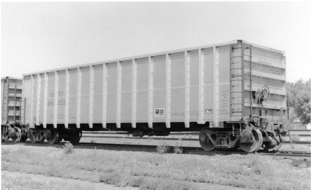
CHTT 640033. (Below). This car was built in December 1990. It still has the 47'0" IL but is a little smaller than the previous 4325's with this one having a 4,200 cubic-foot capacity. The cars were later transferred to Commonwealth Edison Company (CWEX). CHTT = Chicago Heights Terminal Transfer part of the Missouri Pacific / Union Pacific Railroad.
