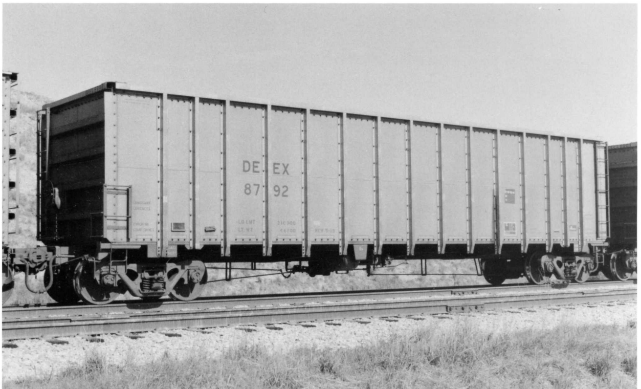
DEEX 8792. (Below). An aluminum-bodied coal gondola. Built in May 1989. Note the barely visible horizontal groove in the middle of the side sheet - something that would show on Thrall's coal gondolas built through the time of this writing. IL changes to 47'0" and cubic-foot capacity is 4,325. However, these cars still sport a 53'1" frame.
