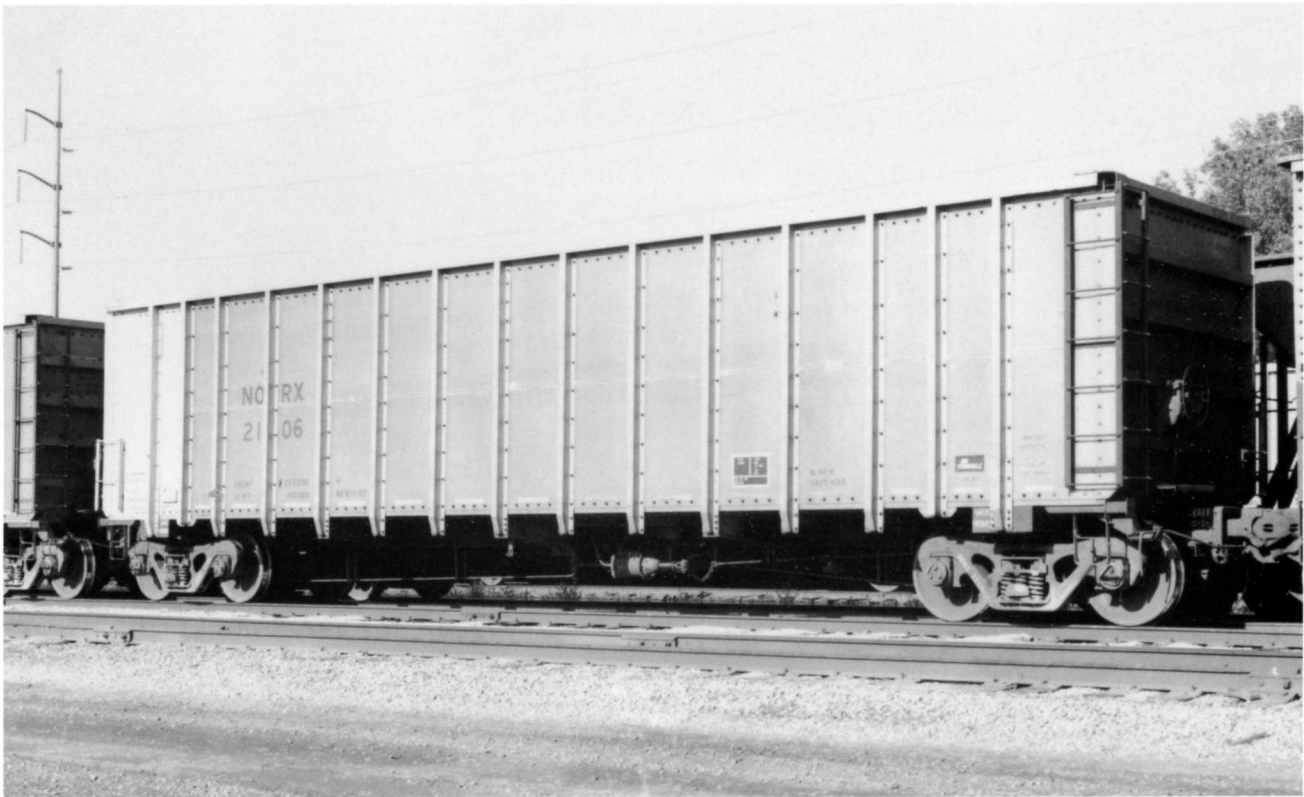
NORX 2106. (Below). Built in November 1989. This aluminum-bodied coal gondola continues the 47'0" IL, 4,325 cubic-foot capacity and 53'1" outside length. Series is NORX 2000-2129 (130 cars). NORX = Northern Indiana Public Service Company based in Hammond IN.
