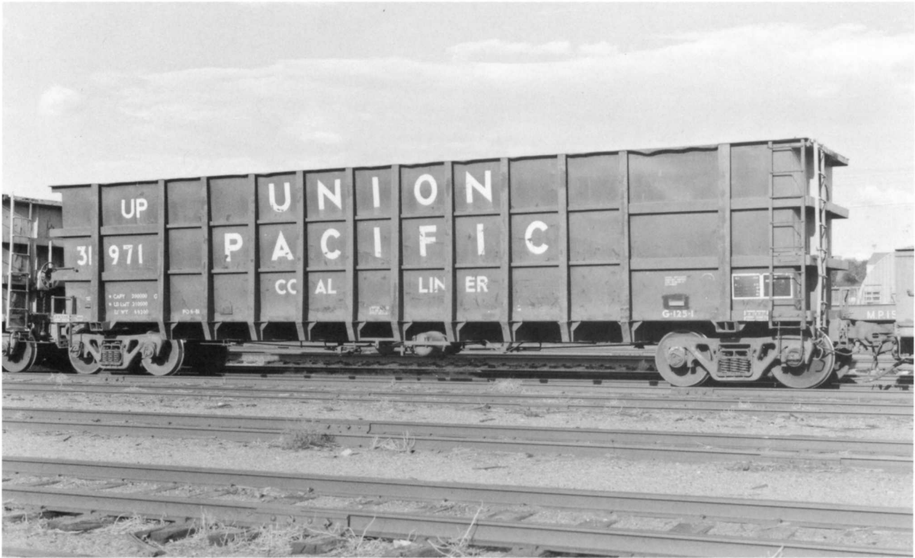
UP 31971. (Above). Thrall built these 125-ton trucked coal gondolas in 1969. Each car had a 3,850 cubic-foot capacity. UP class G-125-1. Note the narrower horizontal "ribs" extending from the second vertical post from each end. Painted in Pocatello, ID during June 1981. Photographed at Laramie, WY during August 1995.
