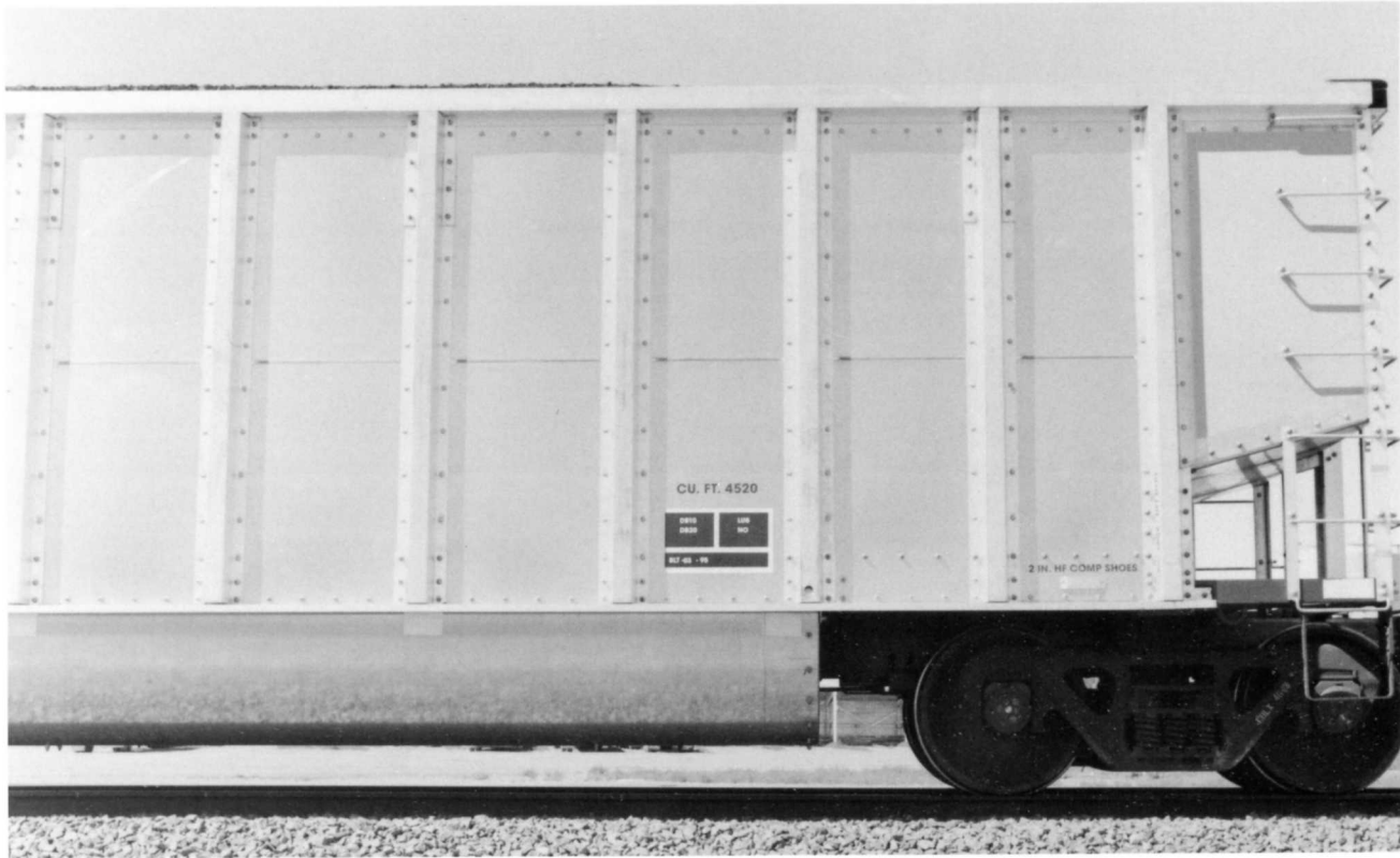
COLX 4649. (Above). Center side detail. The massive rectangular side posts have paired fasteners from top to bottom. Note the three side posts with the interior cross-brace plates (top and bottom).
