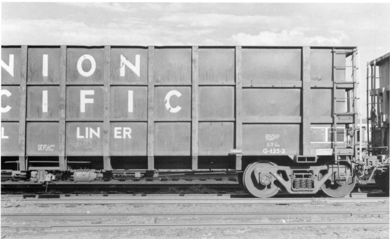
UP 32054. (Above). Left side detail. Relatively little difference between this class and the previous class. However, note the wider bolster and lack of reinforcement gussets on the lower part of the side posts. Painted in Pocatello, ID during April 1981. Note the rare use of a "return to" on a coal car.
