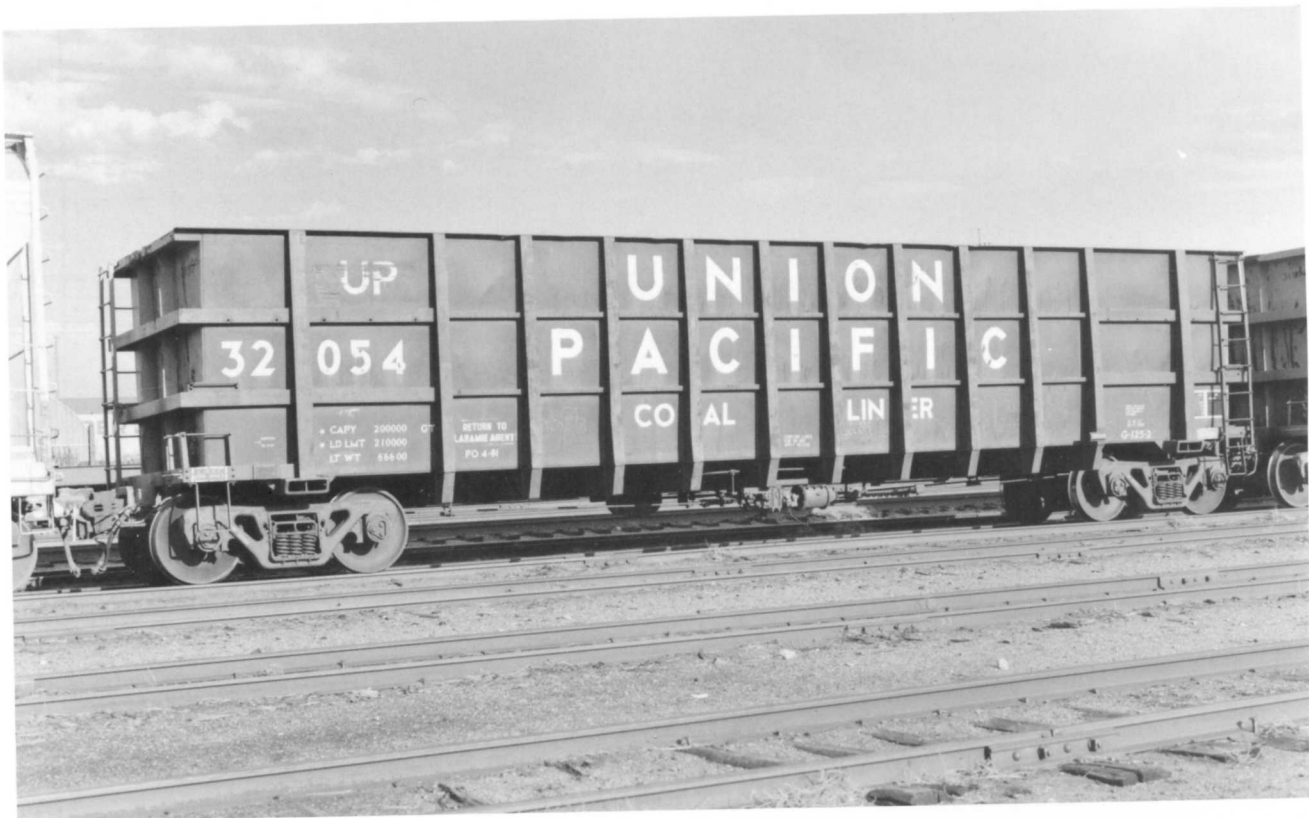
UP 32054. (Below). Thrall built the second class of 125-ton cars for the Union Pacific in 1970. Each car had a 3,700 cubic-foot capacity. Series is UP 32000-32099 (100 cars). 46'11" IL (interior length) was to become a standard for Thrall high-sided coal gondolas.
