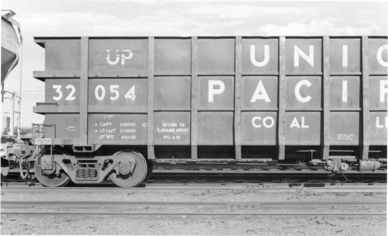
UP 32054. (Above). Left side detail. Relatively little difference between this class and the previous class. However, note the wider bolster and lack of reinforcement gussets on the lower part of the side posts. Painted in Pocatello, ID during April 1981. Note the rare use of a "return to" on a coal car.
