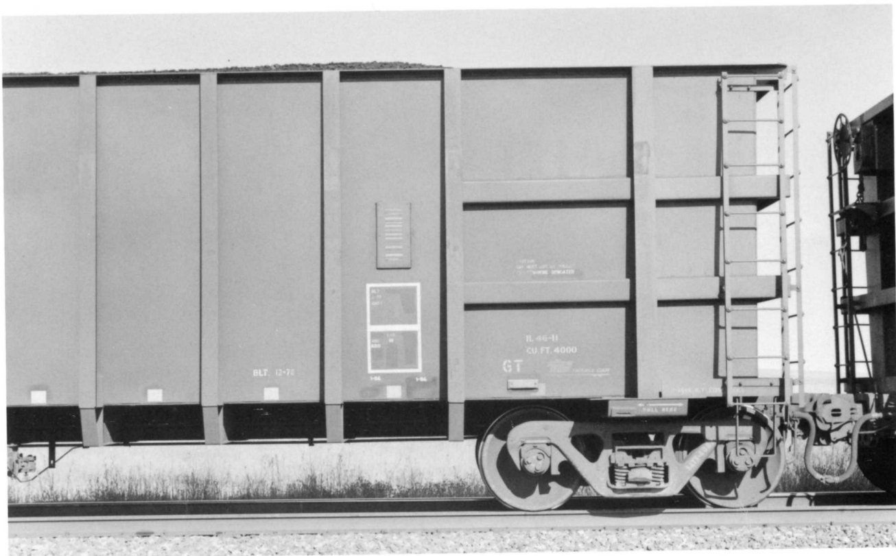
SATX 4082. (Above). Center side detail. Reflectors are a later add on. Photographed in the Powder River Basin of WY during August 1995.
