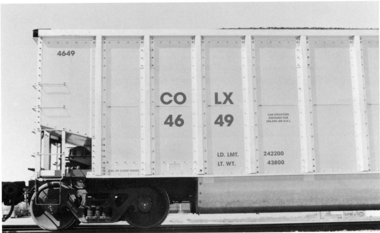
COLX 4649. (Above). Thrall's aluminum-bodied bathtub coal gondola still has that thin horizontal groove along the side. Note the similarity to Johnstown America's bathtub design. Series is COLX 4569-4715 built in 1995. COLX = one of the reporting marks for Wisconsin Power and Light Company. 5
