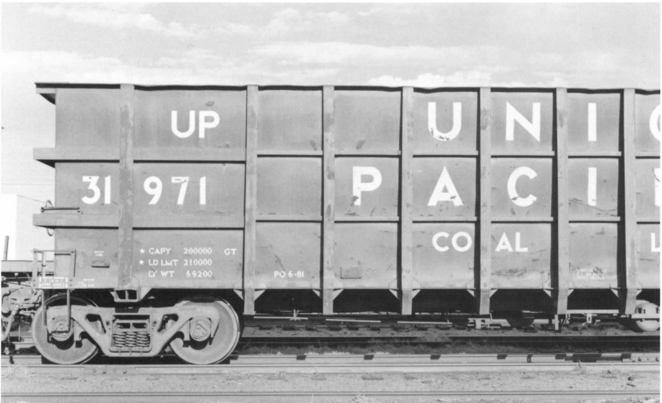
UP 31971. (Above). Thrall built these 125-ton trucked coal gondolas in 1969. Each car had a 3,850 cubic-foot capacity. UP class G-125-1. Note the narrower horizontal "ribs" extending from the second vertical post from each end. Painted in Pocatello, ID during June 1981. Photographed at Laramie, WY during August 1995.
