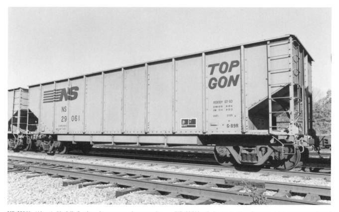
**NS 29061.** (Above). Norfolk Southern began converting a number of old coal hopper into coal gondolas by replacing the original hopper body with a new gondola body. This one was rebodied in July 1993 by the NS Roanoke, VA shops. The cars are gray with black lettering. Photographed in Birmingham, AL during May 1994.
