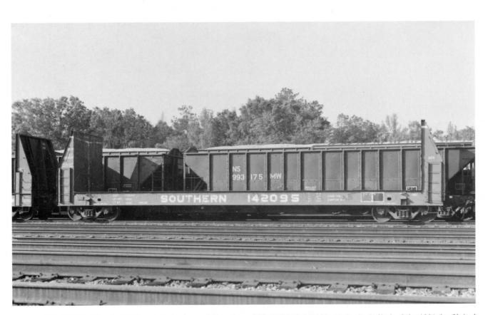
**SOUTHERN 142095.** (Above). Still in original paint as delivered from the builder (Greenville Steel Car) in July 1980. This is a 50-foot Plate C pulpwood car. Series, Southern 141300-142099. The remaining cars would become NS class FS-95 after the merger. Photographed in Crewe, VA during May 1995.
