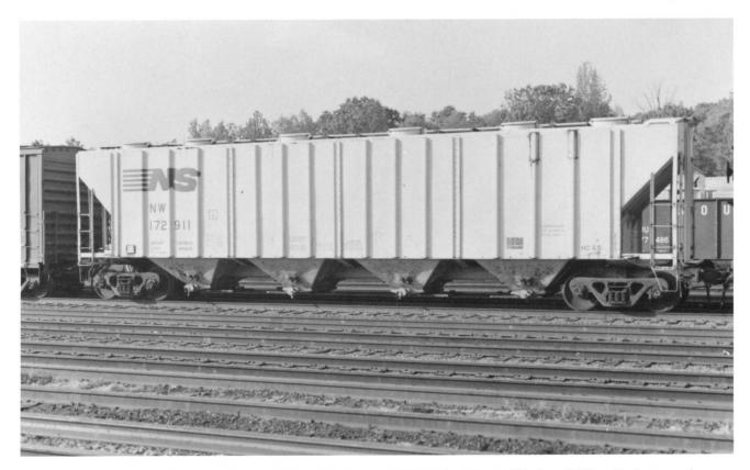
**NW 172911.** (Above). This huge 100-ton 5,200 cubic-foot capacity covered hopper was built in 1967 by N&W's Roanoke, VA shop. Series, NW 172900-172999. N&W/NS class HC-65. Photographed in Crewe, VA during May 1995.
