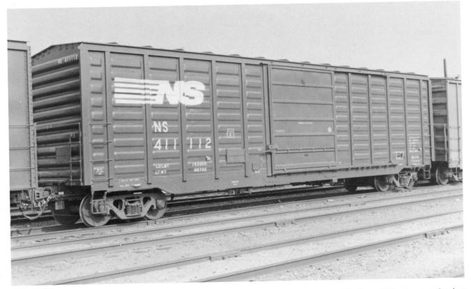
**NS 411112.** (Above). NS has a huge fleet of 70-ton box cars such as this one. This car was originally built as part of the SOU 530500-531499. Built in 1978 by Pullman-Standard's Bessemer, AL plant.
