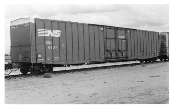
**SOU 9728.** (Above). Southern had some very interesting freight cars - none the least is this 84'4" IL Plate F+ double-plug door box car. The car has a 10,036 cubic-foot capacity, 75-ton load limit (on 100-ton trucks) and is equipped with Pullman's very own 30 inch cushioning device.
