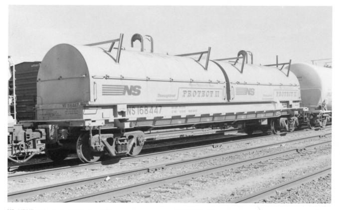
**NS 168447.** (Above). Norfolk Southern's *Protect II* uses insulated covers to reduce temperature change. This car weighs in at 67,800 lbs or about 7,000 lbs heavier than similar cars with non-insulated covers. This car was built in June 1993 by Thrall Car. NS class CS-14. NS 168400-168499. Equipped with Keystone E-15G-B cushioning.
