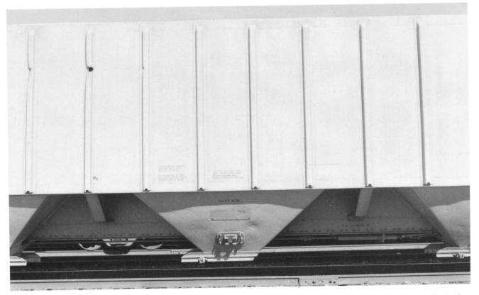
**NS 252101.** (Above). Center section of car side. Caution statements warn operators to close hatches before moving car and having at least one hatch open during unloading.
