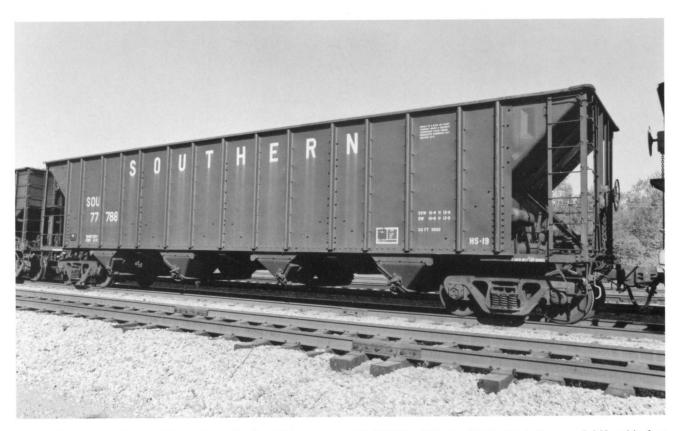
**SOU 77788.** (Above). Built in 1971 by Greenville Steel Car as part of Southern's 77200-77799. Norfolk Southern's influence is shown here with the repaint and new class HS-18. These are 3,600 cubic-foot capacity quadruple hoppers used for coal transport. Photographed in Birmingham, AL May 1994.
