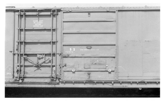
**SOU 551370.** Center section detail. This shows the combination door arrangement of this car. The plug door on the left is an unfamiliar design to me.
