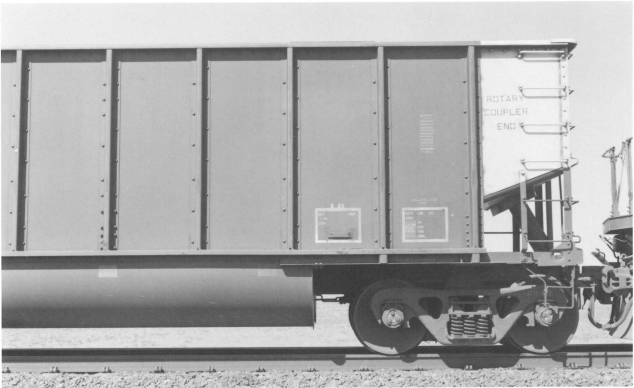
SFIX 607. (Above). Right side view. The A-end with its rotary coupler. The cars have black bodies with white end panels signifying the rotary coupler.
