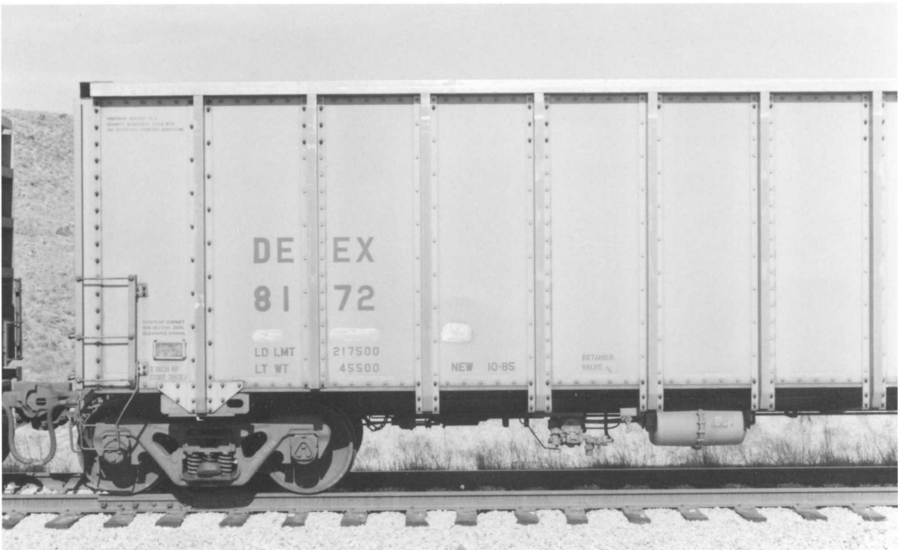
DEEX 8172. (Above). Aluminum-bodied 1985 built Greenville Steel 4,320 cubic-foot design. Series is DEEX 8101-8710 (610 cars). Thirteen ribs. DEEX = Detroit Edison Company based in Detroit, MI.
