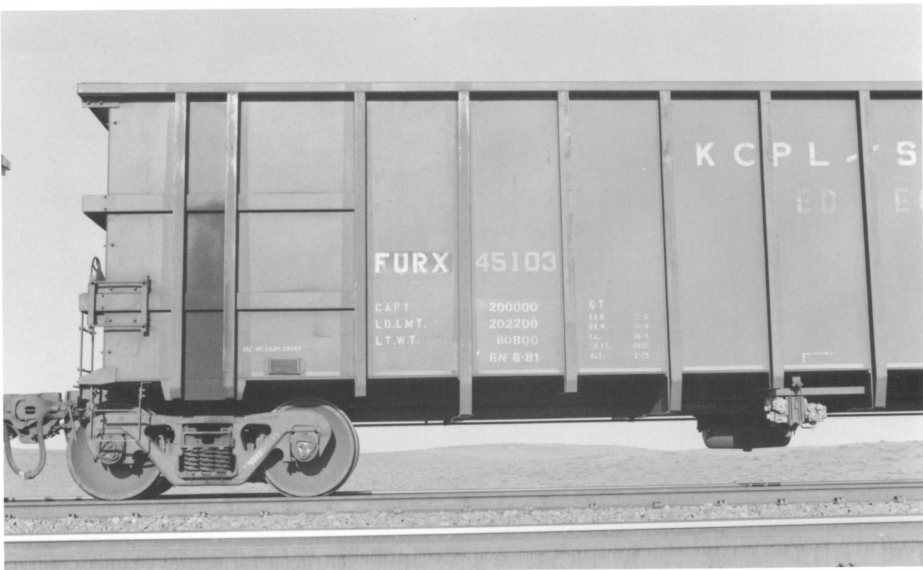
FURX 45103. (Above). Steel-bodied 1979 built Darby Car 4,000 cubic-foot design. Most of us think of Thrall Car's design when it comes to wrap-under rib-side coal gondolas. However, Darby Car of Kansas City, Kansas built a number of this type, too. Series is FURX 45001-45240. These were originally built as KCLX 45001-45240. FURX = First Union Rail based in Rosemont, IL.
