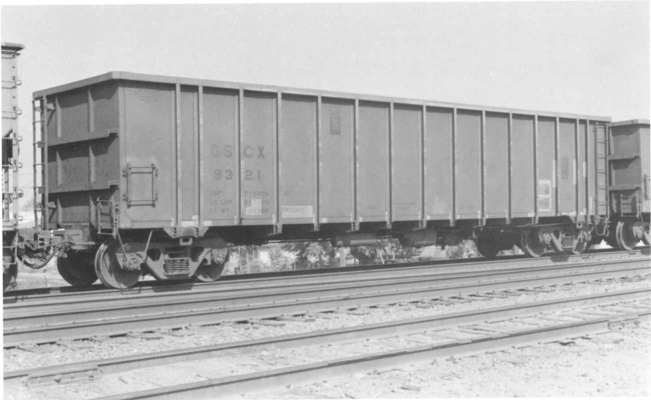
GSCX 9321. (Below). Note how it incorporates elements of a wrap-under design.
