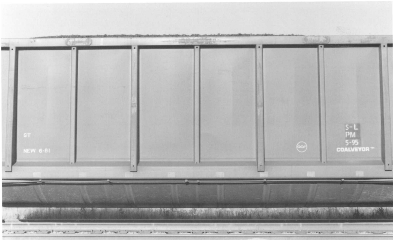
WPSX 255. (Above). Close-up of left side. Note how the ribs alternate in width. The wider ribs go over the lower side sill to the middle. The narrower ribs only go from the bottom of the top chord to the top of the lower side sill.
