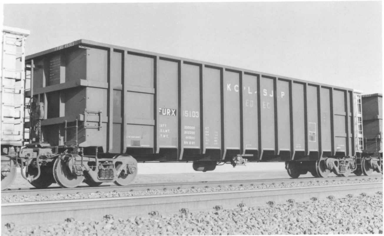
FURX 45103. (Below). Left side detail. Note the dual vertical ribs at the end (Thrall only has one) and the differing heights of the ribs (noticeable by looking along the bottom - Thrall's were all the same height).
