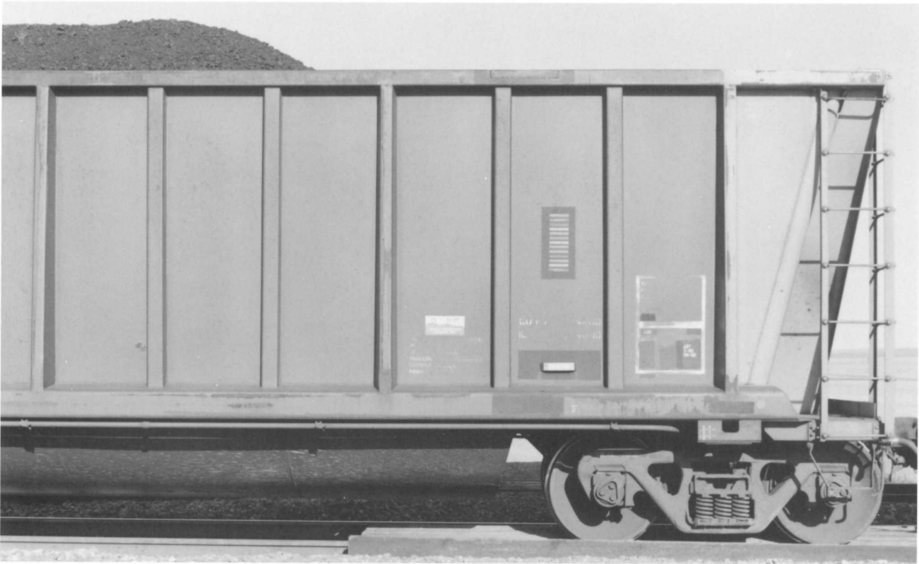
UFIX 19005. (Above). Right side view. The A-end shown here has the full height ladder and rotary coupler end. Note how Berwick's side sill is angular cut at the end. Series is UFIX 19001-19110.
