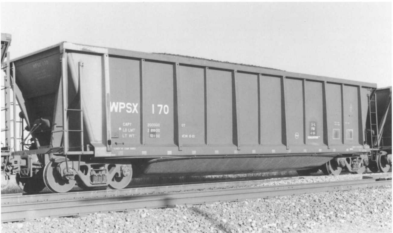
KCLX 7372. (Above) Steel bodied 1980 built ACF 4,240 cubic-foot design. Series KCLX 7371-7491. OL 53'1". This car has double rotary couplers. There were four designs of these early bathtub gondolas that looked very much alike, ACF, Berwick Thrall and Ortner (the Bethlehem/Johnstown cars have more conventional "hopper-like" ends).
