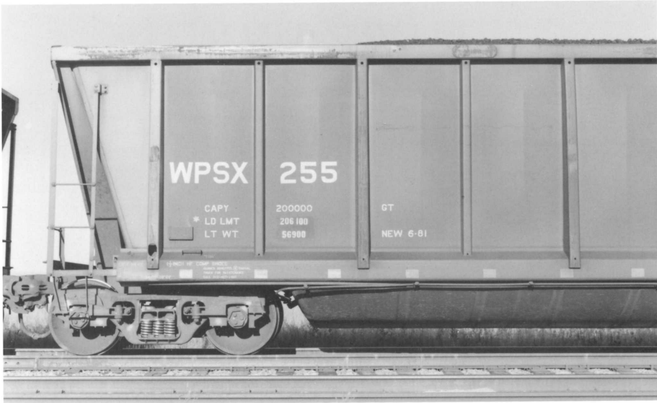
WPSX 255. (Below). Middle side view. Clean all-welded lines. ACF called this the Coalveyor.
