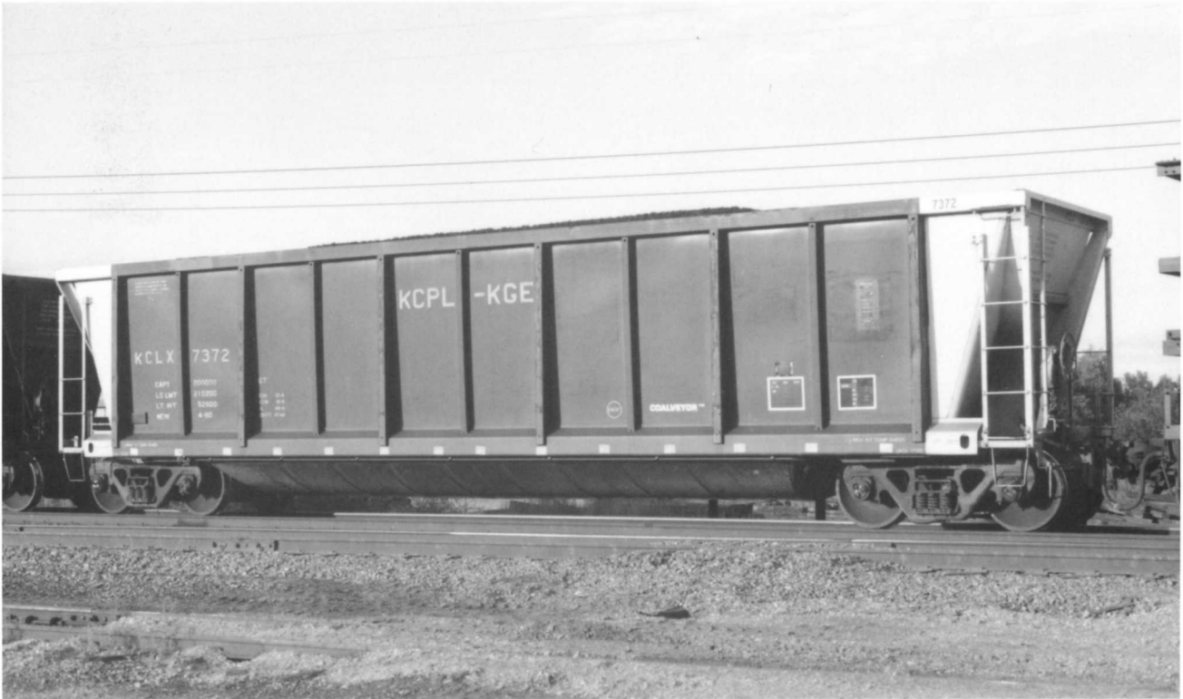
KCLX 7372. (Above) Steel bodied 1980 built ACF 4,240 cubic-foot design. Series KCLX 7371-7491. OL 53'1". This car has double rotary couplers. There were four designs of these early bathtub gondolas that looked very much alike, ACF, Berwick Thrall and Ortner (the Bethlehem/Johnstown cars have more conventional "hopper-like" ends).
