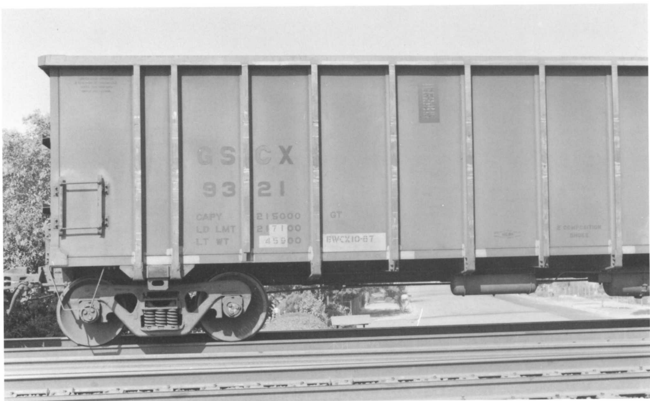
GSCX 9321. (Above). Aluminum-bodied 1972 built Greenville Steel 3,850 cubic-foot design. OL 52'1". Series is GSCX 9000-9344 (345 cars). A car way ahead of its time with its aluminum body - though not the earliest. GSCX = GATX/GLC Leasing Corporation.
