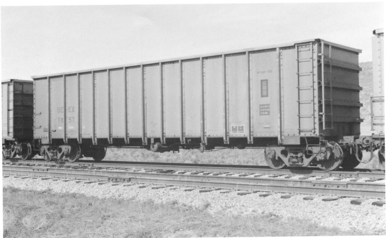
CEPX 1343. (Above). Steel-bodied 1979 built Pullman-Standard 4,000 cubic-foot design. Pullman-Standard also had their version of a high-sided coal gondola. Thirteen ribs. Note the traditional Pullman-Standard end architecture. Series is CEPX 1000-1358. CEPX = Cajun Electric Power Cooperative, Inc.
