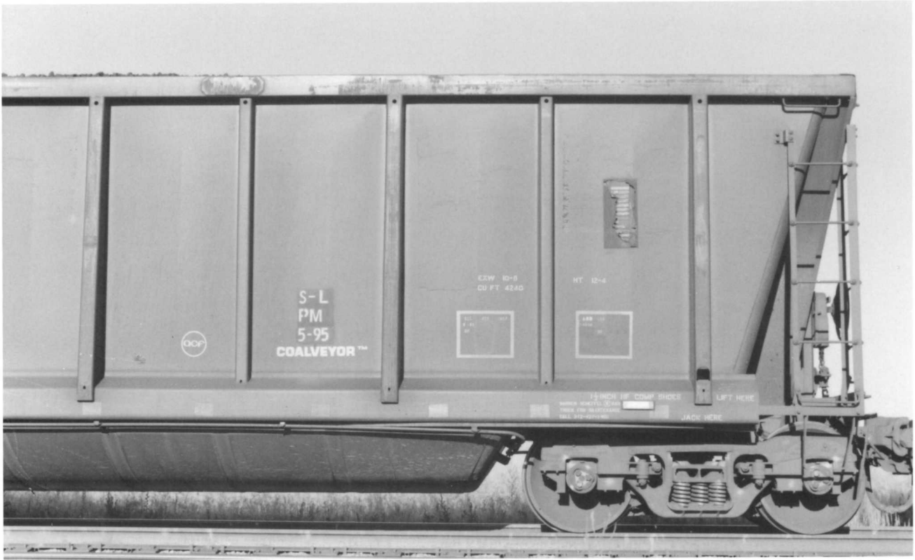
UFIX 7035. (Below). Steel-bodied 1978 built Berwick 4,200 cubic-foot design. Compare to the ACF design. Series is UFIX 7001-7110 (110 cars). UFIX = Houston Lighting & Power Company based in Houston, TX.
