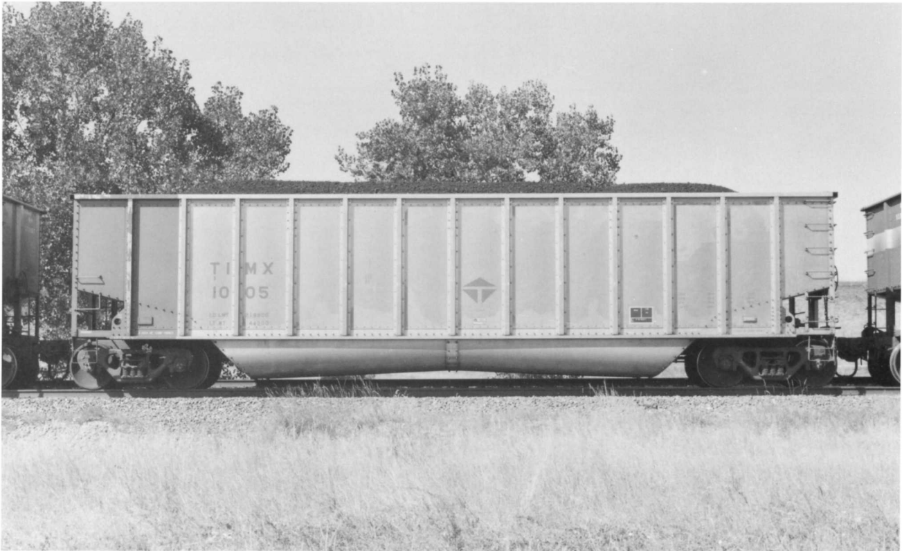
TIMX 1005. (Above). Aluminum-bodied 1992 built Trinity 4,400 cubic-foot design. Trinity's version of the bathtub gondola has center-to-ends taper as can clearly be seen in this side view. The big "T" in the middle is Trinity Industries logo.
