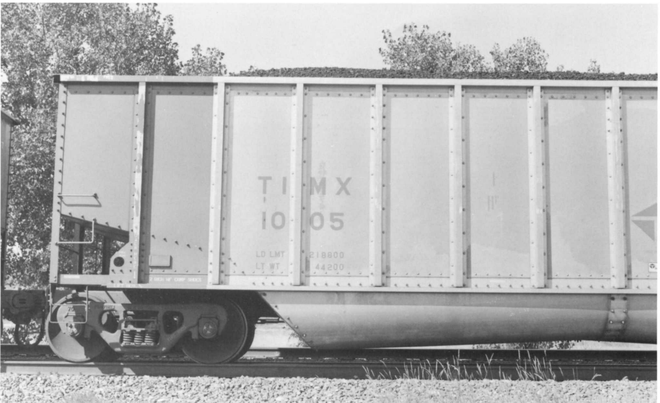
TIMX 1005. (Above). Aluminum-bodied 1992 built Trinity 4,400 cubic-foot design. Trinity's version of the bathtub gondola has center-to-ends taper as can clearly be seen in this side view. The big "T" in the middle is Trinity Industries logo.
