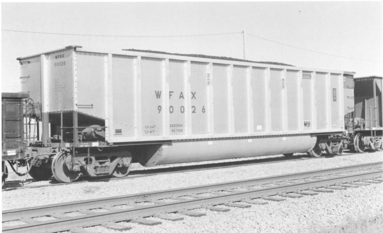
WFAX 90026. (Below). Aluminum-bodied 1990 built Bethlehem Steel 4,300 cubic-foot design. Series is WFAX 90000-90119 (120 cars). Livery is aluminum body with red rotary end panel and black lettering. WFAX = Western Fuels Association, Inc based in Lakewood CO.
