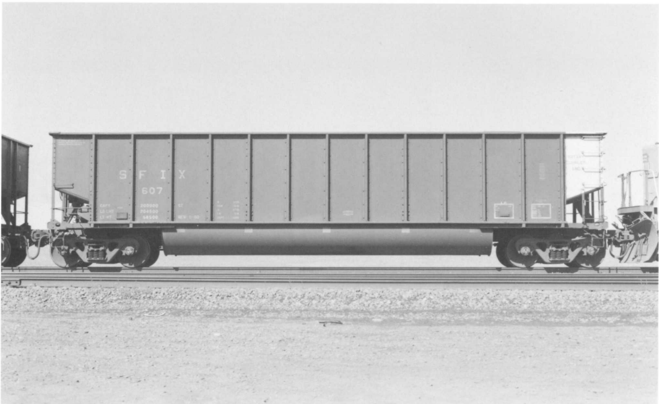
SFIX 607. (Below). Steel-bodied 1980 built Bethlehem Steel 4,000 cubic-foot design. This car could be easily seen as hopper because of the typical hopper-like characters (exterior ribs, ends etc). Series is SFIX 594-1336. SFIX = System Fuels, Inc based in Beaumont TX. OL 53'1"
