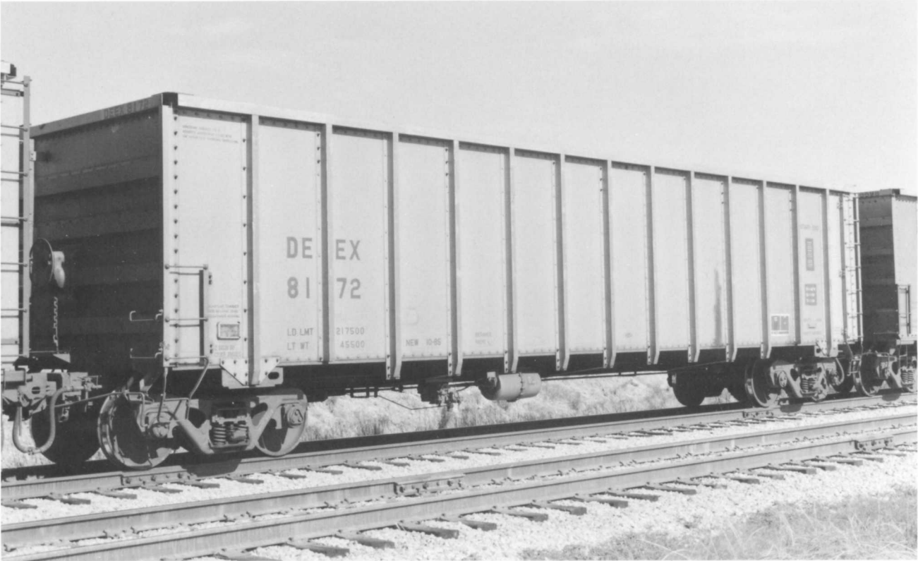
DEEX 8172. (Above). Aluminum-bodied 1985 built Greenville Steel 4,320 cubic-foot design. Series is DEEX 8101-8710 (610 cars). Thirteen ribs. DEEX = Detroit Edison Company based in Detroit, MI.
