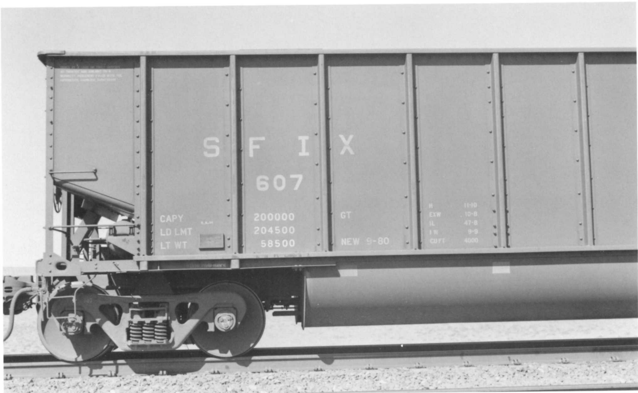
SFIX 607. (Below). The location of the two cross braces can be seen in this view of the middle side. The ribs second from each end in this photo have the cross-braces (note rivet patterns!!)
