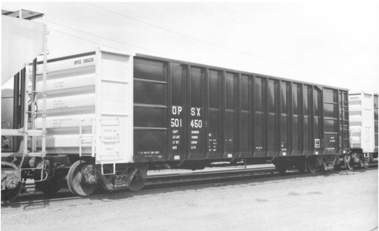
OP SX 501450. (Below). Steel-bodied 1979 built FMC 4,000 cubic-foot design. Series is OPSX 500011-505111 (511 cars). FMC's high-side gondola design has traditional modern "square" gondola/boxcar ends. FMC also had a bathtub gondola design. OPSX = Public Service Company of Oklahoma based in Tulsa, OK.
