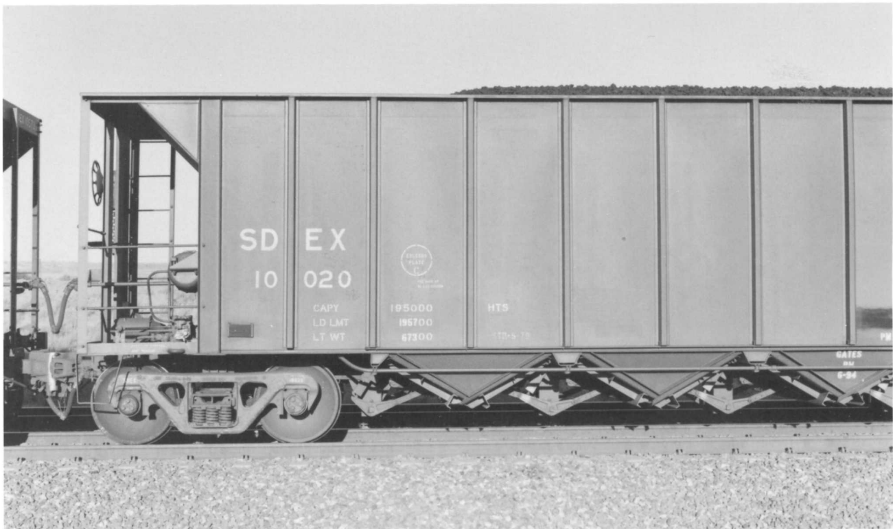
SDEX 10020. (Below). Close-up of the left side reveals the clean lines of an all welded cars. Note arms between bays that open gates. Actual load limit on these 263,000 GRL cars averaged closer to 98-tons.
