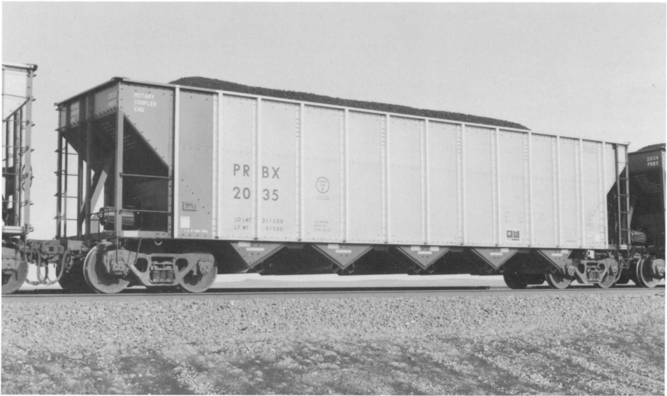
PRBX 2035. (Above). Aluminum-bodied 1994 built Johnstown America 3,990 cubic-foot design. OL 53'1".
