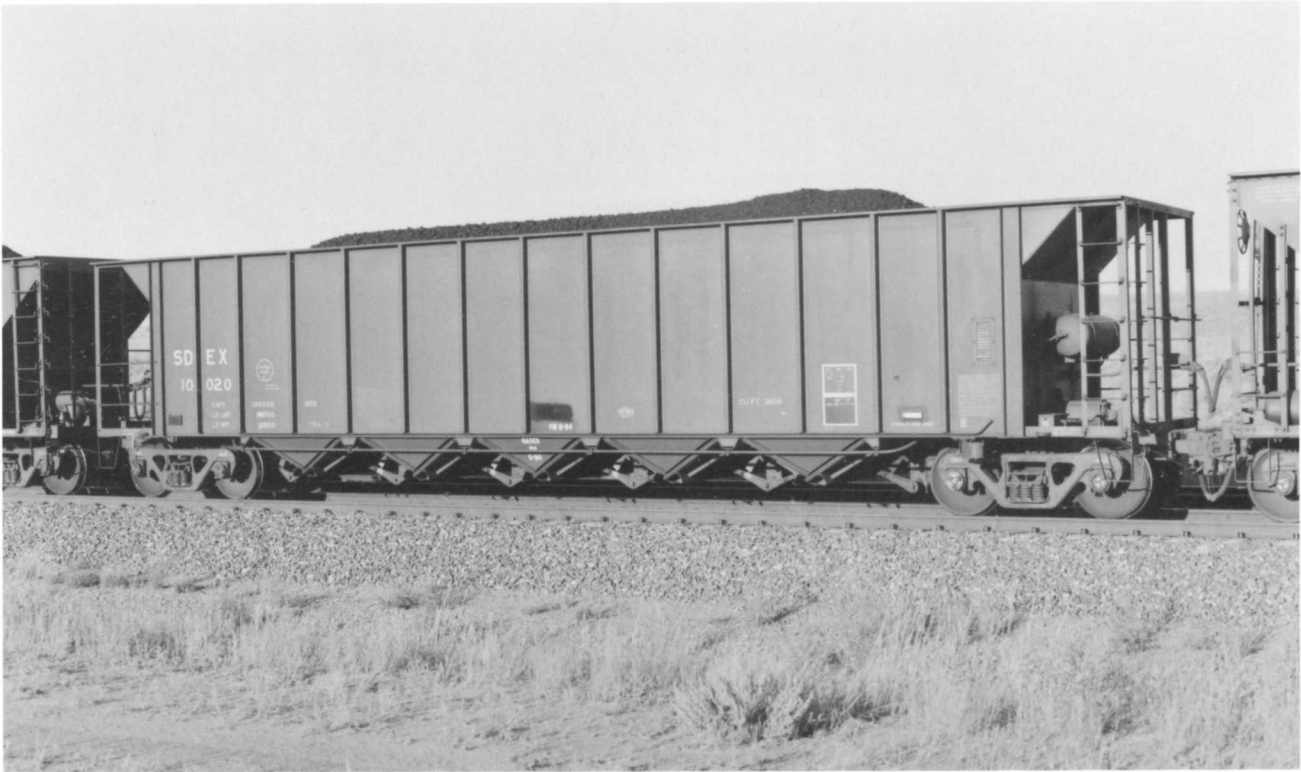
SDEX 10020. (Below). Close-up of the left side reveals the clean lines of an all welded cars. Note arms between bays that open gates. Actual load limit on these 263,000 GRL cars averaged closer to 98-tons.
