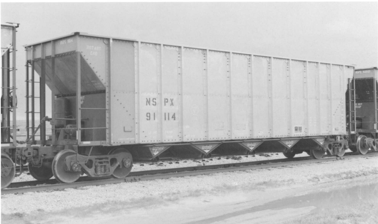
NSPX 91114. (Below). Aluminum-bodied 1992 built Trinity 4,155 cubic-foot design. Pretty much similar to the CRL car except this design is three inches higher. NSPX 91001-91220. NSPX = Northern States Power Company based in Minneapolis, MN.
