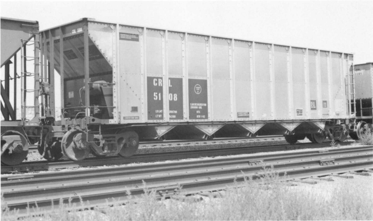
CRL 5108. (Above). Aluminum-bodied 1992 built Trinity 4,028 cubic-foot design. One can see the continued design evolution from the ACCX cars. This one is Plate F+ and has the pick-up shoe actuators. CRL = Chicago Rail Link.
