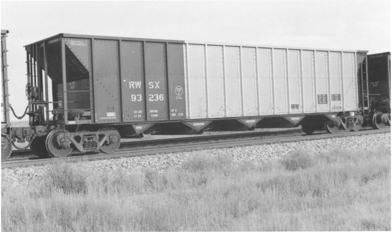
RWSX 93198. (Above). Aluminum-bodied 1993 built Trinity 4,200 cubic-foot design. This sixteen rib car is five-foot longer than the standard Trinity quick-dump cars ( cf ACCX, CRL, NSPX). Series is RWSX 93001-93946 (946 cars).
