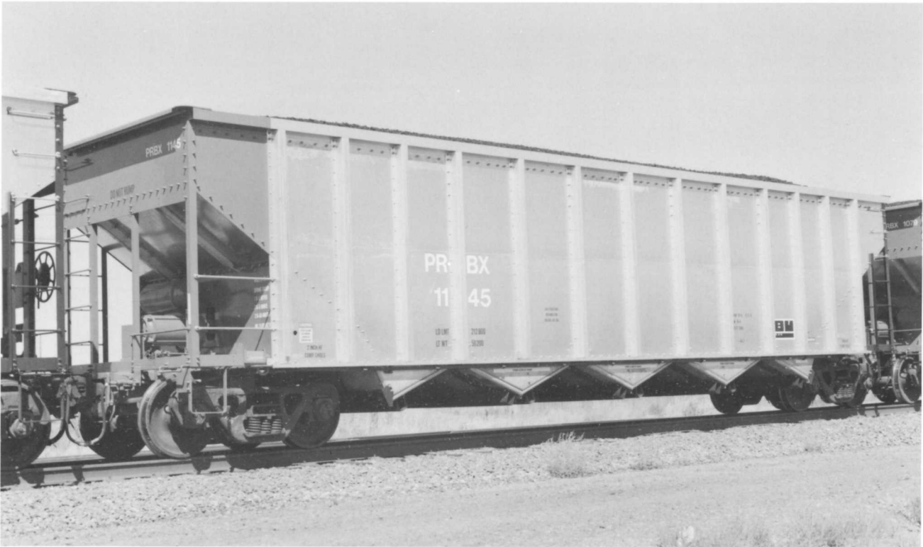
PRBX 1145. (Above). Aluminum-bodied 1994 built Thrall Car 3,980 cubic-foot design. Thirteen ribs. OL 53'1". Series is PRBX 1001-1240.
