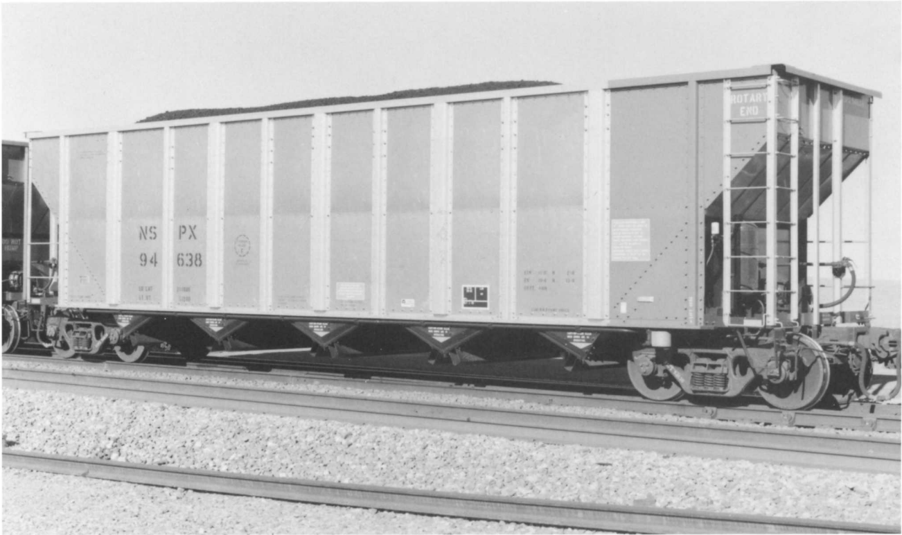
NSPX 94638. (Above) Aluminum-bodied 1995 built Trinity 4,416 cubic-foot design. OL 53'1". Series is NSPX 94501-94735 (235 cars).
