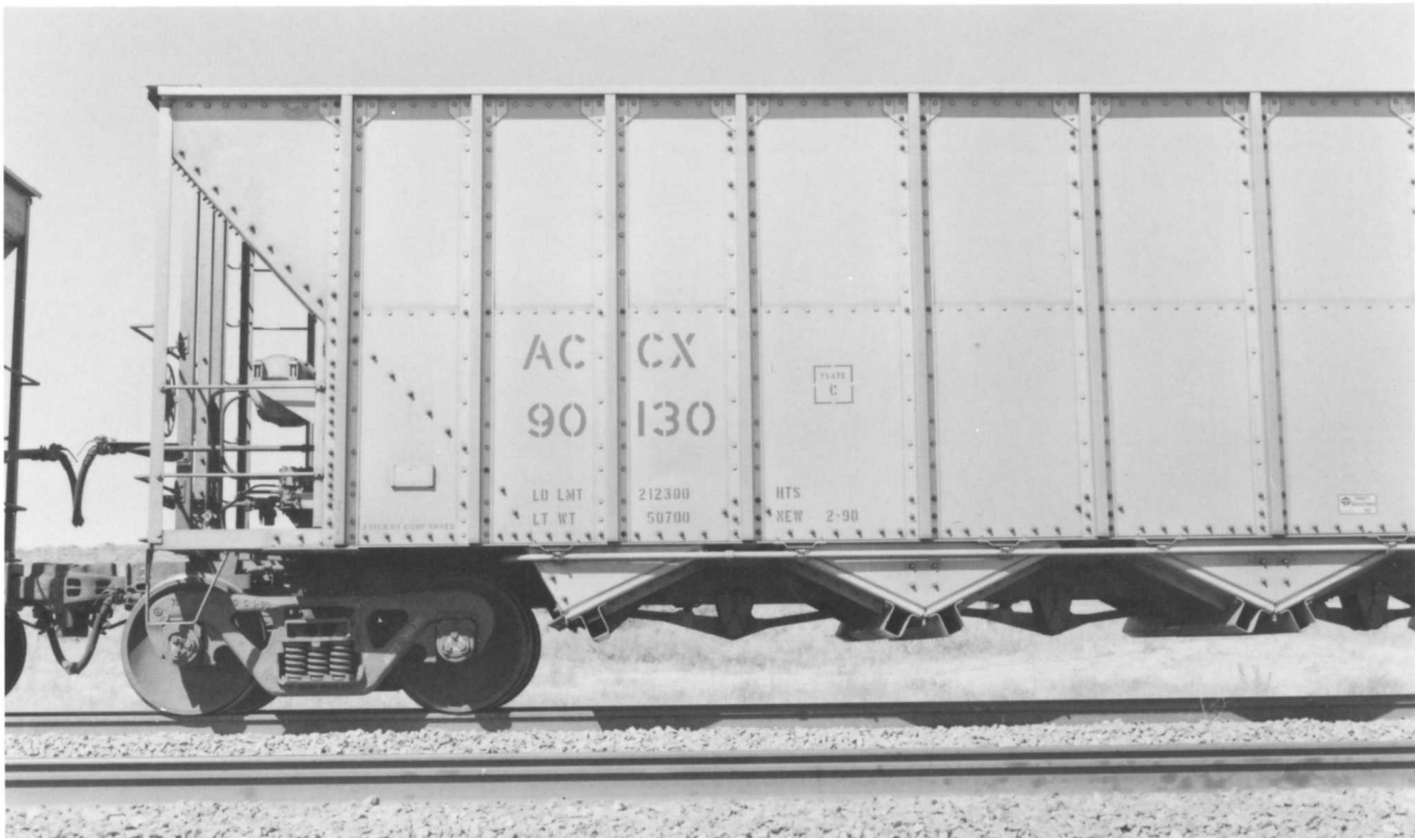
ACCX 90130. (Above). Aluminum-bodied 1990 built Trinity 4,000 cubic-foot design. The horizontal rivet line is more obvious on this car ( cf IPPX 386). Elements of the Ortner design become apparent including the "curved" lower drop of the end sheets into the end hoppers.
