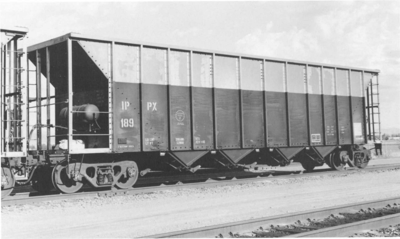
SDEX 10229. (Above). Steel-bodied 1978 Pullman-Standard 4,000 cubic-foot design. Pullman-Standard's design was shorter (53'1") but taller (13'10") than its Ortner counterpart. Note thirteen "riveted" rib side design. Series is SDEX 10131-10260. SDEX = Swindell-Dressler Energy Supply Company based in Amarillo, TX.
