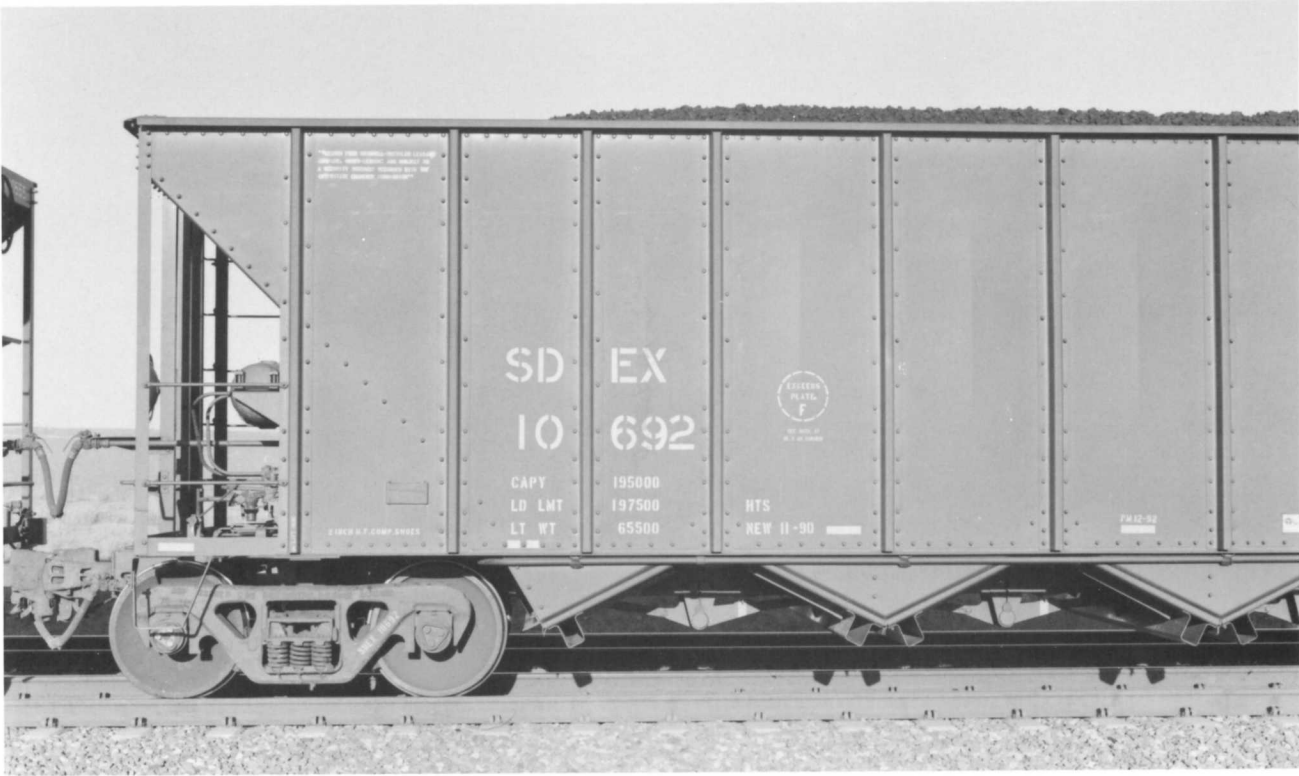
SDEX 10692. (Above). Left side view. Note how the rivet pattern on the ribs change from paired to alternating depending on stress points (greater stress on top and bottom joints).
