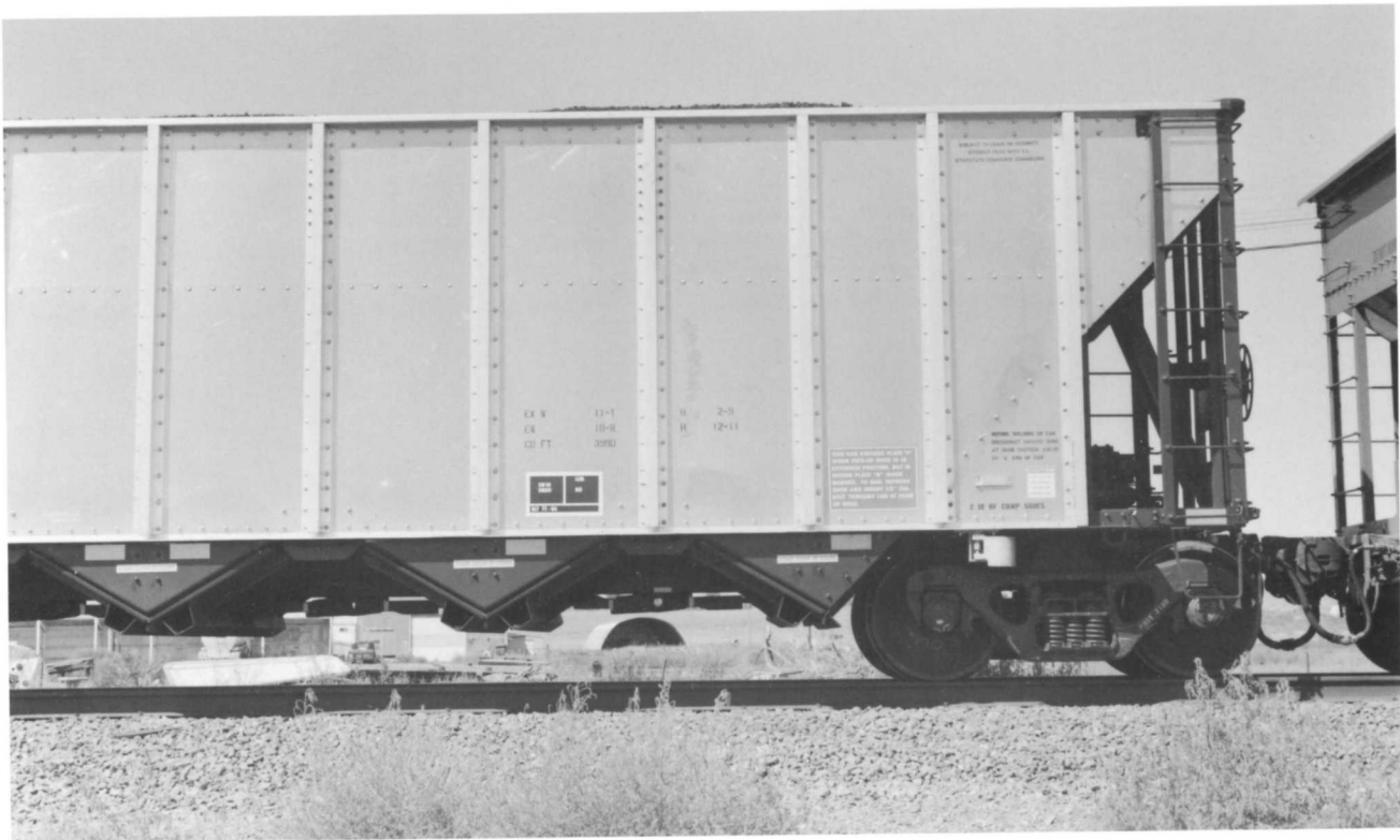
PRBX 2188. (Above). The horizontal row of rivets about two-thirds up the side and the double row of fasteners just under the top chord are evident of this Johnstown America design.
