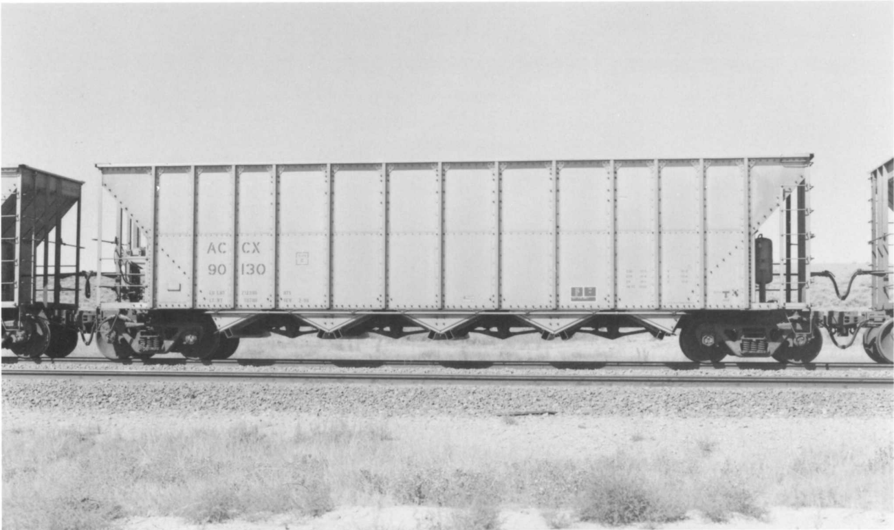
ACCX 90130. (Above). Aluminum-bodied 1990 built Trinity 4,000 cubic-foot design. The horizontal rivet line is more obvious on this car ( cf IPPX 386). Elements of the Ortner design become apparent including the "curved" lower drop of the end sheets into the end hoppers.
