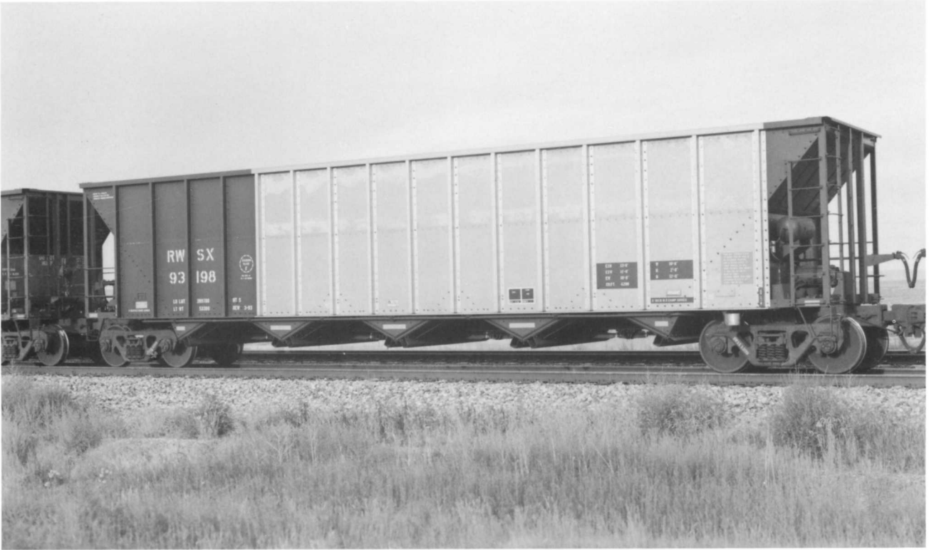
RWSX 93198. (Above). Aluminum-bodied 1993 built Trinity 4,200 cubic-foot design. This sixteen rib car is five-foot longer than the standard Trinity quick-dump cars ( cf ACCX, CRL, NSPX). Series is RWSX 93001-93946 (946 cars).
