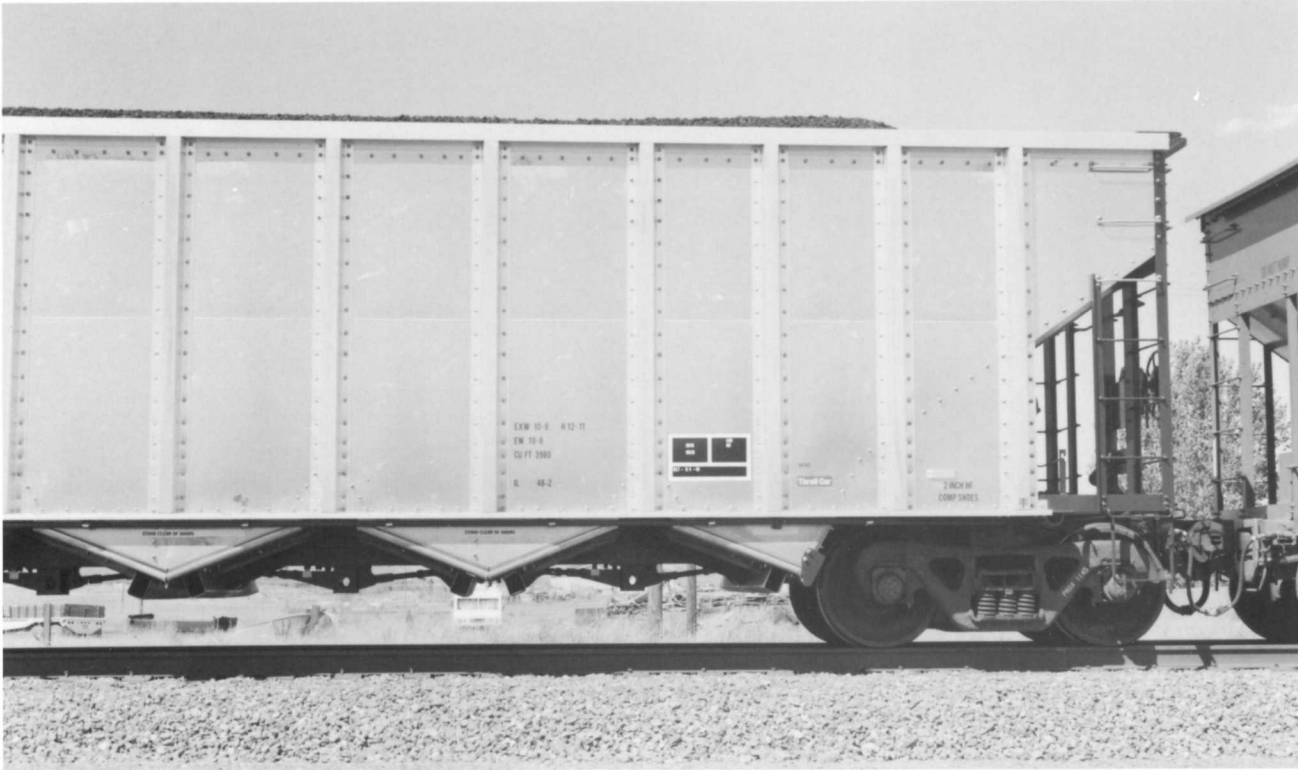
MTPX 94047. (Below). Aluminum-bodied 1994 built Thrall Car 4,040 cubic-foot design. OL remains the same at 53'1". However, height was increased to 13'5" (compared to the PRBX's 12'11").
