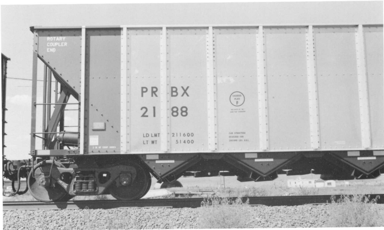
PRBX 2188. (Below). Right side view. Pick-up shoe actuator on "B" end. PRBX = Transisco Leasing Company with home offices in San Francisco CA.
