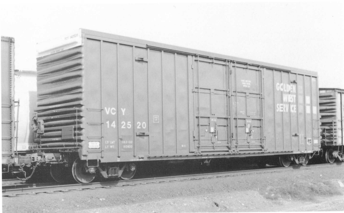
VCY 142520. (Below) This is a 50'7" IL Plate F box car. The car was originally built in 1969 by Gunderson as a 70-ton car. When it was rebuilt into this VCY series it was upgraded to a 100-ton car and had several inches of height added. Note the additional "bars" on the lower part of the end.
