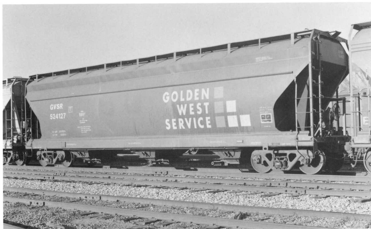
GVSF 524127. (Above) "A" end 3/4 view. This is a 4,650 cubic-foot capacity covered hopper. It was built by ACF in 1969. Equipped with gravity-only outlets. Compare the side-sheet architecture of this earlier car to GVSF 530192 (previous page).
