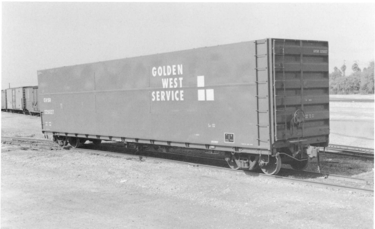
VCY 144069. (Above) 60'10" IL Plate F box car. Built in May 1978 by Pacific Car & Foundry. Class B-100-44. Load limit is 175,200 lbs. Capacity is 7,477 cubic-feet. Its centered double-sliding doors provide a 16-foot wide opening.
