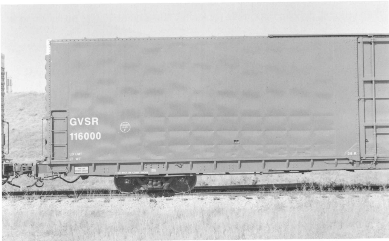
GVSER 116000. (Below) Class B-100-16. Close-up of left side of car. Note the lack of stencilled weights for load limit and light weight (LD LMT and LT WT respectively). The exposed lower portion of the interior posts are a quick identification feature of Pullman-Standard's 86-foot high cubes.
