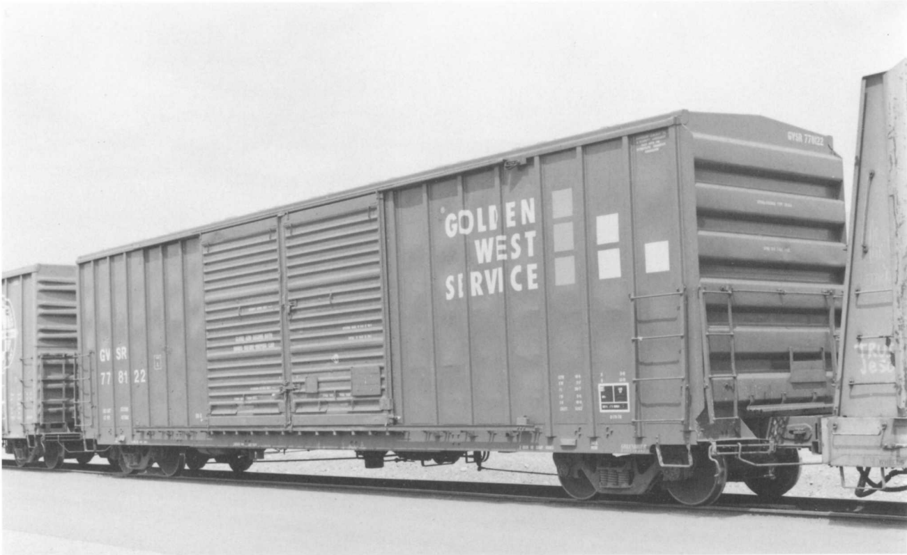
GVSR 778122. (Above) 50'7" IL Plate C box car. Built in June 1975 by FMC, Portland, Oregon. Class B-70-78. Equipped with Hydra-Cushion 20-14A.
