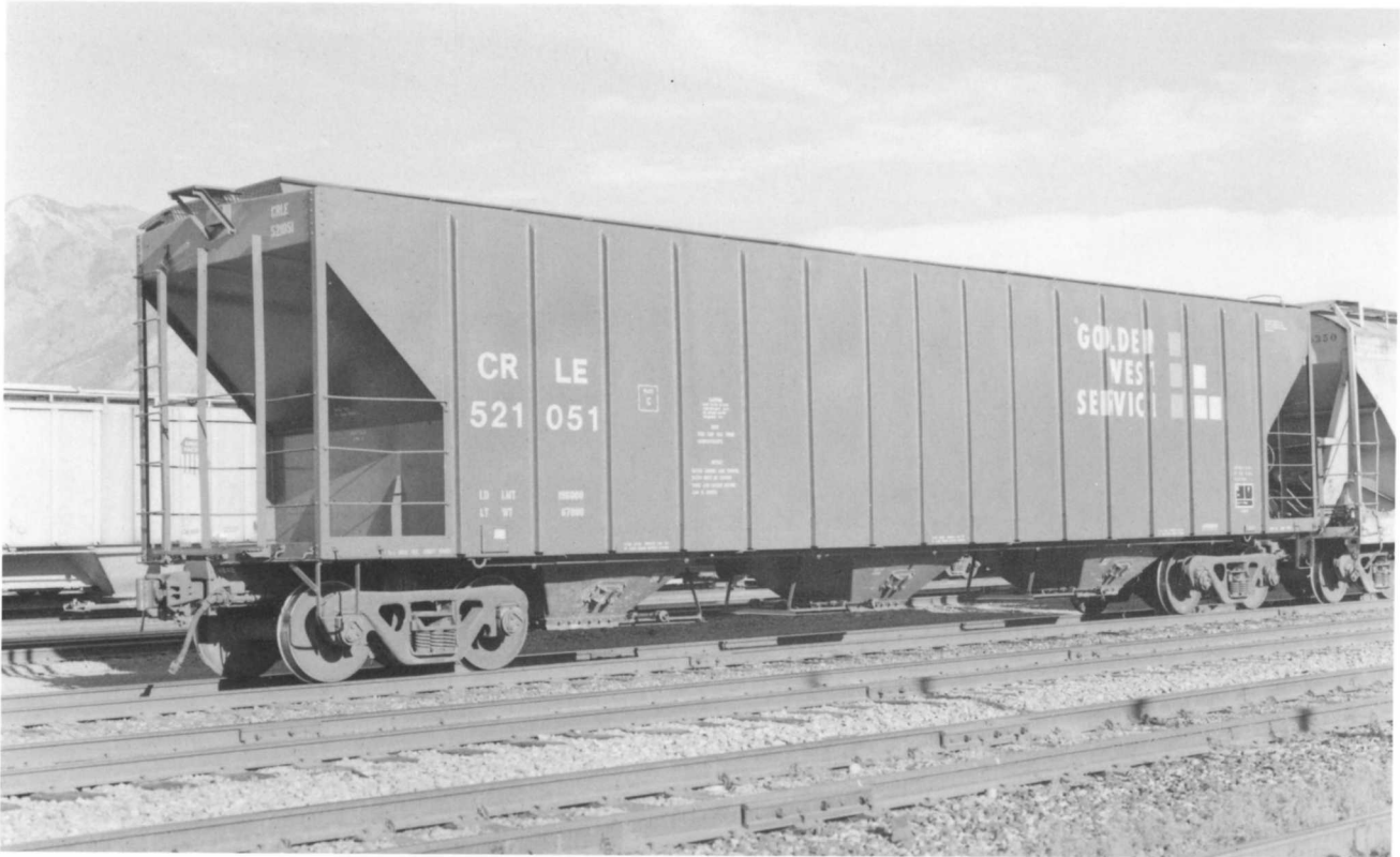
CRLE 521051. (Above) Pullman-Standard also built a number of 4,785 cubic-foot capacity grain cars which were less famous than the 4427's, 4740's or 4750's. Class H-100-21. These were built in 1967. Photographed in Ogden, Utah in 1994.
