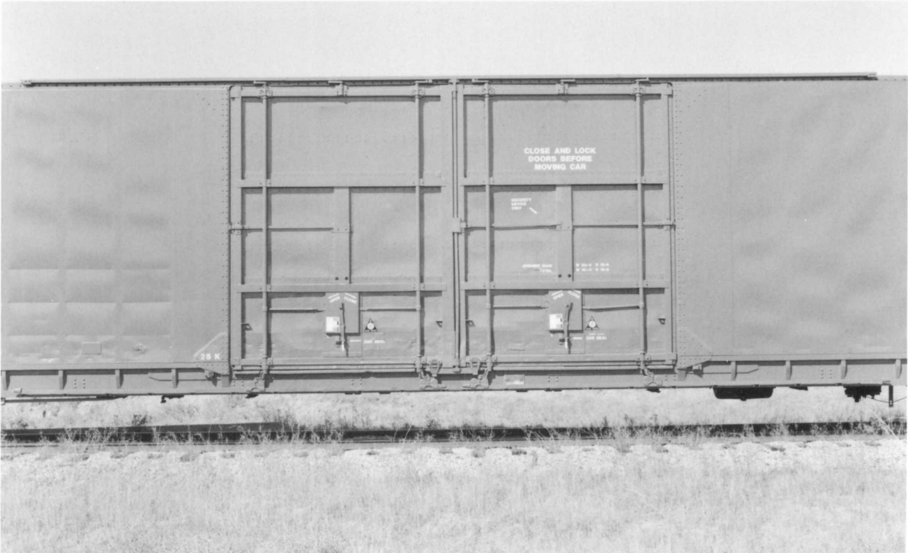
GVSR 116000. (Below) Close-up of right side of car. The car has a stencilled capacity of 10,468 cubic-feet. Most of the 86-foot high-cubes were originally stencilled as having a 10,000 cubic-foot capacity.
