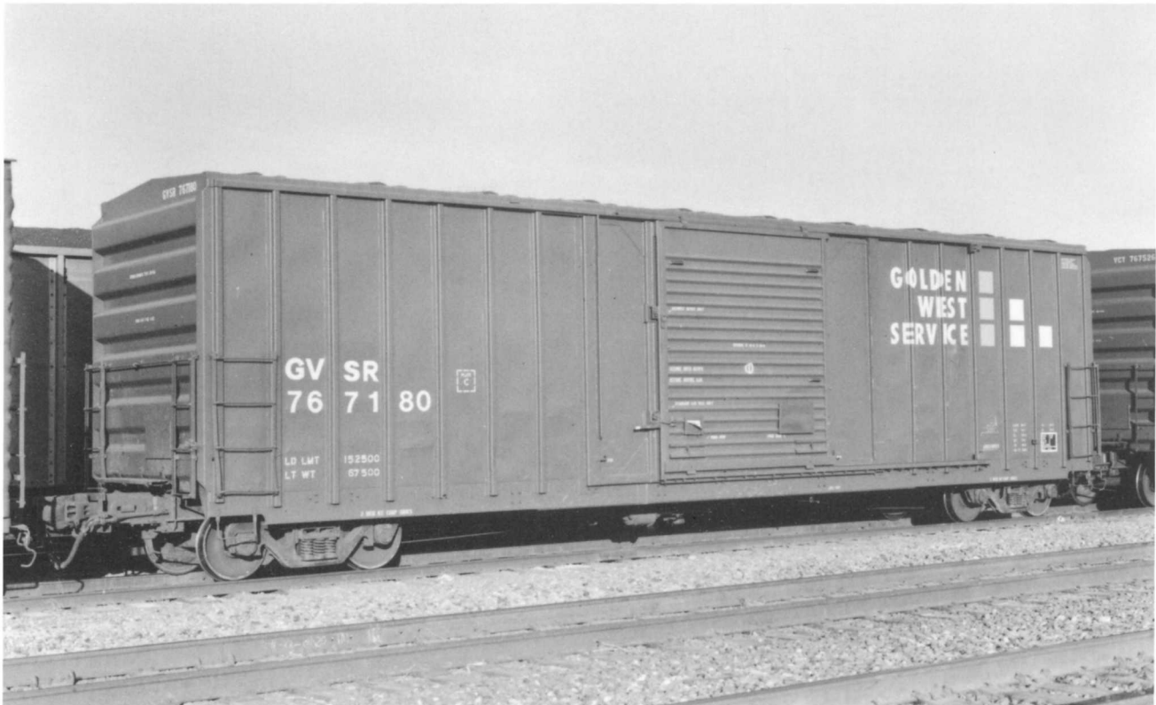
GVSR 767180. (Above) 50'7" Plate C box car. Class B-70-67. This car was originally built in 1973 by FMC as a 16-foot opening double-sliding-door box car. It was converted to a 10-foot opening single-sliding-door box car when painted in the Golden West paint scheme.
