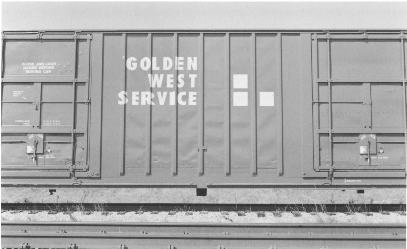
GVSR 719000. (Above) Mid-section detail. The area in the middle barely allows room for both doors to open. Note the Hydra-Cushion cylinder underneath directly under the center rib.
