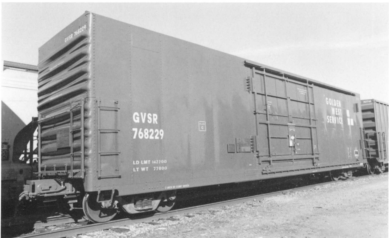
GVSR 767180. (Above) 50'7" Plate C box car. Class B-70-67. This car was originally built in 1973 by FMC as a 16-foot opening double-sliding-door box car. It was converted to a 10-foot opening single-sliding-door box car when painted in the Golden West paint scheme.
