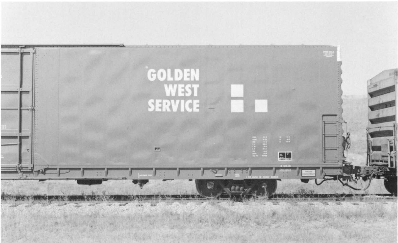
GVSR 116000. (Below) Close-up of right side of car. The car has a stencilled capacity of 10,468 cubic-feet. Most of the 86-foot high-cubes were originally stencilled as having a 10,000 cubic-foot capacity.
