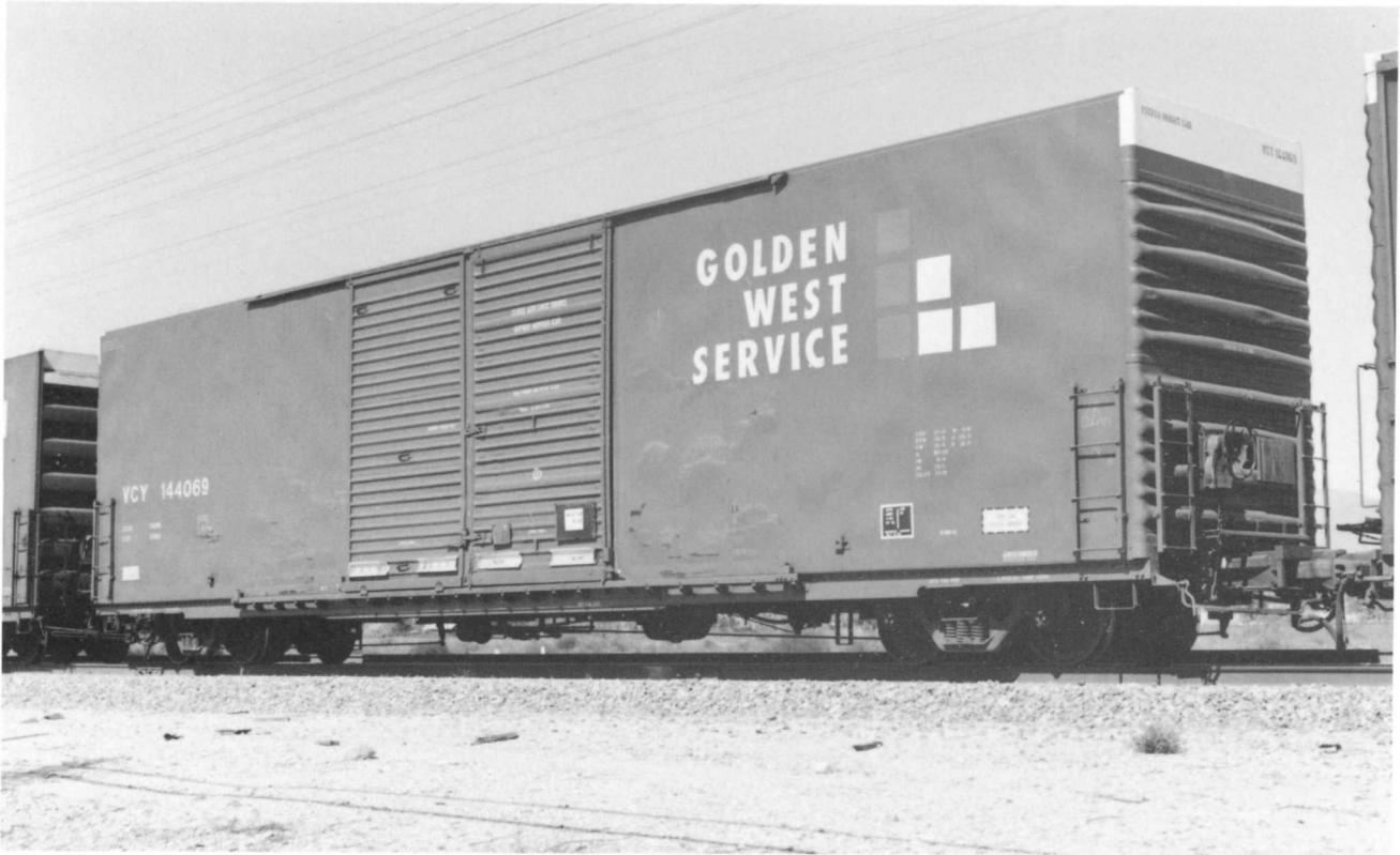
VCY 144069. (Above) 60'10" IL Plate F box car. Built in May 1978 by Pacific Car & Foundry. Class B-100-44. Load limit is 175,200 lbs. Capacity is 7,477 cubic-feet. Its centered double-sliding doors provide a 16-foot wide opening.
