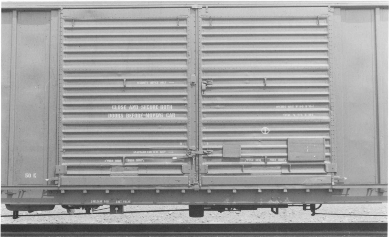
GVSR 778122. (Above) Center side section detail (door area). This car retain its original double-sliding-door configuration. Both of the are Youngstown built doors.
