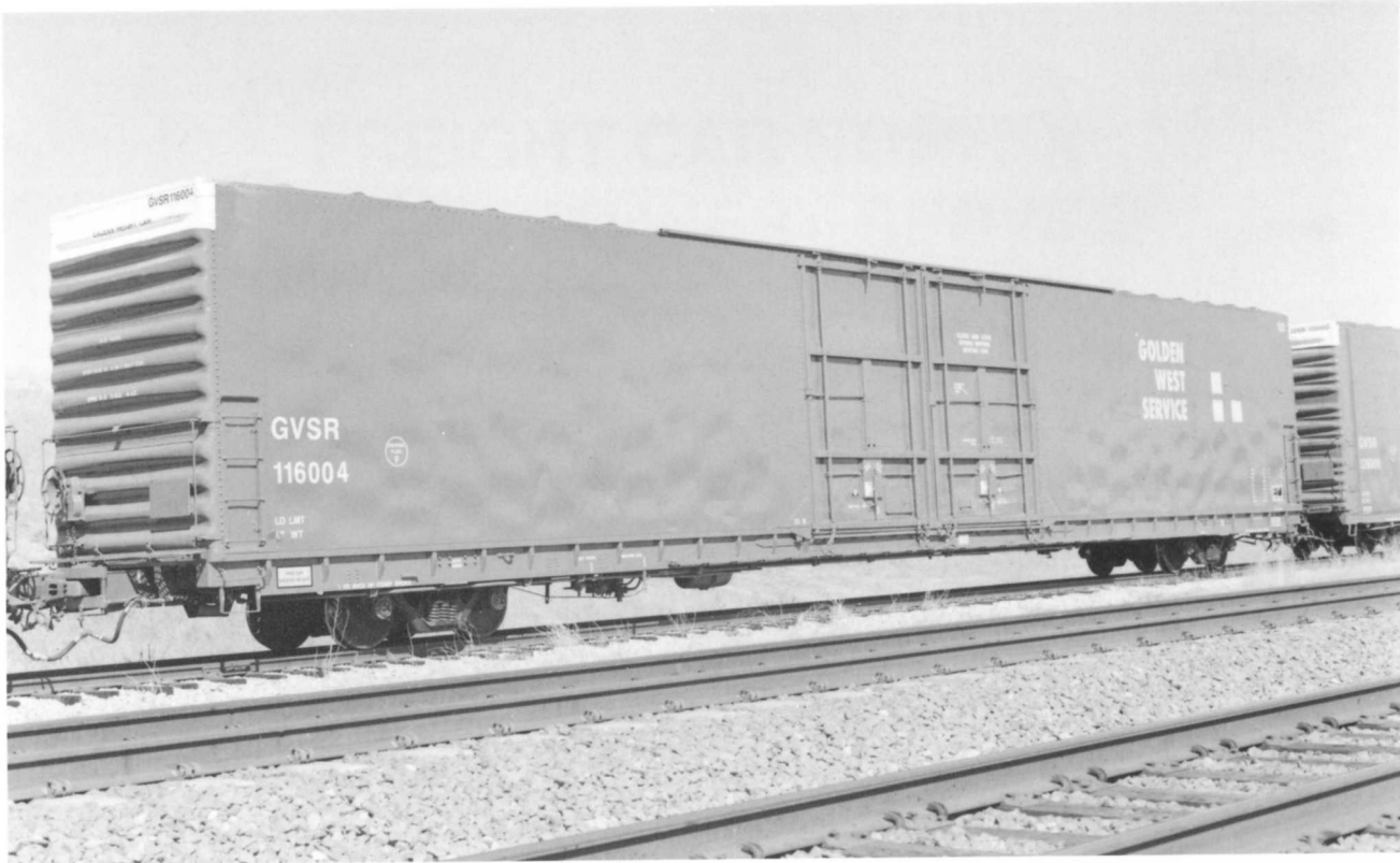
GVSER 116000. (Below) Class B-100-16. Close-up of left side of car. Note the lack of stencilled weights for load limit and light weight (LD LMT and LT WT respectively). The exposed lower portion of the interior posts are a quick identification feature of Pullman-Standard's 86-foot high cubes.
