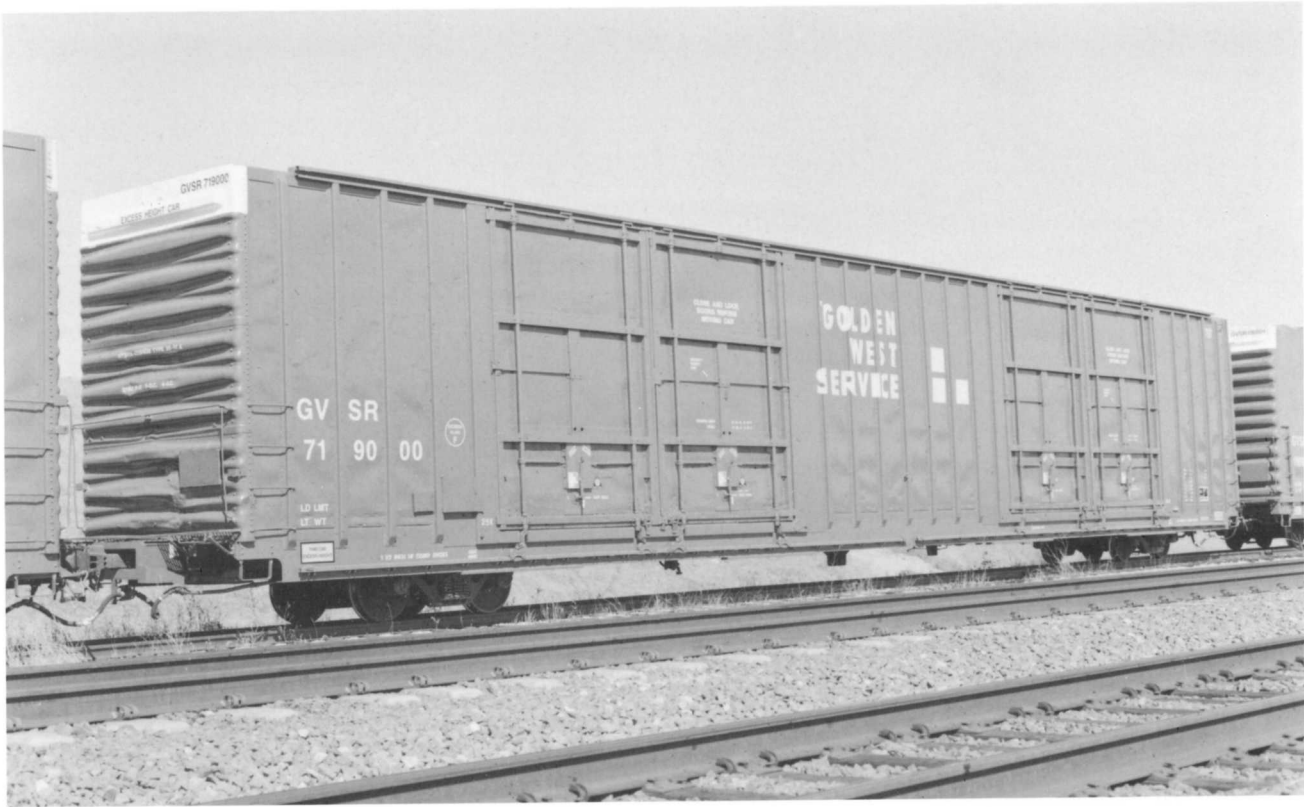
GVSR 719000. (Below) Left side section detail. The exposed side posts (ribs) of this design are a quick identification feature for Pacific Car & Foundry's "86-foot" high-cube.
