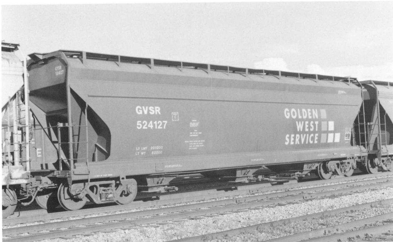
GVSF 524127. (Above) "A" end 3/4 view. This is a 4,650 cubic-foot capacity covered hopper. It was built by ACF in 1969. Equipped with gravity-only outlets. Compare the side-sheet architecture of this earlier car to GVSF 530192 (previous page).
