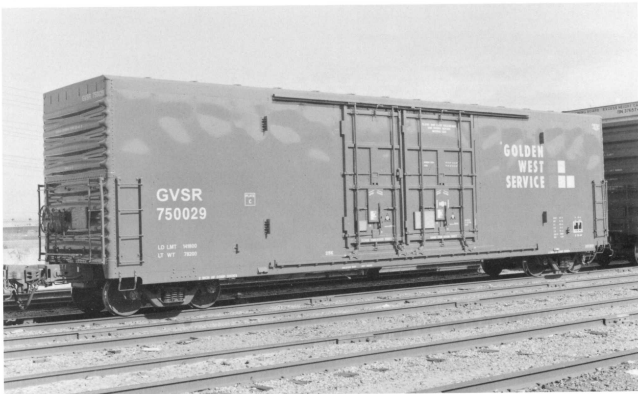
GVSR 750029. (Below). 50'6" Plate C passive refrigerator car (RBL). This one has a modified "door-and-a-half" configuration with an 8-foot and a 6-foot plug door on each side. Built in 1970 by Pacific Car & Foundry. Load limit 141,800 lbs. Capacity is 4,836 cubic-feet.
