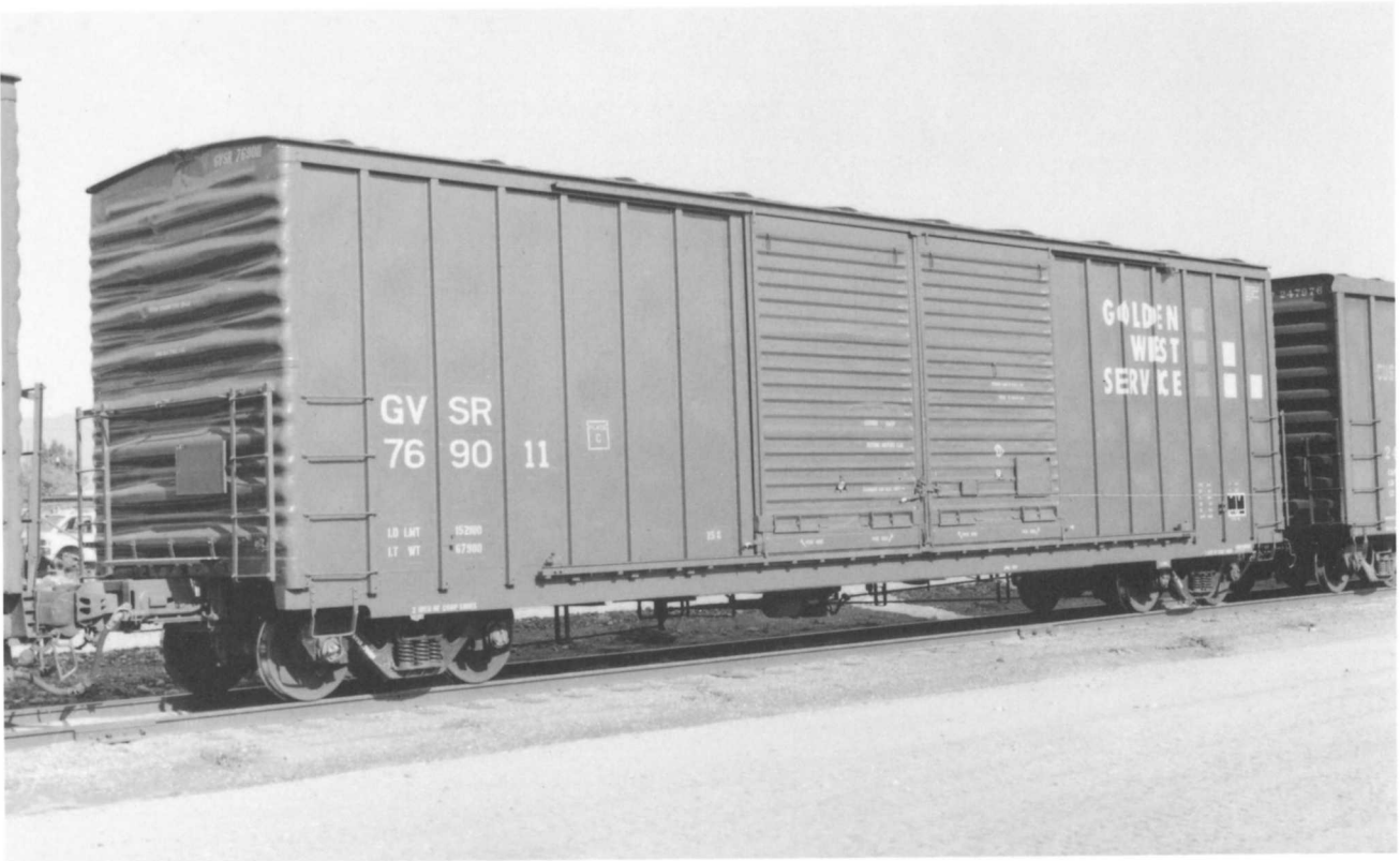
GVSR 769011. (Above) 50'7" IL Plate C box car. Built in 1973 by Pacific Car & Foundry. Class B-70-69. Note the uncharacteristic lettering style or font used for the reporting marks and car number. Load limit is 152,100 lbs. Capacity is 5,258 cubic-feet.
