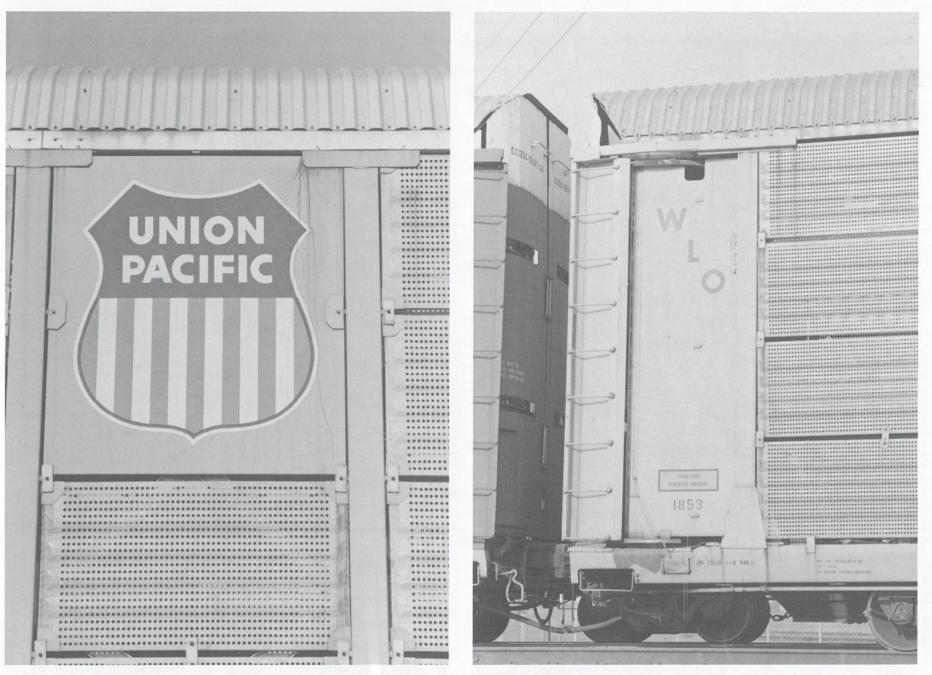
Fig 37. UP's vertical logo panel occupies the A2=B2 positions.
