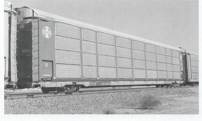
Fig 1. (Above) Santa Fe's ATSF 681 on ETTX 851864. This is a repainted Whitehead & Kales rack. Note the rack number and safety slogan (It's up to you) stencilled on the left end (LE). Rack colors are brown with white data.
