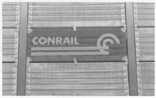
Fig 22. Conrail perforated/corrugated B4 panel.
