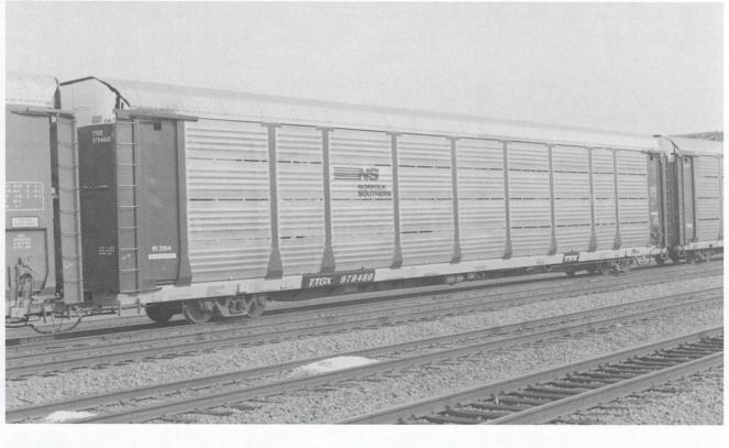
**Fig 11.** (Above) Norfolk Southern's NS 21814 on TTGX 979460. The B3 panel on this rack is solid/corrugated and remains in natural metal color with a black NS logo. The rack structure is brown and white.
