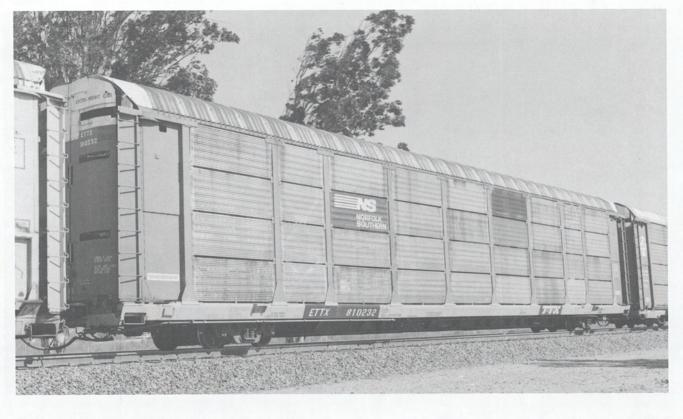
Fig 13. (Above) A repainted rack for the Norfolk Southern. Normally a rack number will appear on the lower left LE. The B3 panel has been replaced and/or repainted with the newer NS logo.
