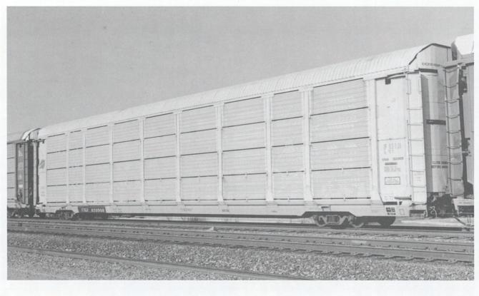
**Fig 5.** (Above) Chicago and North Western's CNW 820908 was originally a tri-level by Whitehead & Kales in May 1979. It was rebuilt into this bi-level car July 1991. This is the bright yellow scheme. CNW racks usually don't have rack numbers. And actually, the CNW rack number on this one is just the car number, repeated.
