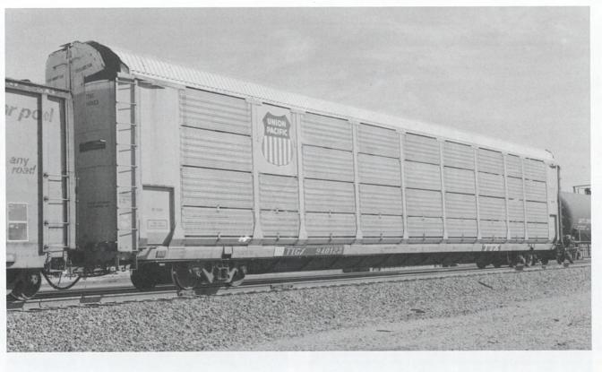
**Fig 17.** (Above) Union Pacific's UP 3448 on TTGX 940123. This has pretty much been the standard paint scheme for UP auto racks since the Eighties. MKT, MP, and WP rack have also appeared in this paint scheme as they get refurbished. In 1996, new UP racks began to appear with the "We Will Deliver" slogan.
