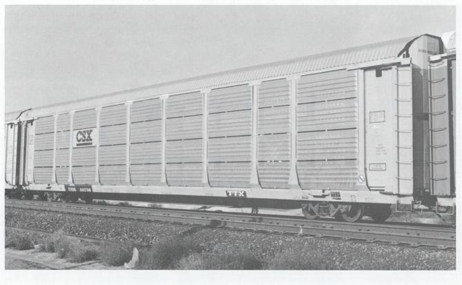
**Fig 9.** (Above) This CSX Transportation rack shows a more common lettering layout for CSX racks. Note the corrugated/solid logo panel on the B3 position. The rack was built by Thrall Car in 1992.
