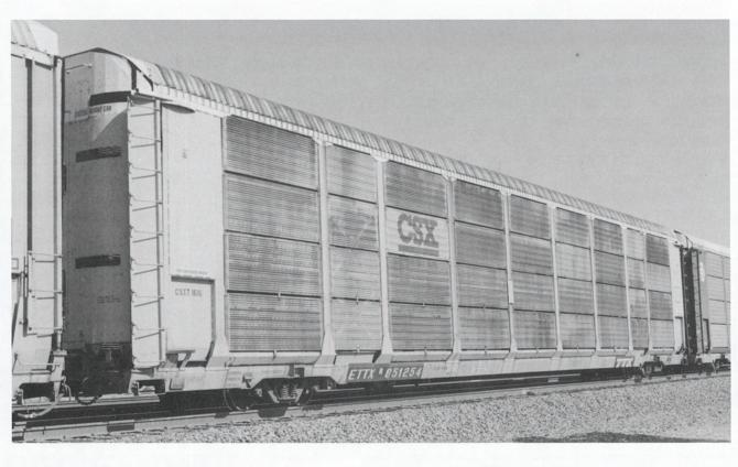
Fig 7. (Above) CSX Transportation's CSXT 1616 has had the rack painted without replacing the panels. Beautiful weathering on those panels! Yellow rack with black data and logo.
