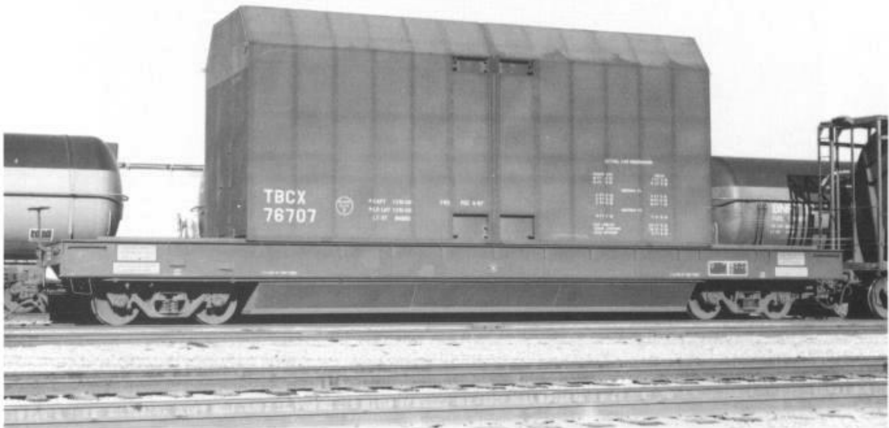
TOP Although not in the Wichita pool, these two cars are also a part of the Boeing fleet. Here TBCX 76707 is captured at the Burlington Northern's North Kansas City yard on September 16 1990. Built by The Maxson Company, this car is unique in that it is a well type flat with sliding hoods. The hoods split open at the center and move to the car ends. Most of these cars are used between Seattle and Stewart, FL. photo courtesy M. D. McCarter
