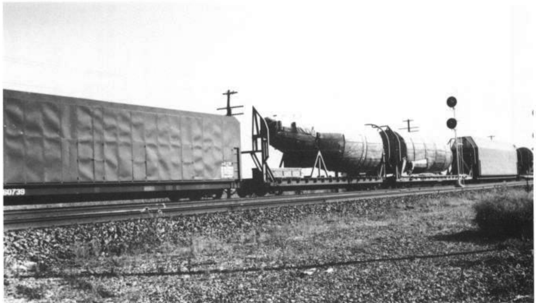
CONVOY! A string of aircraft parts cars hustles thru Ellinor Jct, KS on the way from Wichita, KS to Kansas City, MO on September 9 1990. As is typical, train speeds are high and stops few. The lead car, BN 613139, is carrying a 757 nose section, followed by a skin assembly car. Then there are two flats, (TTMX 80857 followed by ATSF 90096) carrying the fuselage assemblies for another 737 airliner, the worlds most popular jet. Finially, GN 60739 trails, carrying the tail parts for a 737, possibly the one shown in this photo.
