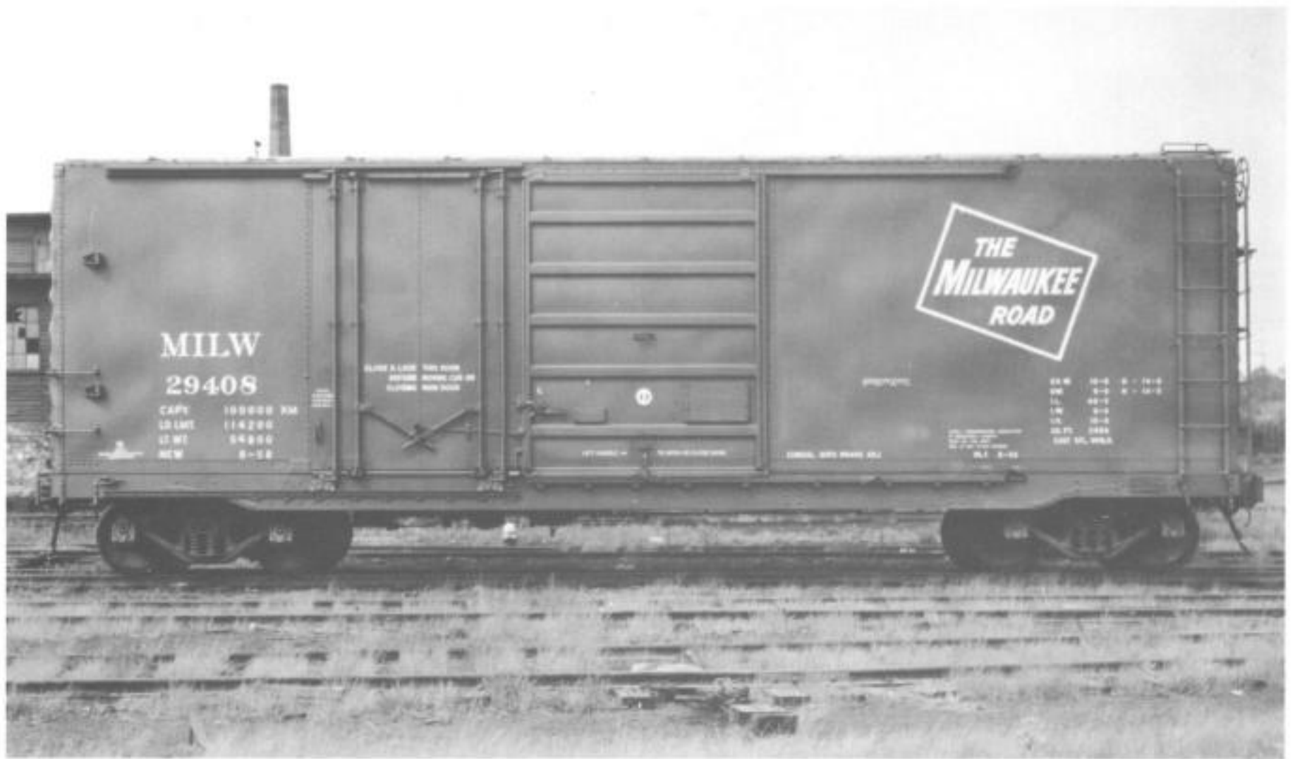
ABOVE This car is part of lot 8449 which was built in 1958 at Michigan City. They were rated at either 3966 cuft. or 50-tons and went into service as the series 29000-29499, a 500 car order. With a 40'5" inside length this group of cars was equipped with combination doors, an 8' sliding door plus a 7' auxiliary plug door. Cars 29000-29399 employed a Camel design while the remainder used the Superior design. All cars were plywood lined and used Barber S-2-A trucks.
