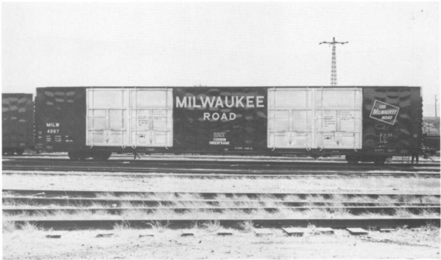
ABOVE Pullman built numerous 86'6" hi-cube cars, including this one from lot 8950B. Thirteen of these Hydroframe-40 equipped cars went into the series 4987-4999. Eight of these Bessemer-built cars were in assigned service to the Chevrolet Company at Indianapolis, IN and the others were assigned to the B&O at Parma, OH, also in Chevy service. Evans bulkheads and 5 DF-2 belt rails were included as were four aluminum Camel plug doors per side. ASF A-3 trucks were used.
