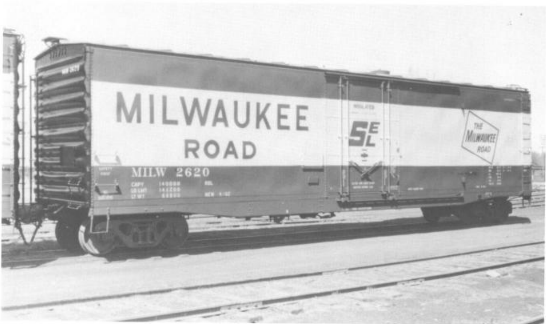
ABOVE Milwaukee 2620 is from lot 8665, built at Michigan City in April 1962. Fitted with a 9-belt Spartan Easy Loader system, this car was part of the 55 car series 2600-2654. They were rated at 70-tons or 4465 cuft. and insulated. Notice that the ends are painted black. The Superior doors were 8' wide and the trucks were the Barber S-2-A type.
