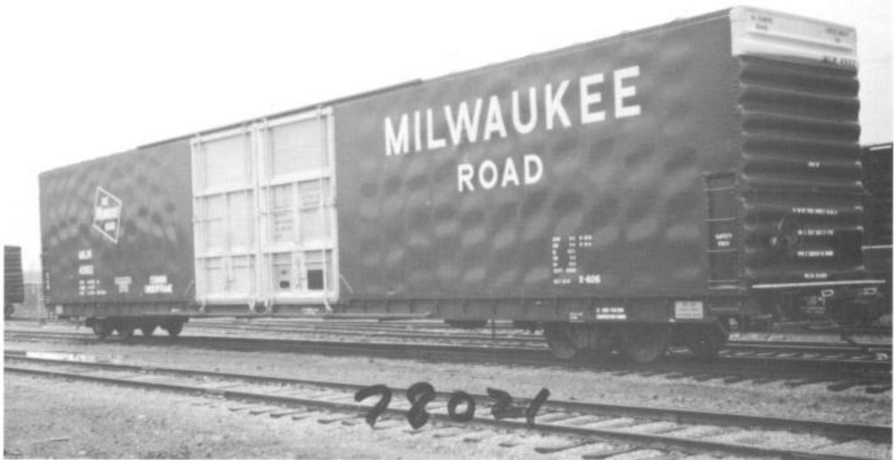
ABOVE This Bessemer-built hi-cube is one of five built in 1967 as lot 9275G. In Ford service assigned to the NYC at Monroe, MI, this car is rated at 70-tons or 10,000 cuft. Placed in the series 4978-4982, they used dual Equipco load dividers and five rub rails. Twin Camel aluminum plug doors were also fitted. Notice that this car has accidentally been marked with the Pennsy class "X60G", apparently a mistake from the stenciling drawings. Most of the cars to various railroads from lot 9275 were so marked.
