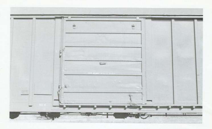
(Above) **BAR 4600**, door area detail. The SCD sliding door has been minimally stencilled with only the width and height of the door opening.
