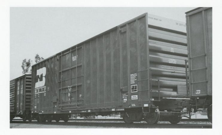
(Above). A very angled shot of **BN 287107**. This is part of the latest group of 300 box cars from Gunderson. This one was built in December 1994. Each of the cars are 50'6" inside length with a 6,269 cubic-foot capacity. The cars are equipped with 12-foot plug doors and 100-ton trucks. They will be used primarily for the paper industry.
