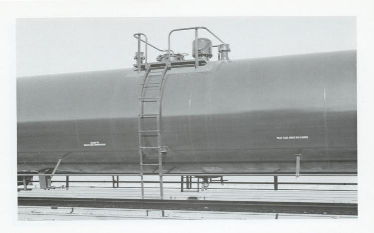
(Above) Middle section of GATX 79878 shows the top platform arrangement and lower outlet. Livery is standard black with white lettering.
