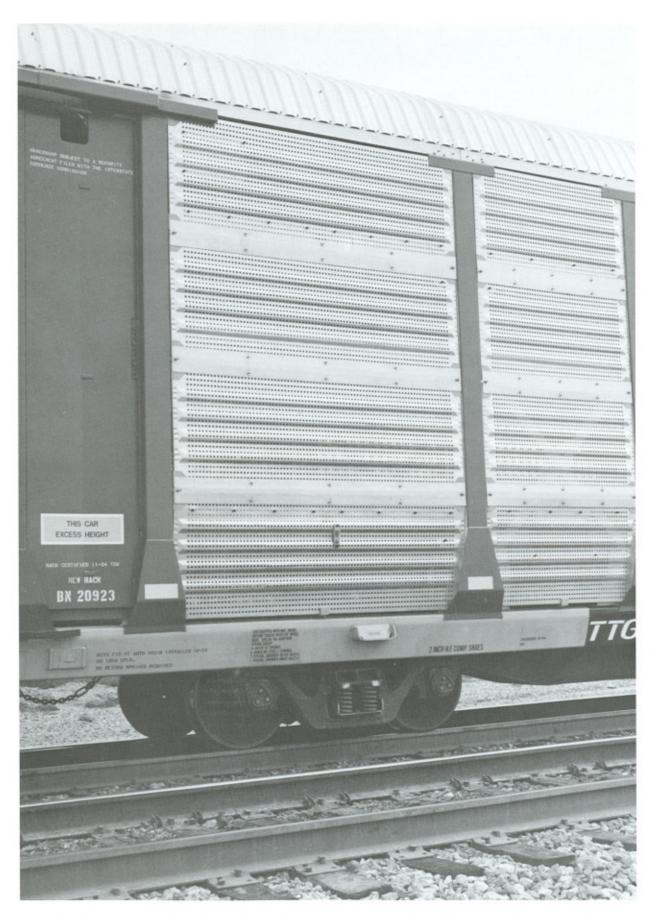
(Above) Burlington Northern rack number 20923 on TTGX 974807 exhibits the new solid filler panels designed to secure the gap formerly found between the perforated panels. This also eliminates the small vertical washer-plates that used to be in the middle of each perforated panel. This is the first new-built racks that BN has received since 1991. The rack was built in November 1994 by Thrall Car's Winder GA plant.
