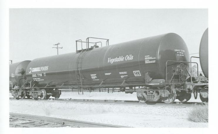
(Above) CRGX 7790 is part of a 250 car order built October through December by Trinity's Longview TX plant. Notice the new Cargill livery with no less than three different styles of léttering! The Cargill logo is green (and black). The 25,500 gallon cars are used for vegetable oil transport. Series is CRGX 7640-7889.
