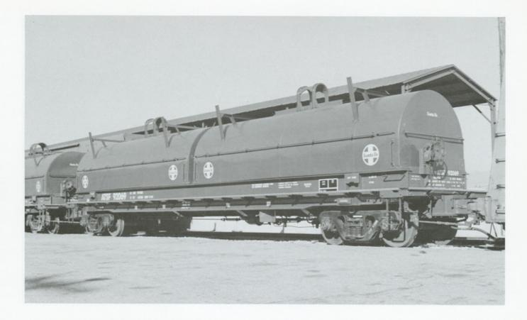
(Above) ATSF 92069 is part of a new series of coil-steel cars built by Thrall Car. These are essentially the same as those acquired in 1993. The cars are Santa Fe brown with white markings. Santa Fe class is FT-110. This group of cars appear to have all been built in November 1994. Photographed in Vernon, CA December 1994.
