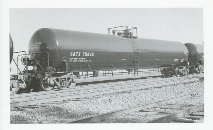
(Above) GATX 79845. This car was built in November 1994 by Trinity's Longview, Texas plant. These are 30,000-gallon noninsulated un-coiled 111A100W1 tank cars used for transporting alcohol. There are 85 cars in the series GATX 79842-79926. (Below) A detail of GATX 79878 shows the non-insulated Trinity (GATX-derived) design saddle. This car was built in December 1994 and is part of the same series as GATX 79845. The two cars illustrated here are being leased to the High Plains Corporation.
