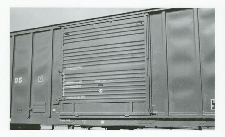
(Above) **OAR 3405** door area view. Note the modified PS-like door reinforcement gussets. The 12-foot sliding door has been equipped with a lower push plate to ease opening.
