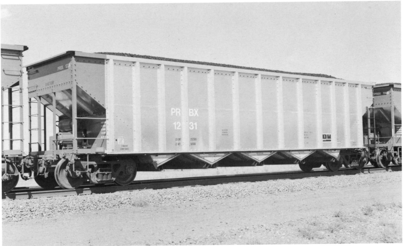
(Below) ROIX 57694 . Thrall has also been building plastic hoppers for 1994. ROIX 57667-57747 (81 cars) were built in February 1994 for Shintech Inc. Each car has a 5,800 cubic-foot capacity.
