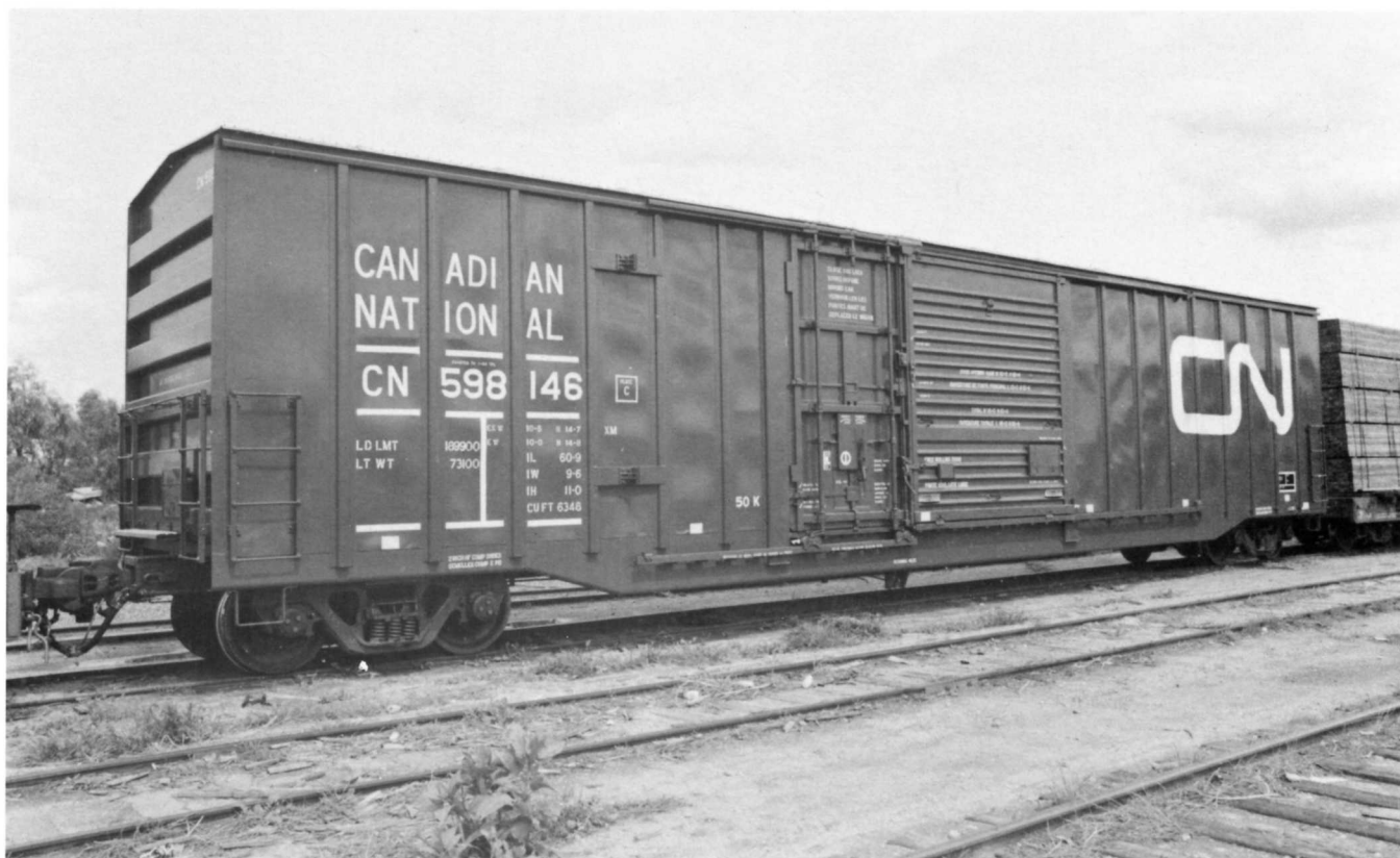
(Below) CN 598146 . This is part of a series of 500 box cars numbered CN 598000-598499. The cars were built December 1993 through February 1994 by the Trenton Works. The cars have 100-ton trucks. Each have a 6,348 cubic-foot-capacity. The cars are not cushioned.
