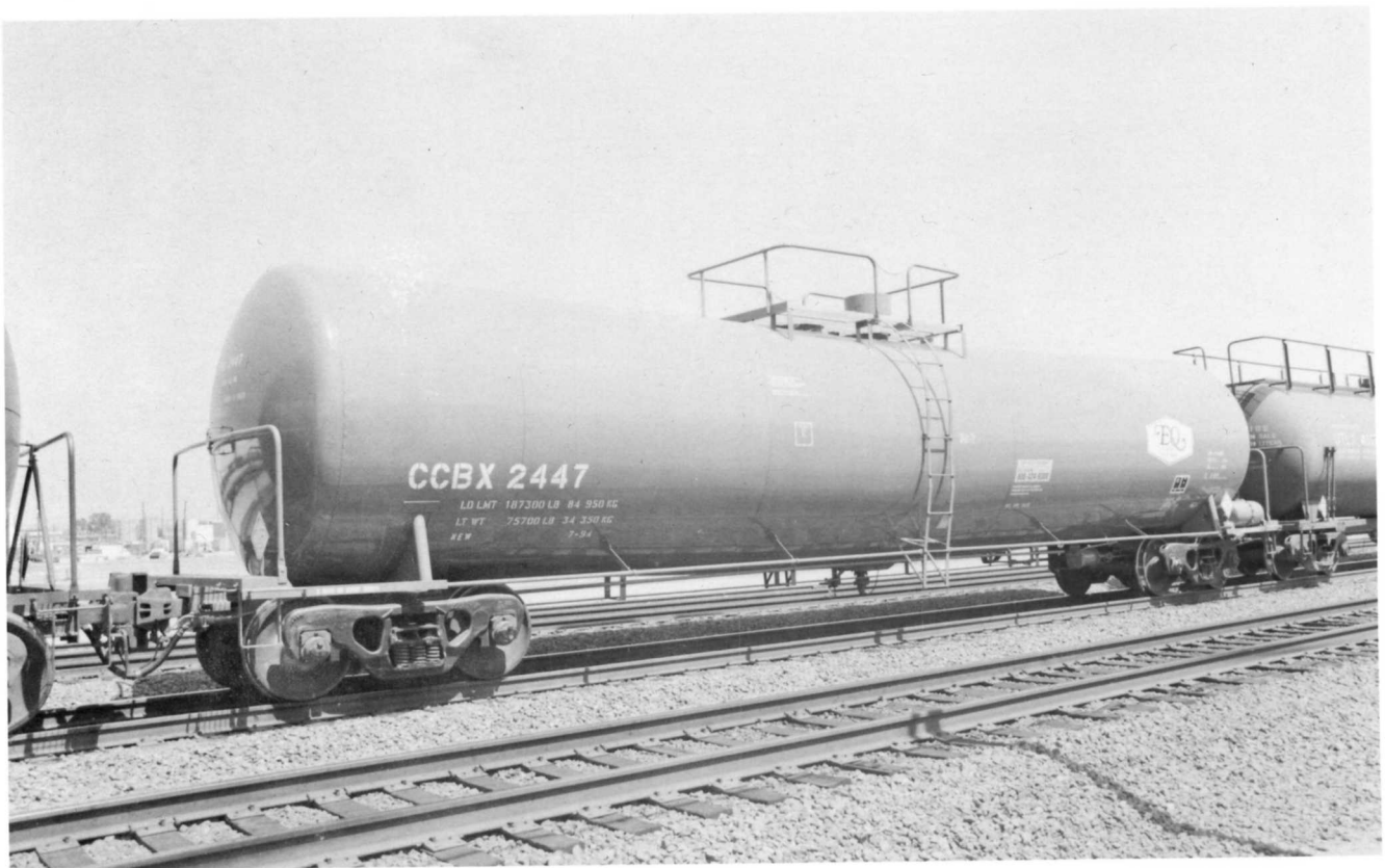
{Below} CCBX 2447 was built in July 1994 by Union Tank Car Co. CCBX 2401-2450 (50 cars) were delivered to Union Carbide in June and July 1994. Each car has a circa 24,600 gallon capacity. The cars have insulated uncoiled 111A100W3 tanks. Livery is Union Carbide blue tank with white lettering and data.
