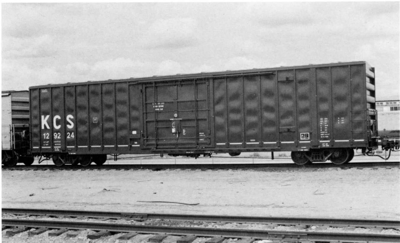
(Below) KCS 129224 . Kansas City Southern acquired 225 new 60-foot box cars in 1994. The cars, numbered KCS 129000-129224, were built January through February 1994 by Gunderson Inc of Portland OR. Livery is standard KCS brown body with white lettering.
