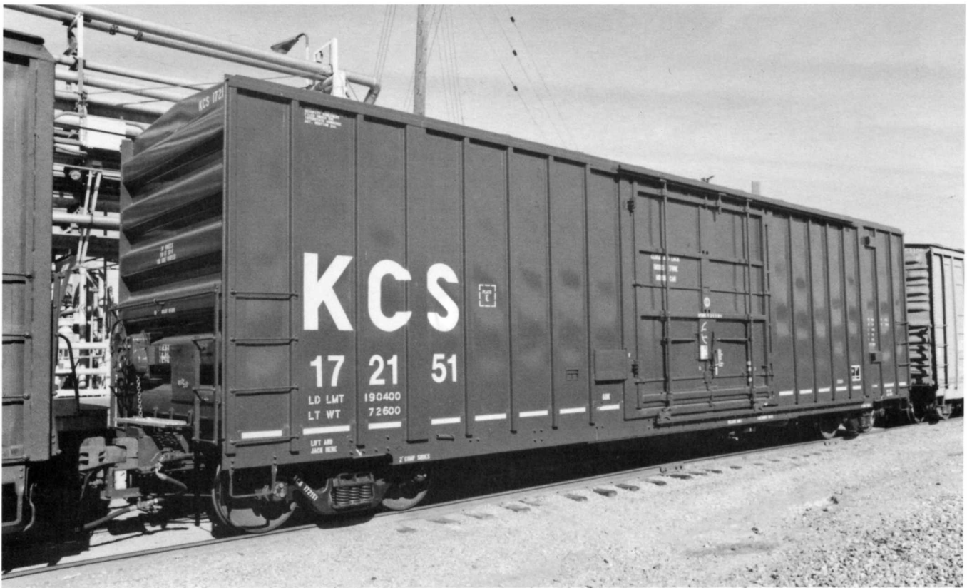
(Above) KCS 172151 is part of the 300 car series numbers KCS 172000-172299. The 50'6" box cars were built in October 1993 by Gunderson Inc of Portland OR. Each is equipped with end-of-car-cushioning and 12ft plug doors. Livery is standard KCS brown with white lettering.
