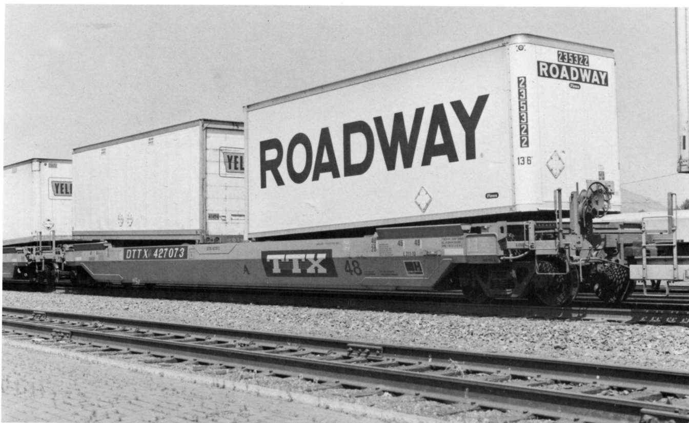
(Above) DTTX 427073 demonstrates double trailer capability. This is part of the first 110 three-unit drawbar connected Gunderson "All-Purpose Husky Stack" cars built for TTX. The cars, numbered DTTX 427000-427109 were built in August 1994. TTX class is GWA30. Each well can carry two short or one long trailer or double stacked containers. Photographed on the UP in La Grande OR during August 1994.
