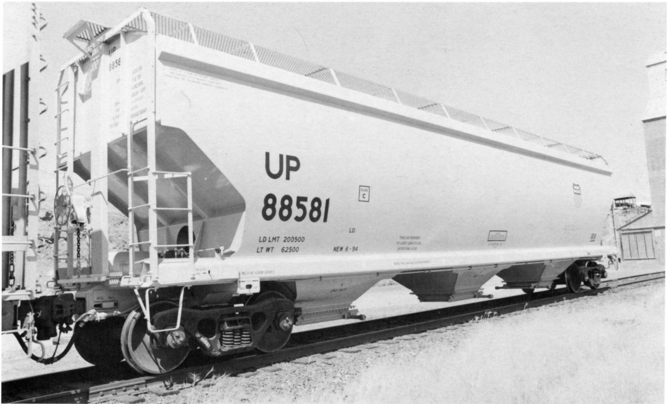
(Above) UP 88581 is a first for the Union Pacific. Canadian builder National Steel Car built 1,000 of these for the UP in 1994. The cars have a 5,116 cubic-foot capacity. New Union Pacific class is CH-100-119. Photographed August 1994 in western Idaho.
