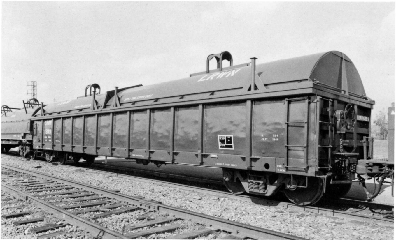
(Above) LRWN 6389 was originally built as part of the ICG 246100-246199 series. The 100-ton 2,240 cubic-foot gondola cars were rebuilt November 1993 through January 1994 for coil steel transport. The cars are leased from GERSCO to the Southern Pacific. Livery is SP brown with white lettering.
