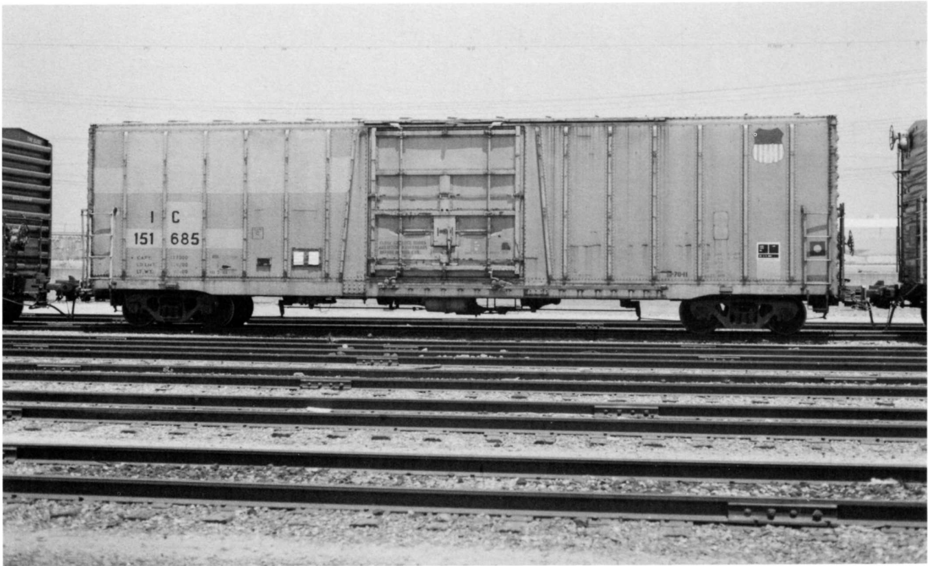
(Above) IC 151685 . The Illinois Central is operating a number of RBL refrigerator cars from various UP/MP/TP series. This car was a former UP class BI-70-11. The 151600-series cars were acquired in 1994.
