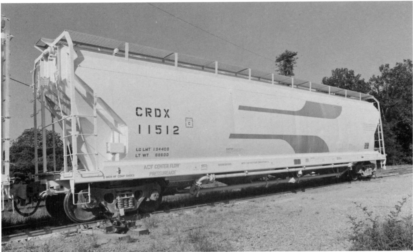
(Above) CRDX 11512 . Chicago Freight Car Leasing acquired fifteen new ACF PD 5000's in August 1993. The cars were built at ACF's Milton PA plant. Numbers are CRDX 11500-11514. Shown here during May 1994 in Macon GA.
