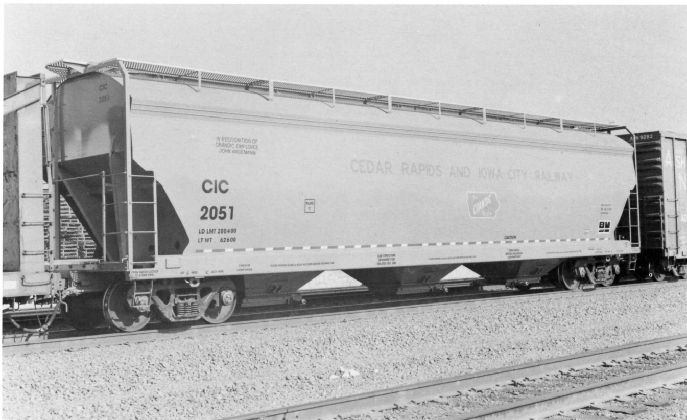
(Above) CIC 2051 is part of 100 cars delivered to the Cedar Rapids and Iowa City Railway in June 1994 by Thrall Car. Each car has a 5,150 cubic-foot-capacity. The cars are attractively multi-colored with gray body, black data, red lettering, and conspicuity stripes.
