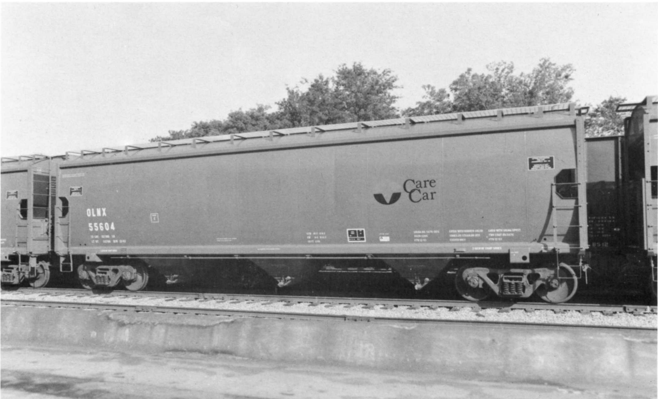
(Below) OLNX 55604 . Olin acquired 18 of these 4,301 cubic-foot capacity covered hoppers in late 1993. OLNx 55591-55608 were built in December 1993 by Trinity Industries. Livery is light brown with white lettering. Photographed May 1994 in Augusta GA.
