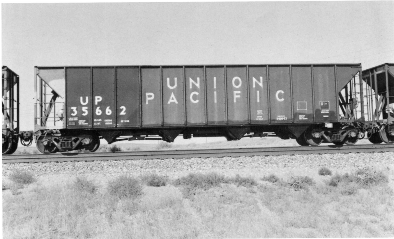
(Below) UP 35662 . Looks like a standard quad hopper coal car right? Wrong - note the pickup shoe under the first panel to the right and the gate arms. UP has converted a number of former conventional hoppers into auto dump hoppers. The cars have been renumbered into the UP 35600-series and re-classed to a new H-100-53 class. Photographed in August 1994 in Bill WY.
