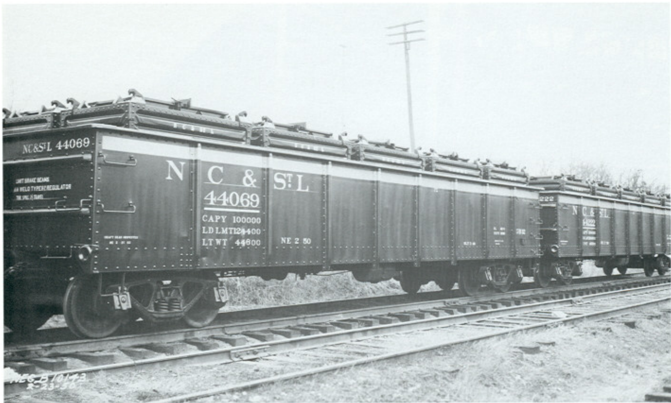
TOP: The N.C. & St.L employed a small number of container equipped gondolas, as shown here. These cars, out of the Railroad class GB-12, were fitted out with ten Youngstown Steel Door 145 cu.ft. containers for commodities such as limestone, silica and other items used in the foundry trade. Interestingly, by 1952, these cars had not been listed in the Official Railway Equipment Register as having been converted, though the photograph clearly shows the conversion was accomplished at Nashville in February of 1950. photo courtesy The University of Louisville BOTTOM: NC 18339, out of the XM-30 class, is shown in San Francisco in July 1954. Built in 1937, these cars survived for quite some time. Note the streaking from the slogan. photo courtesy W.C. Whittaker
