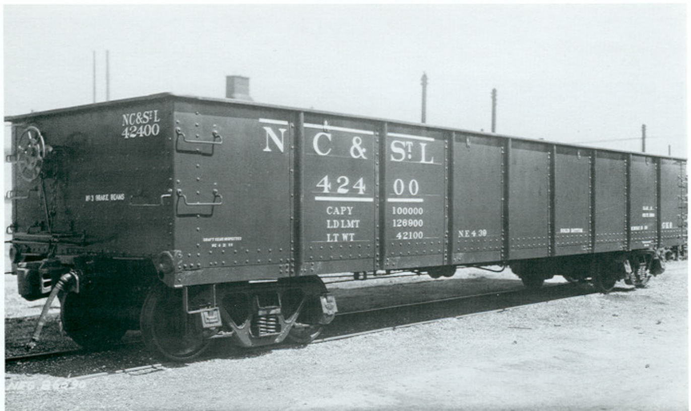
TOP: Boxcar 18300 was one of 500 cars built by Pullman to the AAR 1932 design. Built in 1937, they were from Pullman's lot 5561. The paintwork on this car is very similar to that shown in the lower stenciling drawing on pages 16-17. photo courtesy The Smithsonian neg # 2206 frame 43617 BOTTOM: NC 42400, rebuilt in 1939 at Nashville, is a class GK-6 car. Built originally at ACF in 1919, these cars were rebuilt thru 1940, for a total of 200 cars. Notice the tiedown anchor holes and reinforcement plates alongside the top side chords. photo courtesy The University of Louisville
