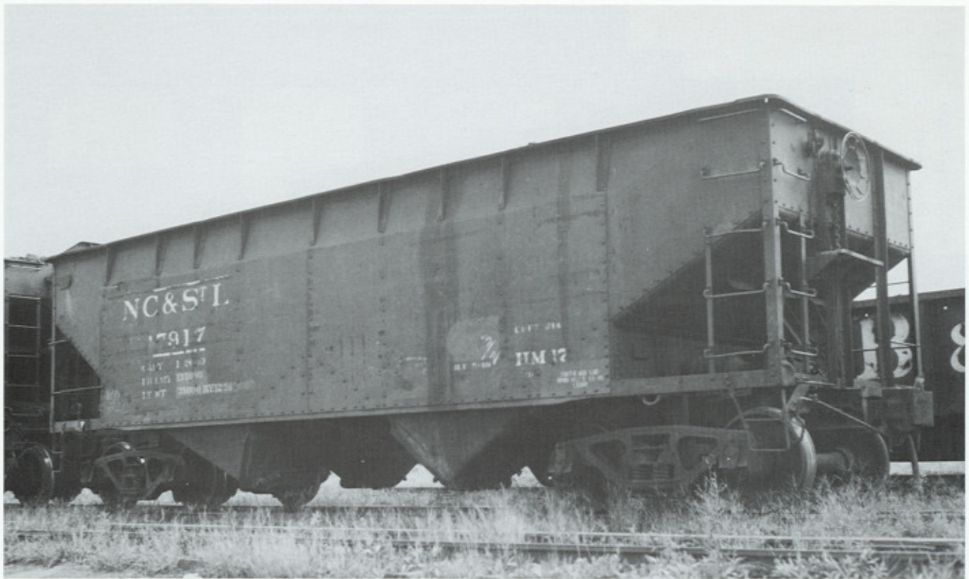
TOP: Though having seen fresher days, NC 47917 is still in the paint that she was manufactured in when built at Pullman's Bessemer plant in May 1949. One of the HM-17 class, and 500 strong, this was the largest single order of coal twins procured by the NC. Paul Dunn photo courtesy Rich Burg BOTTOM: From a much earlier time, #47166 shows quite a different set of lines. ACF built in 1926 at ACF's Madison, IL. plant, it was road classed as HT-00, "HT" being the MCB car class for twin hoppers at the time. The car is marked "for company coal only E.M. Wrenne". photo courtesy Ed Hawkins and ACF
