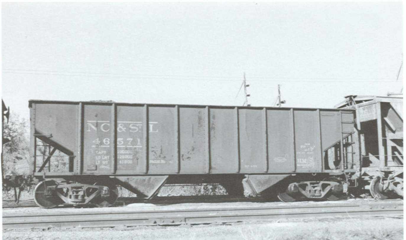
Two views of the series 46500-46899 built by Pullman-Standard in 1953 at Bessemer. These cars were not assigned NC class numbers by the railroad. TOP: 46694 is shown in coal service in the late 1950's. Looking closely, the slight dishing out of the side sheets may be seen. These were incorporated to strengthen the sheets somewhat. photo courtesy Chuck Yungkurth/Rail Data Services BOTTOM: NC 46571, also in coal service, location unknown, probably in the early 1960,s. photo courtesy Jay Williams/Jay Williams collection
