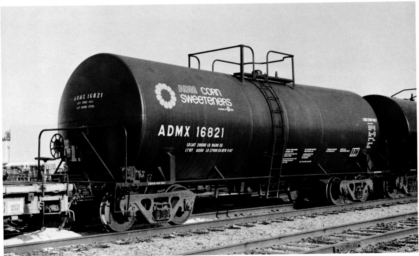
(Above) ADMX 16520 was built in March 1987 by TRN LGV. (Below) ADMX 16821 was built in May 1987 by TRN LGV. These 17,675 gallon (average) tank cars were also needed to replace the smaller size (16,700/17400 gal avg) used by the leased fleet. Note the difference in lettering arrangement in this car and the above one. The "consult owner before....." lettering group is to the right of the ladder on this car (BR side); while being to the left of the ladder on the car above (BL side).
