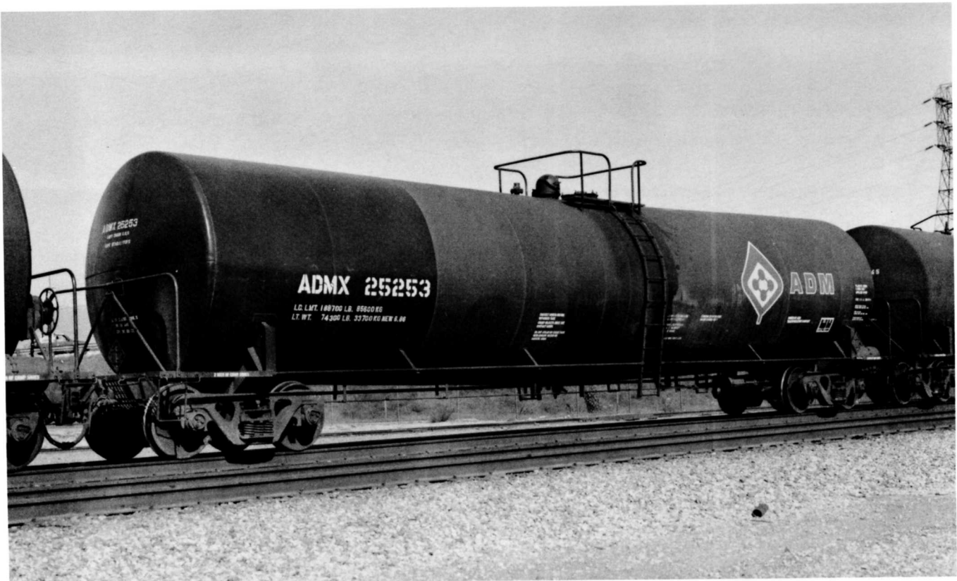
(Below) ADMX 25253 was built in June 1986 by TRN LGV. These 25,500 gallon tank cars are usually employed in vegetable oil service. They are insulated and equipped with heater coils to assist with unloading. I call this paint scheme the "ADM" scheme. One end of the car has been repainted.
