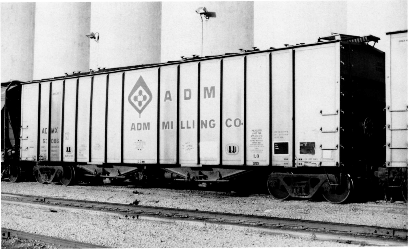
(Above) ADMX 53086 was built in June 1981 by GATX. This is one of GATX's famous Airslide covered hoppers. This version has a 4566 cubic foot capacity. Gray carbody. Photographed in August 1992 in Kansas City, MO.
