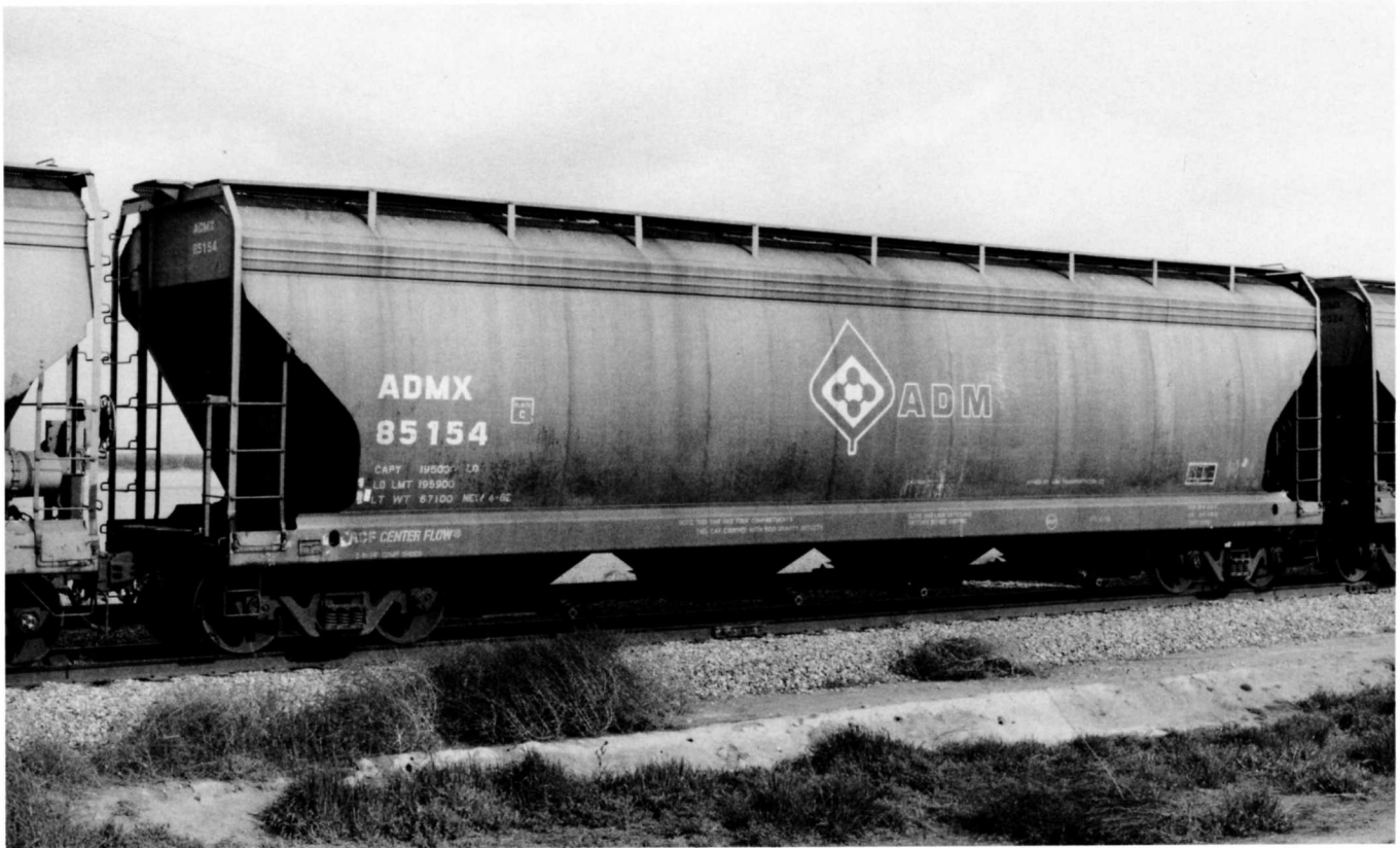
(Above) Probably the only Center Flow covered hoppers made at ACF's St Louis plant were from the ADMX 85001-85250 series as illustrated by ADMX 85154 above. Built April 1982. Blue carbody, white lettering.
