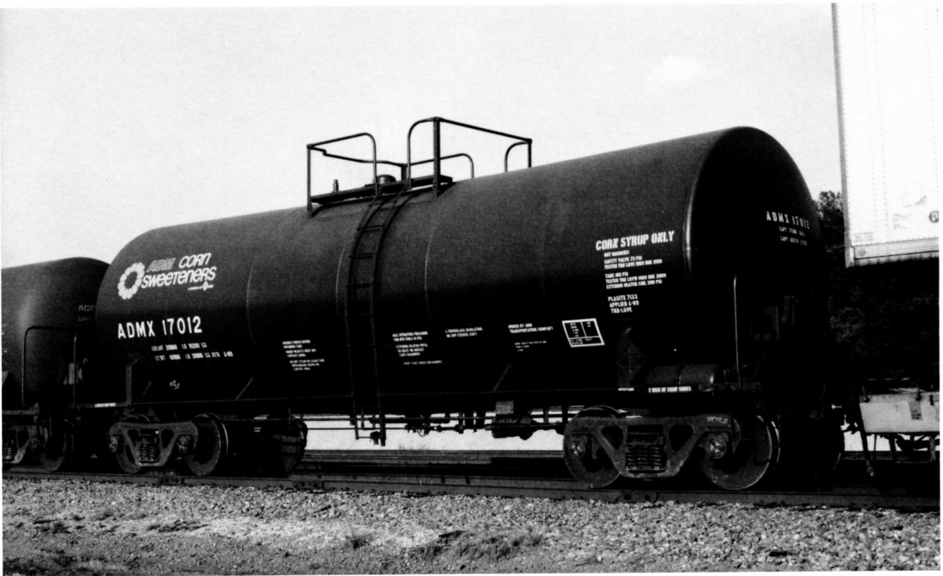
(Above) ADMX 17012 was built in April 1989. Plasite 7133 is a standard lining used by ADM. Corn syrup cars are insulated and are equipped with heater coils.
