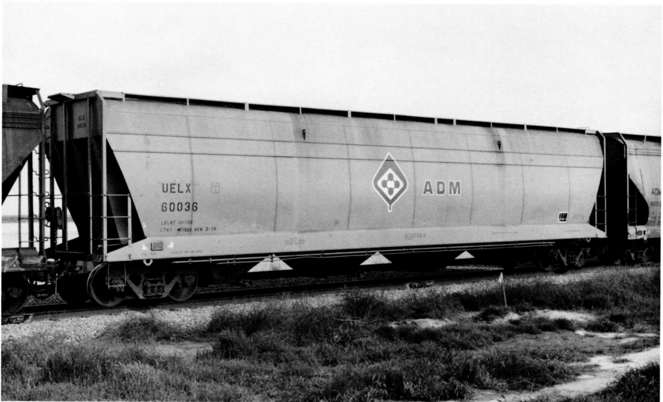
(Below) UELX 60036 was built in March 1978 by US Railway Equipment, Blue Island. Note the sharp side sill and car body angles on the ends which easily separates this design from the ACF Center Flows. Yellow carbody with black lettering.
