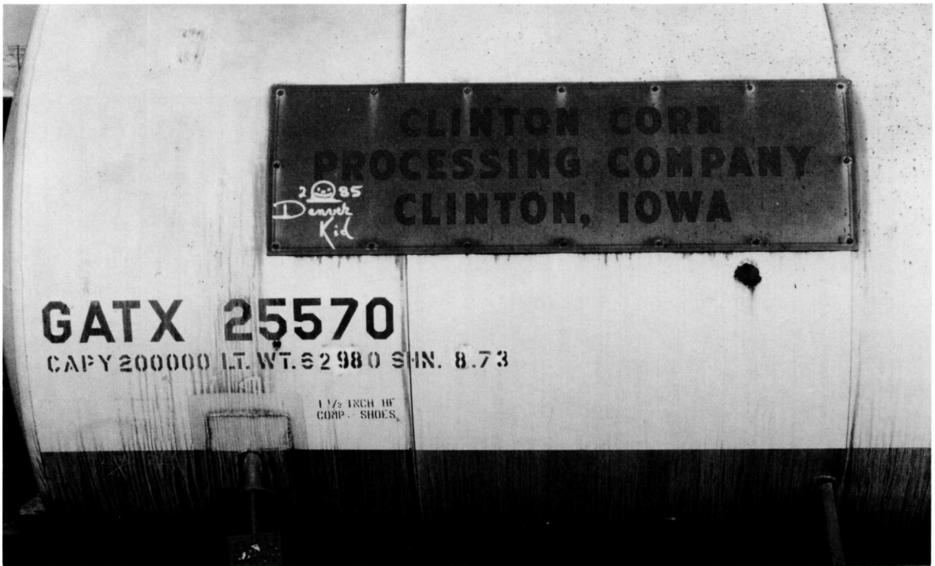
(Above and Below) These photos show the red and gold Clinton Corn Processing logo on GATX 25570. The car was reconditioned in 1979. Note how the logos are actually plates attached to the outside jacket of the tank car.
