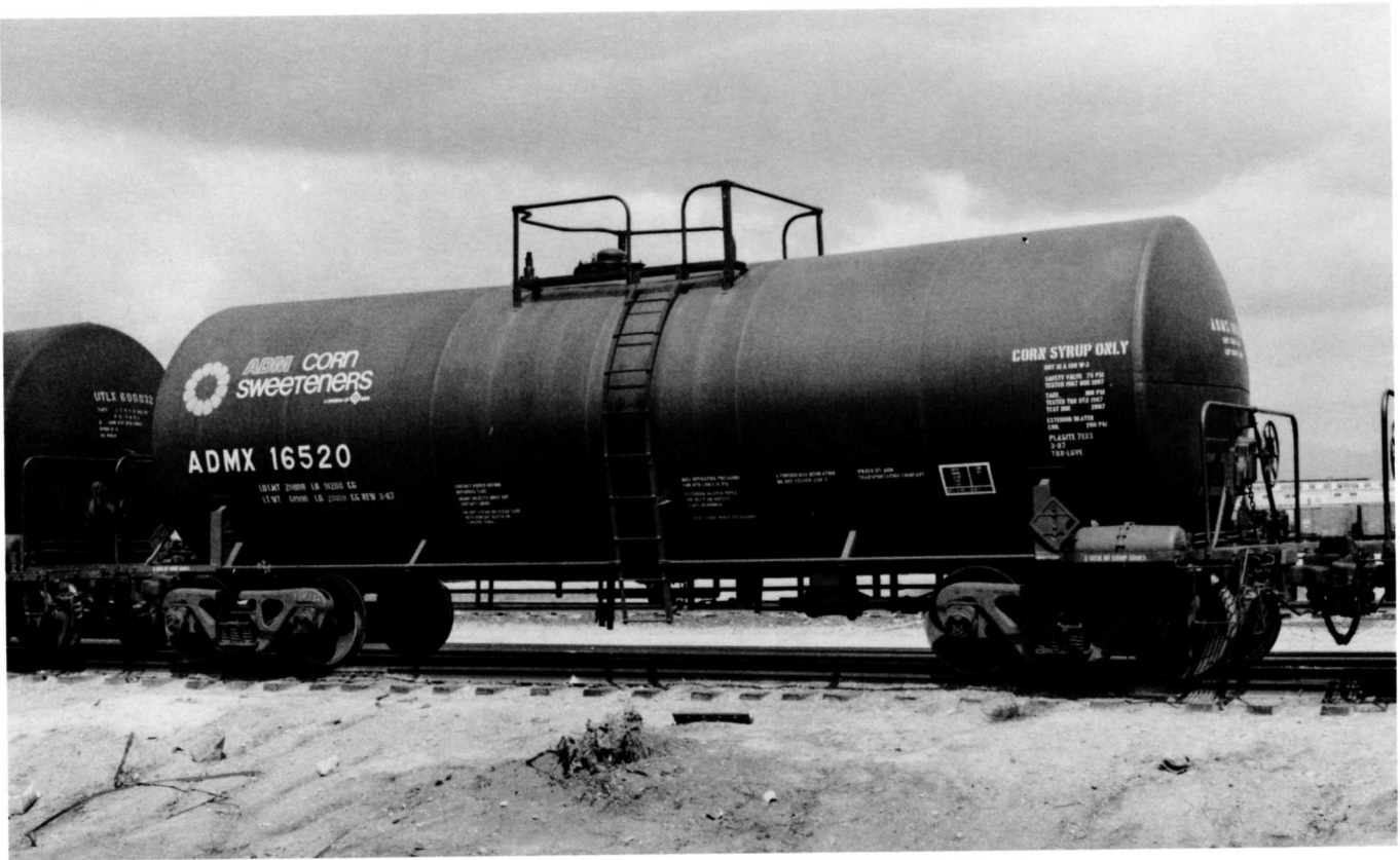
(Above) ADMX 16520 was built in March 1987 by TRN LGV. (Below) ADMX 16821 was built in May 1987 by TRN LGV. These 17,675 gallon (average) tank cars were also needed to replace the smaller size (16,700/17400 gal avg) used by the leased fleet. Note the difference in lettering arrangement in this car and the above one. The "consult owner before....." lettering group is to the right of the ladder on this car (BR side); while being to the left of the ladder on the car above (BL side).
