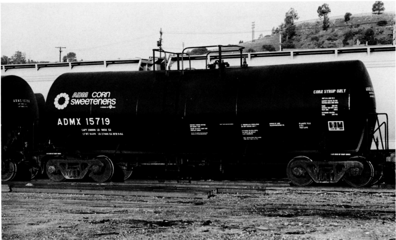
(Below) ADMX 15719 was built by Trinity's Longview, TX plant (TRN LGV) in September 1984. ADM's own reporting mark fleet soon began to replace the huge fleet of tank cars leased from GATX, NATX, and UTLX between 1984-1989.
