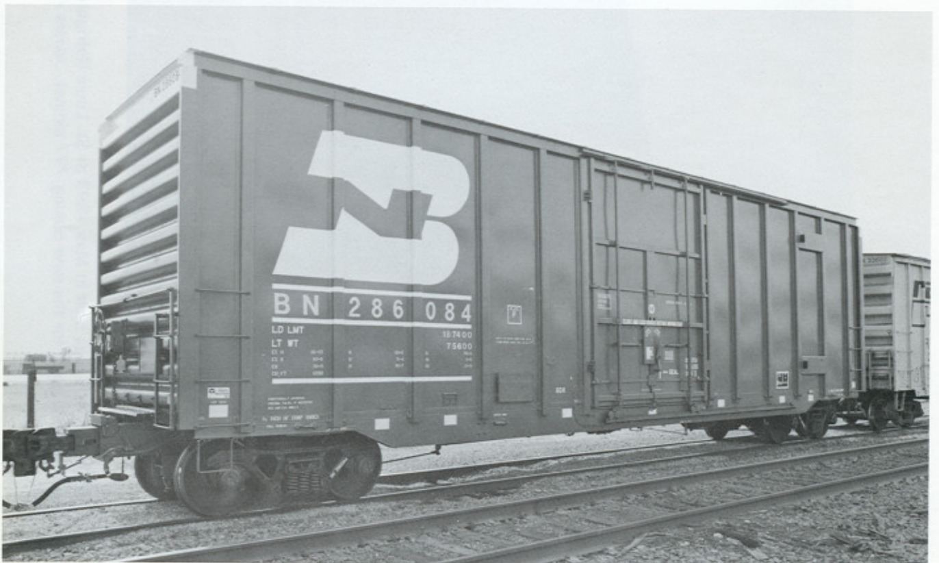
(Above and Below) BN 286084 and 296107 are part of a series of 157 high-cube 50'6" IL box cars being operated by Burlington Northern primarily for paper products transport. These are the first Trinity built box cars since the 1987 order for CSX (Gunderson has dominated the box car market since the mid-Eighties). Of note is the 10-foot plug door. All of the recent order of box cars for the BN have had 12-foot or wider door openings.
