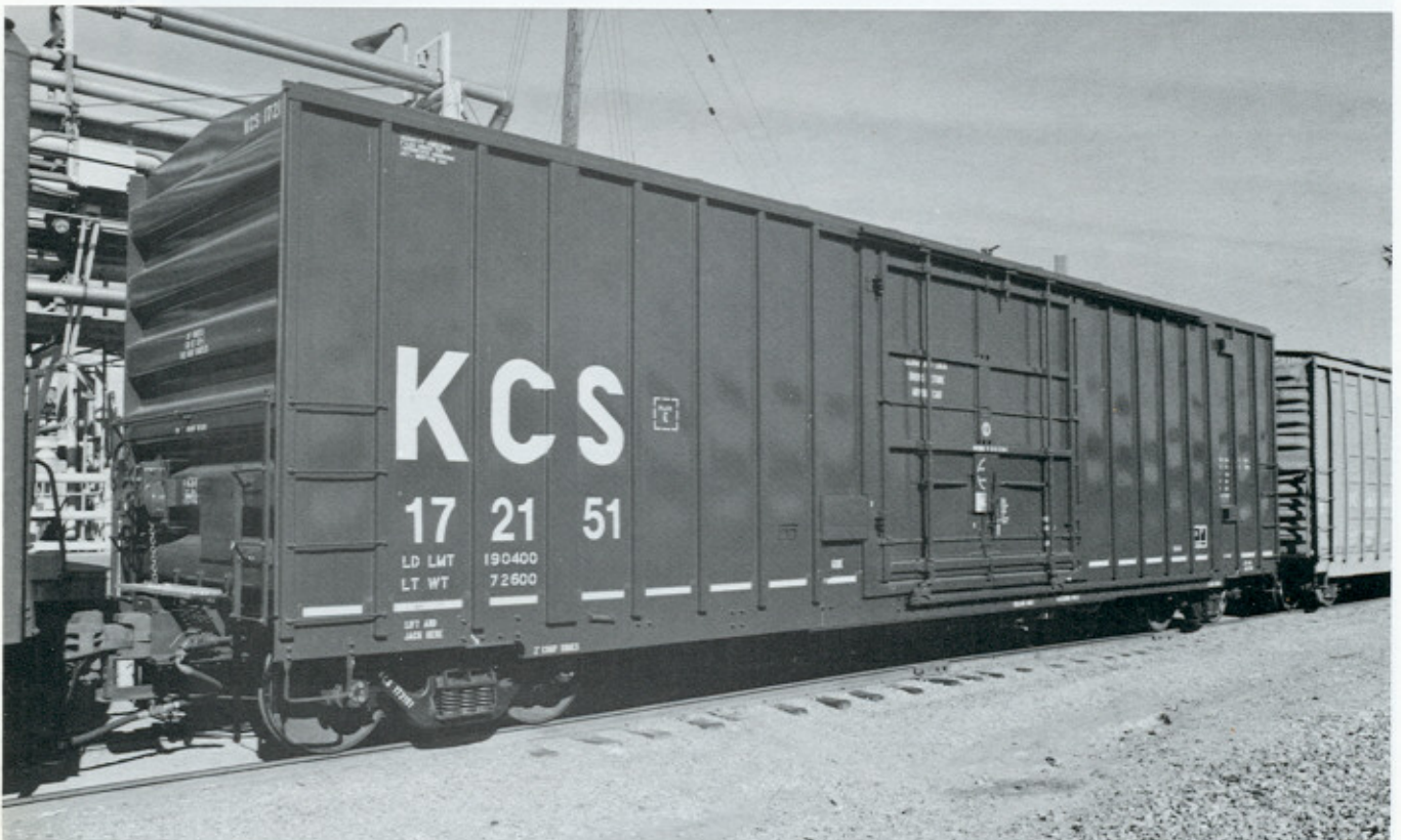
(Below) KCS 172151 is part of a series of 300 box cars built in October and November 1993 by Gunderson of Portland, OR. Note the extra wide rib (between "C" and "S" in KCS). Livery is brown and white.
