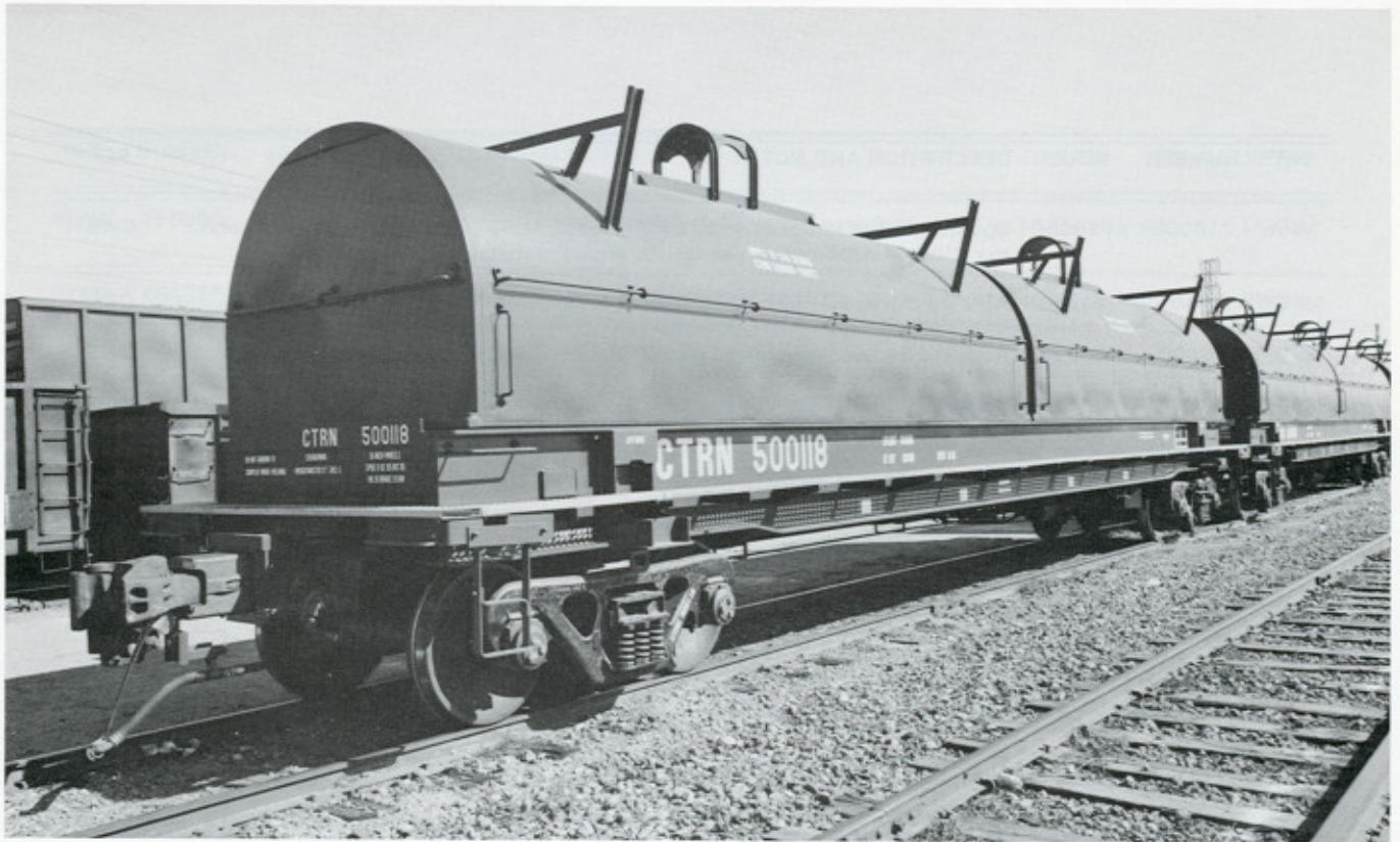
(Above) CTRN 500118 was built in September 1993 by Thrall Car. The series is being leased to Southern Pacific (SP class F-100-21) for coil steel transport. Livery is SP brown and white. CTRN are the reporting marks for the Central of Tennessee Railway & Navigation Company, Inc. (Below) GATX 29542 was built in February 1993 by Trinity. This 100-ton 30,000 gallon tank car is being leased by Minnesota Corn Processors for alcohol transport. Fremont, NE August 1993.
