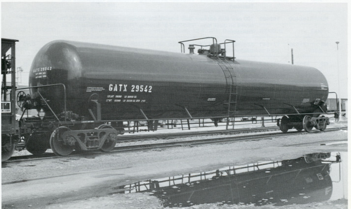
(Above) CTRN 500118 was built in September 1993 by Thrall Car. The series is being leased to Southern Pacific (SP class F-100-21) for coil steel transport. Livery is SP brown and white. CTRN are the reporting marks for the Central of Tennessee Railway & Navigation Company, Inc. (Below) GATX 29542 was built in February 1993 by Trinity. This 100-ton 30,000 gallon tank car is being leased by Minnesota Corn Processors for alcohol transport. Fremont, NE August 1993.
