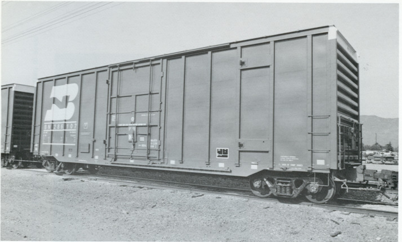
(Above and Below) BN 286084 and 296107 are part of a series of 157 high-cube 50'6" IL box cars being operated by Burlington Northern primarily for paper products transport. These are the first Trinity built box cars since the 1987 order for CSX (Gunderson has dominated the box car market since the mid-Eighties). Of note is the 10-foot plug door. All of the recent order of box cars for the BN have had 12-foot or wider door openings.
