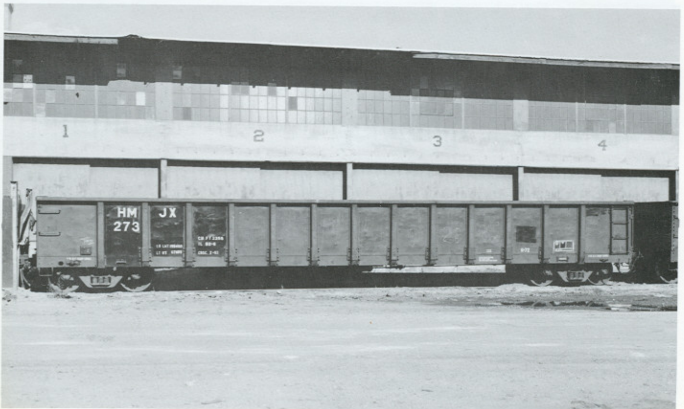
(Below) HMJX 273 was originally a Norfolk & Western class G-72 gondola with short end bulkheads. Helm had Corbin Railway Service Co cut the bulkheads off and place a new top chord on the ends. Photographed August 1993 in Salt Lake City, UT.
