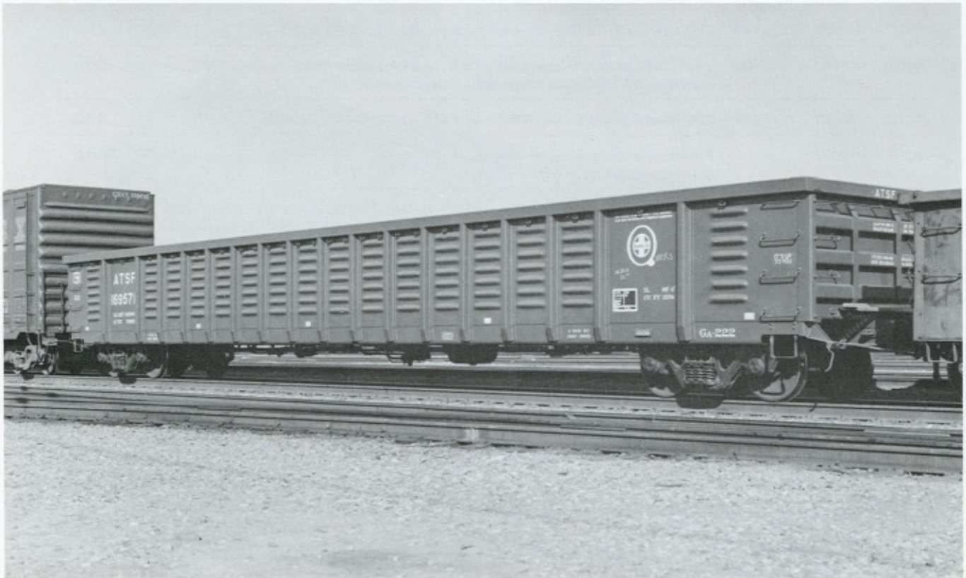
(Below) ATSF 169571 is one of the new 65'2" IL gondola cars built by Bombardier's Sahagun, Mexico in early 1993. Photographed October 1993 in San Bernardino, CA.
