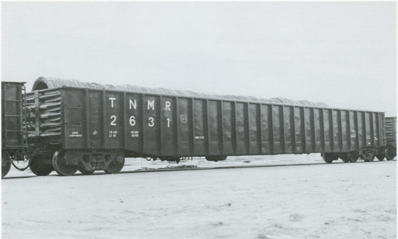
(Above) TNMR 2631 is a 66'0" IL gondola car that was refurbished in 1993 for its owner, David J. Joseph Company. TNMR 2600-2699 were formerly EJ&E 90600-series cars. (Below) WCTR 102000 is part of the 101900-102199 series delivered in 1979 by Pacific Car & Foundry. The series is currently undergoing a rebuilding program on selected cars which includes increasing the capacity from 5148 cf to 5326 cf by raising the roof.
