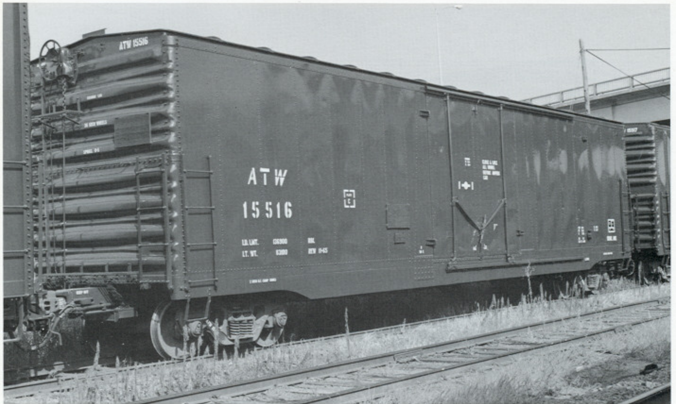
(Above and Below) ATW 15516 and ATW 15519 are part of the series, ATW 15500-15528 being leased from Helm Financial Corporation. The series of RBL refrigerator cars is a mixture of former Missouri Pacific and MKT cars. Railcar Nebraska's Omaha shops began refurbishing these in mid 1993 for operation under the Atlantic and Western Railway. Shown here August 1993 in Omaha, NE.
