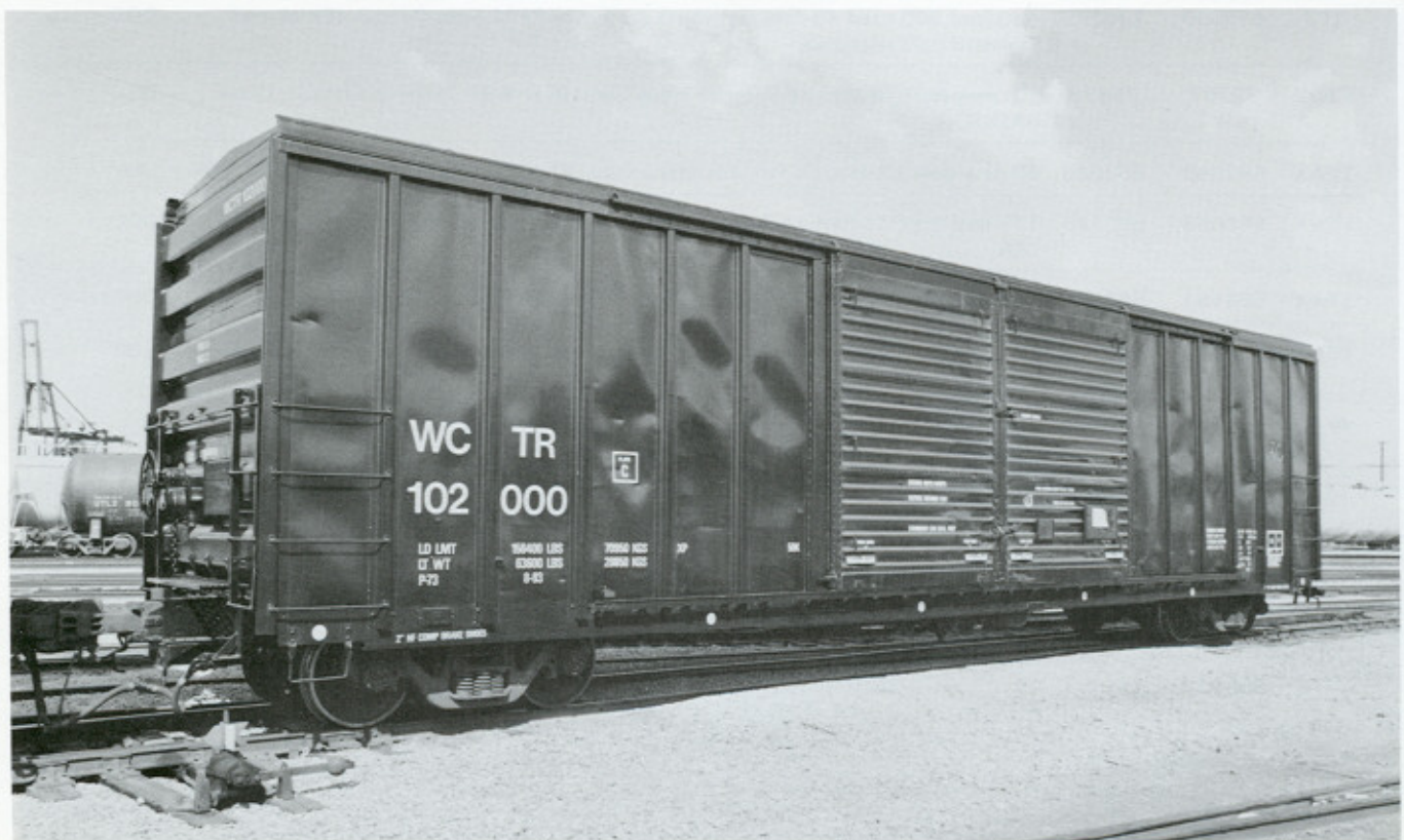
(Above) TNMR 2631 is a 66'0" IL gondola car that was refurbished in 1993 for its owner, David J. Joseph Company. TNMR 2600-2699 were formerly EJ&E 90600-series cars. (Below) WCTR 102000 is part of the 101900-102199 series delivered in 1979 by Pacific Car & Foundry. The series is currently undergoing a rebuilding program on selected cars which includes increasing the capacity from 5148 cf to 5326 cf by raising the roof.
