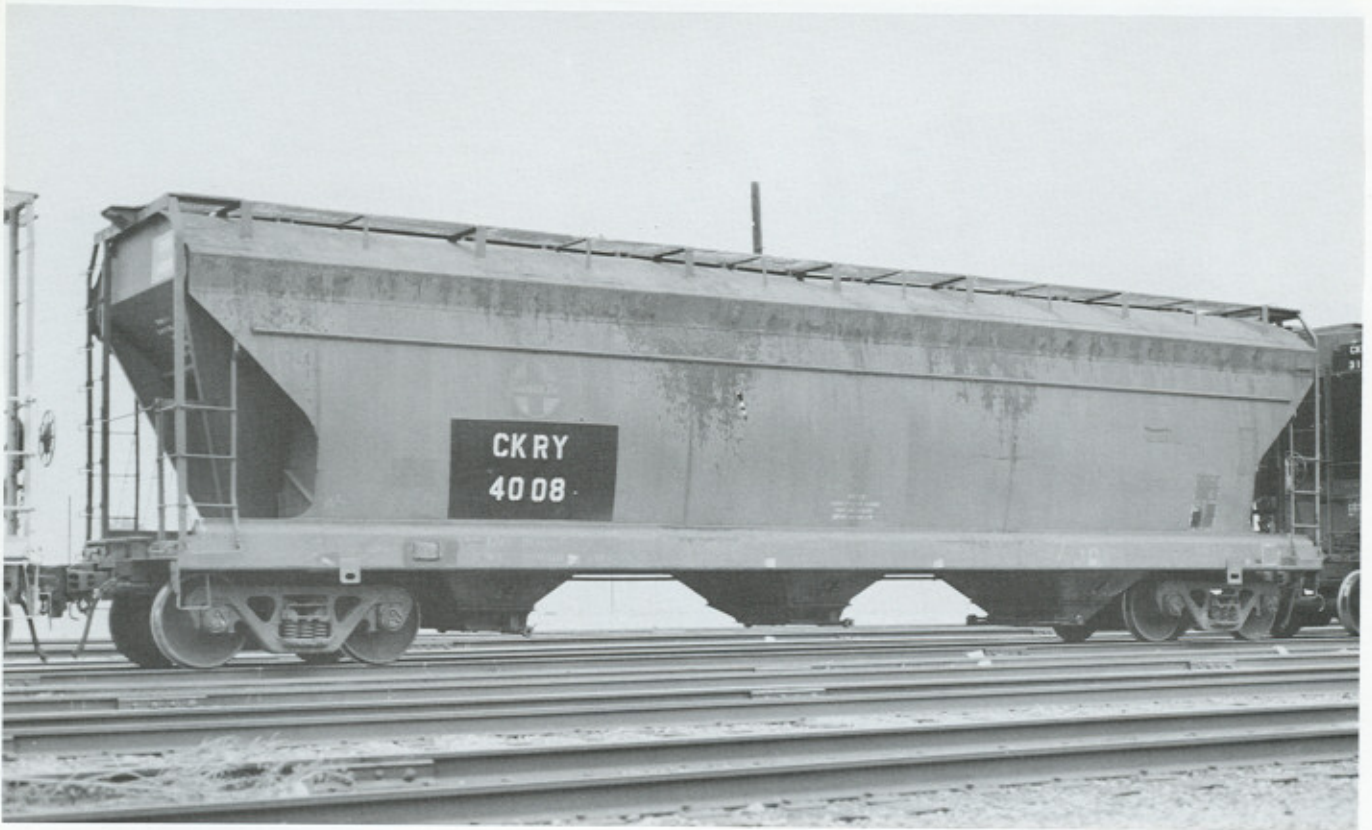
(Above) CKRY 4008. Central Kansas Railway acquired a number of former Santa Fe grain cars in 1993. This ACF Center Flow is from the Santa Fe class GA-174. Photographed November 1993 in Vernon, CA.
