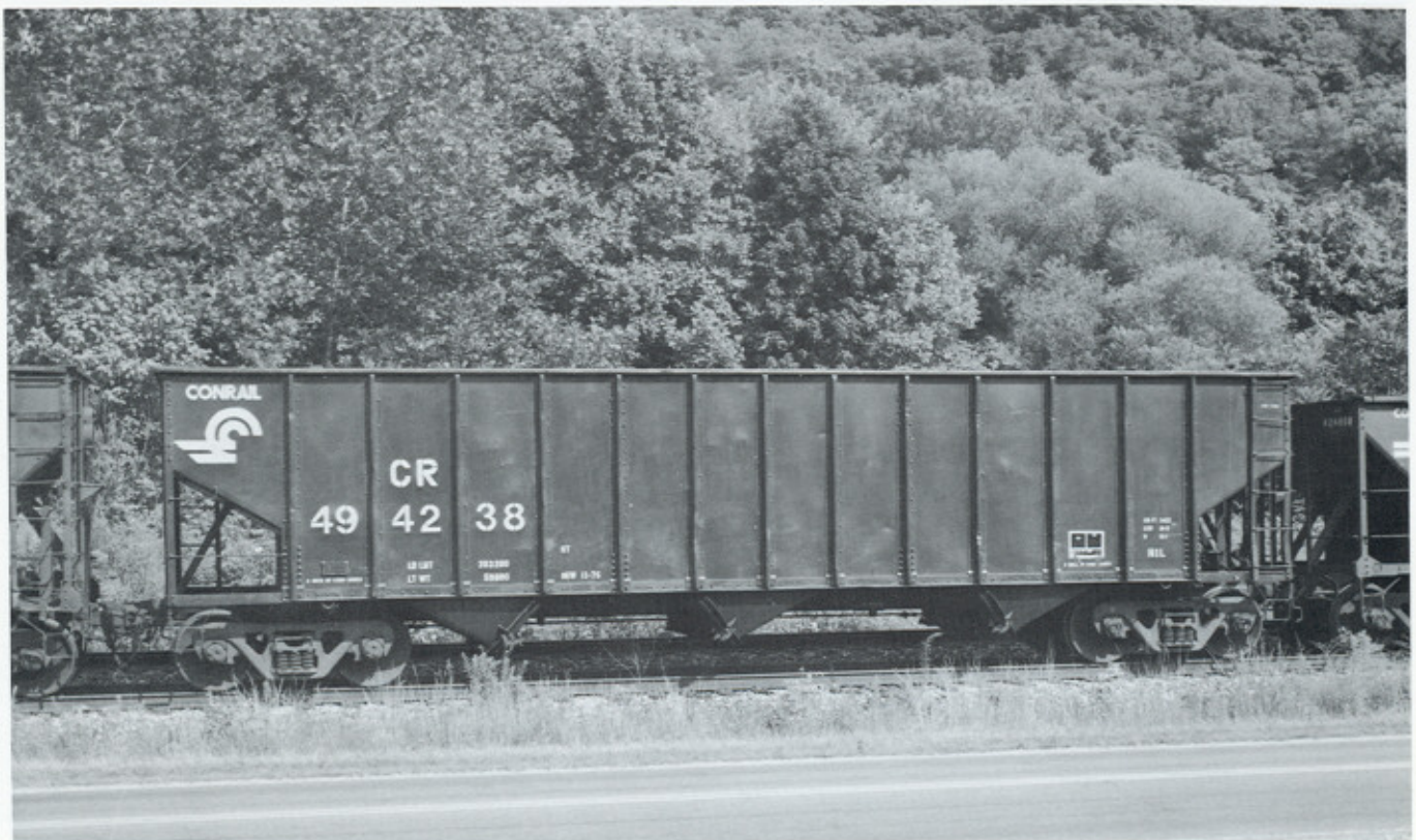
(Above) CHTT 9101 was built in 1966 as part of the MKT 9100-9130 series. The 4180 cubic foot General American Airslide covered hoppers were refurbished in early 1993 when they were transferred to the CHTT reporting mark. CHTT (Chicago Heights Terminal Transfer) is part of the Missouri Pacific which is part of the Union Pacific system. (Below) CR 494238 is part of 273 coal hoppers that were originally built for the Santa Fe (see news note for further details). Shown here in Diamond, West Virginia August 1993.
