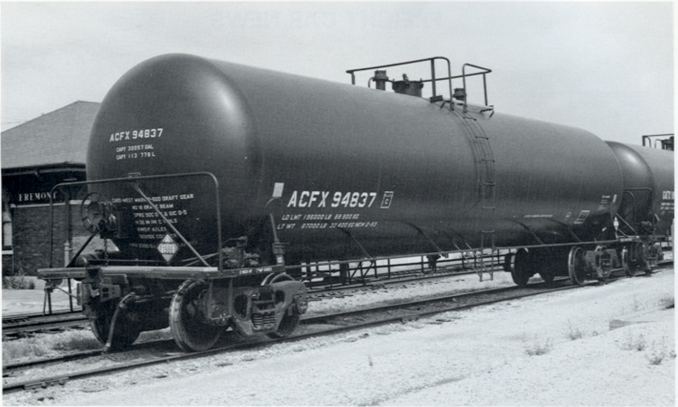
(Above) ACFX 94837 was built in February 1993 by ACF's Milton PA. This 100-ton 30,000 gallon non-insulated, non-coiled tank car is leased to Minnesota Corn Processors for alcohol transport. Photographed August 1993 in Fremont, NE. (Below) AM 627 is part of the series, AM 600-634. These are 52'6" IL gondola cars with a 2494 cubic foot capacity. This particular car has been repainted in full A&M livery complete with logo.
