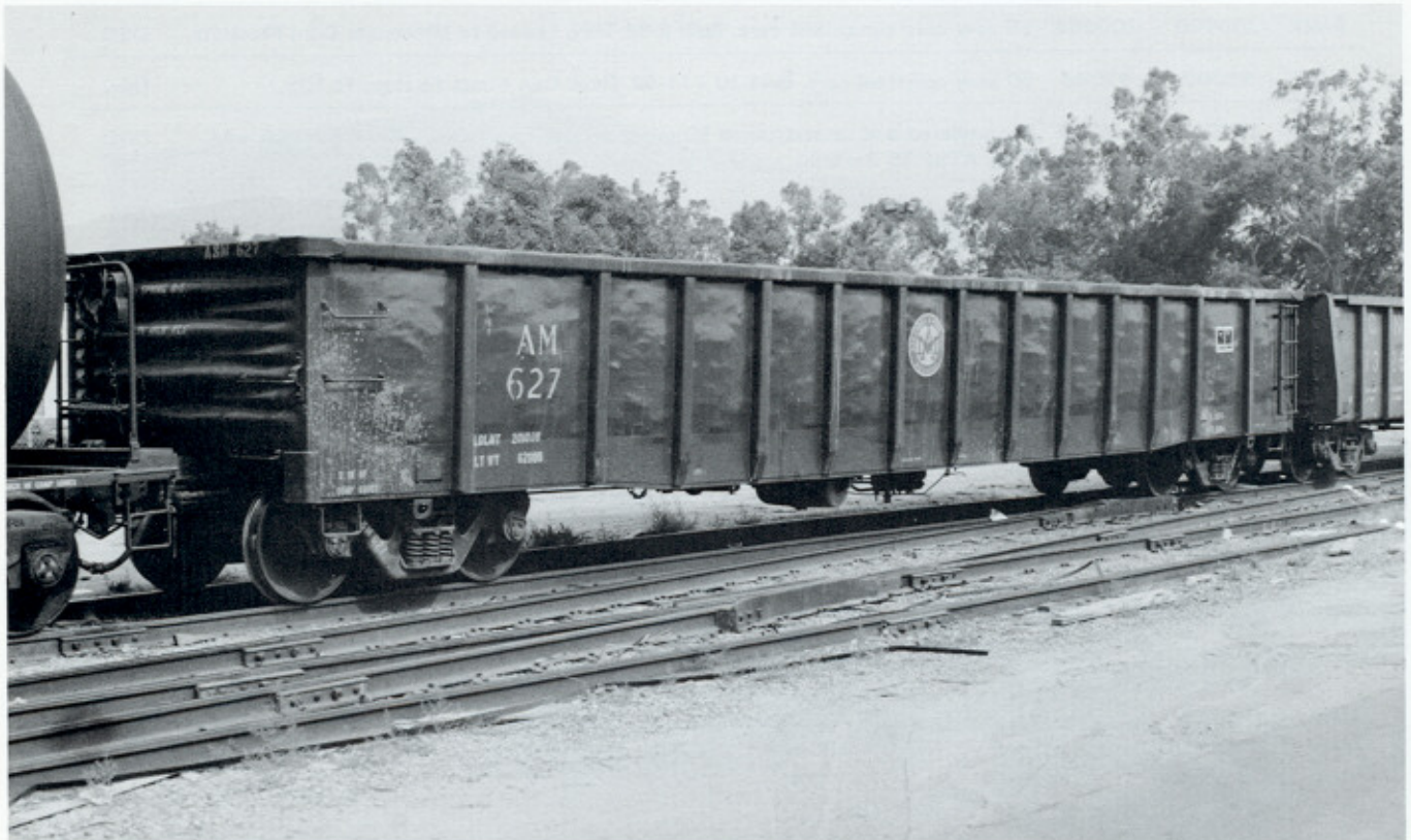
(Above) ACFX 94837 was built in February 1993 by ACF's Milton PA. This 100-ton 30,000 gallon non-insulated, non-coiled tank car is leased to Minnesota Corn Processors for alcohol transport. Photographed August 1993 in Fremont, NE. (Below) AM 627 is part of the series, AM 600-634. These are 52'6" IL gondola cars with a 2494 cubic foot capacity. This particular car has been repainted in full A&M livery complete with logo.
