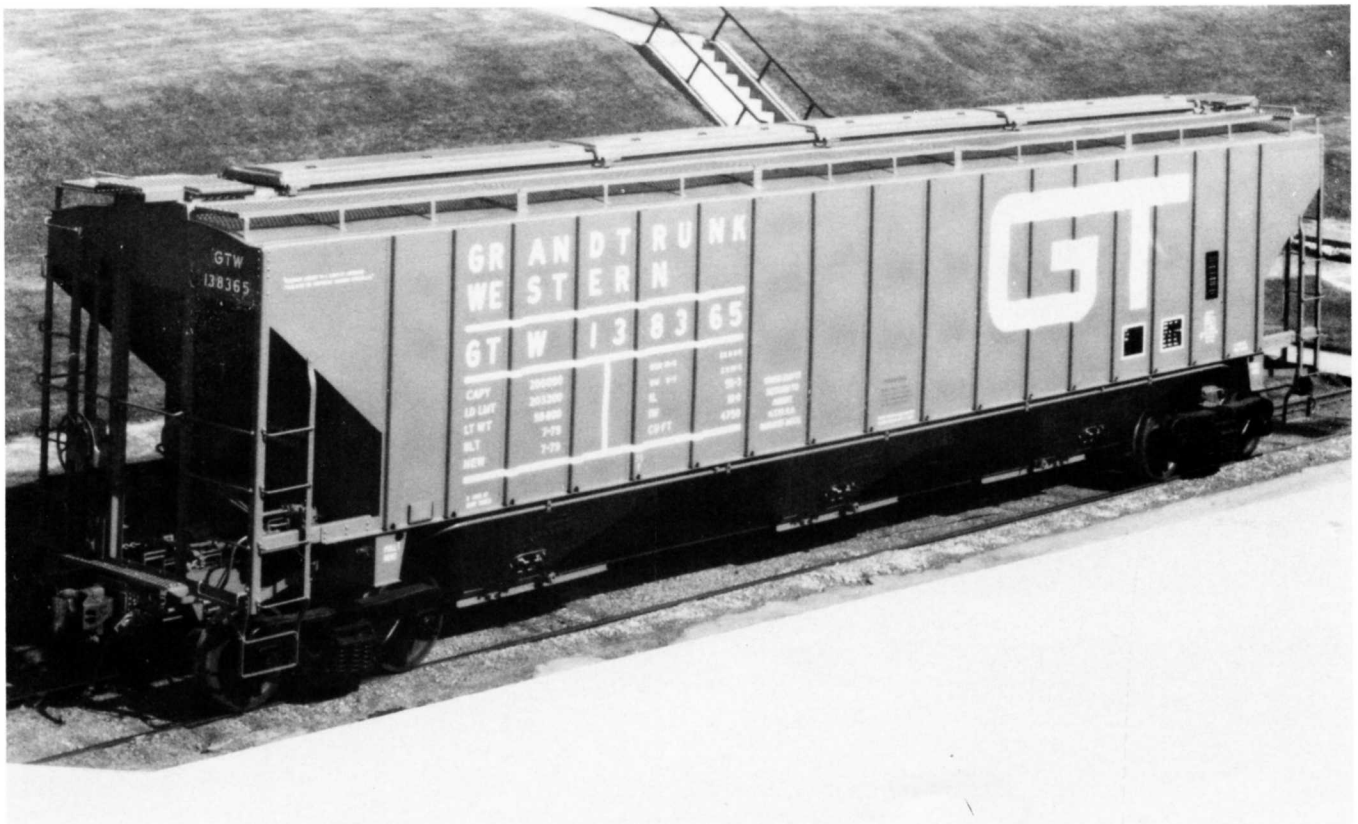
Below - GTW 138365. Built July 1979 by Pullman-Standard. Series, GTW 139350-138449. 100-ton 4750 cf covered hopper. Pullman-Standard photo, FCJ collection.
