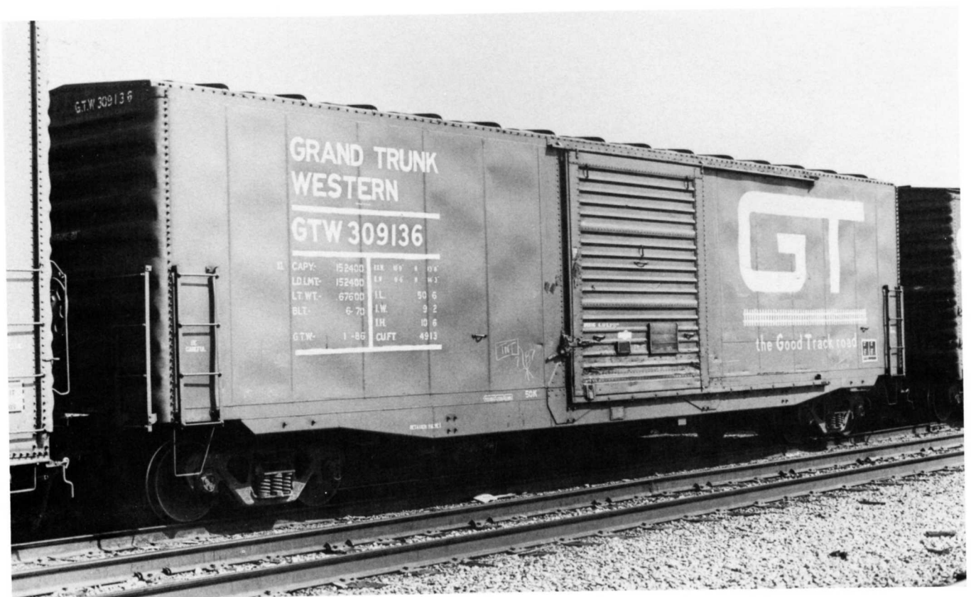
Below - GTW 309136 was built in June 1970 by Pullman-Standard as part of the GTW 309000-309299 series. 70-ton 50'6" IL 4913 cf capacity. Painted by GTW's Port Huron Shops in January 1985. Seen here in auto parts service.
