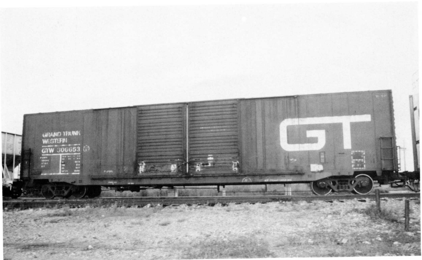
Above - GTW 306653 was built in 1968 by American Car & Foundry's St Louis plant. This 100-ton 60'9" IL 6564 cf capacity box car is used for auto parts transport. Original GTW brown and white paint scheme. Shown here passing through Kansas City, MO on September 11, 1990. James Kinkaid photo.
