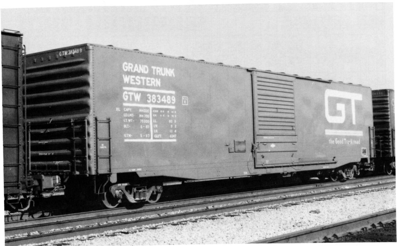
Below - GTW 383489 was built in August, 1967 at Pullman-Standard's Michigan City plant. The 60'9" Plate E box car was being used in auto parts service when photographed in late 1987. It was painted GTW blue and white in May, 1987. 6347 cf capacity.
