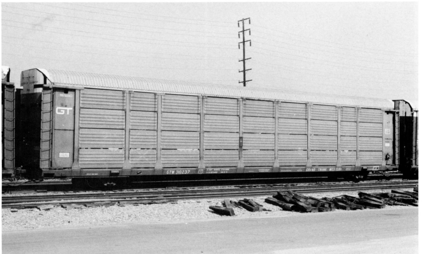
Below - GTW 310237 was built originally built as part of the GTW 304400-304453 series in 1966. It was re-racked in 1981 by Whitehead & Kales and renumbered into the GTW 310211-310256 series. GTW blue & white scheme.
