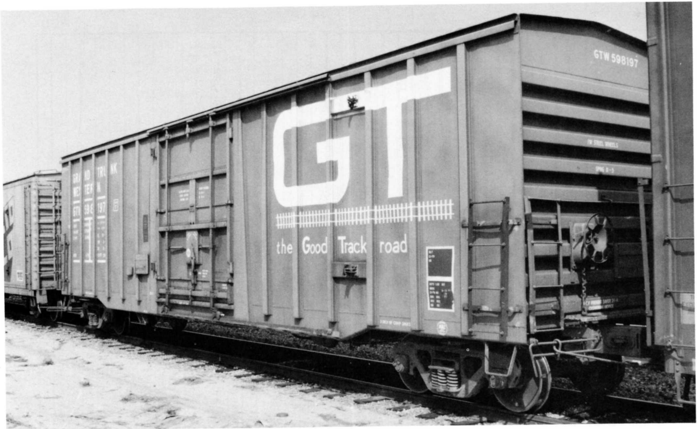
Above - GTW 598197 was built in 1979 by National Steel Car. The 70-ton 50'6" Plate C box car is part of 200 cars of the series GTW 598000-598199 built for food products transport. Note the 10'0" plug door and ACF Freight Saver 20-A cushioning device. Capacity is 5182 cf.
