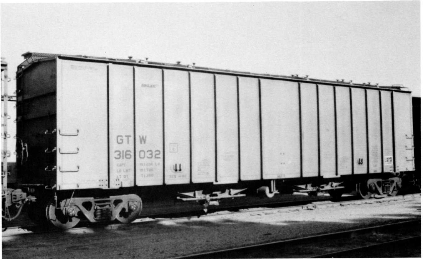
Above - GTW 316032 is a GATX Airslide® covered hopper. The series, GTW 316038-316037, was built in April 1982 at GATX's East Chicago plant. This is the 4566 cf version two-compartment airslide (other versions are 4180 cf and 4895 cf, earlier and later respectively). Mike Foley photo.
