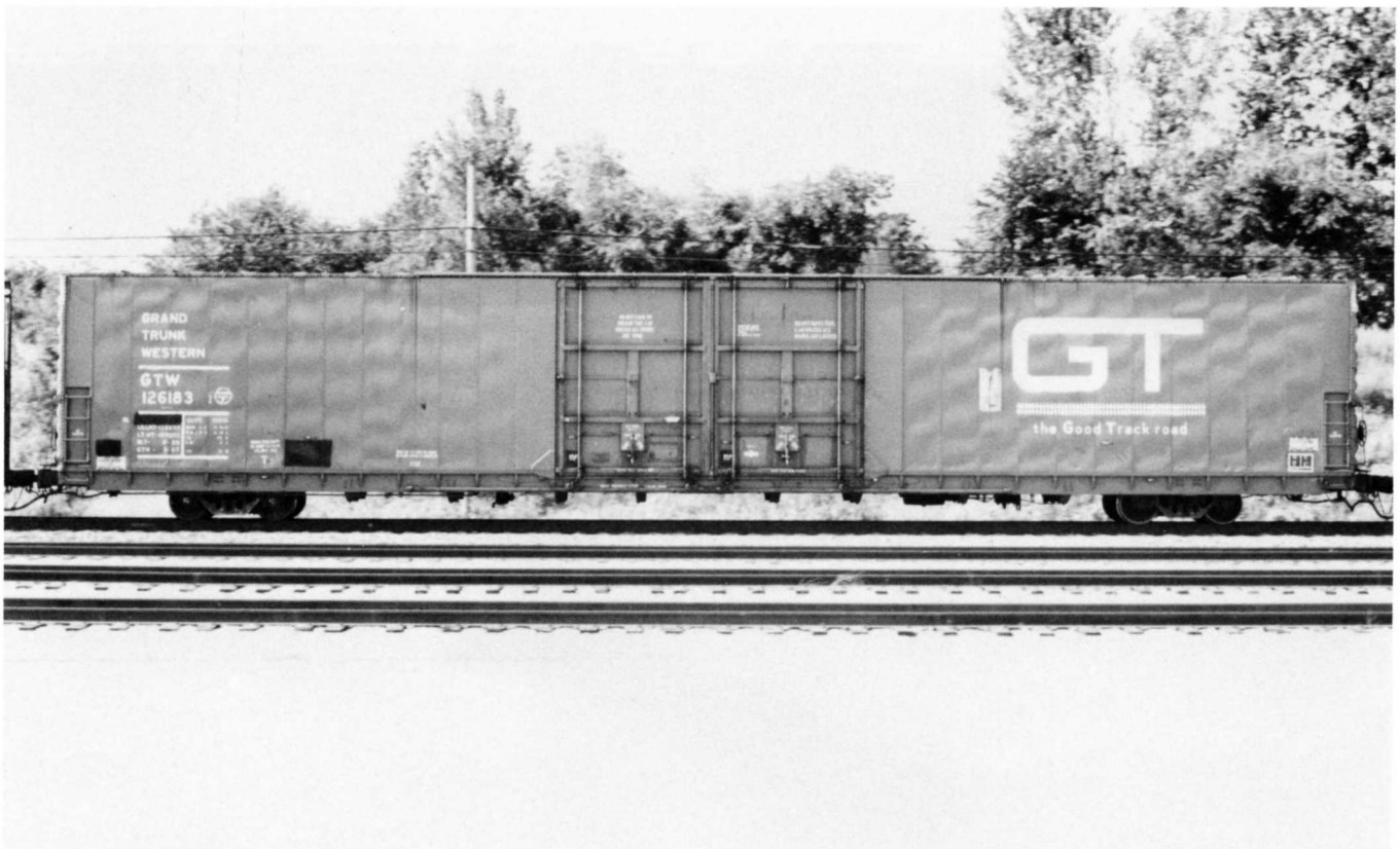
Above - GTW 126183 is part of the GTW 126100-126210 series built in 1965 by Pullman-Standard as DTI 26100-26210. 70-ton 86'6" IL 10000 cf capacity. James Kinkaid photo.
