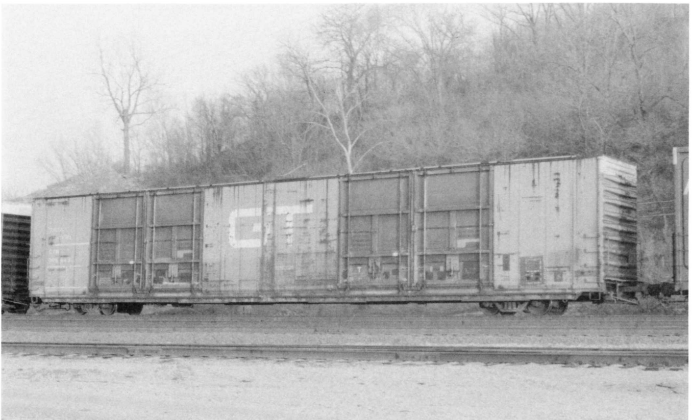
Below - GTW 305843 was built in 1969 by Greenville Steel Car. This is a 70-ton 86'6" IL 10000 cf capacity box car for auto parts service. Note the double-double door arrangement. Photographed 1992 in Kansas City, MO. James Kinkaid photo.
