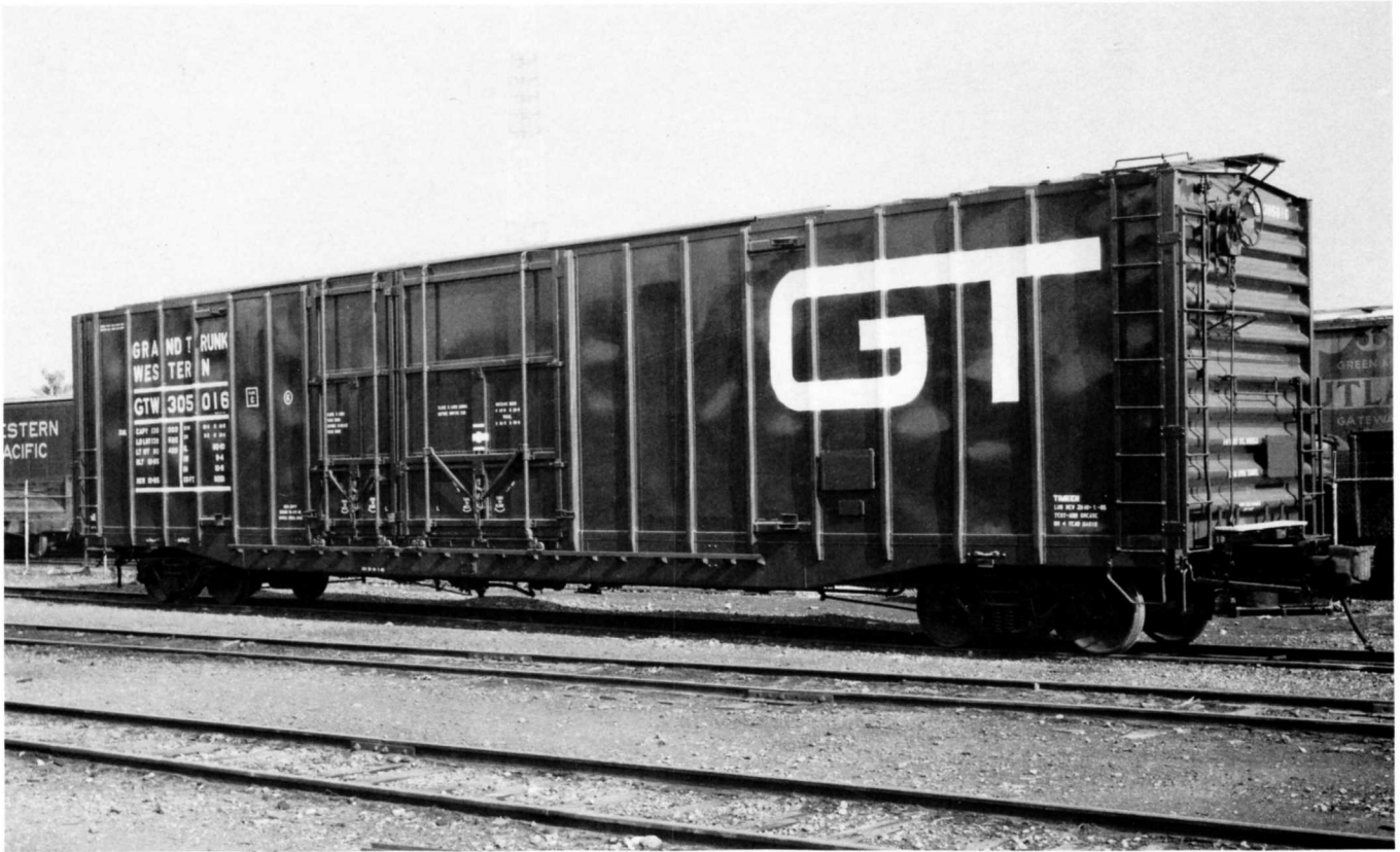
Above - GTW 305016 was built in October 1965 by Pullman-Standard's Bessemer plant. 60'10" IL 6091 cf capacity. Note 10' and 6' plug doors. The car is marked "when empty return to Battle Creek, Michigan." Photo taken October 13, 1965. (the car series this car is a part of does not appear in this roster - this photo is included for historical interest). Pullman-Standard photo, FCJ collection.
