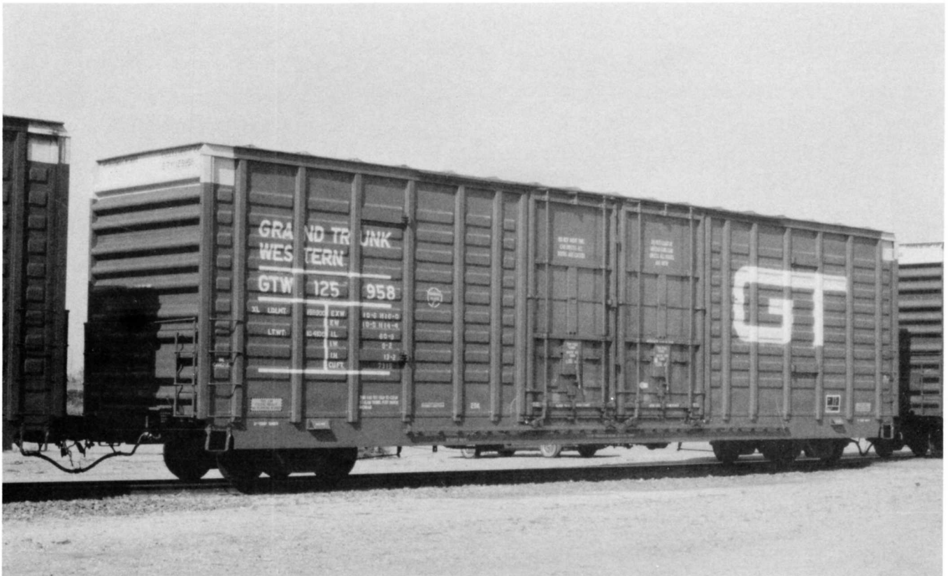
Above - GTW 125958 was built in 1974 by Pullman-Standard as part of the DTI 25950-25964 series. The 100-ton Plate F+ box car has a capacity of 7315 cf. Painted GTW blue and white scheme. Photographed September 1992 in Kansas City, MO. James Kinkaid photo.
