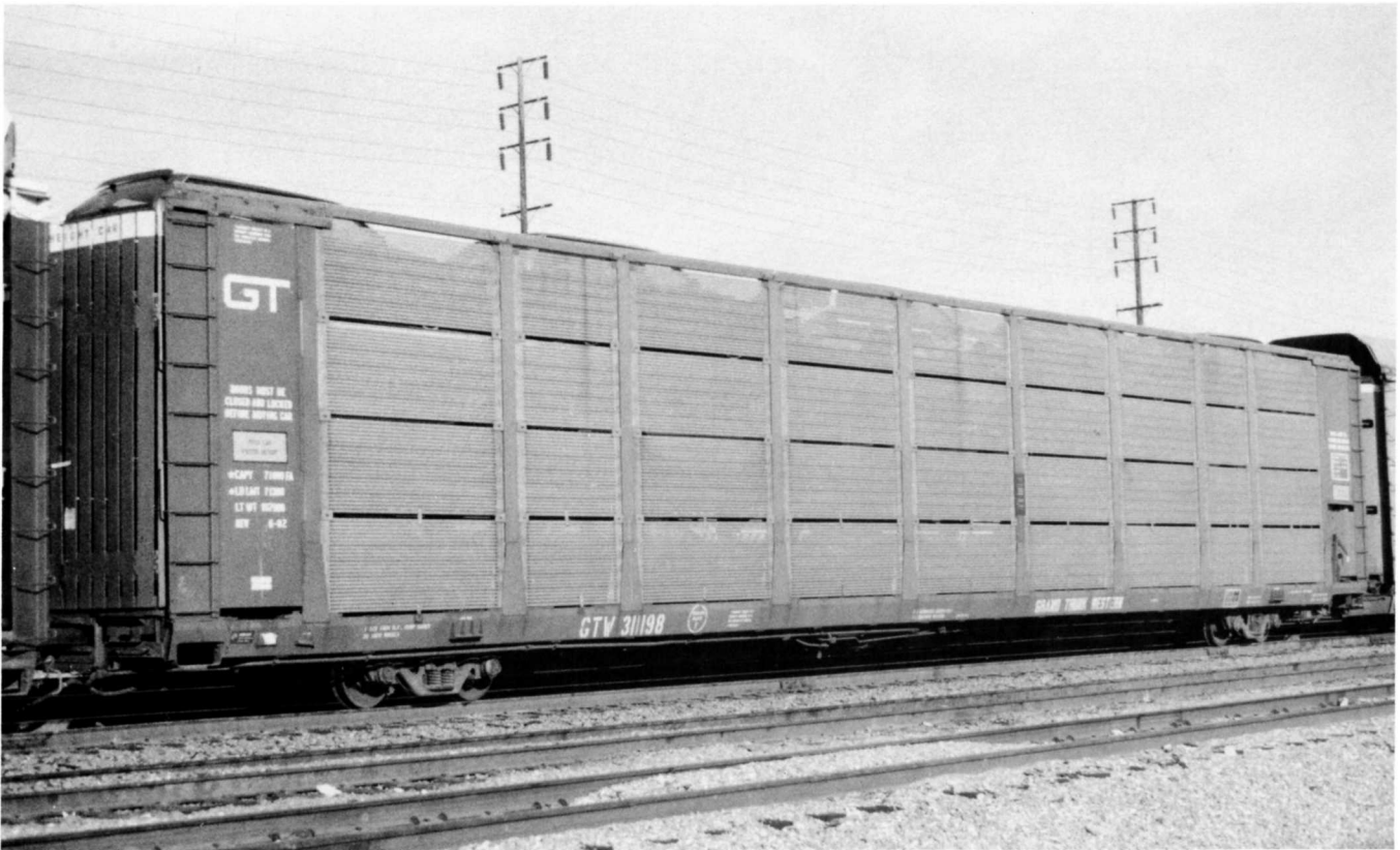
Above - GTW 311198 is part of the GTW 311157-311208 series that were originally built as GTW 304628-304735 in 1966. This car was re-racked in June 1982 by Portec. Note the R.A.V.E. doors and no roof.
