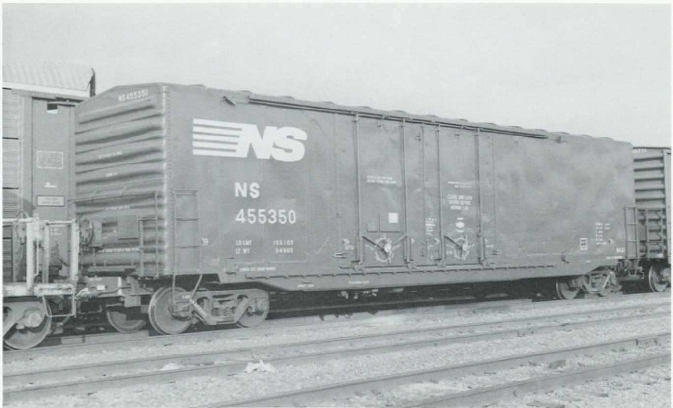
NS 455350. This car was originally built as part of the NW 160000-161999 series by ACF in 1969. It has a 70-ton 4972 cubic-foot capacity. NS class is B-121 (the "BS-121" class stencilled on this car appears to be an error). Photographed April 1993 in Atlanta, Georgia.
