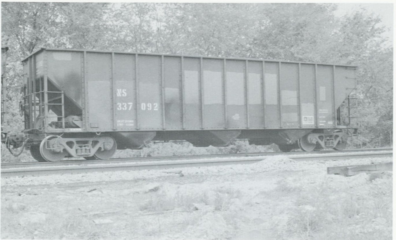
NS 337092 was originally built in 1973 by Bethlehem Steel Car as part of UP 36900-37199 (UP class H-100-9). The Norfolk Southern began leasing these from Helm in 1993. NS class H-53. Photographed April 1993 in Birmingham, Alabama.
