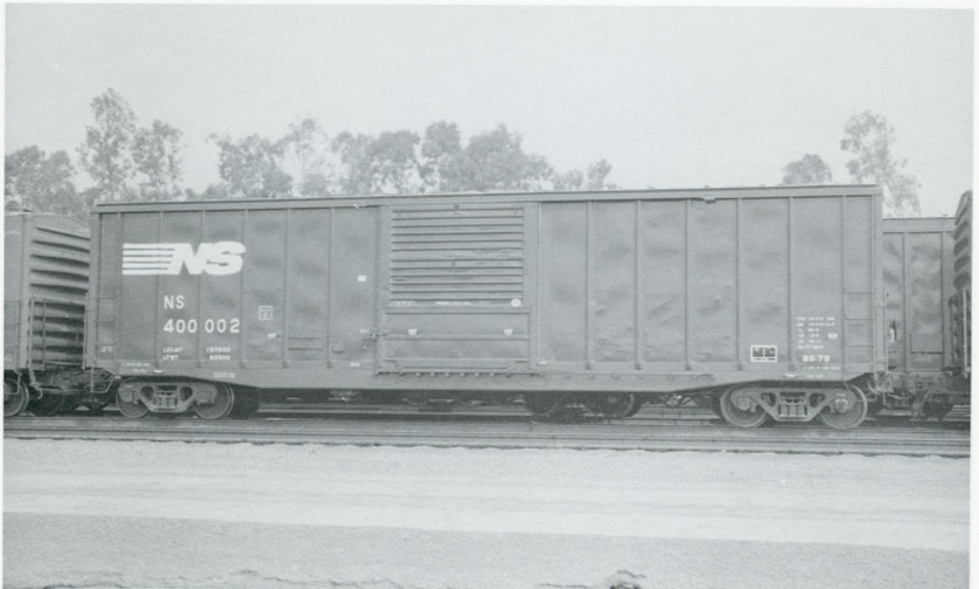
NS 400002. Originally part of the SOU 40500-41499 series built by Pullman-Standard in 1968-69. NS class BS-79. 5,219 cubic-foot capacity. Present series is NS 400000-400999. This car was repainted by Southern's Hayne Shop (Spartanburg, SC) in January 1992.
