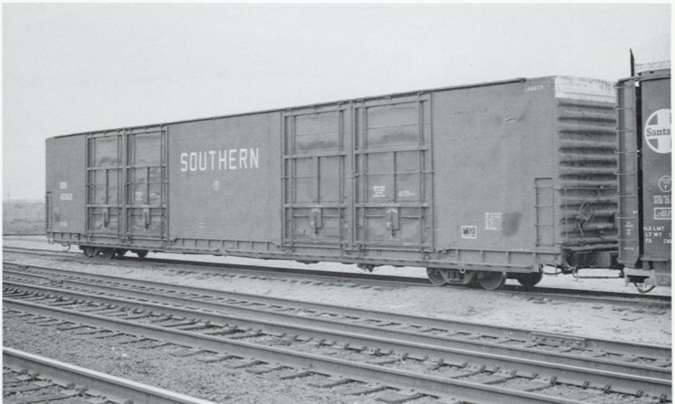
SOU 42360. This 70-ton 10,000 cubic-foot capacity 86'6" IL box car was built in February 1965 by Pullman-Standard. Note the "ribbed" lower side sills characteristic of the Pullman-Standard design. This car was painted in the interim paint scheme before the NS began stenciling classes on the cars.
