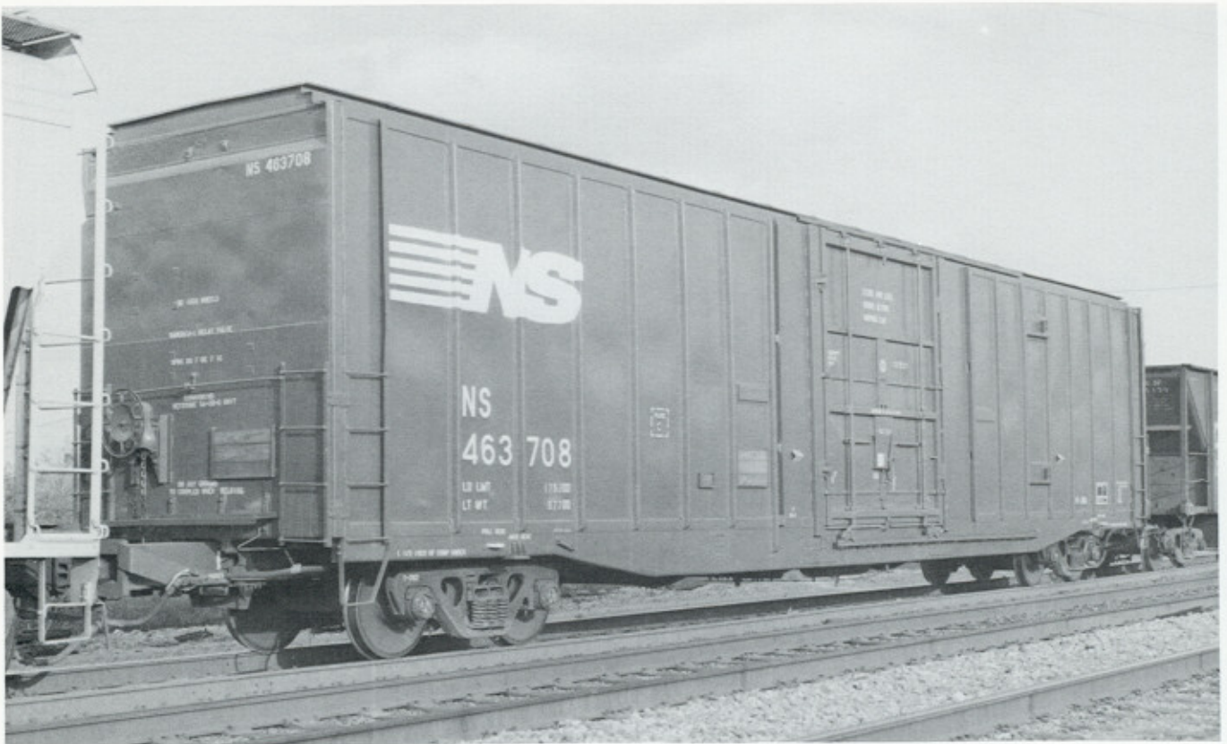
NS 463708 was rebuilt in November 1992 by Kustom Karr in Green Cove Springs, FL from the SOU 16080-16399 series. It originally had a double door with a 16-foot opening. When it was rebuilt a new 10-foot YSD plug was installed and the three-foot on either side of the door was filled. The roof was also rebuilt to a new configuration. Photographed April 1993 in Atlanta, Georgia.
