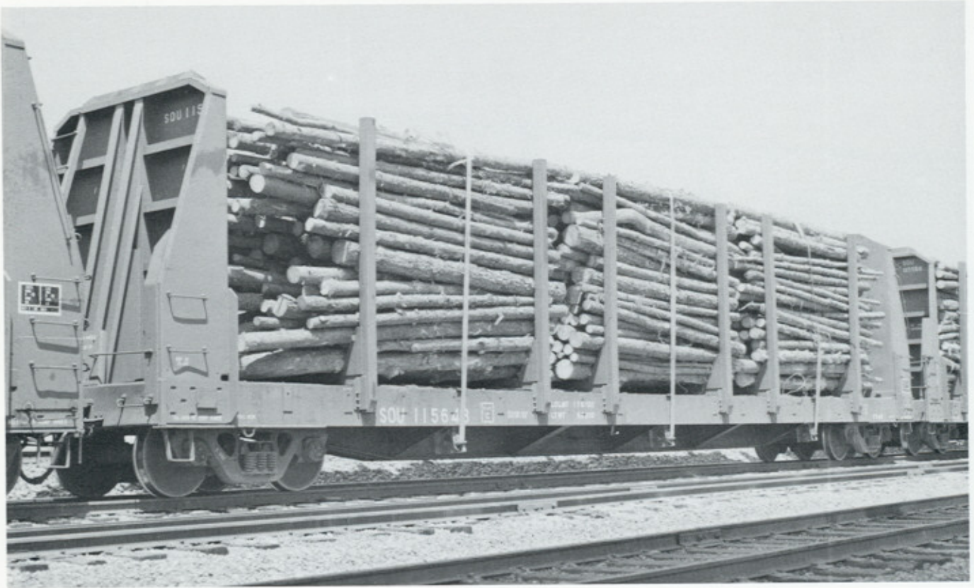
SOU 115648. This 58'6" bulkhead flat car was built in 1965 by Thrall Car. NS class FS-60. The cars come equipped with twelve permanent steel stakes and three lading band tie-downs. The car was painted in December 1989. Series, SOU 115600-115699.
