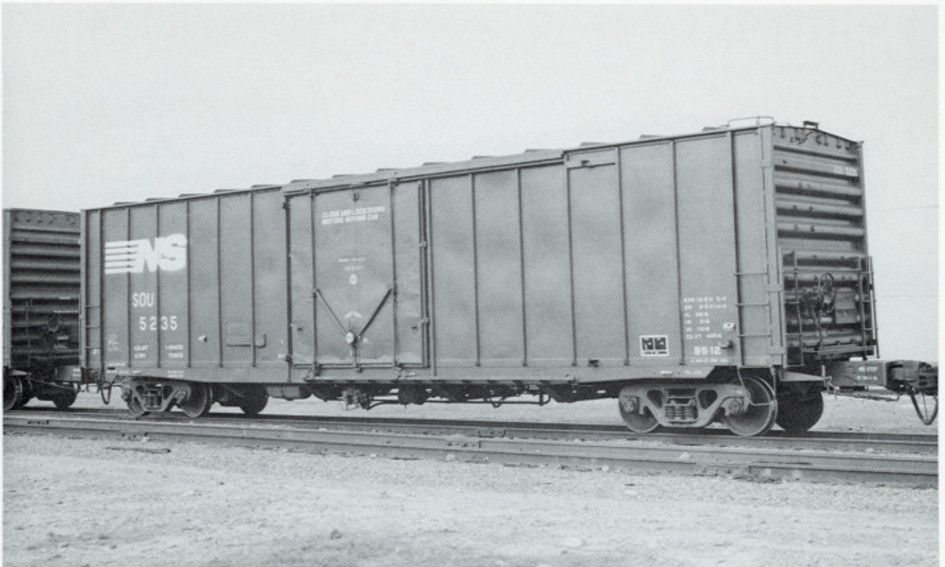
SOU 5235 was built in 1963 by Pullman-Standard's Bessemer, AL plant. Series is SOU 5000-5499. This car has a 70-ton 4954 cubic-foot capacity. Inside length, 50'6". The car was painted in January 1989 by the Southern. NS class BS-12. Photographed March 1991 in central California.
