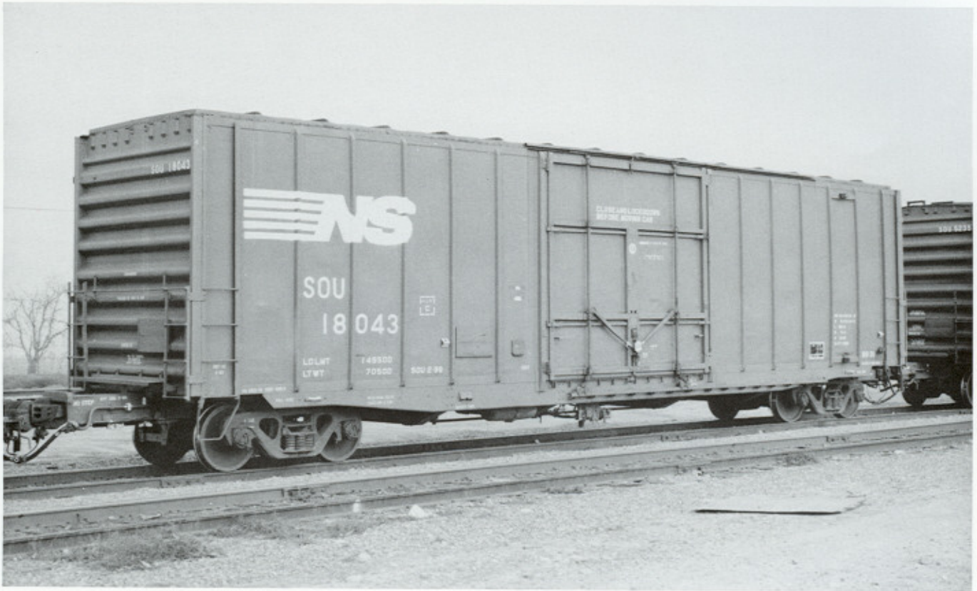
SOU 18043 is part of the series SOU 18000-18499. Built in 1965 by Pullman-Standard's Bessemer, Alabama plant. The car has a 70-ton 5,139 cubic-foot capacity. 50'6" IL. Note the wide 12'0" plug door. Painted in February 1989 SOU HE. Photographed March 1991 in central California.
