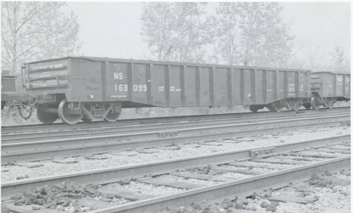
NS 168099 was originally built in May 1964. Series, NS 168000-168099. NS class PS-5. Capacities are 100-tons or 1,911 cubic-feet. 52'6" IL. Equipped for coil steel service. Note the 91,600 lb light weight. Photographed April 1993 in Birmingham, Alabama.
