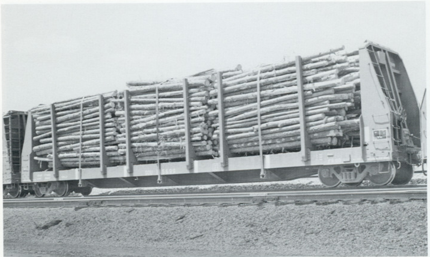
SOU 115699. Another car of the FS-60 class. This one was painted in November 1989. Notice the long 55'6" truck centres. Both of these cars were photographed April 1993 in Doraville, GA
