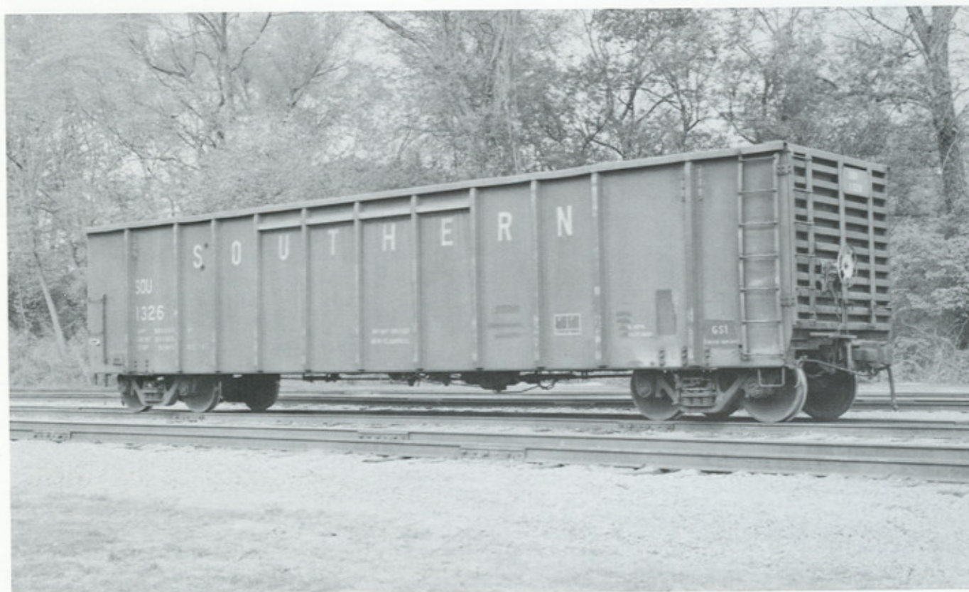
SOU 1326 is part of the SOU 1000-1749 series built by Pullman-Standard in 1960. It's one of the first aluminum GT gondola cars placed into service. Capacities are 105-tons or 3,620 cubic-feet. NS class GS-1. Photographed April 1993 in Atlanta, GA
