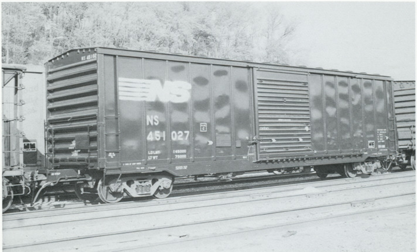
NS 451027 was built in 8-70 by Pullman-Standard as part of the SOU 550000-550949 series. 70-ton 5,219 cubic-foot capacity. 50'6" IL. This car was repaired and painted April 1992 by the Hayne Shops. Photographed just after leaving the shop in Asheville, NC.
