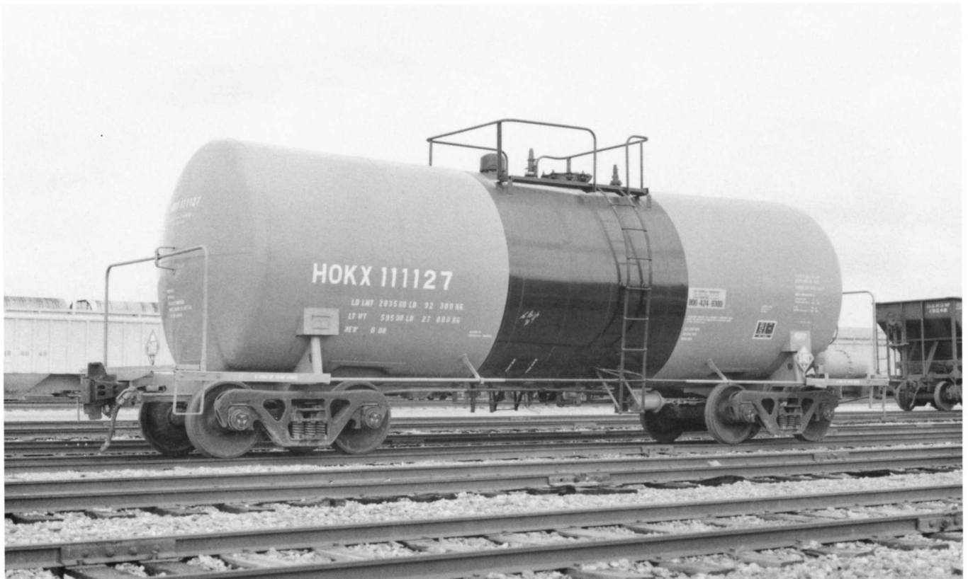
Below - HOKX 111127. Built in August 1988 by Union Tank Car Co. Caustic soda transport. Capacity 16,478 gallons. AAR car type code T104. DOT 111A100W1. Gray with black center band. White lettering. Lined with Plaschem 2310 September 1986 at Union Tank Car Altoona, PA. Length 42'3".
