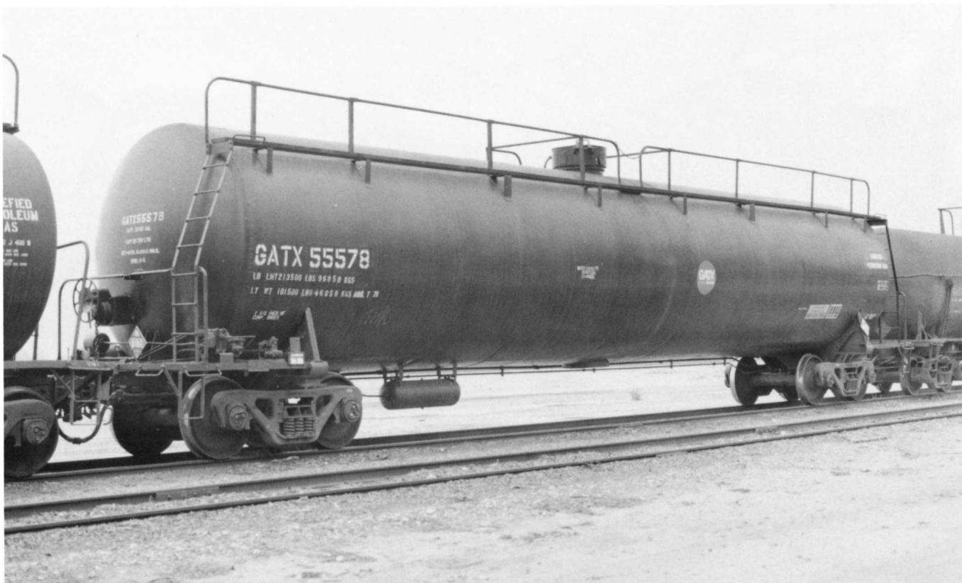
Below - GATX 55578. Built in December 1968 by GATX Sharon. Liquefied Petroleum Gas transport. 125-ton trucks (note the brake reservoir below). AAR car type code T389. DOT 112J340W. Capacity 32,160 gallons. Length 62'11".
