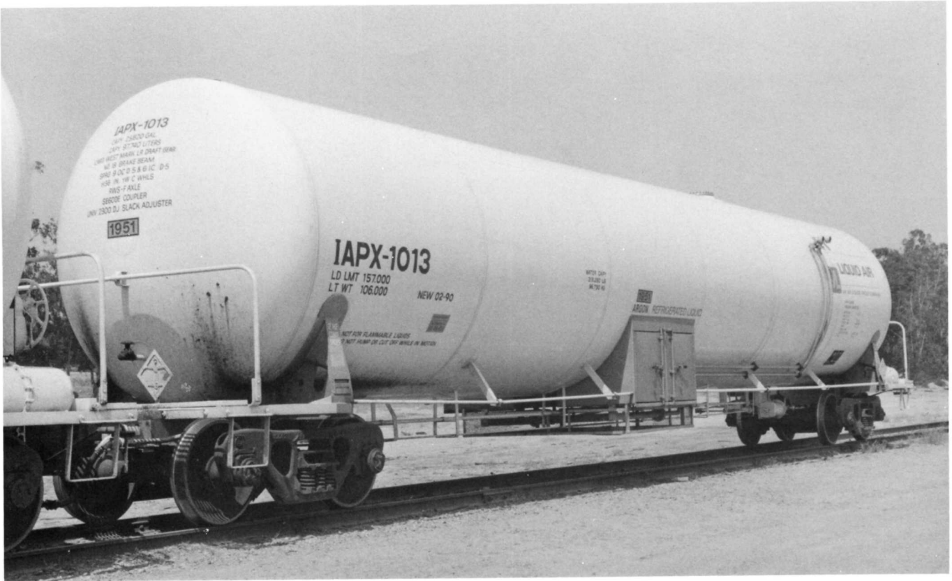
Above - IAPX 1013. Built in February 1990 by ACF MILT. Capacity 25,820 gallons. Argon transport. AAR car type code T767. AAR class 204W. IAPX is currently the reporting mark for Liquid Air Corporation.
