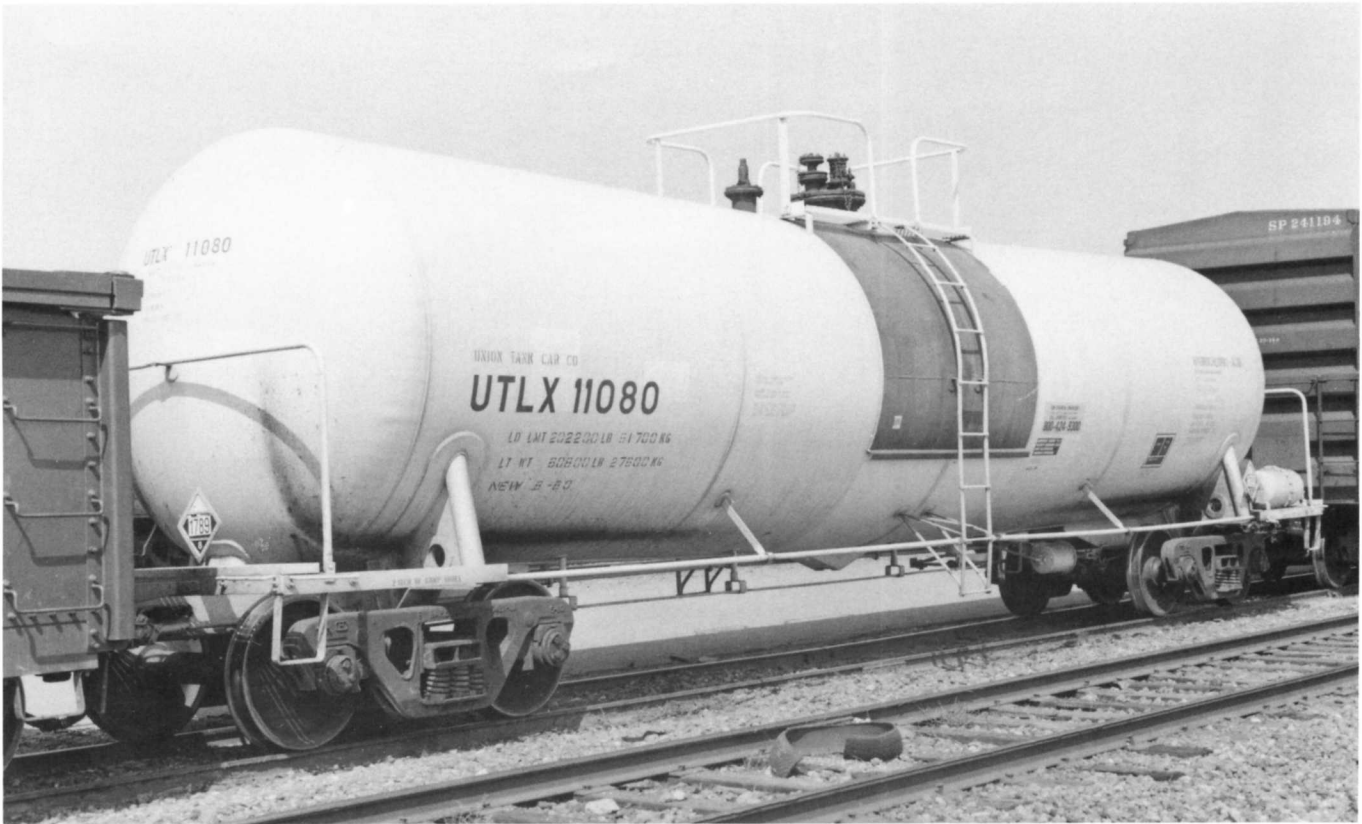
Above - UTLX 11080. Built in August 1980 by Union Tank Car Co. Hydrochloric acid transport. Capacity 20,561 gallons. Leased to Miles Inc. DOT 111A100W5. Lined with Uniroyal 5872 in September 1986 by Akron Rubber Co.
