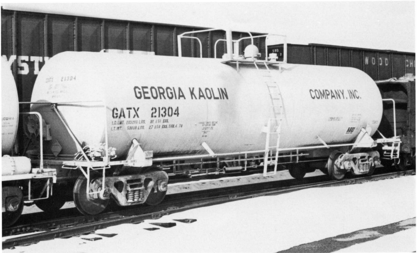
Above - GATX 21304. Built in April 1978 by GATX Sharon. Clay slurry transport. AAR car type code T104. Leased to Georgia Kaolin Company Inc. DOT 111A100W1. Capacity 14,004 gallons. Insulated. Length 45'10". Oscar Kimsey photo.
