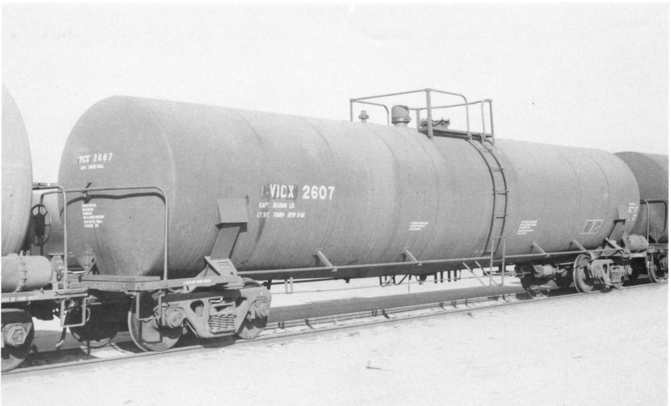
Above - VICX 2607. Built in August 1981 by Trinity Industries. Capacity 23,622 gallons. AAR car type code T106. Insulated. Equipped with heater coils. Note the early Trinity saddles close resemblance to North American designs. Photographed December 1991. Length 59'8".
