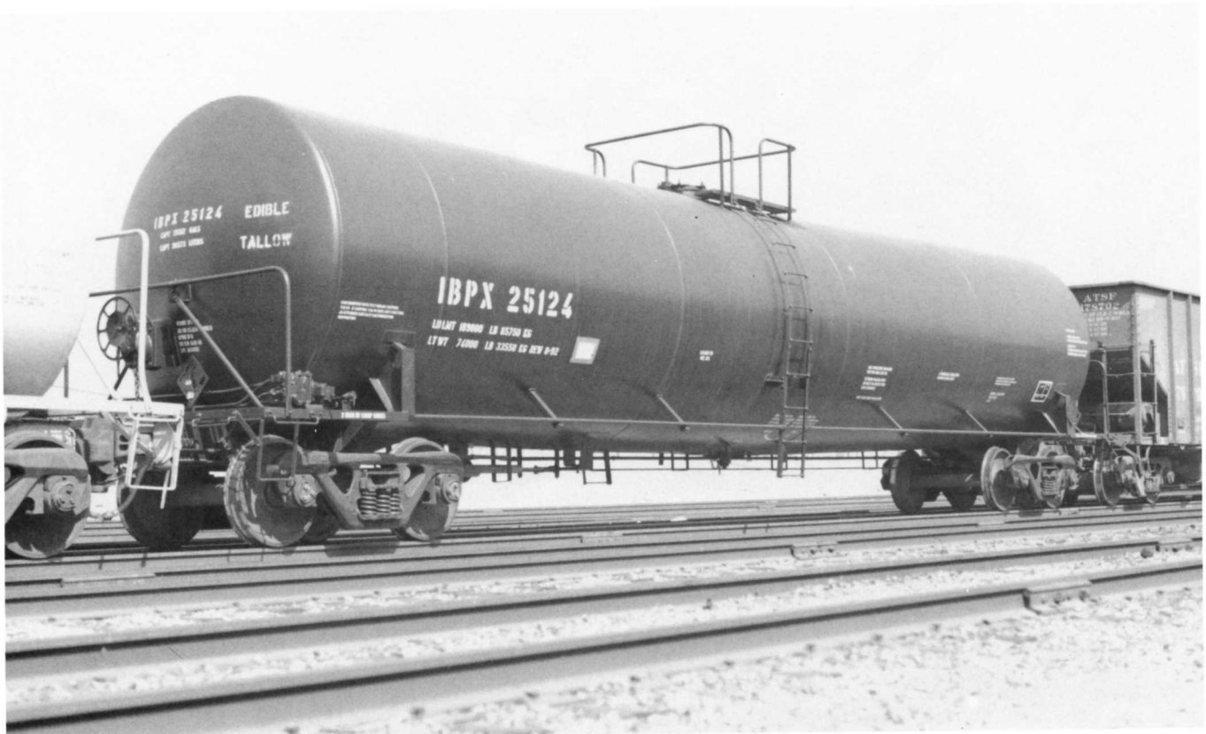
Below - IBPX 25124. Built in August 1992 by Trinity Industries. Tallow transport. Capacity 25,512 gallons. AAR car type code T107. Length 59'4".
