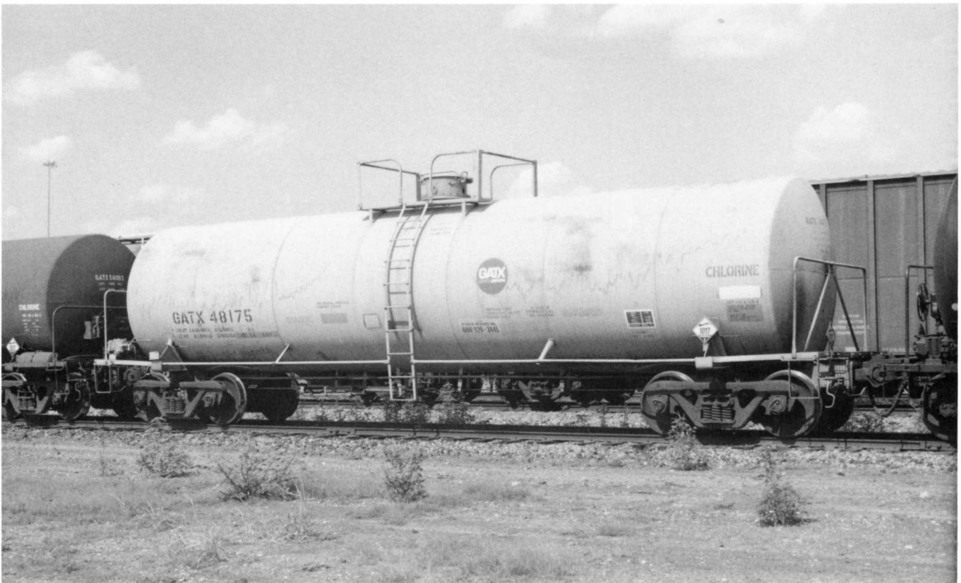
Above - GATX 48175. Built August 1976 by GATX Sharon. Part of series, GATX 48151-48270. Chlorine transport. Capacity 90-tons. DOT 105A500W. Insulated. No Coils. AAR car type code T564. Leased to Occidental Chemical Co. Photographed August 1991 in Ft. Worth TX. Length 48'4".
