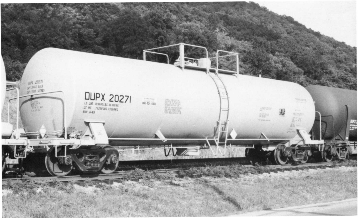
Above - DUPX 20271. Formaldehyde transport. Part of series, DUPX 20257-20281. Capacity 20,663 gallons. DOT 111A100W1. AAR car type code T105. Photographed August 1985 in Diamond WV.
