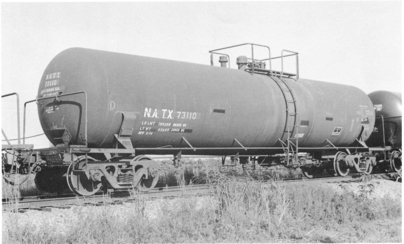
Above - NATX 73110. Built in March 1974 by NACC TX. Capacity 20,594 gallons. AAR car type code T105. Non-insulated. Length 52'10".
