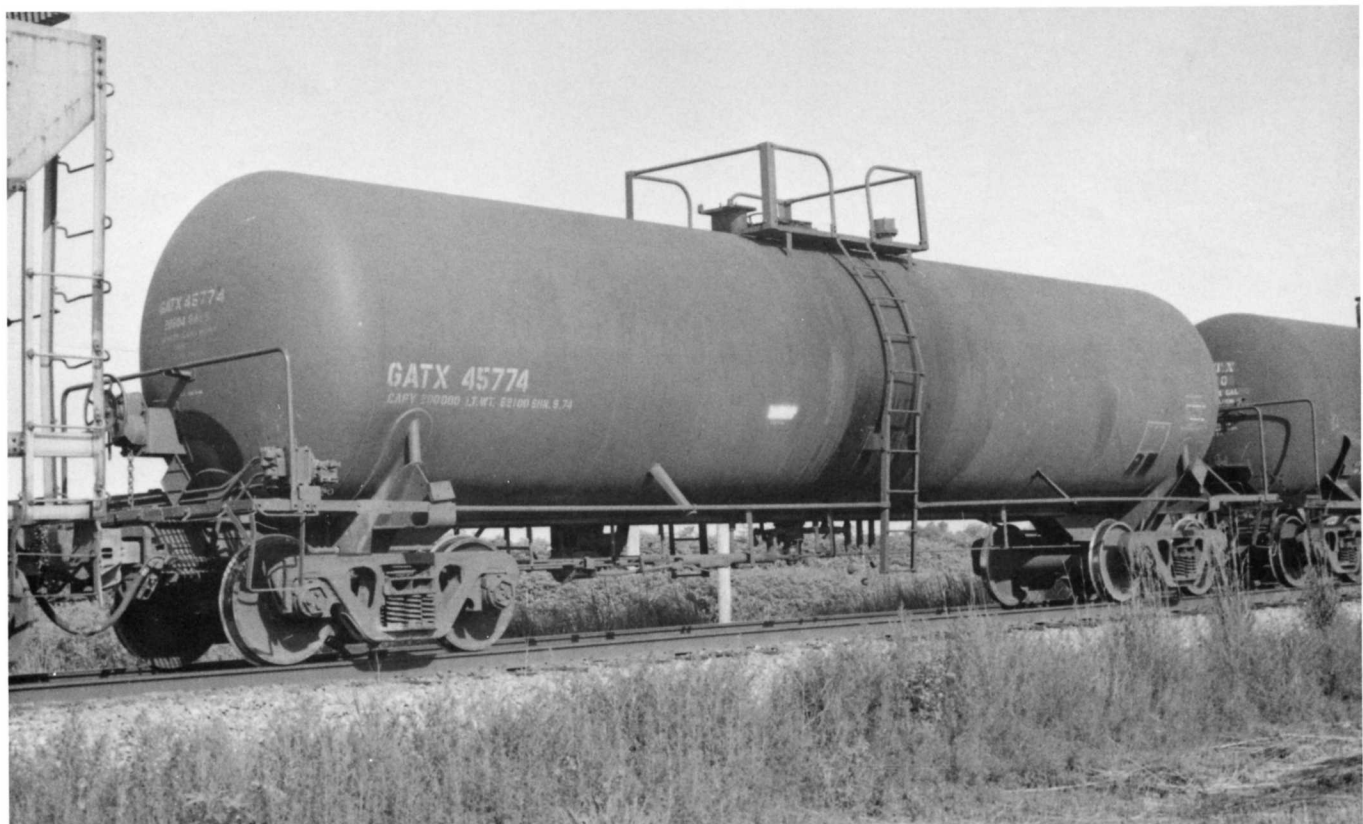
Below - GATX 45774. Built in September 1974 by GATX Sharon. Capacity 20,604 gallons. AAR car type code T105. Non-insulated. Heater coil equipped. DOT 111A100W1. Length 51'4".
