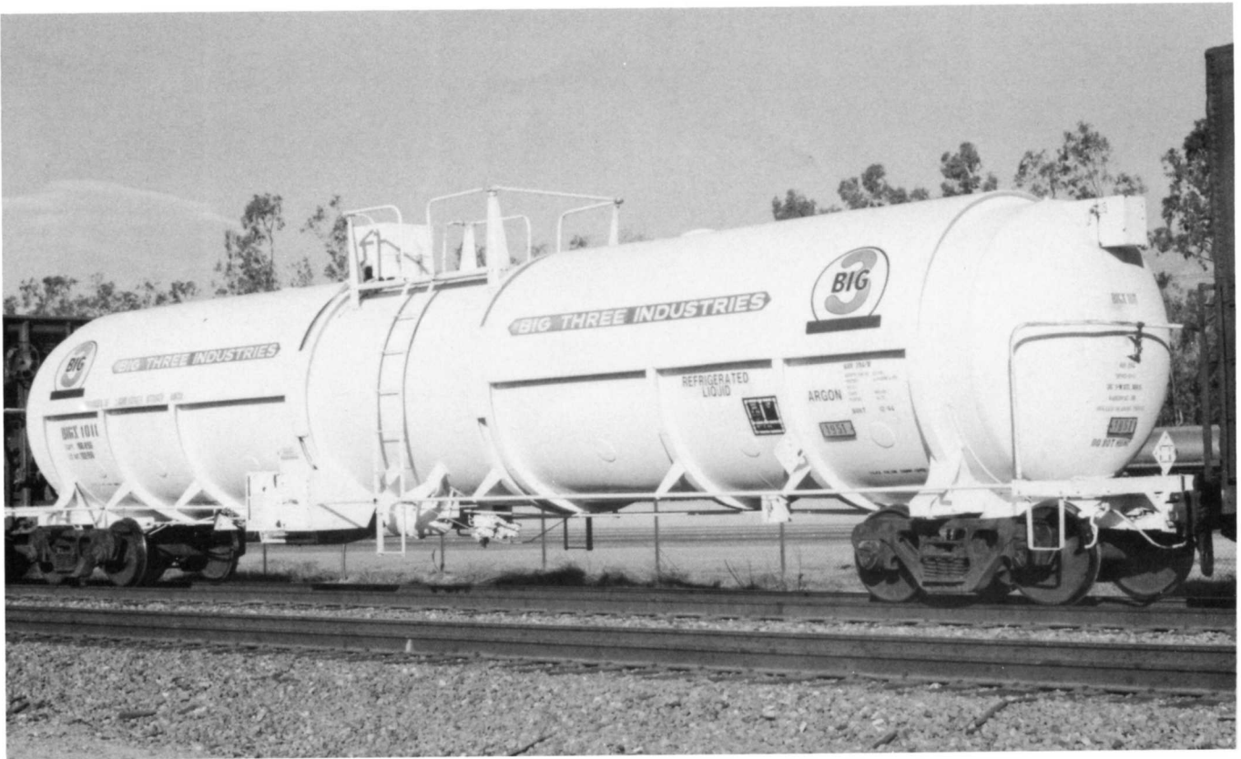
Above - BIGX 1011. Built in December 1964. Argon transport. AAR class 204-W. AAR car type code T764. Monoseries car. Big Three Industries cars are now a part of the Liquid Air Corporation.
