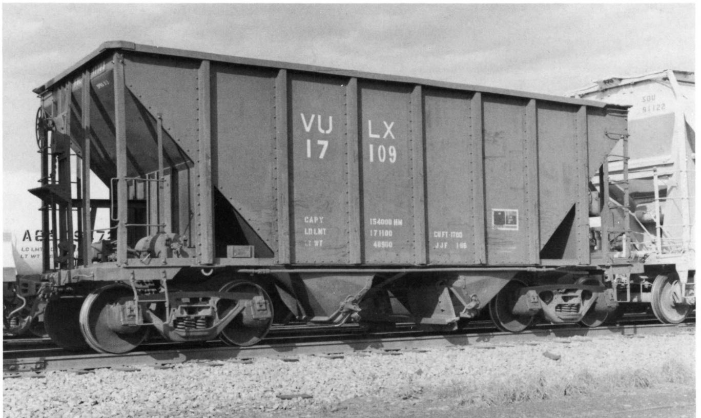
Below - VULX 17109. Vulcan Materials Company, Construction Material Group presently has six of these 1700 cf 70-ton HM type hopper cars in service. This car was built in April 1961. It was painted and repaired by Finnigan Industries Inc in April 1986. Photographed April 1993 in Atlanta GA. David G. Casdorff photo.
