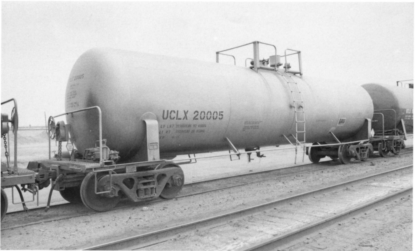
Above - UCLX 20005. Built in June 1975 by Richmond Tank Car Houston TX. Methyl Chloroform transport. AAR car type code T105. This is probably the closest prototype to the MDC 50-foot tank car in HO scale. Non-insulated. Length 50'7".
