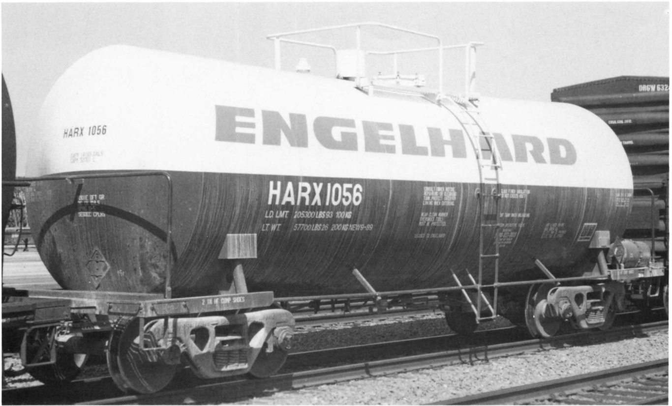
Above - HARX 1056. Built in September 1989 by Hargis. Clay slurry transport. Capacity 14,169 gallons. DOT 111A100W1. Leased to Engelhard. Insulated. For a short time Hargis built tank cars in Gordon GA of Union Tank Car design. All known production were for clay slurry transport.
