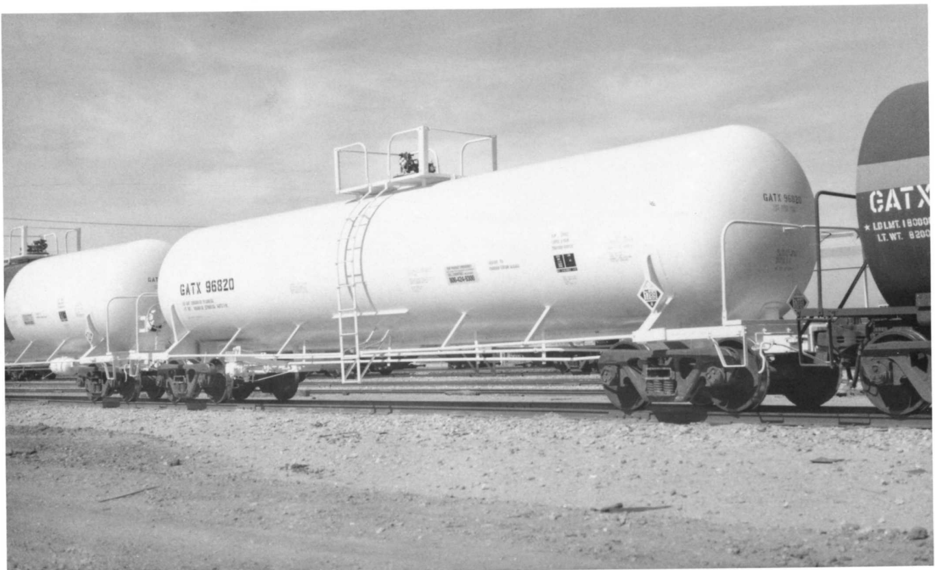
Below - GATX 96820. Built in March 1966 by GATX Sharon. Rebuilt in January 1991 to a DOT 111A100W5 for hydrochloric acid transport. Capacity 20,528 gallons. AAR car type code T055. Length 56'3". Leased to Pioneer Chloroalkali.
