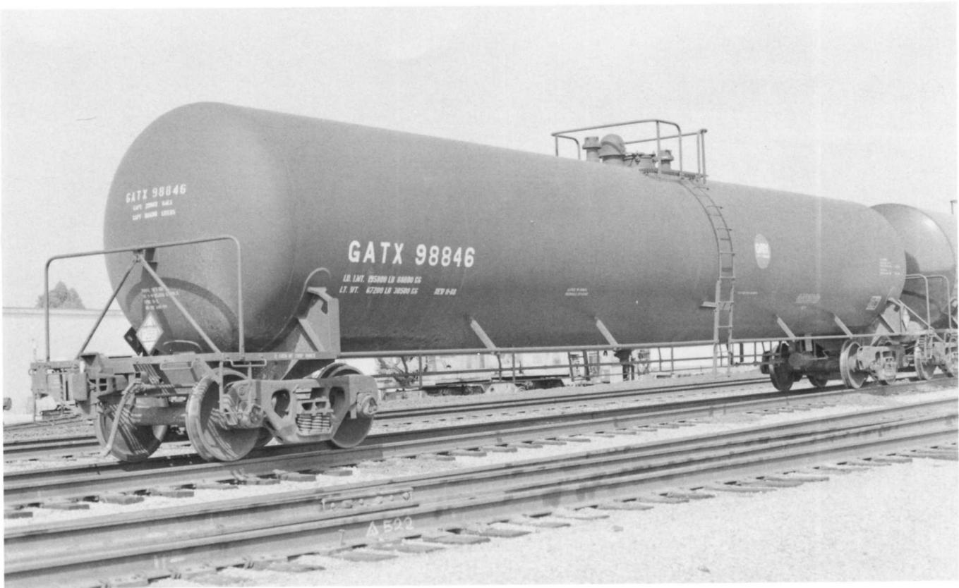
Above - GATX 98846. Built in November 1988 by Trinity Industries. Petroleum naphtha transport. Capacity 29,983 gallons. AAR car type code T108. Non-insulated. No coils. DOT 111A100W1. Leased to Unocal Chemicals Division. Length 67'11".
