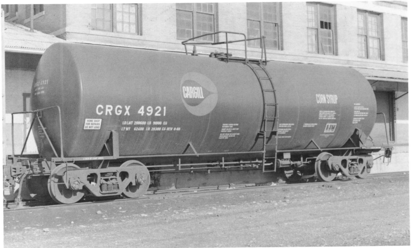
Below - CRGX 4921. Built in August 1988 by Trinity Industries, Longview, TX plant. Corn syrup transport. DOT 111A100W1. AAR car type code T104. Capacity 17,590 gallons. Insulated. Heater coil equipped. Photographed August 1992 in Salt Lake City, UT.
