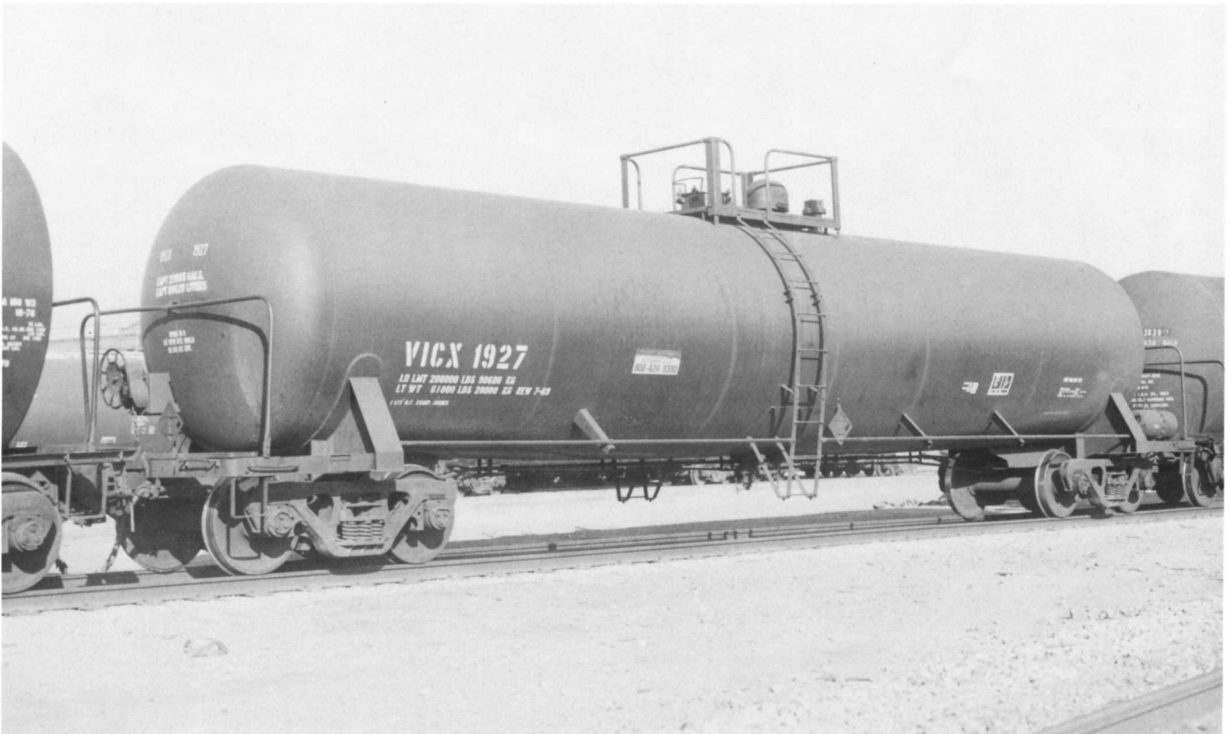
Below - VICX 1927. Built September 1969 by ACF Milton. Capacity 23,585 gallons. AAR car type code T106. DOT 111A100W1. Non-insulated. VICX is a reporting mark for Vista Chemical Co. Length 55'11".
