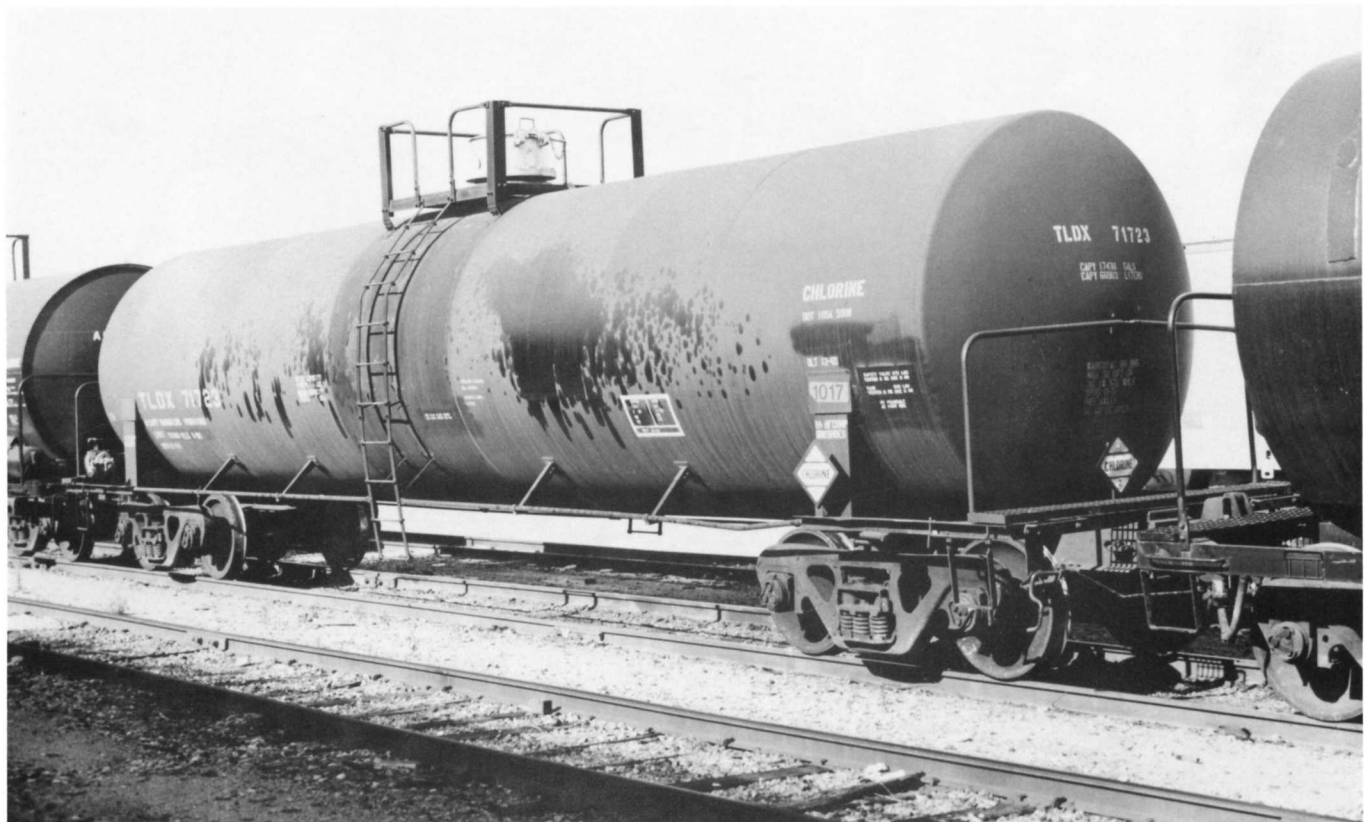
Above - TCDX 11058. Built in August 1977 by Union Tank Car Co. Sulphuric acid transport. Capacity 12,389 gallons. Here is another rare case of an insulated and coil equipped T054. HERSITE lined in January 1989. DOT 111A100W2. Photographed May 1993 in Atlanta GA. TCDX is presently a Union Tank Car reporting mark. Below - TLDX 71723. Built in December 1969 by Richmond Tank Car Houston, TX. Chlorine transport. Capacity 90-tons. AAR car type code T564. DOT 105A500W. TLDX is now a GERSCO reporting mark (originally Transport Leasing). Length 50'6".
