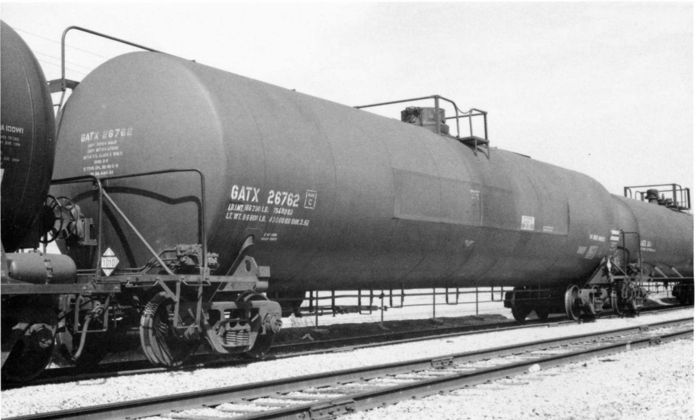
Below - GATX 26762. Built in March 1982 by GATX Sharon. Butadiene transport. Plate C (note flattened sides designed to keep car within Plate C limits). Capacity 33,605 gallons. AAR car type code T909. Length 65'11".
