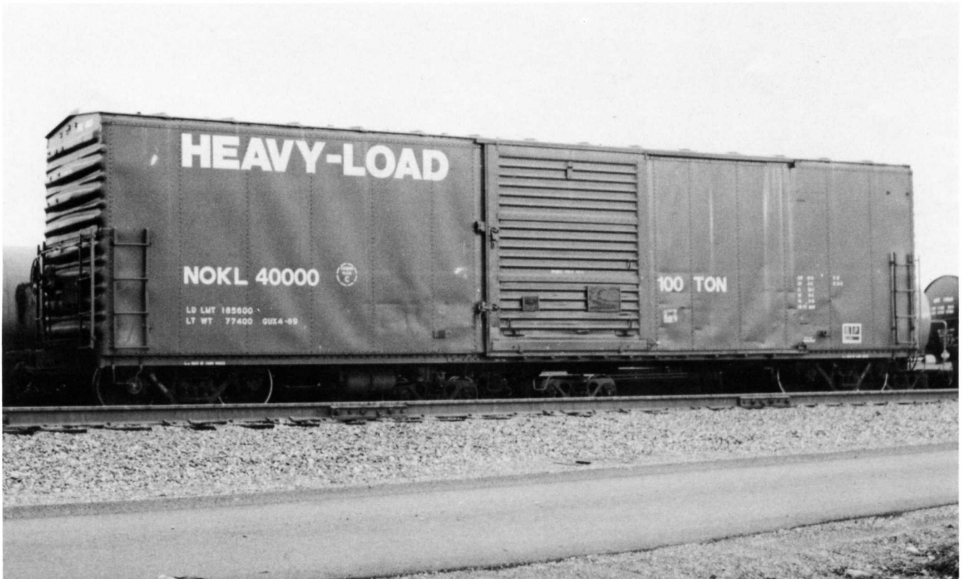
Below - NOKL 40000 was rebuilt in April 1989 to this "Heavy-Load" car. An extra heavy-duty floor is used in this car for metal service. 4644 cf capacity. Brown car with white lettering. Monoseries car. Ken M. Ardinger photo.
