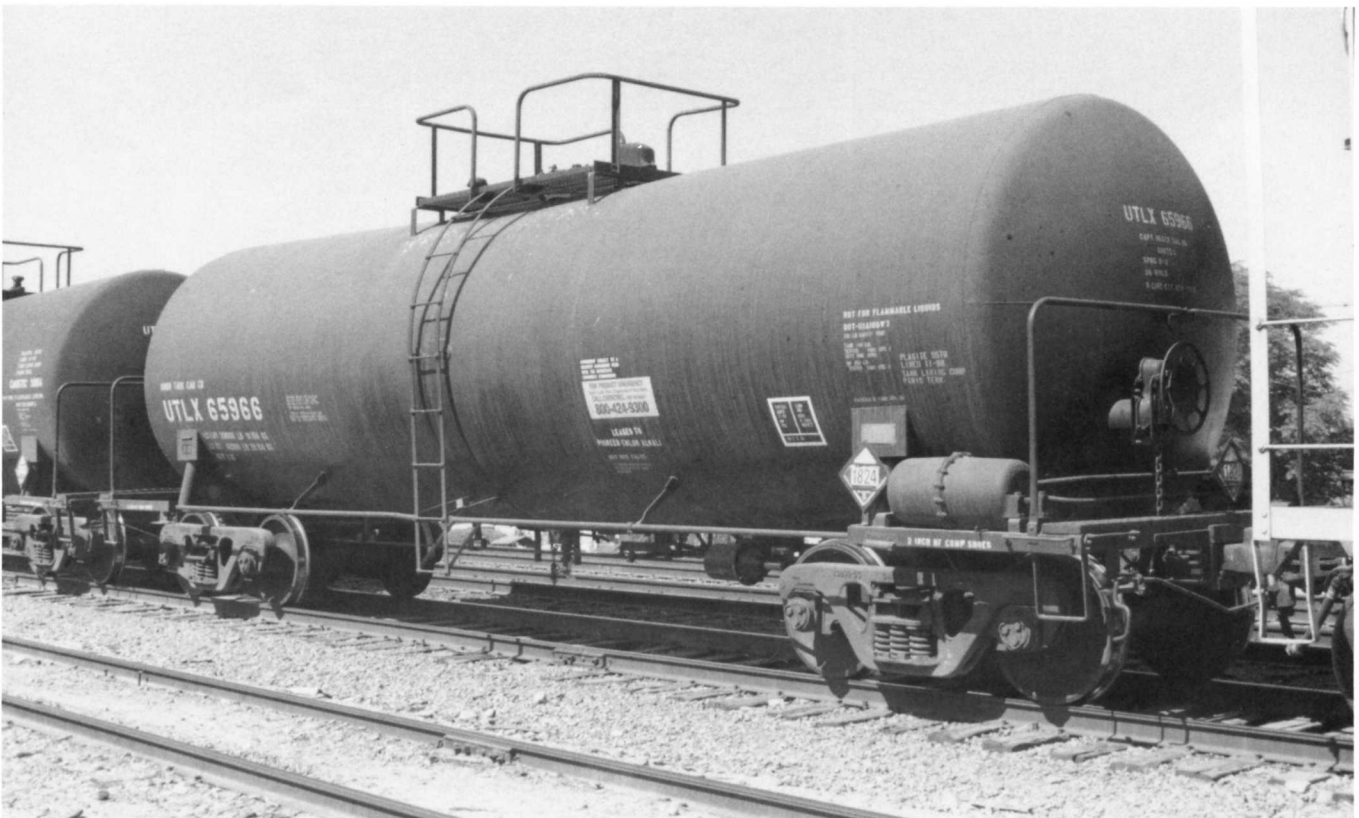
Below - UTLX 65966. Built in January 1981 by Union Tank Car Co. Caustic Soda transport. Capacity 16,372 gallons. Leased to Pioneer Chloroalkali. AAR car type code T104. DOT 111A100W3. Length 44'3".
