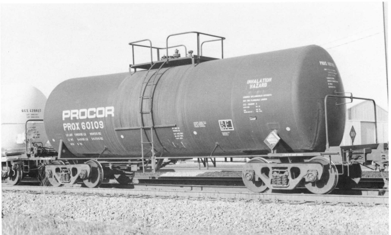
Below - PROX 60109. Built in June 1991 by Union Tank Car Co. Nitrating acid transport. Capacity 13,132 gallons. DOT 111A100W2. AAR car type code T054. Insulated. Heater coil equipped. (Most T054's are for sulphuric acid transport, non-insulated and not equipped with coils). PROX is Procor Limited. Photographed May 1993 in Atlanta GA.
