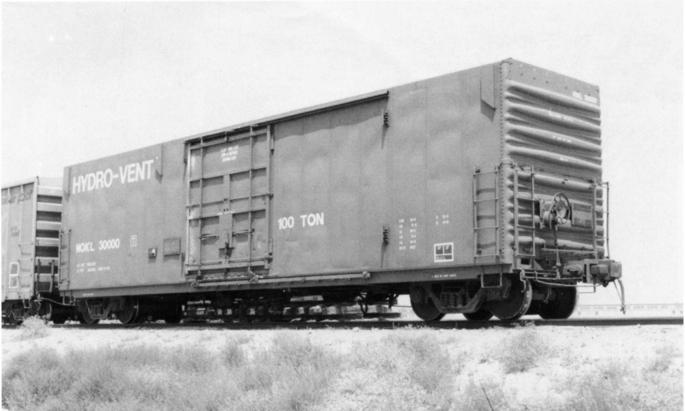
Above - NOKL 30000 was rebuilt in March 1989 by Gunderson Portland OR to this "Hydro-Vent" car. Brown car with white lettering. There are six large vents (3 on each side). 5027 cf capacity. This is a one car series. Photographed April 1993 at Mira Loma, CA. David G. Casdorph photo.
