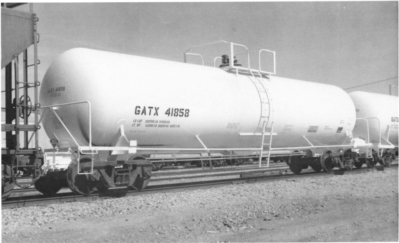
Above - GATX 41858. Built in June 1972 by GATX Sharon. Rebuilt in January 1991 to DOT 111A100W5 for hydrochloric acid transport. Capacity 21,947 gallons. AAR car type code T056. Leased to Pioneer Chloroalkali. Most hydrochloric acid tank cars are T055's. The gallon capacity on this car went just over the limit into the T056 category. Length 54'0". Below - GATX 57730. Built in September 1986 by Trinity Industries Longview TX plant. Phosphoric acid transport. Capacity 14,371. AAR car type code T104. DOT 111A100W1. Lined with Uniroyal 5980 in October 1986 by Smith Industries. Length 45'5".
