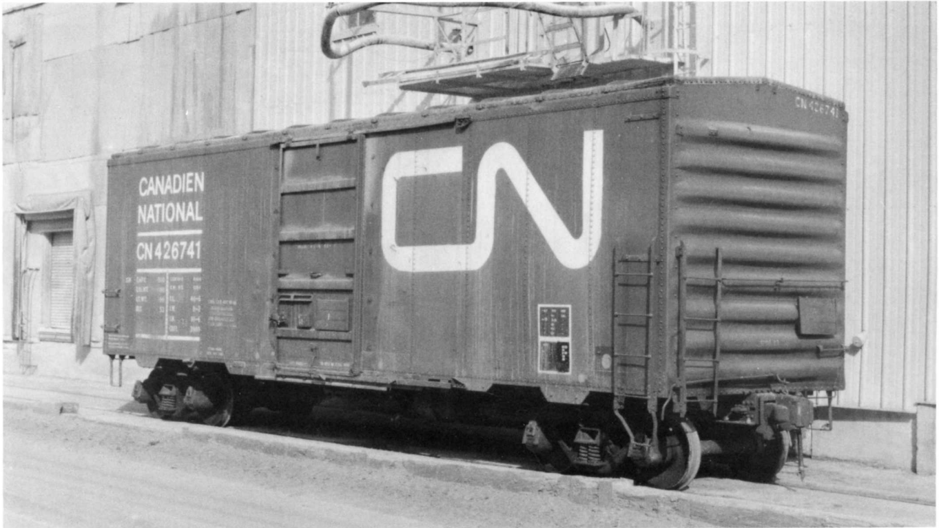
Above - The above photowas incorrectly printed in Freight Cars Journal 55 on page 10. The above is a corrected printing. CN 426741. Built August 1953. Series CN 426000-427606. Saskatoon, SK. April 21, 1991. Mark Kindrachuk photo.
