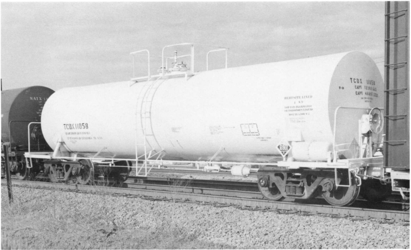
Above - TCDX 11058. Built in August 1977 by Union Tank Car Co. Sulphuric acid transport. Capacity 12,389 gallons. Here is another rare case of an insulated and coil equipped T054. HERSITE lined in January 1989. DOT 111A100W2. Photographed May 1993 in Atlanta GA. TCDX is presently a Union Tank Car reporting mark. Below - TLDX 71723. Built in December 1969 by Richmond Tank Car Houston, TX. Chlorine transport. Capacity 90-tons. AAR car type code T564. DOT 105A500W. TLDX is now a GERSCO reporting mark (originally Transport Leasing). Length 50'6".
