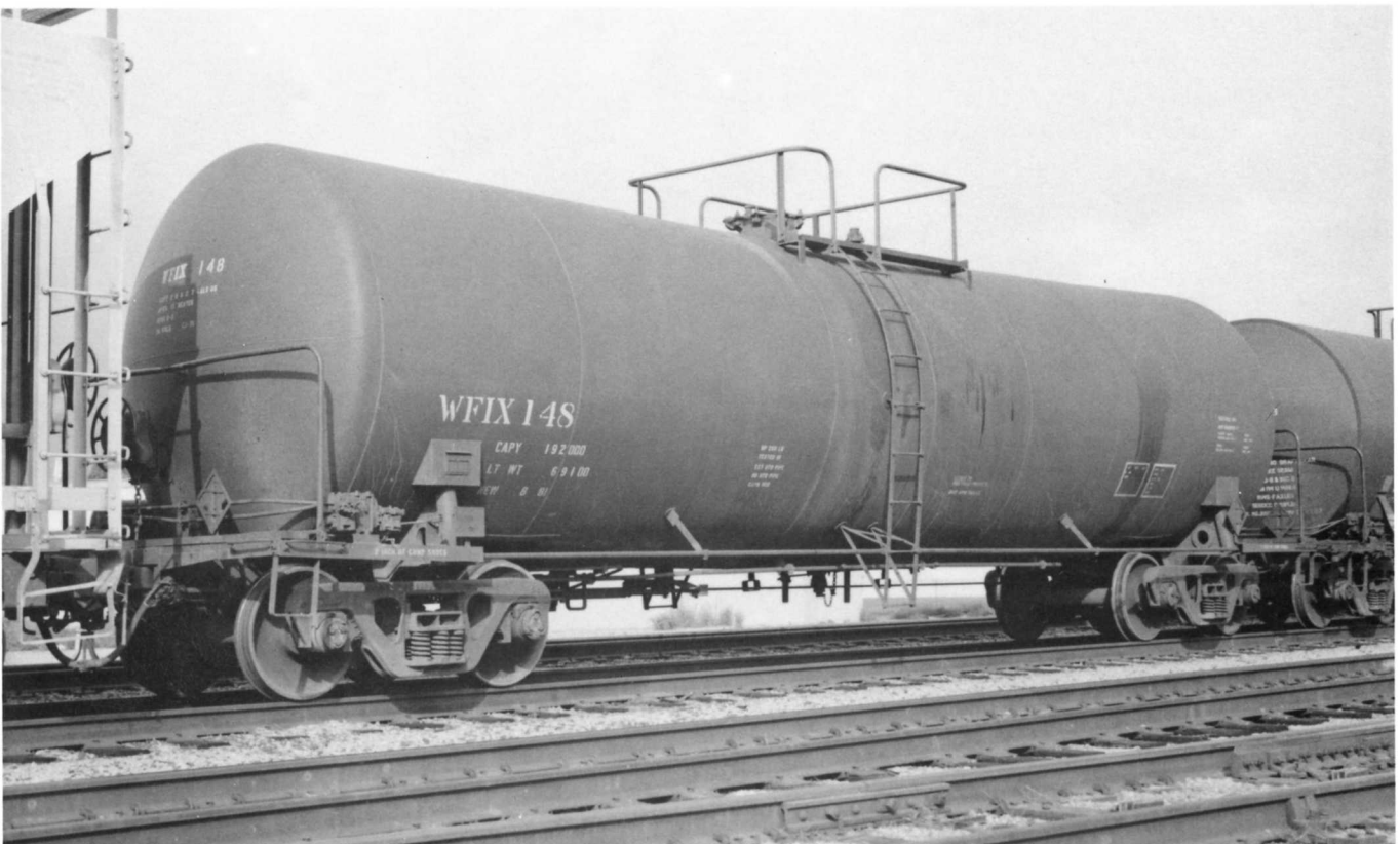
Below - WFIX 148. Built in August 1981 by Union Tank Car Co. Capacity 20,667 gallons. AAR car type code T106. DOT 111A100W3. Insulated. Equipped with heater coils. WFIX is now part of the GERSCO fleet. Photographed March 1992 in Industry CA.
