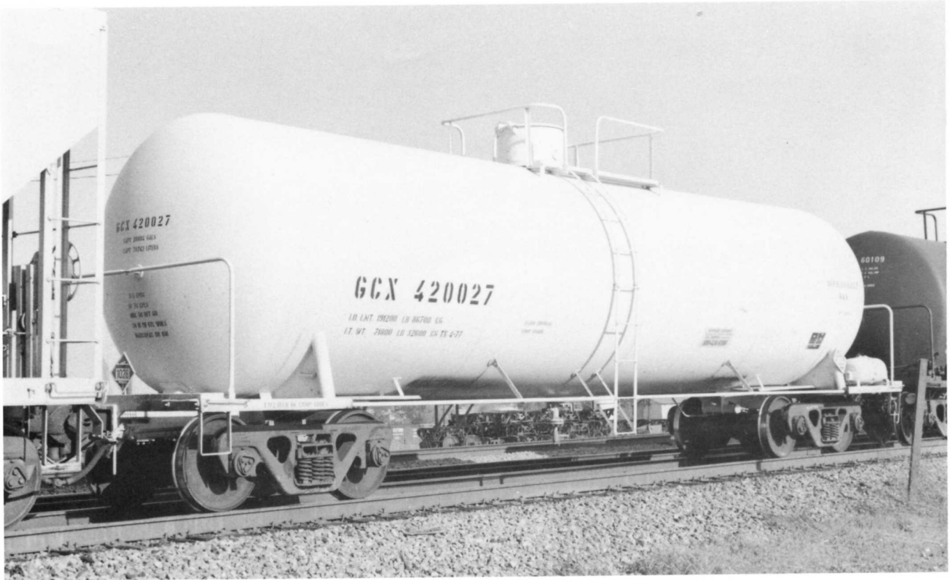
Above - GCX 420027. Built in June 1971 by Union Tank Car Co. Dichlorodifluoromethane transport. Capacity 20,804 gallons. AAR car type code T655. DOT 114A400W. Part of series GCX 420016-420029. Photographed May 1993 in Atlanta GA. GCX is the reporting mark for Alltank Equipment Corporation.
