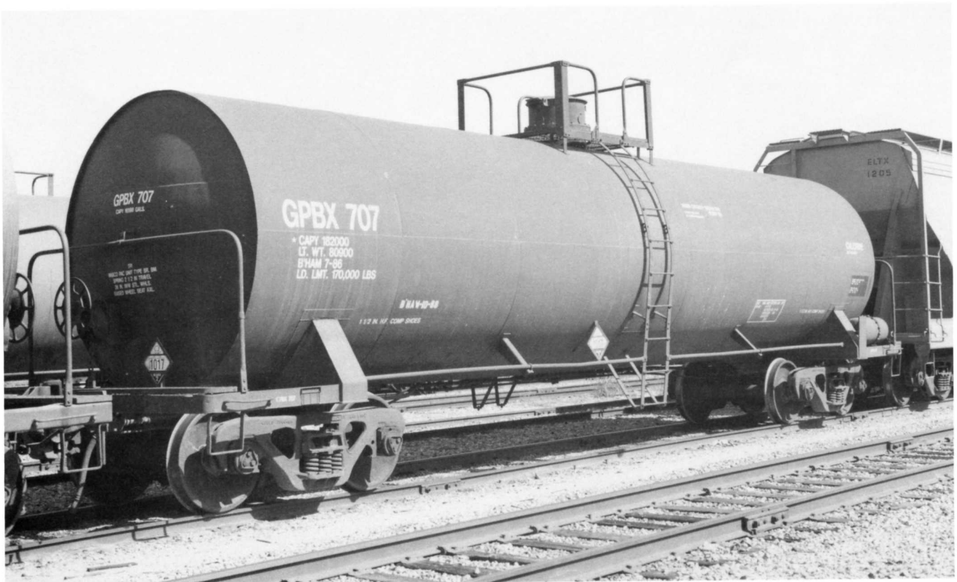
Below - GPBX 707. Built in October 1967 by ACF Milton. Chlorine transport. Capacity 85-tons. AAR car type code T564. GPBX is the reporting mark for Georgia-Pacific Corporation Bellingham Division. Length 45'3".
