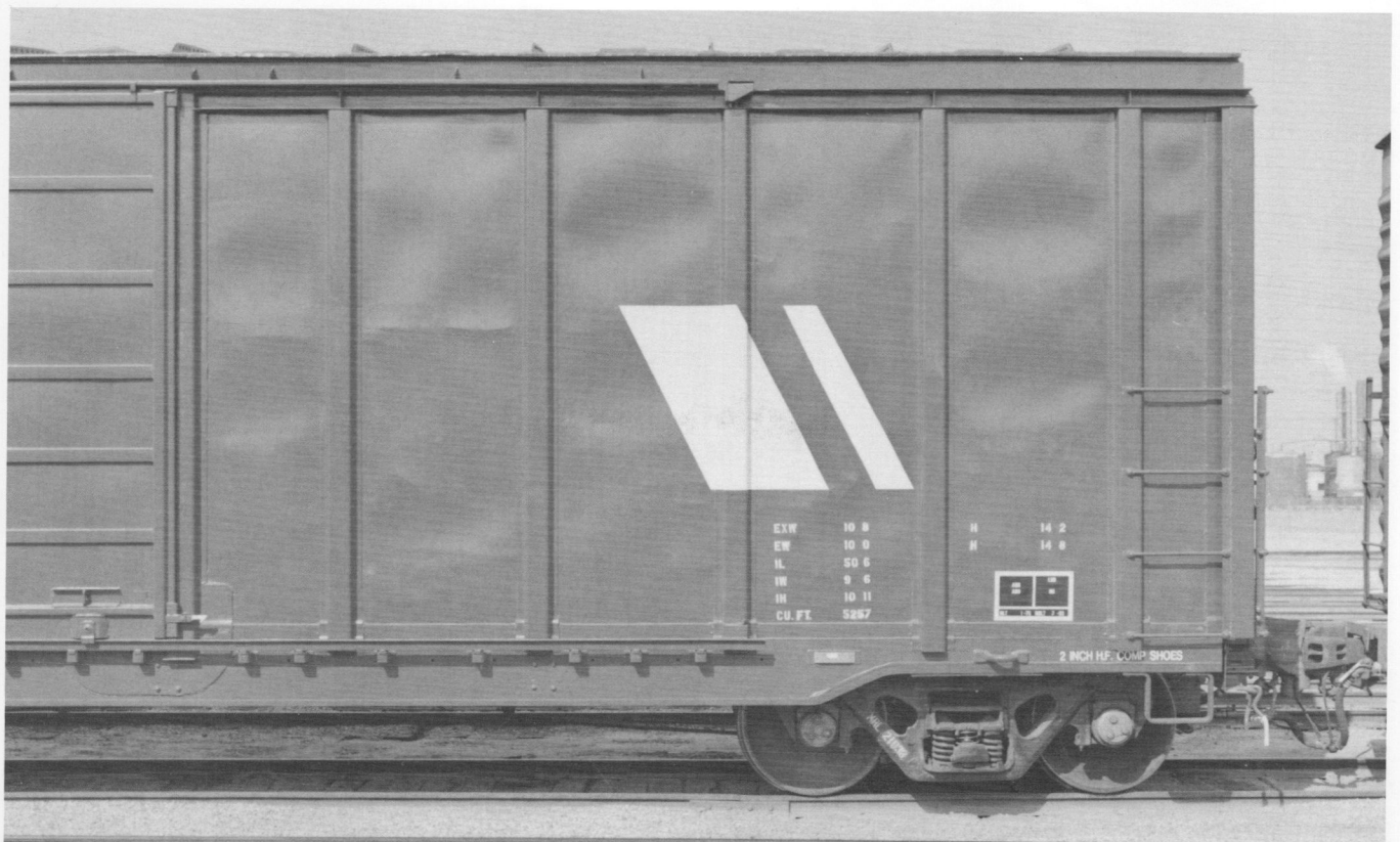
(Above) A 3/4 view of the end shows how the roof was raised just above the posts. The inside height was raised four inches. (Below) Side view to right of door showing markings and continued channel above posts. Note also that the door opening height was also increased by four inches.
