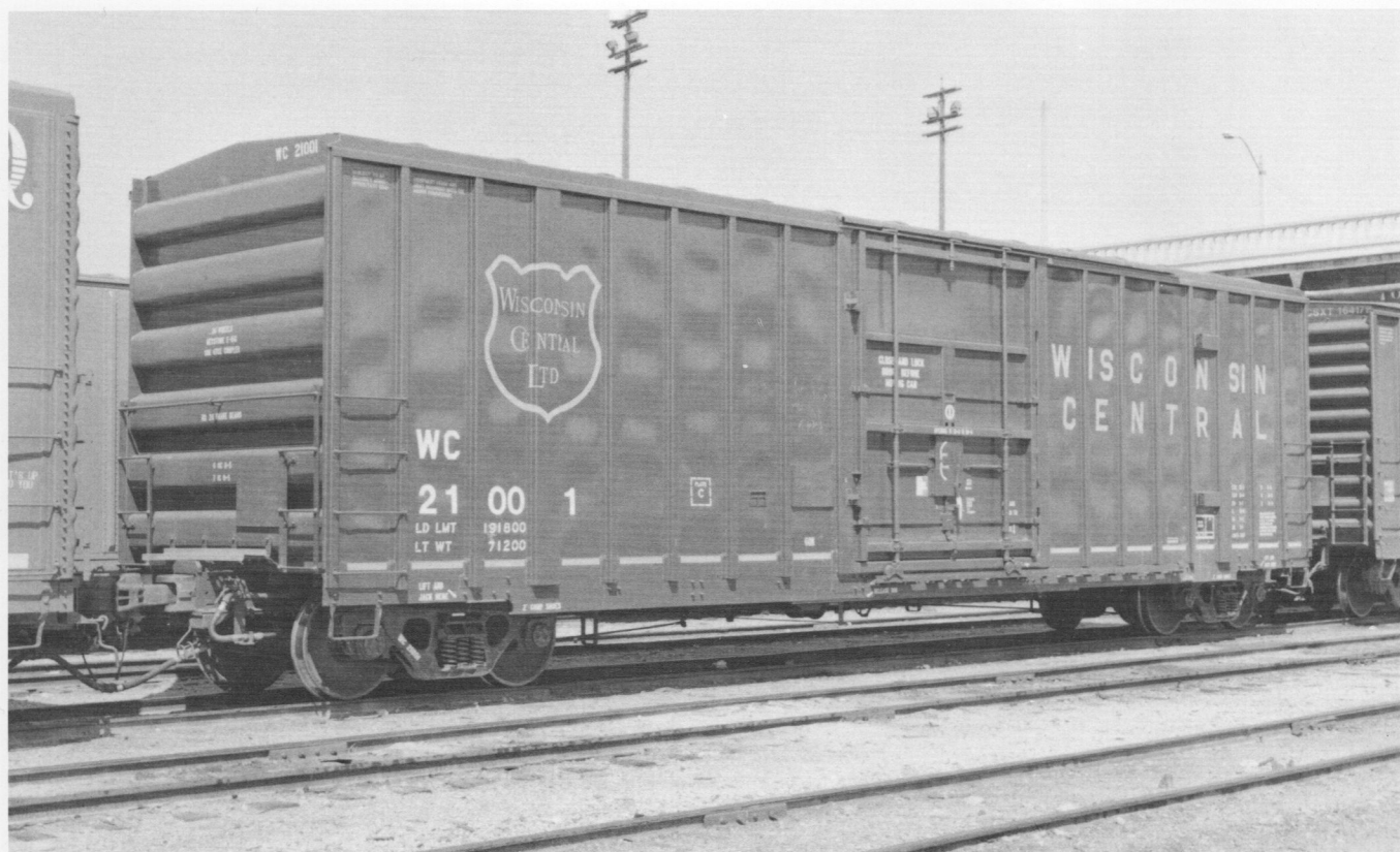
(Above) MRL 11014 was built in 2-93 by Gunderson's Portland OR plant. Photographed in April 1993 Kaiser, CA (SP). Hal Brown/D.G. Casdorph photo. (Below) WC 21001 was built in January 1993 by Gunderson. Note the extra-wide ribs (e.g. the one going through the middle of the WC herald). D.G. Casdorph photo.
