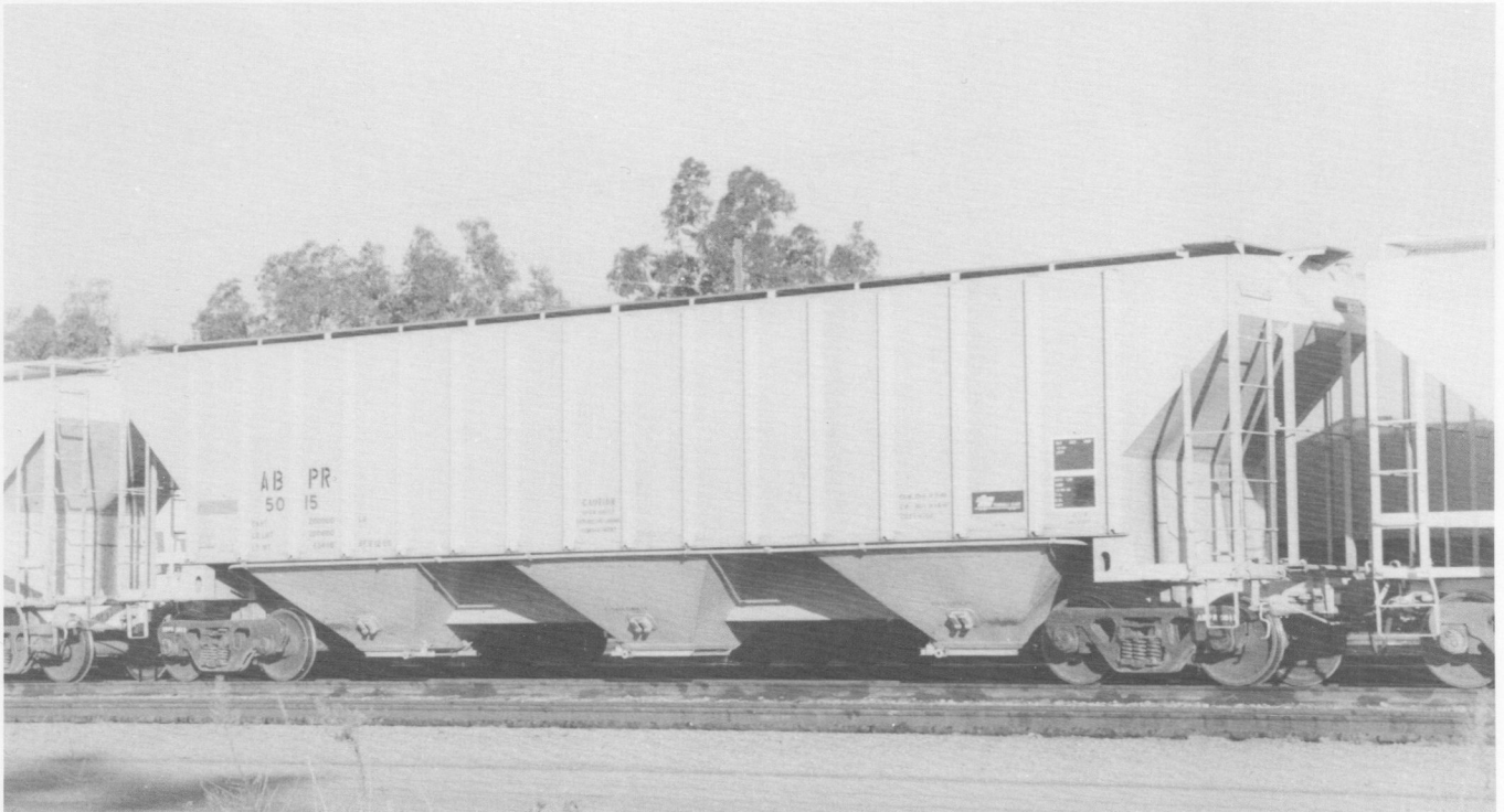
(Above) ABPR 5015 was built in December 1980 by Thrall Car. Note 16 ribs on this 4750 cf design. (Below) ACL 117162 was still in active coal transport service when photographed at Huntington WV in September 1985. Capacity, 2470 cf.
