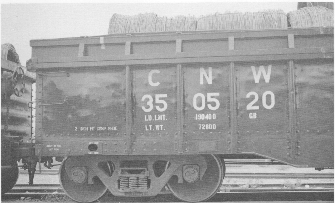
(Above) CNW 350520 was originally built by Greenville as part of the P&LE 50000-50799 series. The cars were rebuilt in 1991 with extended sides and ends. (Below). Series is CNW 350500-350719 (220 cars). GERSCO owner-lessor. Capacity, 2443 cf.
