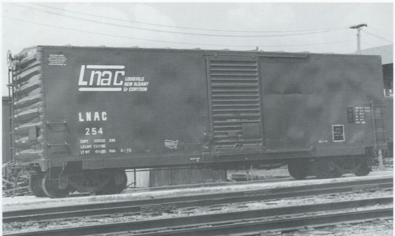
(Above) LNAC 100. 110XM. Refurbished USEX WA 12-71 (Lot 1104). Built 3-52. (Below) LNAC 254. 110XM. Refurbished USEX WA 6-72 (Lot 1115). There were 150 cars refurbished between March and June 1972.
