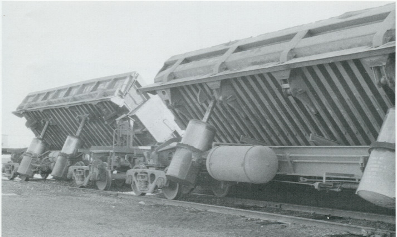
(Above) ATSF 185140 (left) and ATSF 186238 (right) showing bodies in the dump position underneath. Note the difference between the Magor (left) and Difco (right) designs. (Below) ATSF 186140 from the load side. James A. Kinkaid both photos.
