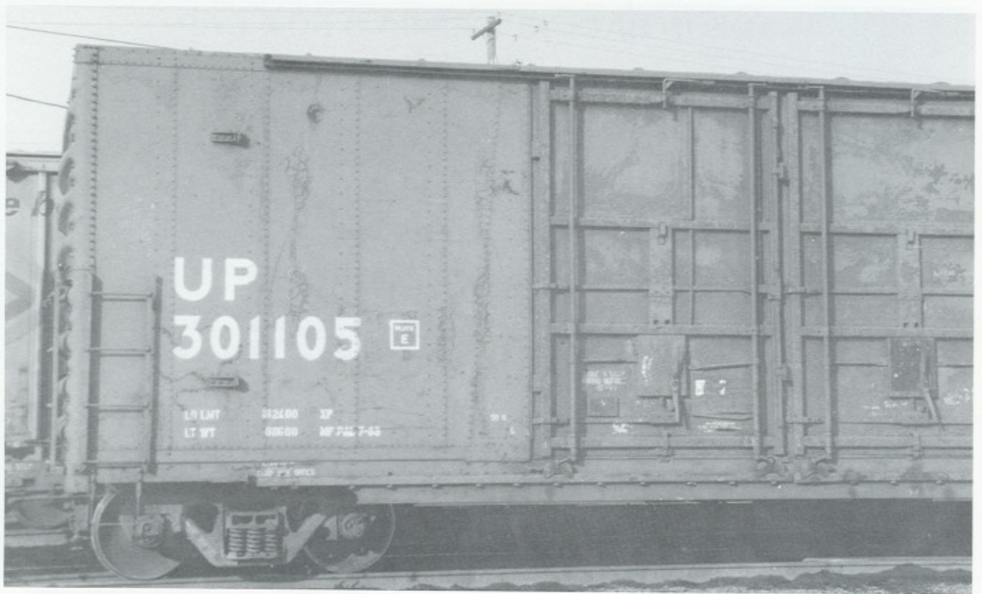
(Above) A view of the left side of the car, showing the simple, white lettering that has been stenciled on the brown paint. Note the Plate E clearance notice to the right of the car number. Only the light weight and load limit of the car are given. (Below) A view of the right side of the car, showing the Union Pacific shield, with the car class and dimensions below it. Judging from the peeling paint, the "We Can Handle It" slogan and a larger UP shield were once on the side of the car.
