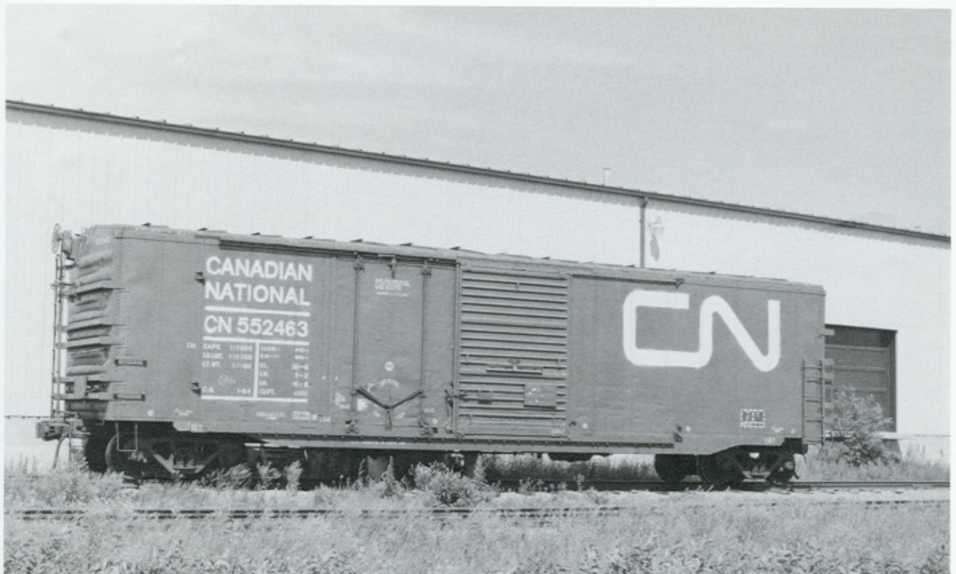
(Above) CN 551684. Built 11-57. 119XM. Series, CN 551000-551893. Saskatoon, SK. March 12, 1991. (Below) CN 552463. 115XM. Staggered 16'0" door opening. Series, CN 552000-552622. Mark Kindrachuk both photos.
