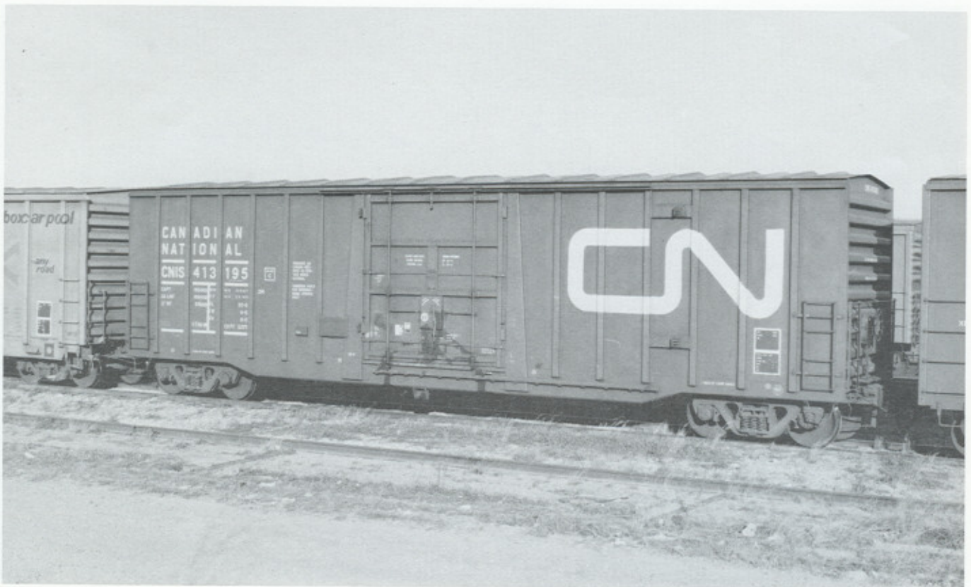
(Above) CN 411953. Built 1-74 NSC. 158XM. 4794 cf. 12'0" door opening. Series, CN 411900-411999. Jasper, AB. October 9, 1991. (Below) CNIS 413195. Built 2-80 NSC. 195XM. 5277 cf. 10'0" door opening. Series, CNIS 413000-413199. Hinton, AB. October 12, 1991. D.G. Casdorff Both photos.
