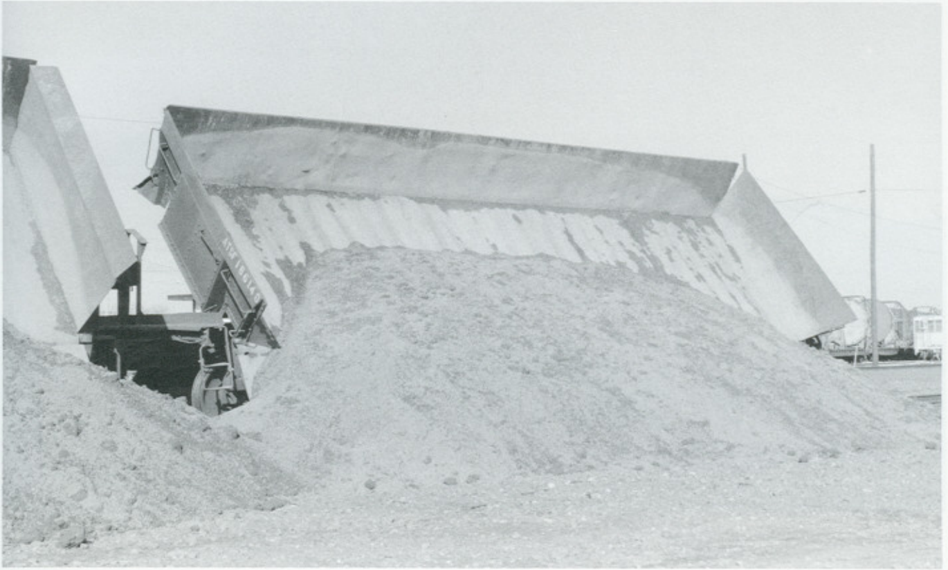
(Above) ATSF 185140 (left) and ATSF 186238 (right) showing bodies in the dump position underneath. Note the difference between the Magor (left) and Difco (right) designs. (Below) ATSF 186140 from the load side. James A. Kinkaid both photos.
