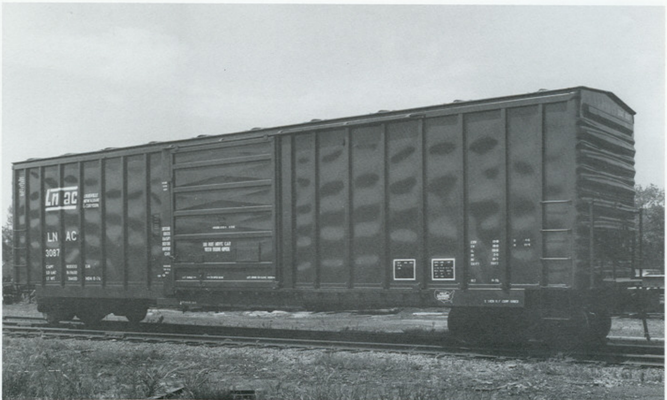
(Above) LNAC 3005. 110XP. Rebuilt 5-73 USEX WA (Lot 1183). This car was assigned to the DT&I at Toledo, OH. (Below) LNAC 3087. 162XM. Built new 8-76 USEX BI (Lot 1400 from 1389). 5077 cf. Plate B box car. Note end on this car compared to LNAC 3005 above.
