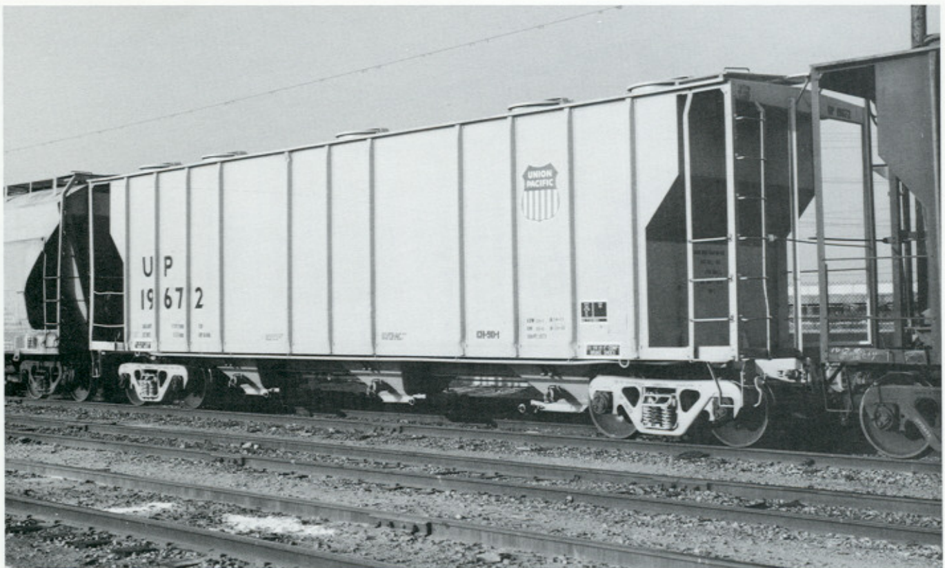
(Above) Type PS 3510. MP 707015 was built in 1962 by Pullman-Standard. It was refurbished in September 1988. (Below) Type PS 3572. UP 19672 was built in 1962 by Pullman-Standard. Note the gravity and pneumatic outlets. Painted in June 1988. Series UP 19300-19699.
