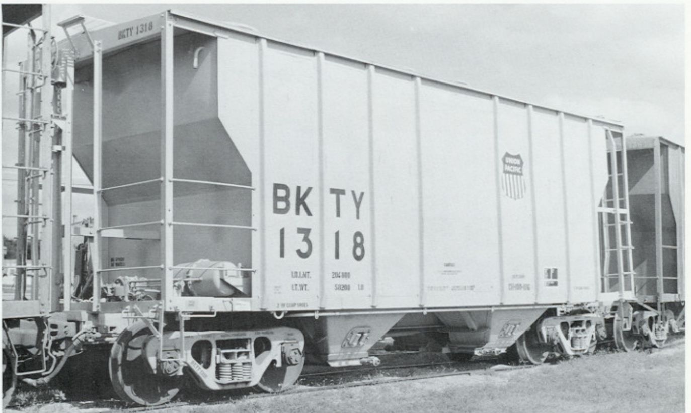
(Above) Type POX 3000. MKT 720026 was built in 6-82 MFC CLIL (Portec). Series MKT 720000-720029. Mike B. Foley photo. (Below) Type PS 2600. BKTY 1318 was built in 1966 by Pullman-Standard. Series BKTY 1300-1374. Photographed in Lincoln NE August 1992.
