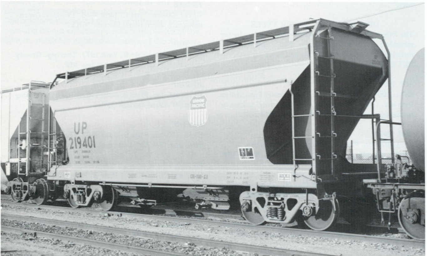
(Above) Type ACF 2970. UP 219319. Series UP 219300-219800. These are former Rock Island cars. This car was painted at the Pocatello shops in March 1985 in the light gray scheme. (Below) UP 219401 was painted in 1988 in the darker (slate) gray scheme.
