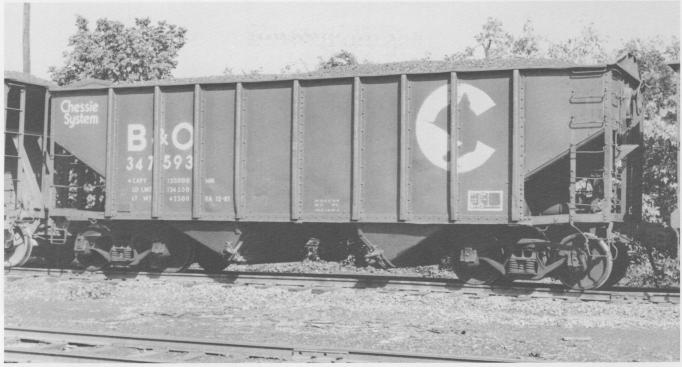
(Above) B&O 347593 photographed at Huntington WV in September 1985. Still in pretty good shape for forty years of service! Built 12-46. 2141 cf. It's ex C&O 347593, rebuilt from an offset-side car in 1963 (nee from C&O 47500-48989). (Below) IHB 7746 was ADN 7746 built by USEX. Photographed at Mira Loma, CA in April 1991.
