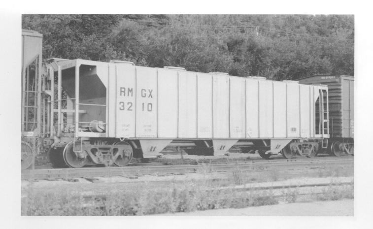
(Above) RMGX 3210 (Railcar, Ltd) was rebuilt in 11-90 by KKX GCS. Originally built in 1-65. Capacity, 2929 cubic feet. Photographed in Kansas City, MO in August 1992. (Below) SLC 1104 is from the GWR 11002-11559 series, nee FGEX 1000-1600 (mechanical reefers). Note the "Keep me loaded" slogan to the left of the door. Photographed in October 1988.
