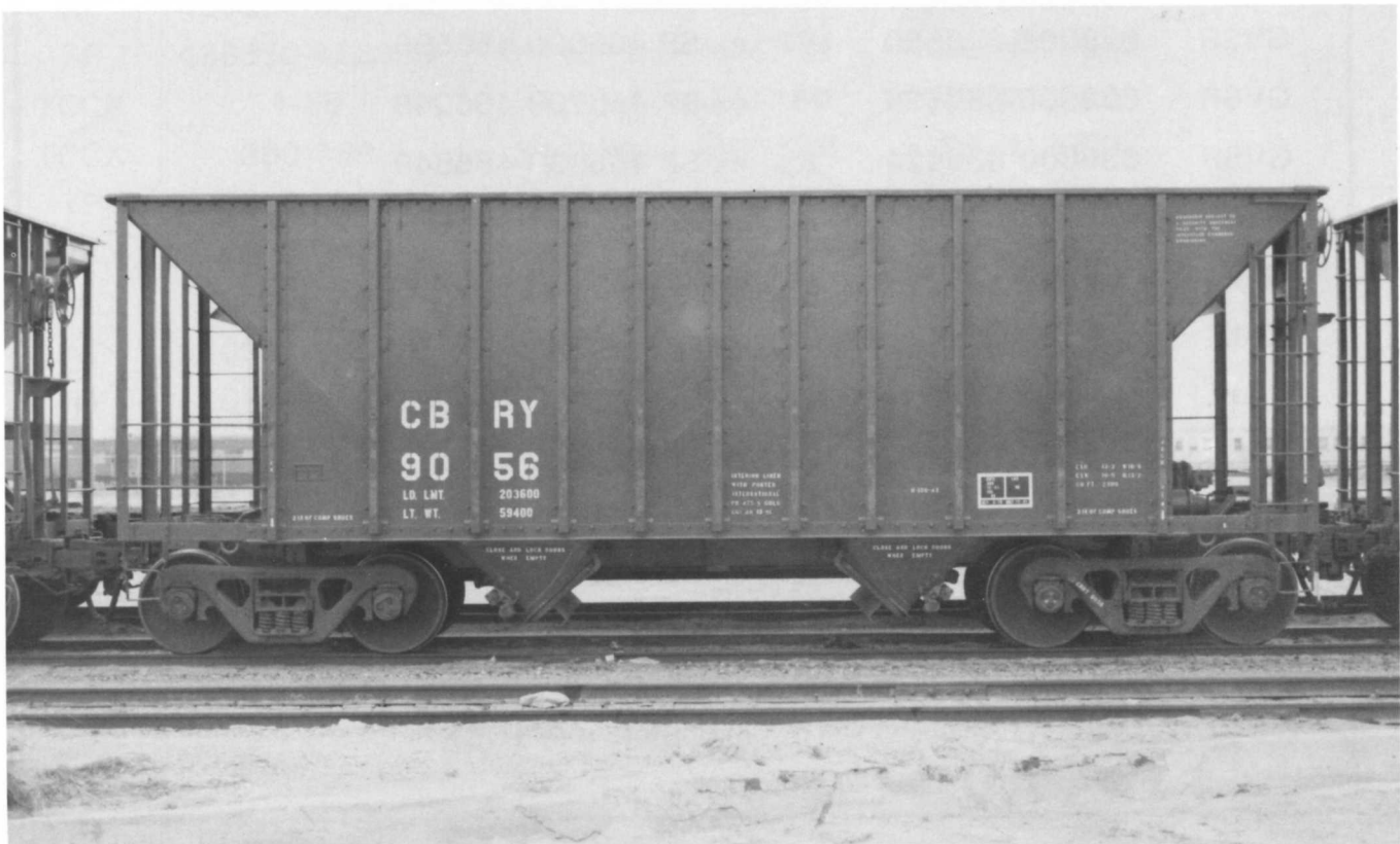
(Above) ATW 9123 was rebuilt 3-92 in Atchison, KS with a "kit" supplied by Johnstown America. Class H-100-43. (Below) CBRY 9056 was rebuilt in 12-91 with a kit like the ATW car above. This car is also class H-100-43. Both photos, David G. Casdorff.
