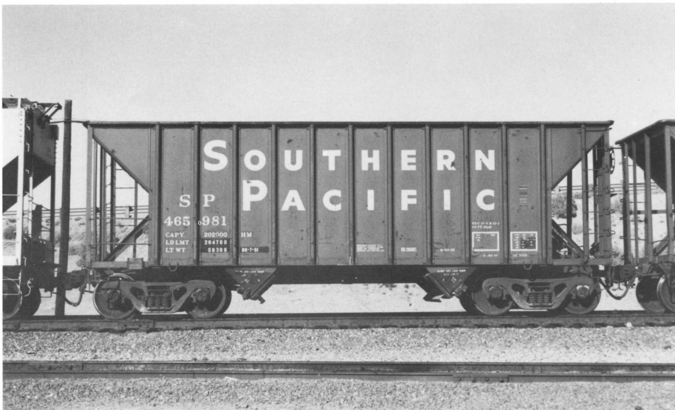
(Above) SOU 100307 was built in 1976 by GSC GV. Class HS31. This car was painted in 5-87. Note the rivets on lower part of the end ribs. (Below) SP 465981. One of the 350 cars built by Pacific Car & Foundry in 1976 for the Southern Pacific. Both photos, David G. Casdorph.
