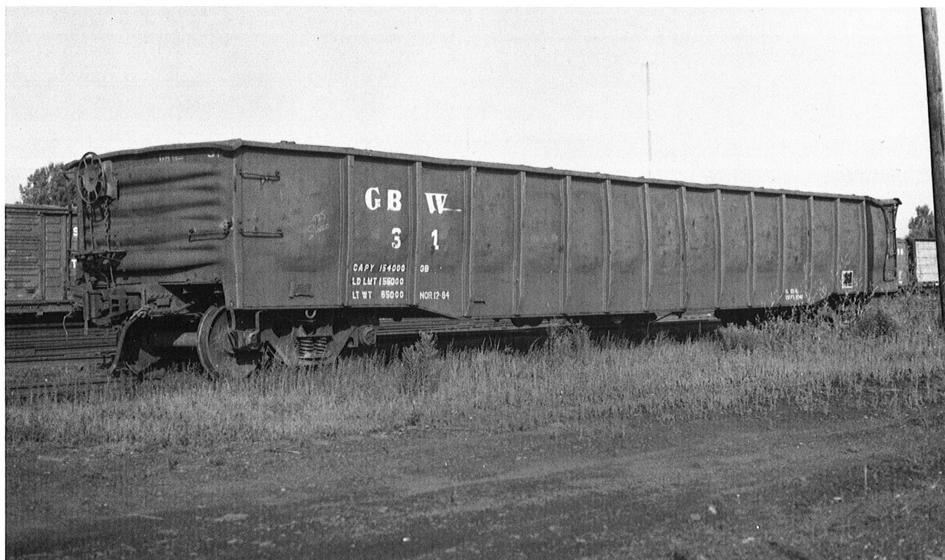
GBW 31 was built in April 1966. 70-ton mill gondola. 2340 cu.ft. capacity. Green Bay, WI August 1992.
