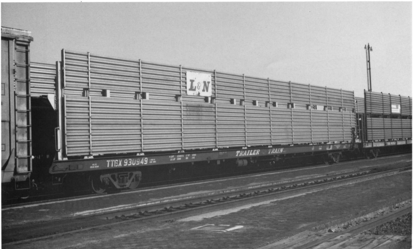
(Above) SSW 84861 appears to have a corrugation style with a slight bevel in the design. (Below) TTBX 930949 with L&N rack. The beveled corrugation design is a little more evident here. Note only two rows of panels (a row here is defined as not having a large visible gap between). Also, classic Trailer Train scheme on flat car.
