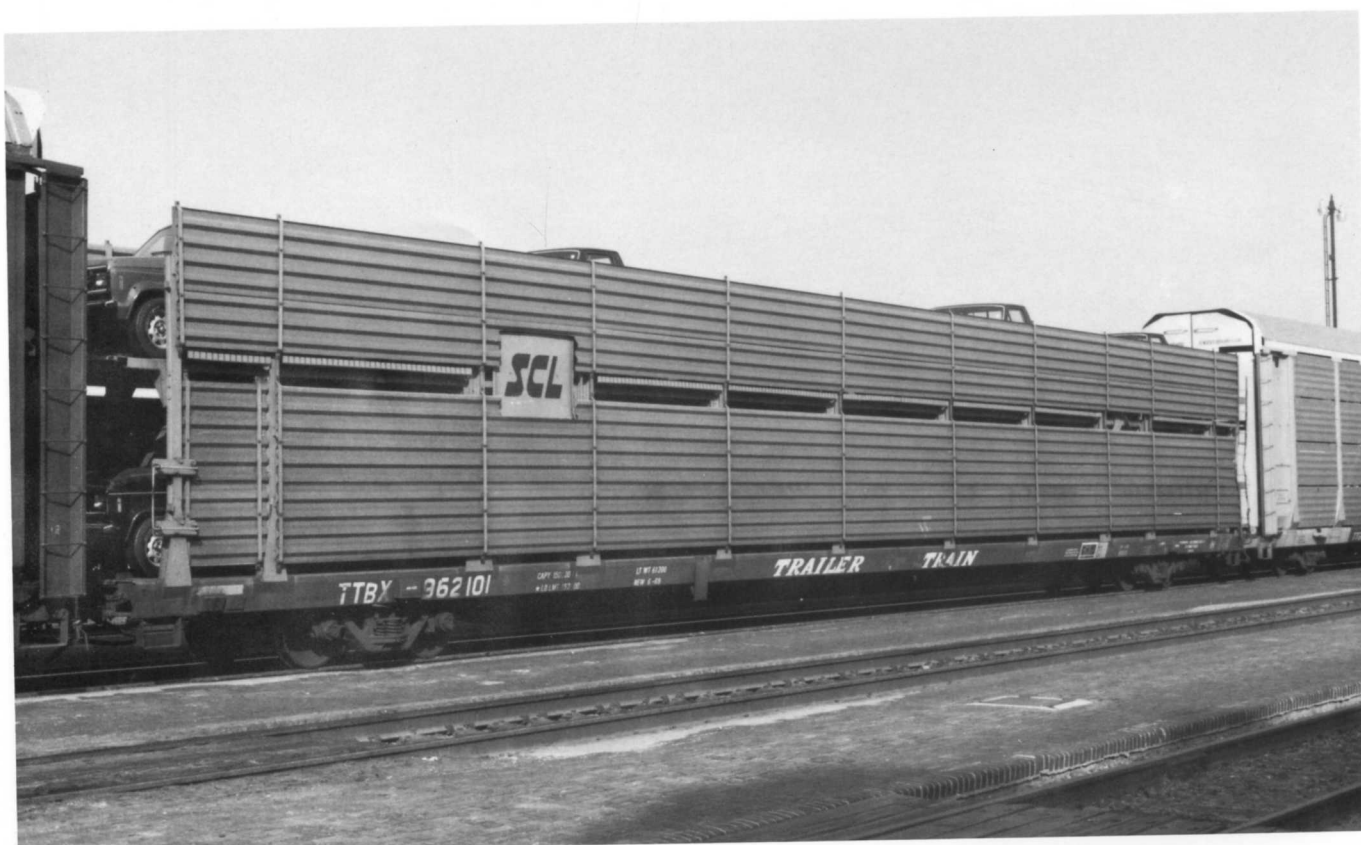
(Above and Below) TTBX 962101. Another example of the beveled corrugation pattern. Note how the logo panel is "split" across the upper deck (others shown have been above or below the deck).
