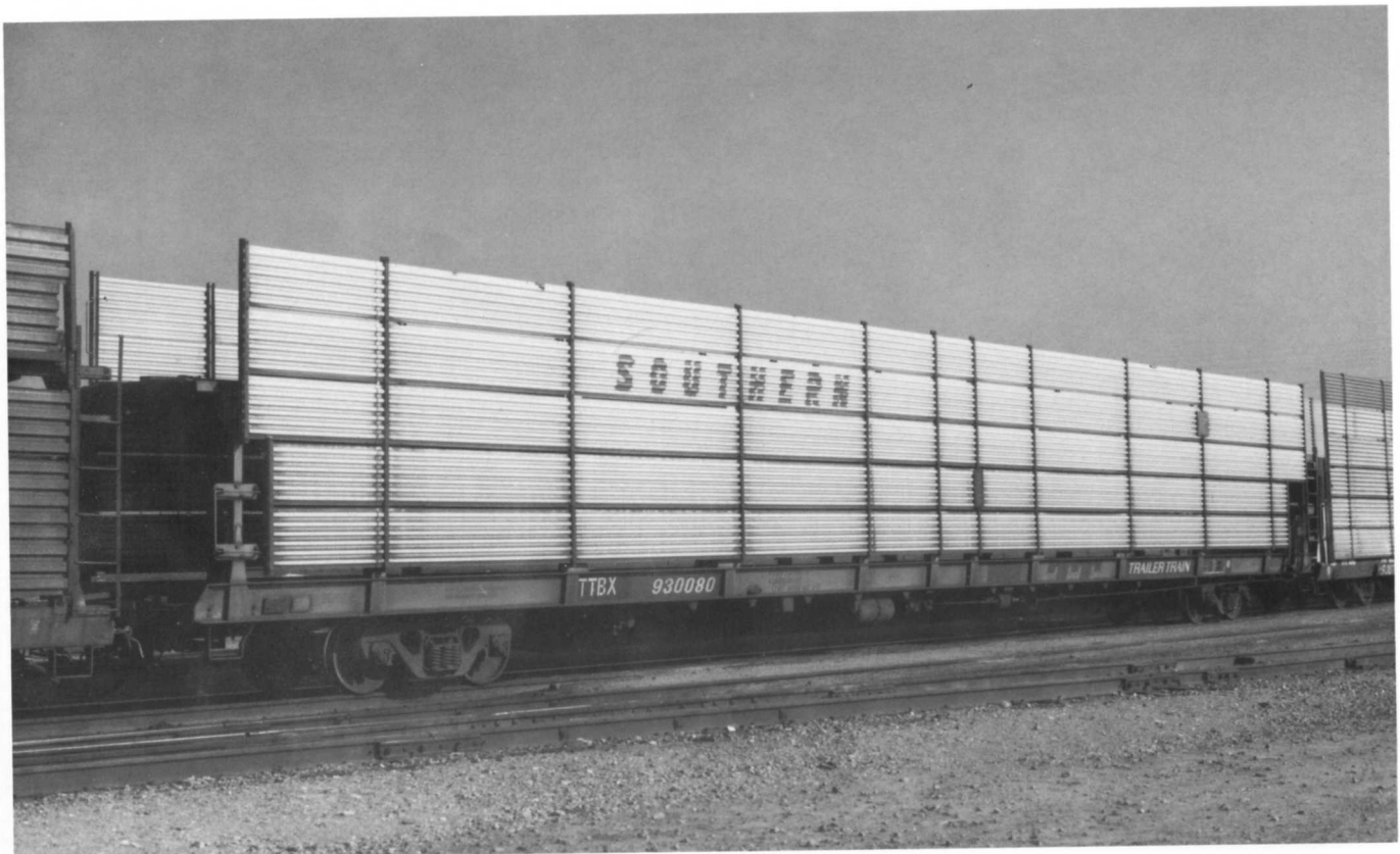
(Above) TTBX 962169. Again, a thin rounded corrugation type on these panels. Here there are five rows of panels. (Below) TTBX 930080. Similar to above rack but differences in placement of the panel supports and end of racks (note notches). Also visible is the stylised "F" of Ford Motor Co on the second support from the right.
