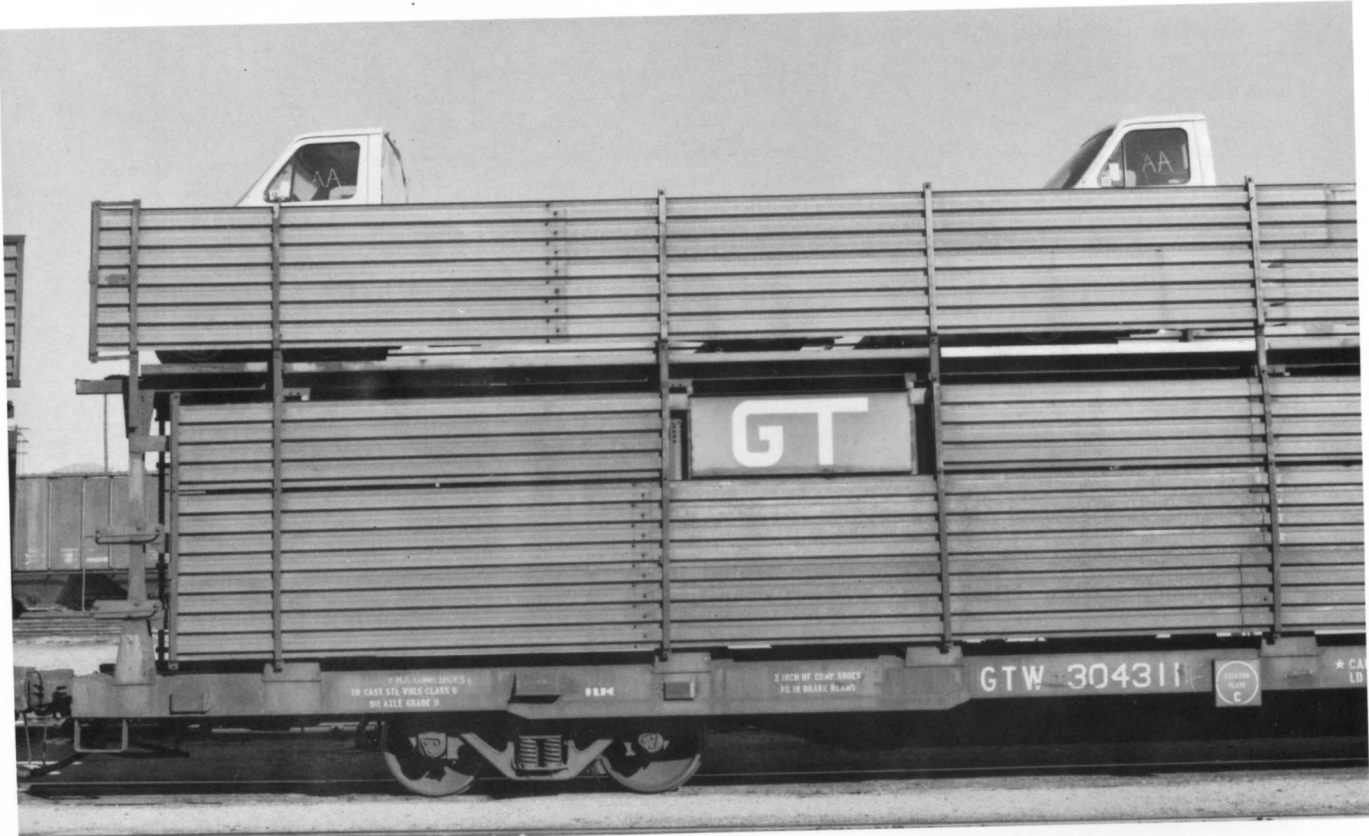
(Above) TTBX 910315 with Conrail rack. This rack has a wide squared type of corrugation on the panels. Note the brackets for the logo panel. This was one of the last open, paneled, racks built for a U.S. railroad. Built in 1980. (Below) GTW 304311 displays a slightly different style of square corrugated panel. Of note also is the W&K flat car. Note the logo (stylised "W") and unique side sill architecture.
