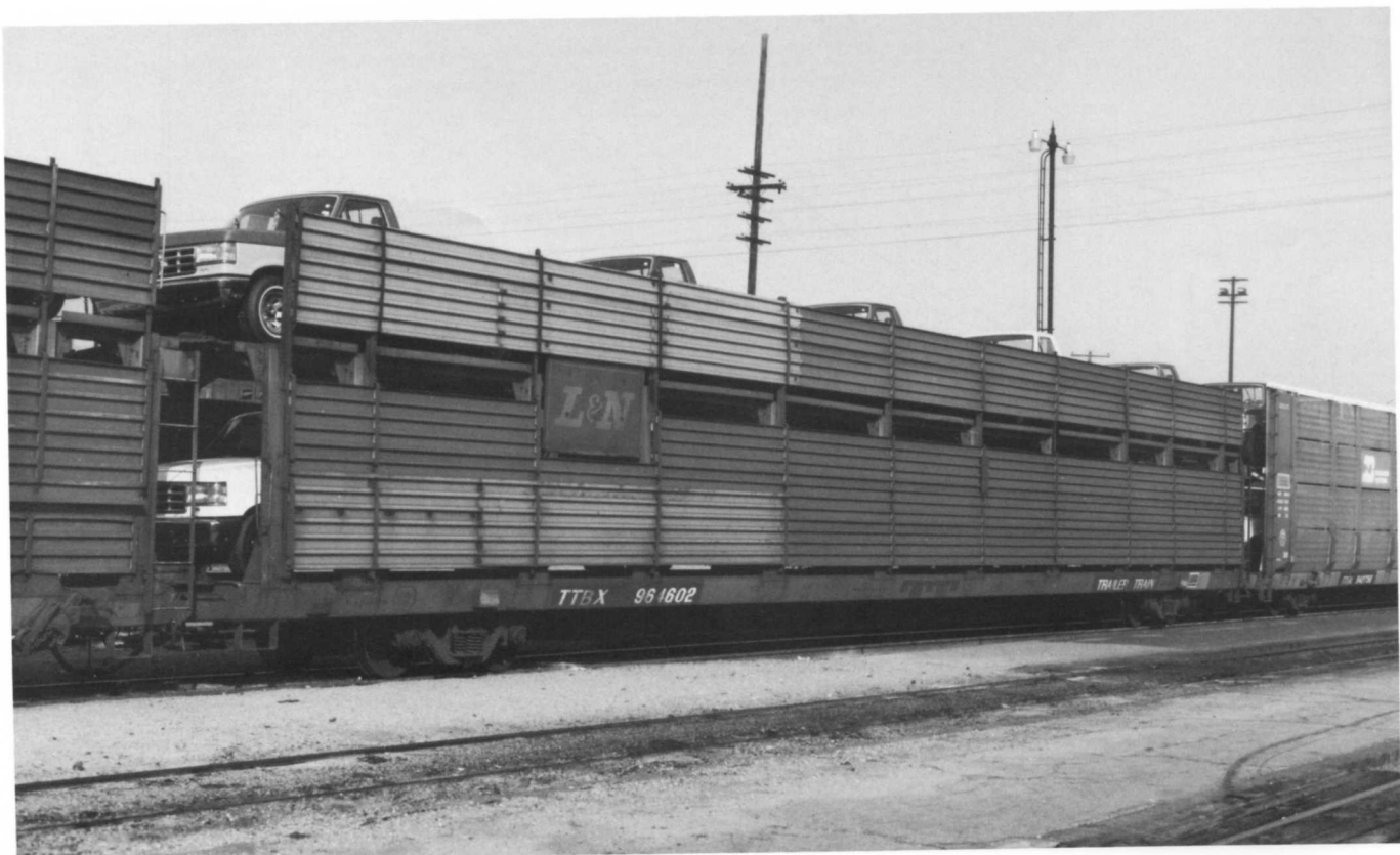
(Above) An overall view of TTBX 942015 / L&N rack with three rows of panels. Compare to TTBX 964602 (Below) having two rows of panels and different corrugation style. This type corrugation appears as a thin squared style with wider spacing. Also note location of logo-panel.
