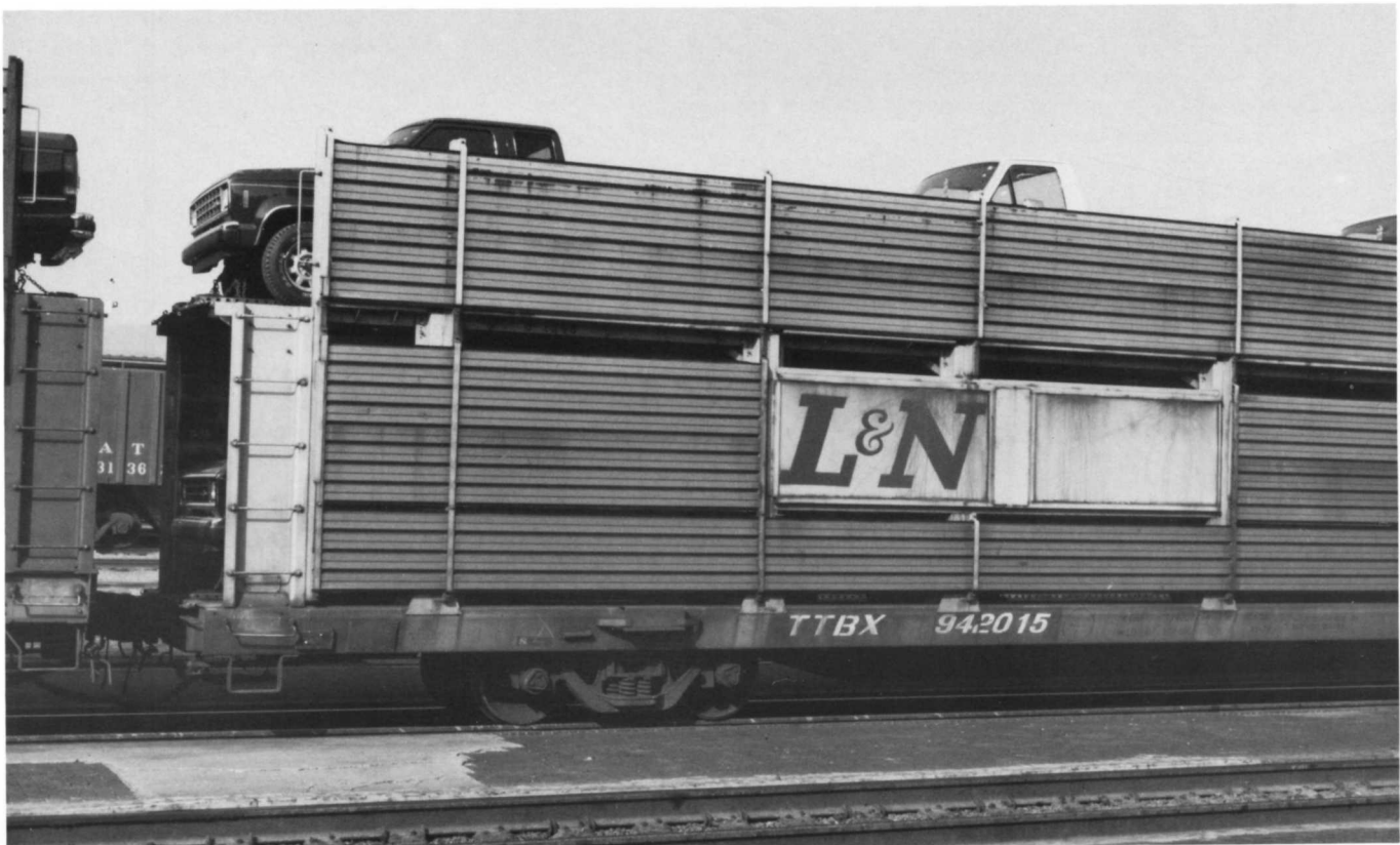
(Above) TTBX 964213 with DRGW rack. On the left is an interesting ladder arrangement. Also, of interest is the location of the "logo panel," below the upper deck (compare to the UP rack). (Below) TTBX 942015 with L&N rack. Note the size and style of logo panel on this rack. But, note how the spacing of the panel supports are about the same as above.
