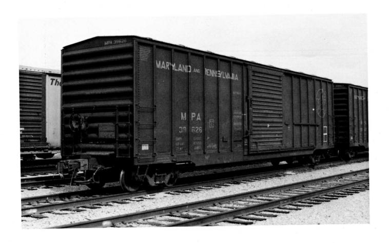
(Above) MPA 39626 built was in 1979 as part of Lot 41800. This series came equipped with 15" end-of-car cushioning. (Below) NW 604515 was built as part of Lot 37700 in 1979. These fascinating 60-foot 100-ton Plate F + box cars were used in auto parts service by many railroads. Both photos by David G. Casdorph.
