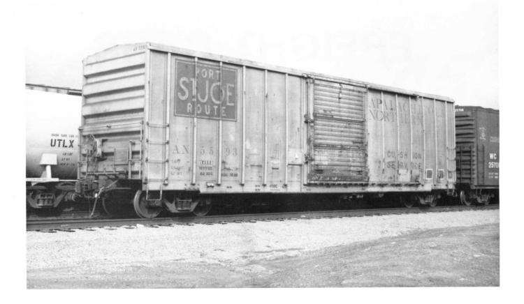
(Above) AN 5593. 154XM. Built in 1978 by FMC. 5347 cu ft capacity. Itel owner-lessor. (Below) ATSF 87913 was built in 1966 by Transco. Class Ga-146. Series, ATSF 87900-87949. Ptd 7-91.
