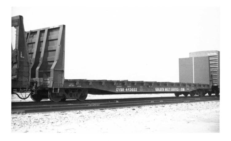
(Above) GVSR 443022. 57'0" IL 70-ton FBS. Note new horizontal corrugations on bulkheads. (Below) GVSR 528033. Built in 1972 by ACF HTG. 4650 cu ft capacity. ex-SSW. Class H-100-28.
