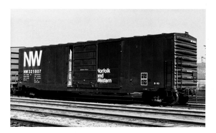
(Above) NW 321807. Class B-90. Built in 1959 by the Wabash. 4935 cu ft capacity. Ptd NW PR 11-79. (Below) NW 601239. Class B-120. Built in 1969 by Thrall Car. 6000 cu ft capy. Painted 7-84.
