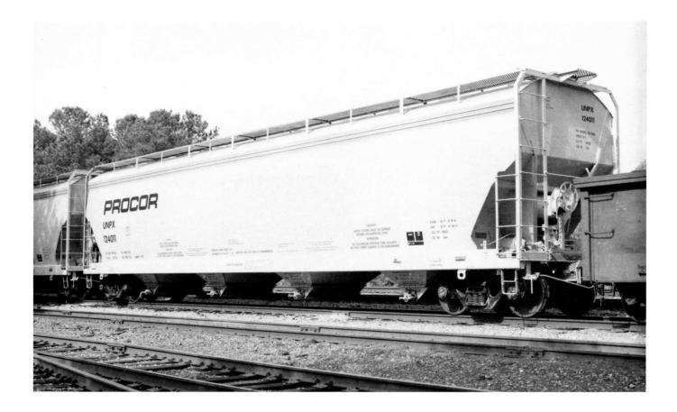
(Above) UNPX 124011. Built 1-92 TC CH. 5800 cu ft capacity. Cartersville, GA May 1992. (Below) UP 148120. Class G-100-17. Blt 1977 PCF RN. 6500 cu ft capacity. Wood chip transport.
