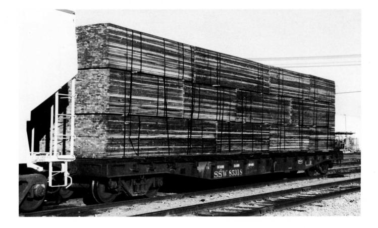
(Above) SSW 85318. Series, SSW 85200-85399. Built by Thrall. 53'6" IL general-service flat car. (Below) SOO 23160. Built 1-81 PS BUT. 4750 cu ft design. Itel owner-lessor. Former Pullman Leasing.
