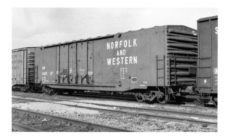
(Above) NW 51218. Class B-22. Built 7-65 ACF. Stencilled 4783 cu ft capacity. Ptd 12-84. (Below) NW 283132. Class B-51. Built in 1964 by ACF. 6190 cu ft capy. ex-NKP 83132.
