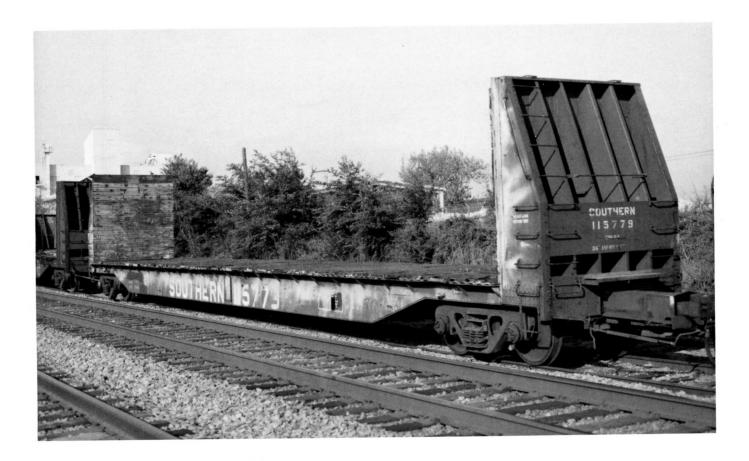
(Above) SOU 115779. Built 12-63 by Pullman-Standard. 67'0" IL. Photo at Bessemer, AL May 1992. (Below) SOU 141952. Built 6-80 GSC GV. 159LP. 50'0" IL. Pulpwood transport.
