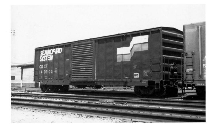
(Above) CSXT 140903. Built 1-80 JJF. 5277 cu ft capacity. 50'6" IL Plate C general-service box car. (Below) CSXT 141970. Blt 1975 PCF RN. RBOX class XCF10. ex-SBD, exx-C&O, nee-RBOX.
