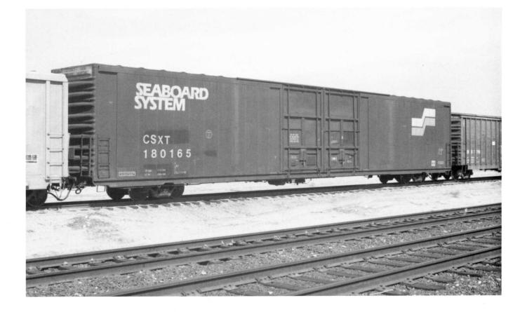
(Above) CSXT 180165. 86'6" IL Plate F+ box car. 10000 cu ft capy. Ptd 3-84. Restencilled CSXT 11-89. (Below) DOWX 2758. Built in 1982 by ACF HTG. 2980 cu ft capacity. Silica sand transport.
