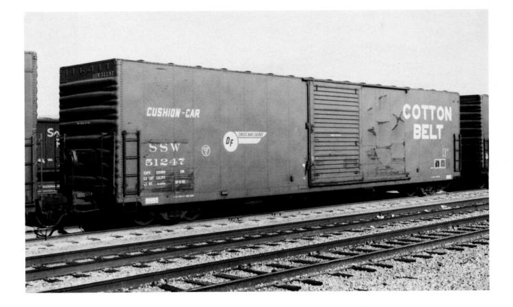
(Above) SSW 51247. Series, SSW 51240-51279. 60'8" IL Plate E. DF Cross Bar Loader equipped. (Below) SSW 57656. 50'2" IL Plate C. DF-B loaders removed 5-91 and converted from RBL to RB.
