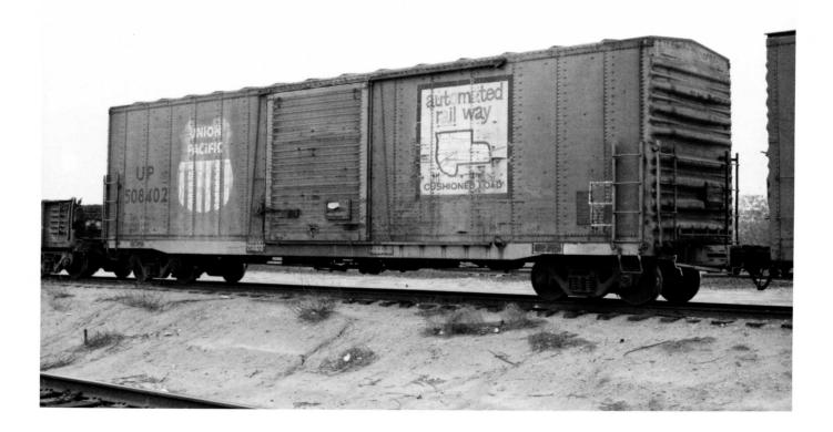
(Above) UP 508402. Class B-70-7. Built 1970 UP OM. 5277 cu ft capacity. (Below) UPFE 462880. Built 3-66 PCF RN. Class R-70-16. Rebuilt 7-92 UP PO. Laramie, WY August 1992.
