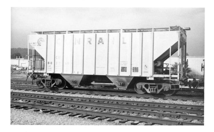
(Above) CR 883789. Class C-13A. 3000 cu ft capacity. Built 9-77 PS BUT. Freight Liner 900 lined. (Below) CRYX 1085. Cryogenic refrigerator car. 4825 cu ft capacity. Atlanta, GA May, 1992.
