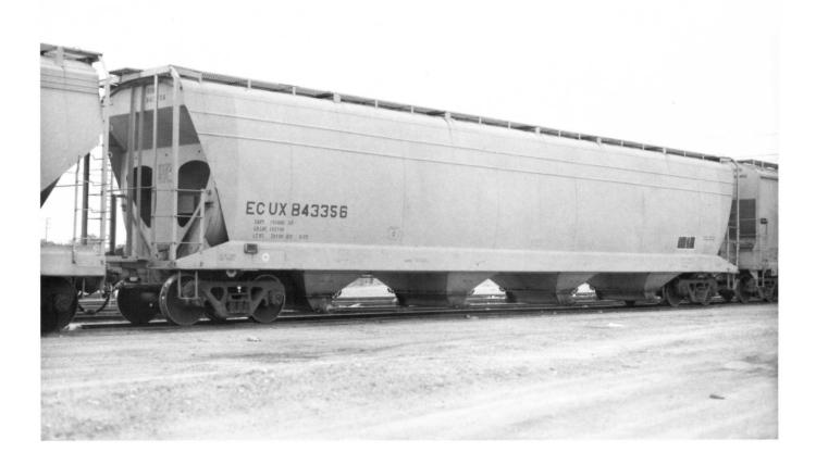
(Above) ECUX 843356. Built 5-75. North American hi-cube quad-hopper design. (Below) ECUX 857033. Built 4-87 TC CH. 5800 cu ft. capacity. Series, ECUX 857000-857049.
