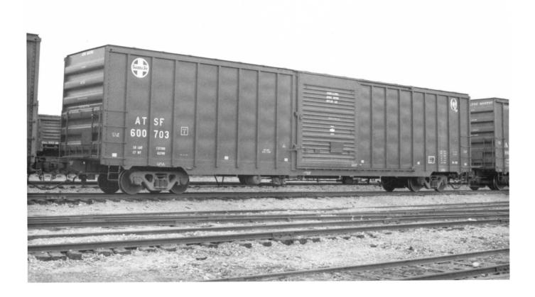
(Above) ATSF 600703. Class Bx-194. Built 1979 by FGE AX. 6333 cu ft capacity. Ptd 4-91. (Below) BN 439281. 100-ton grain hopper. 4427 cu ft capacity. Ptd 11-88.
