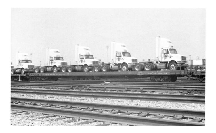
(Above) ATSF 88655. Built in 1969 by GATC. 89-0 L saddleback flat car. Seen here delivering J.B.Hunt tractors. (Below) ATSF 308695. Class GA-161. Built 1967 PS BUT. 4427 cu ft capacity.
