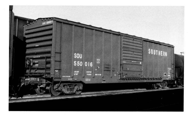
(Above) SOU 550016. Built in 1970 by Pullman-Standard. 145XL. 50'6" Plate C. 5219 cu ft capacity. (Below) SP 691767. Built 3-76 PCF RN. Class B-100-35. Capacity, 5570 cu ft. RBL. 60'10" IL Plate C.
