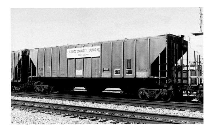
(Above) TLDX 6923. Built 3-67 PS BUT. 4427 cu ft capacity. Lined DC Polyclutch 41303 3-14-67. (Below) TRNX 500368. Built 8-79 QC FW. Trinity 4750 cu ft design.
