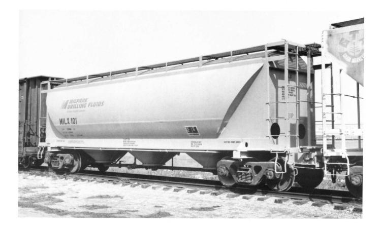
(Above) MILX 101. Built 11-81 BUT MURF. 2785 cu ft capacity. Pressure-differential. (Below) MNS 606. Built 5-73 USEX WA. Lined ADM 475 6-73 TLC, Paris, TN. 4750 cu ft capacity.
