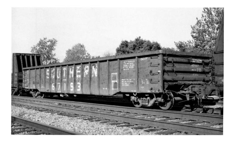
(Above) SOU 67193. Built 4-80 GSC GV. 2264 cu ft capacity. Bessemer, AL, May 1992. (Below) SOU 97749. Class HCS-60. Built in 1967 by Pullman-Standard. 4000 cu ft capacity.
