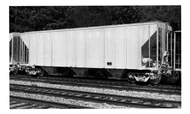
(Above) SOU 6582. Class HCS-17. Built 6-64 by Magor. 4000 cu ft capacity. Spartanburg, SC May 1992. (Below) SOU 42360. Built 2-65 by Pullman-Standard. 10000 cu ft capacity. Painted SOU HE 1-84.
