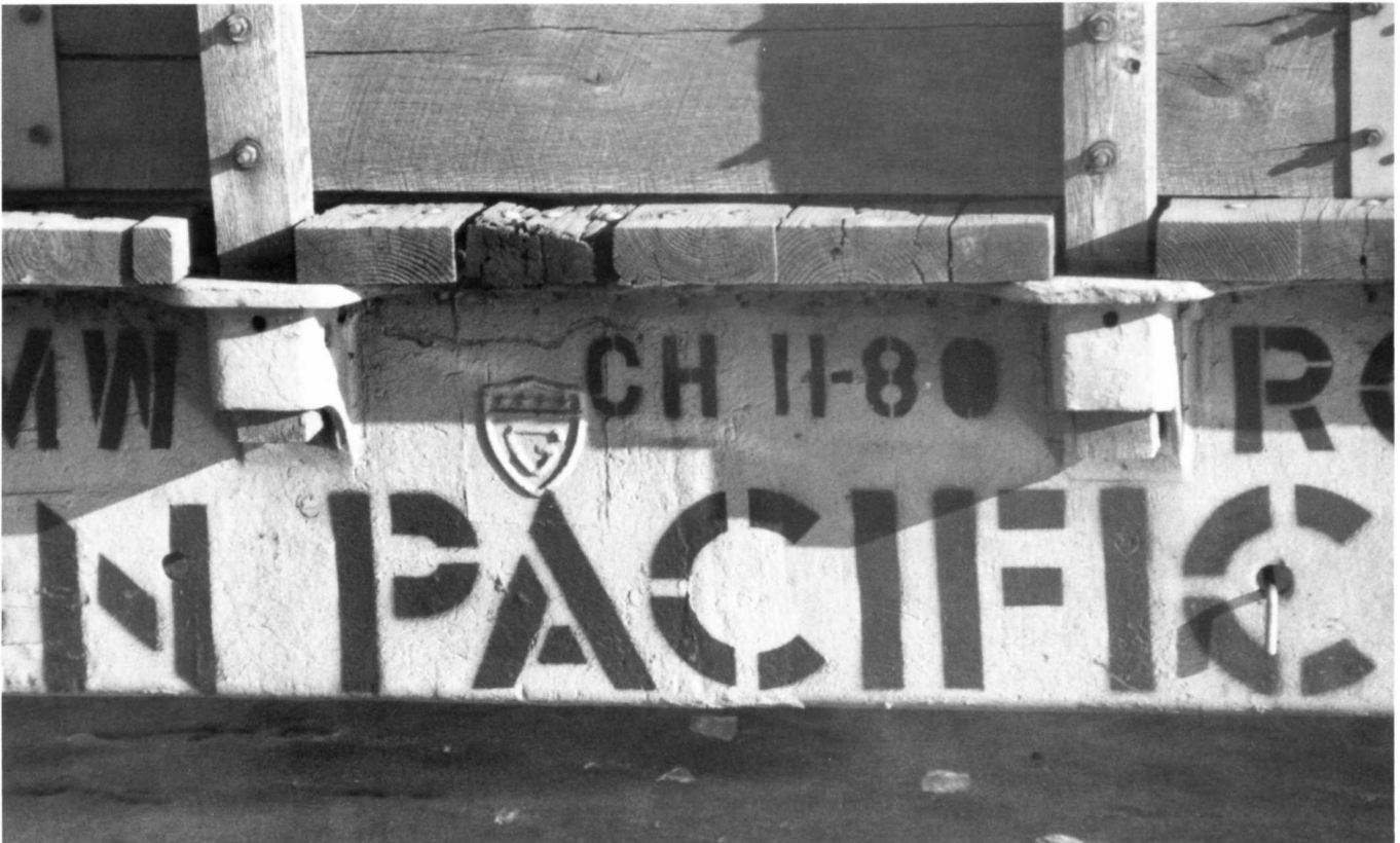
(Above) View of the end of the car. The brake shoe information is in white letters on a black background. Note the gondola side enclosure does not extend all the way to the end of the car. (Below) Note the "G" casting logo of General Steel Castings. Also, note how the frame castings included the stake pockets, minimizing the time required to put the car together and lessening the chances of the pocket loosening or corroding.
