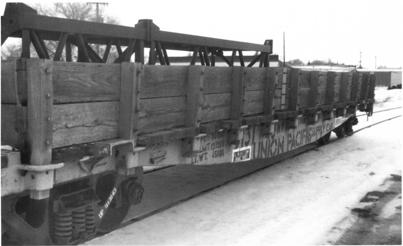
(Above) Close-up #913143. Tapered wood pieces have been hammered into the side stake pockets, and then the wooden board slats bolted onto the side pieces to form a gondola. Note car number on trucks. Wooden boards for deck and sides have not been painted. (Below) Close-up of middle of 913143. This car has been stencilled as a supply car for the roadmaster. Note how stencilling has been crammed into available space. The wood sides that form the sides to make the gondola enclosure have been spliced together with metal plates.
