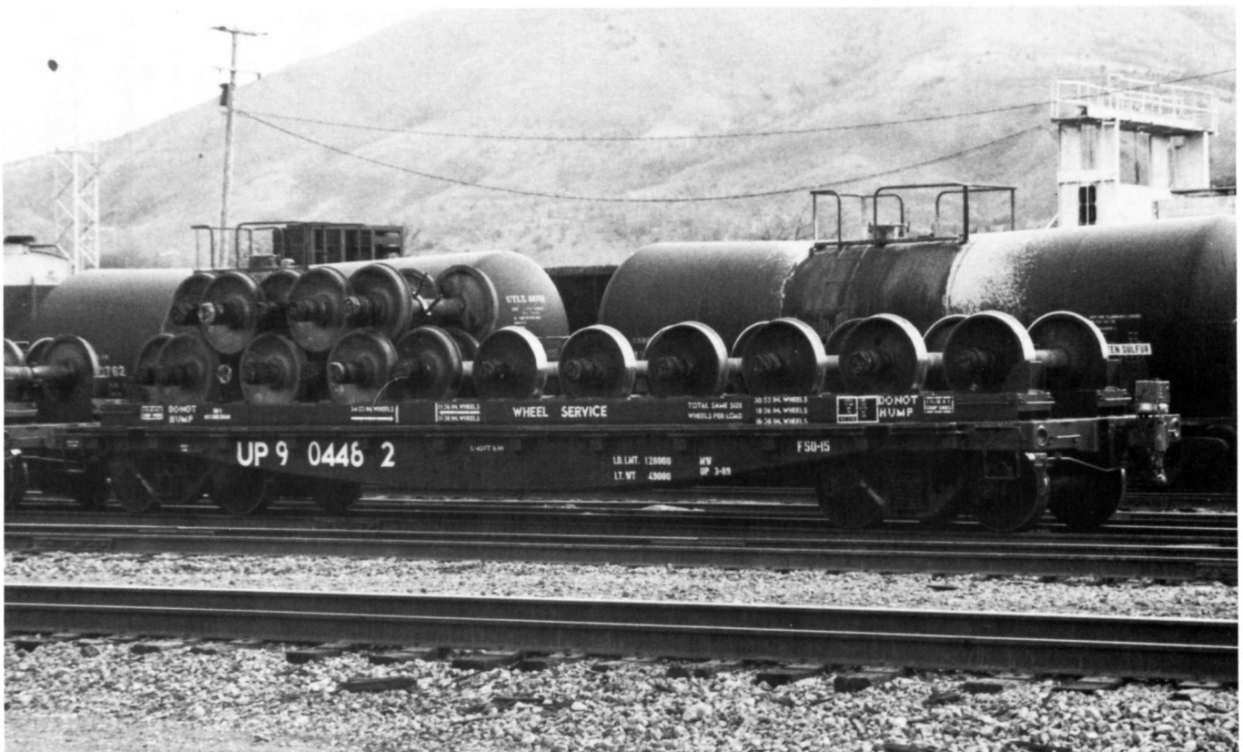
(Above) A wheel car in service, at Pocatello, ID, November 1989. This car was rebuilt to transport various sizes of wheelsets. The car decks have been modified to hold the wheelsets, with a metal framework and openings for the wheels. They also have a walkway using a metal grating on the top. (Below) UP 904482. Pocatello, ID, November 1989.
