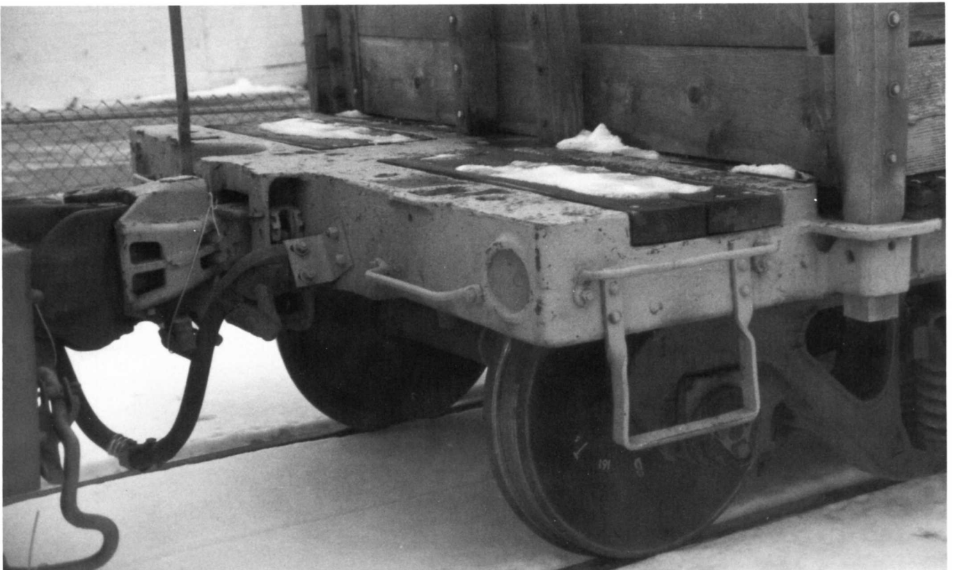
(Above) A close view of the stake pockets, showing how they were reinforced and an integral part of the car frame. The castings had a slightly rough texture, but paint hid most of the rough spots. (Below) "B" end view. Note the poling pockets which were later banned by the ICC as unsafe. The reinforced metal angle by the coupler was used to protect the air hose. The sill step was made from strap metal and riveted onto the car frame.
