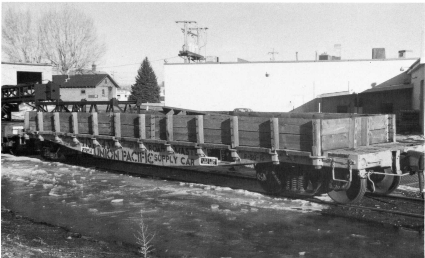
UP 51649 at Nampa, ID in February 1991 where it was being used in MoW service. Painted freight car red with Armour yellow paint. Note the ACI label, installed in the 1960's is still on the side of the car. (Below) UP 913143. This car is painted with the standard MoW green, and sturdy wood sides have been added to form a gondola to hold miscellaneous parts and pieces. Idaho Fall, ID, February 1991.
