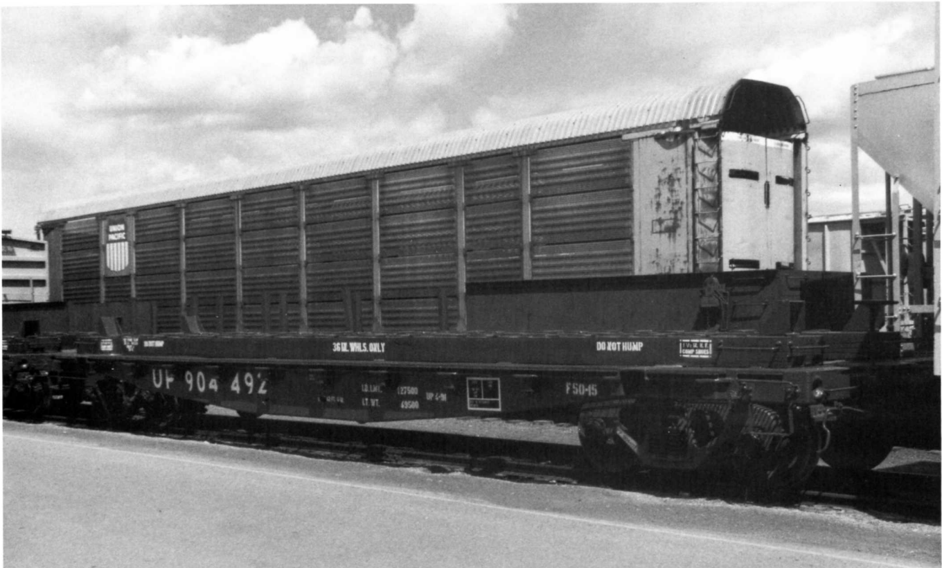
(Above) A view from above showing the brake wheel, flush body casting with deck and uncoupling lever. Note the stake pocket on the end of the car frame which was also used to help secure loads. (Below) UP 904492, painted in Pocatello April 1991. The car is freight car red with white lettering. These wheel cars are used to transport worn wheelsets to the Pocatello shops and return the re-machined wheelsets to the appropriate location. Note the cars are not to be humped. This car is restricted to carrying 36 inch wheels only.
