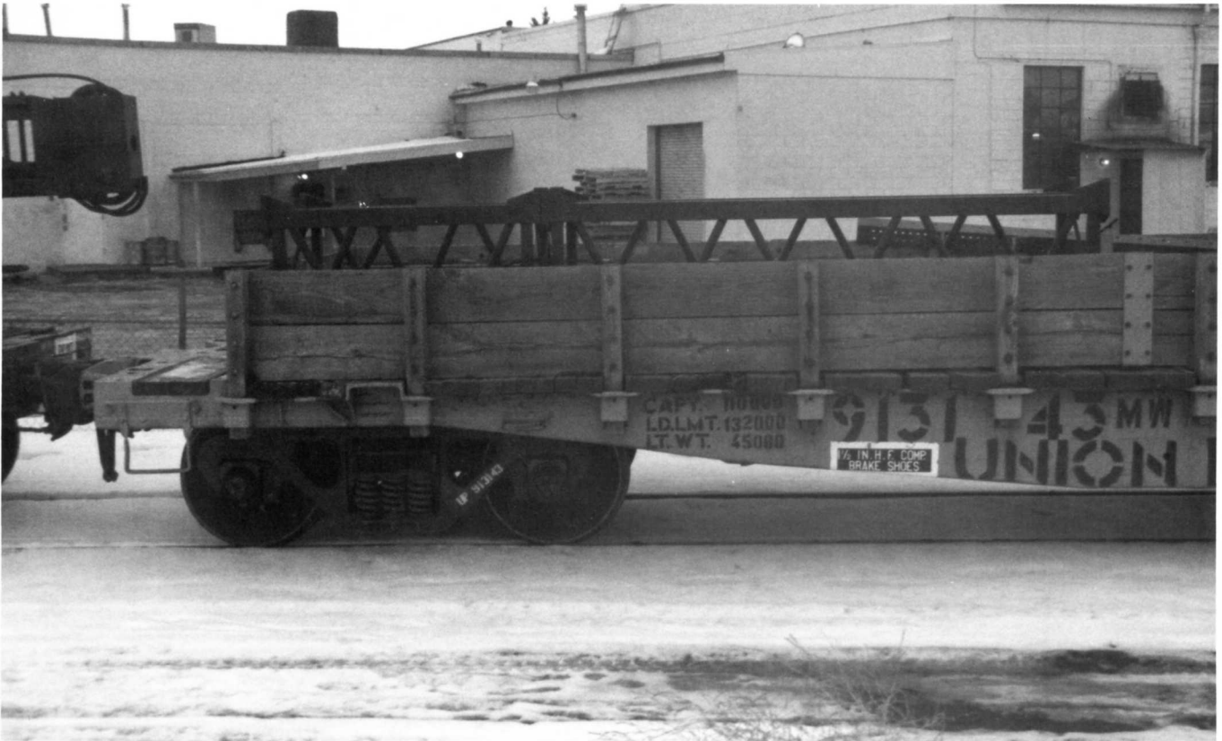
(Above) View of the end of the car. The brake shoe information is in white letters on a black background. Note the gondola side enclosure does not extend all the way to the end of the car. (Below) Note the "G" casting logo of General Steel Castings. Also, note how the frame castings included the stake pockets, minimizing the time required to put the car together and lessening the chances of the pocket loosening or corroding.
