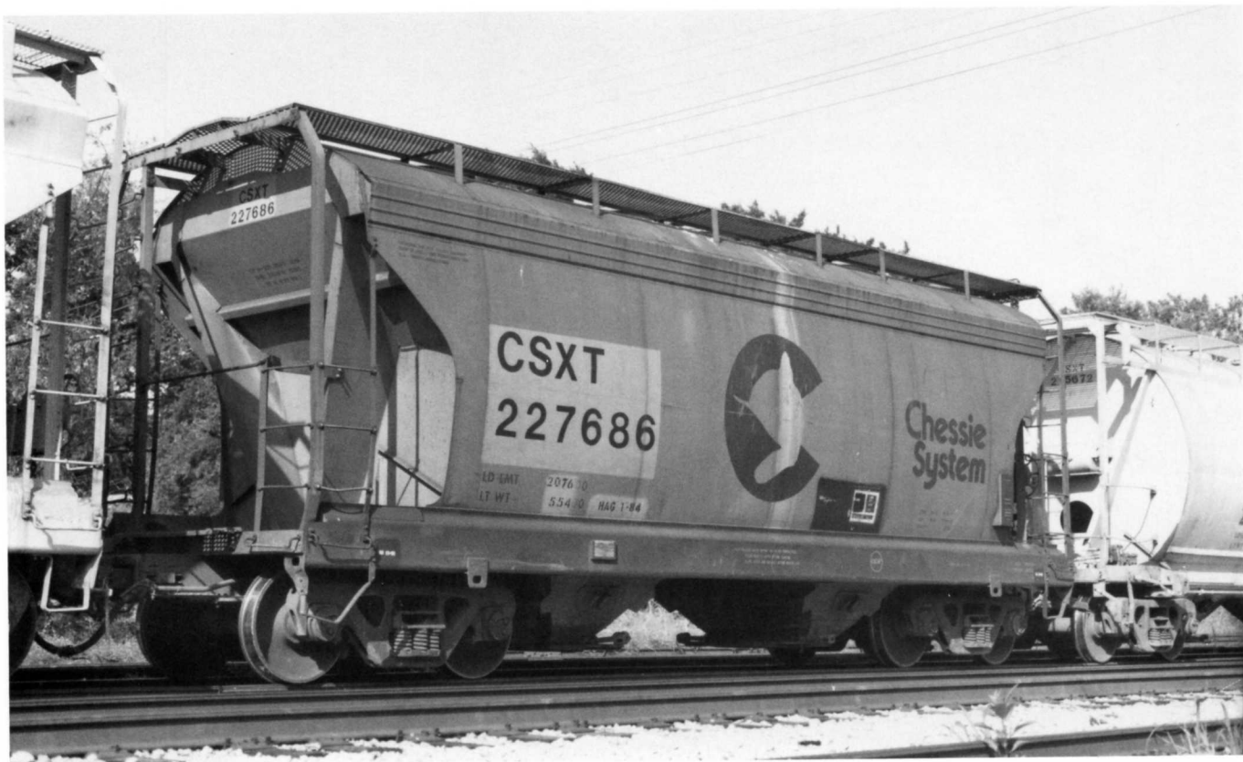
(Above) CSXT 227686. Built in 1976 by ACF. Capacity, 2700 cu ft. (Below) CSXT 240342. Former L&N 204172. Built in 1967 by Pullman-Standard. Capacity, 3510 cu ft.
