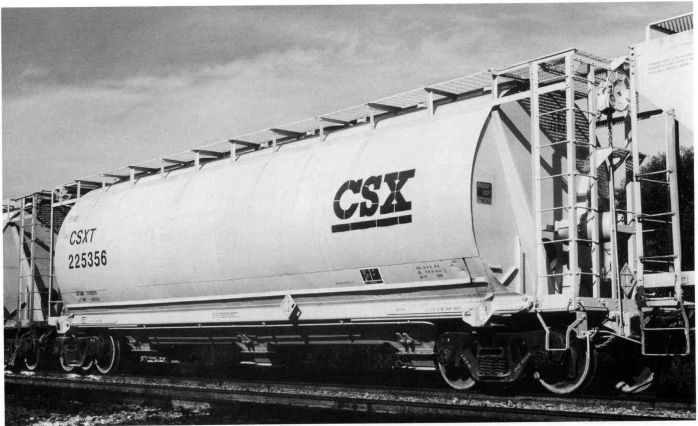
(Above) CSXT 225356. Former B&O 836076. Built in 1964 by ACF. Capacity, 3700 cu ft. (Below) CSXT 225416. Former B&O 836148. Built in 1964 by ACF. Capacity, 3700 cu ft. Despite their 27 years of services, these cars appeared in first class condition in 1991 when these were photographed.
