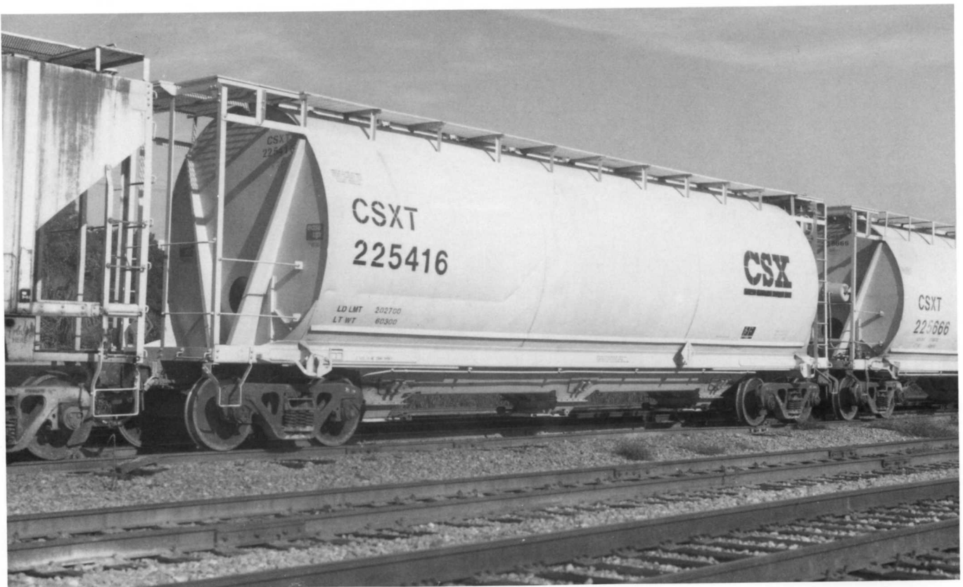
(Above) CSXT 225356. Former B&O 836076. Built in 1964 by ACF. Capacity, 3700 cu ft. (Below) CSXT 225416. Former B&O 836148. Built in 1964 by ACF. Capacity, 3700 cu ft. Despite their 27 years of services, these cars appeared in first class condition in 1991 when these were photographed.
