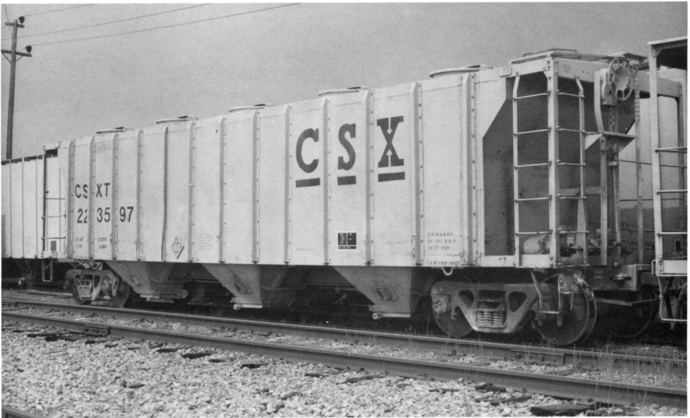
(Above) CSXT 223597. Former ACL 89427. Built in 1965. Painted 5-89 MRS. Capacity, 2929 cu.ft. Note riveted ribs. (Below) CSXT 224398. Former SCL 832078. Originally SAL 32078. Built in 1967. Painted 3-89 RA. Capacity, 2929 cu.ft.
