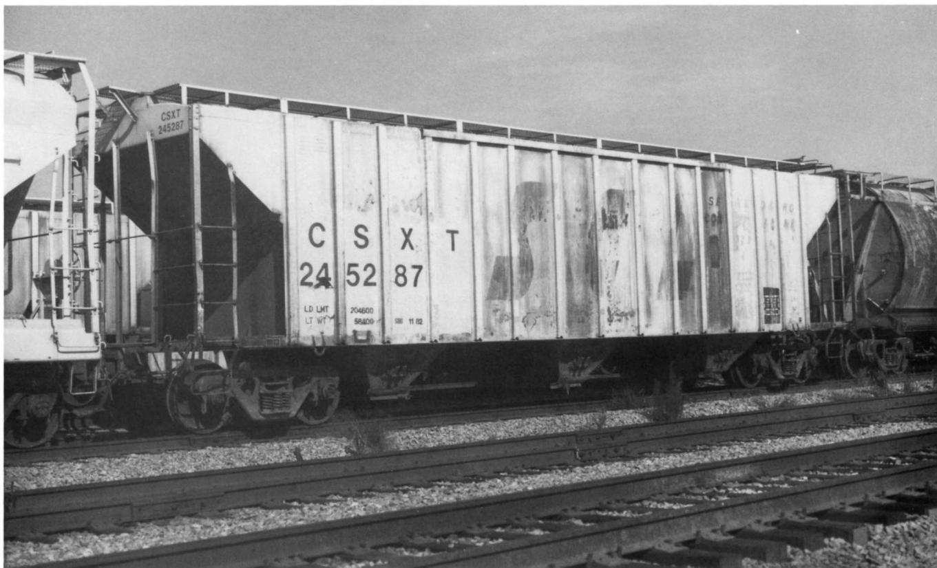
(Above) CSXT 245287. Former SCL 240147. (Below) CSXT 245842. Former SCL 240702. Both cars built in 1973 by Pullman-Standard. Capacity, 4000 cu ft.
