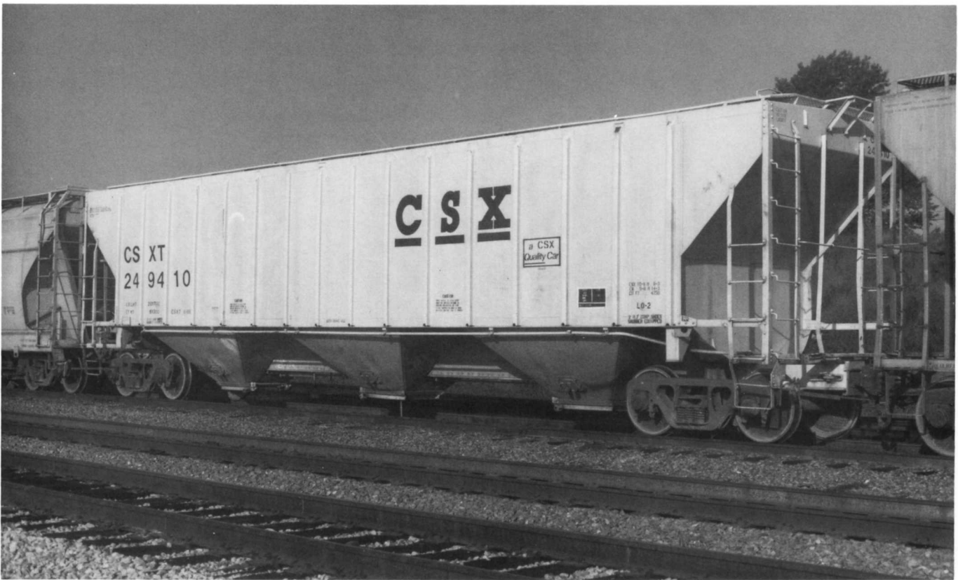
(Above) CSXT 249410. Former SCL 241220. Built in 1970 by Pullman-Standard. Capacity, 4740, cu ft. (incorrectly stencilled 4750 cu ft - note 16 ribs). (Below) CSXT 249557. Former L&N 240017. Built in 1969 by Pullman-Standard. Capacity, 4800 cu ft. Painted 2-89 DR.
