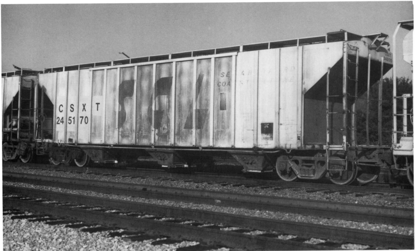
(Above) CSXT 245035. Former SCL 689137 (ACL 89137). Built in 1964 by Pullman-Standard. Capacity, 4136 cu ft. (Below) CSXT 245170. Former SCL 240030. Built in 1973 by Pullman-Standard. Capacity, 4000 cu ft.
