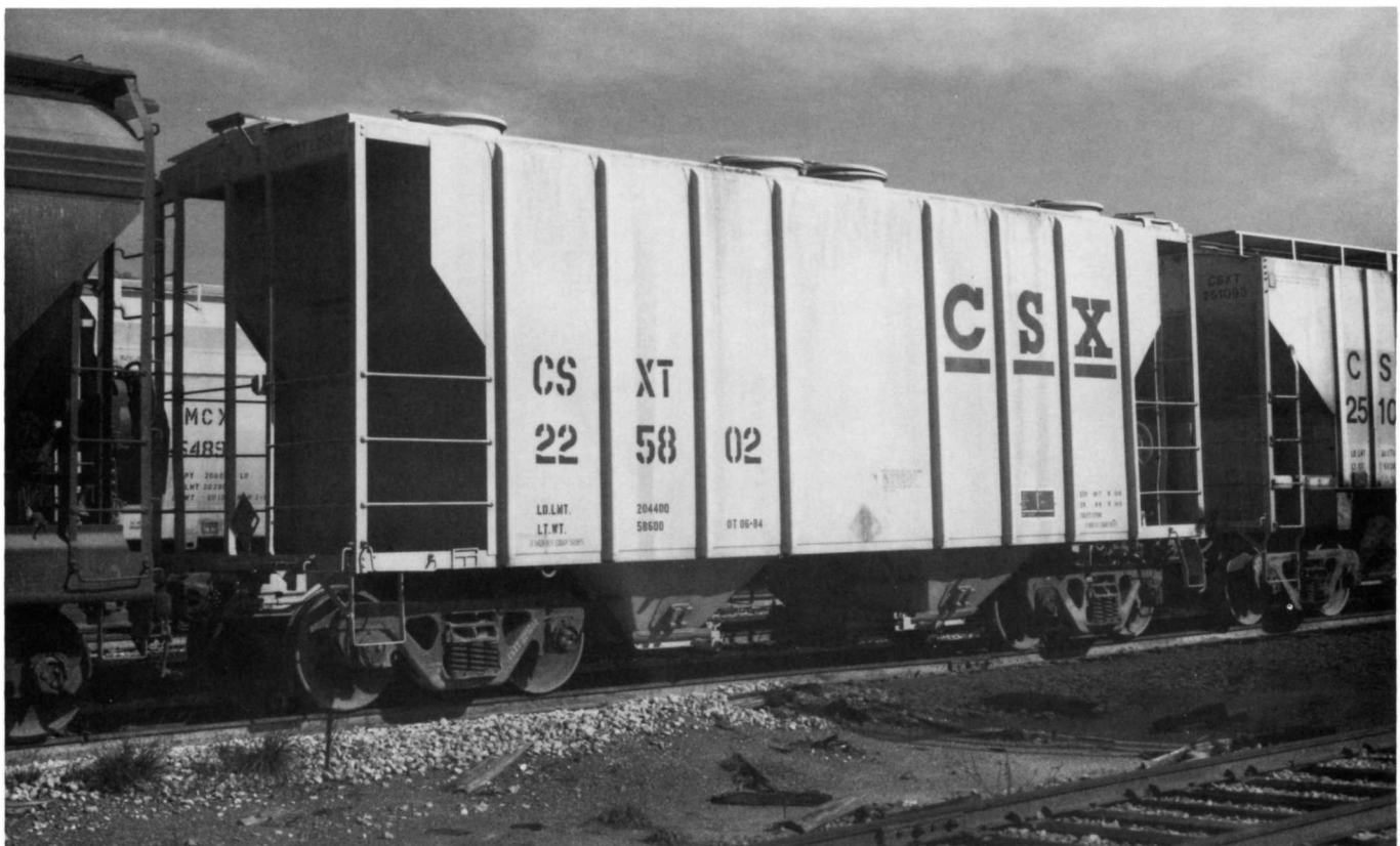
(Above) CSXT 225666. Former B&O 837543. Built in 1965 by ACF. Capacity, 3500 cu.ft. (Below) CSXT 225802. Former B&O 600434. Built in 1966 by FMC. Capacity, 2700 cu.ft. Photographed in Tampa, FL in phosphate service during 1991.
