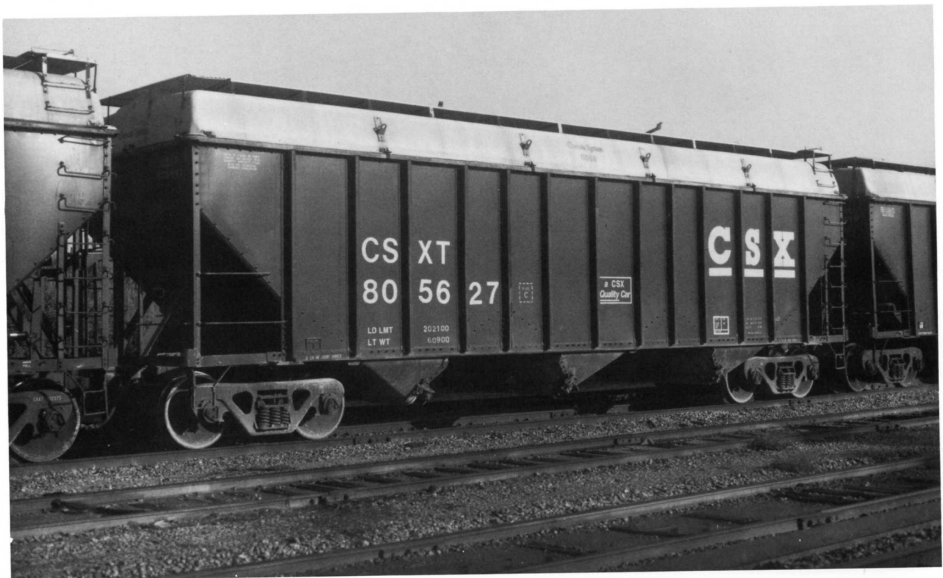
(Above) CSXT 260617. Built in 1989 by Trinity. (See also drawing on pp. 10-11 this issue). (Below) CSXT 805627. Former B&O 66684. Built in 1969 by the Raceland shops. Capacity 3418 cu ft. Often during peak season these coal hoppers with "hopper toppers" are cleaned and used for phosphate transport.
