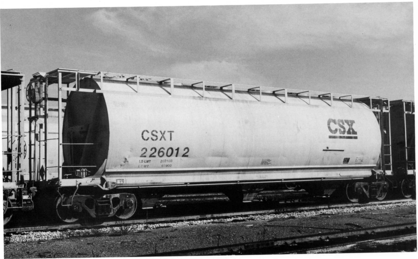
(Above) CSXT 226012. Former B&O 601076. Built in 1966 by ACF. Capacity, 3500 cu ft. (Below) CSXT 226799. Former C&O 601281. Built in 1970 by ACF. Capacity, 3560 cu ft.
