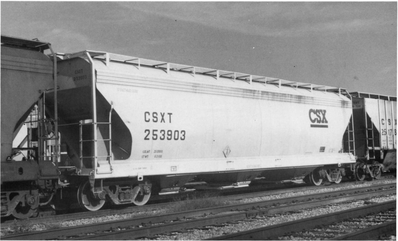
(Above) CSXT 253903. Former B&O 603529. Built in 1971 by ACF. Capacity 4707 cu ft. (Below) CSXT 254522. Built in 1978 by ACF.
