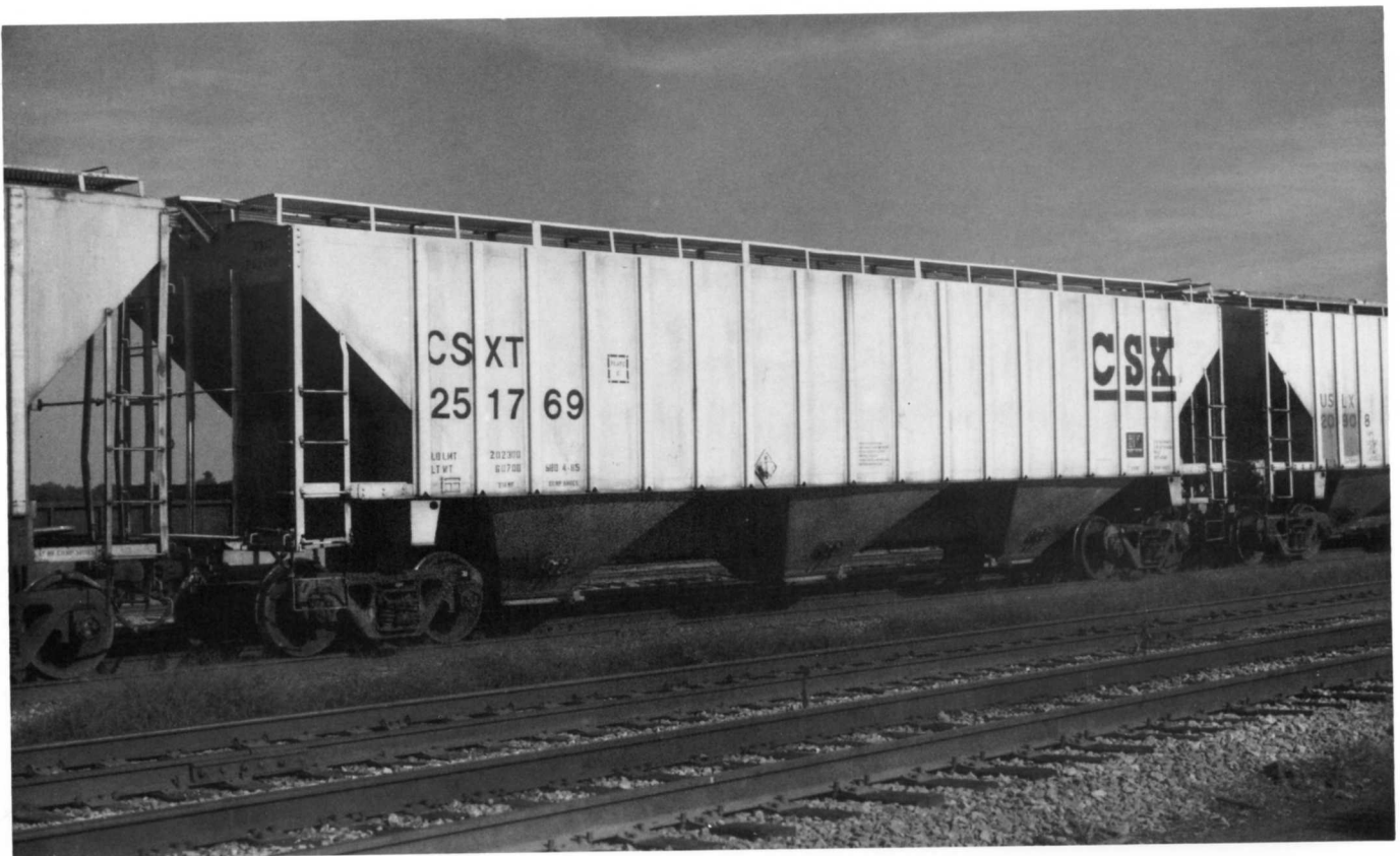
(Above) CSXT 250680. Former L&N 242620. Built in 1981 by Pullman-Standard. Capacity 4750 cu ft. Note 18 ribs. (Below) CSXT 251769. Former SCL 242310. Built in 1977 by Pullman-Standard. Capacity, 4750 cu ft.
