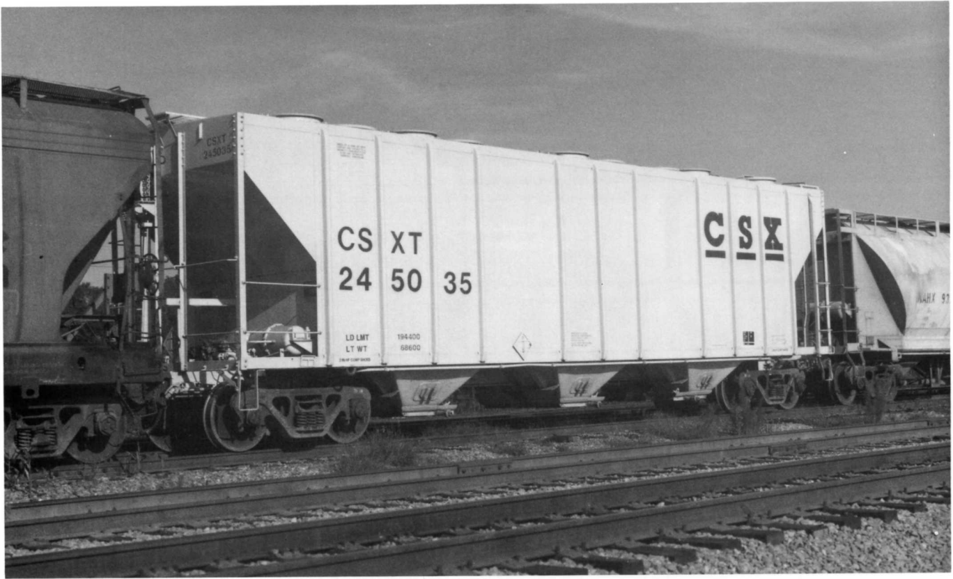
(Above) CSXT 245035. Former SCL 689137 (ACL 89137). Built in 1964 by Pullman-Standard. Capacity, 4136 cu ft. (Below) CSXT 245170. Former SCL 240030. Built in 1973 by Pullman-Standard. Capacity, 4000 cu ft.
