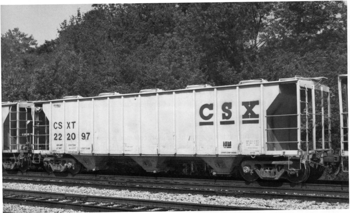
(Above) CSXT 222097. Former ACL 121127. Built by Pullman-Standard in 1966. Capacity, 2929 cu ft. (Below) CSXT 223329. Former ACL 122359. Built in 1966. Painted 5-89 HAR GRDN. Capacity, 2929 cu ft. Note welded ribs.
