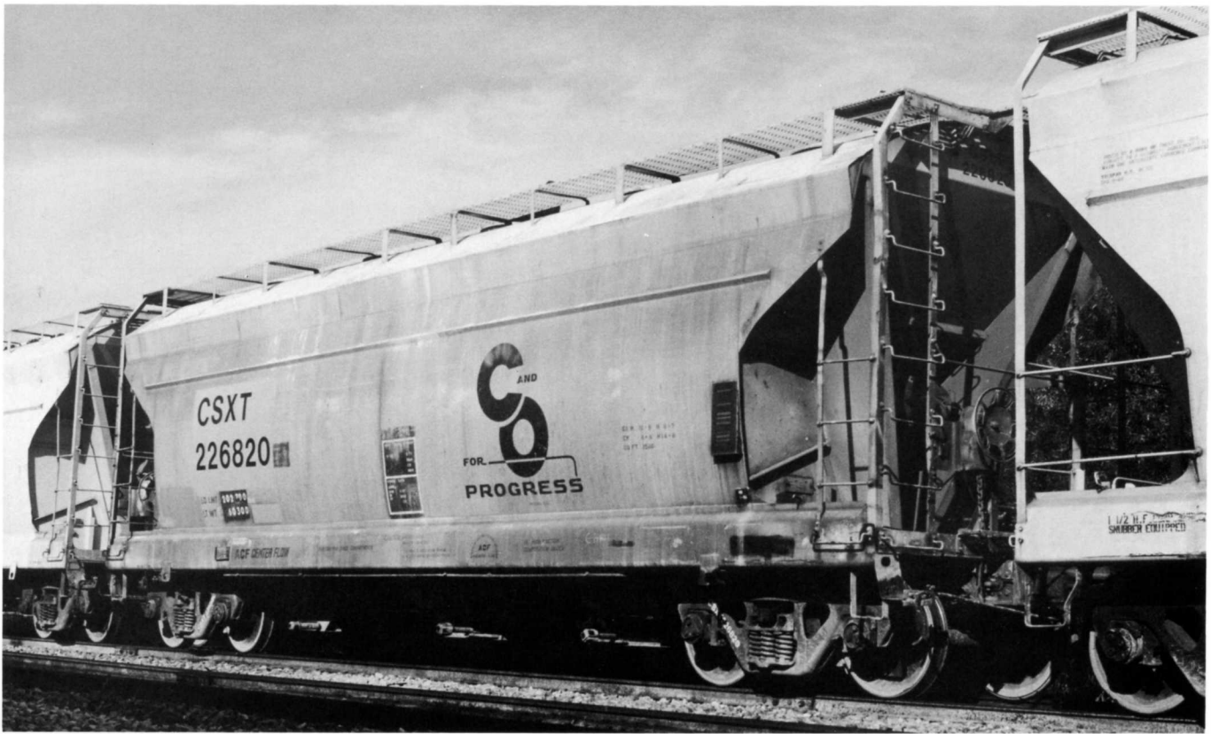
(Above) CSXT 226820. Former C&O 601303. (Below) CSXT 226894. Former C&O 601377. Both cars built in 1970 by ACF. Capacity, 3560 cu ft.
