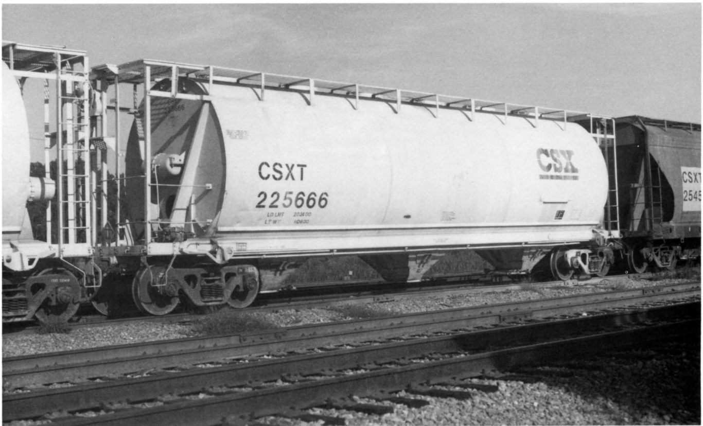
(Above) CSXT 225666. Former B&O 837543. Built in 1965 by ACF. Capacity, 3500 cu.ft. (Below) CSXT 225802. Former B&O 600434. Built in 1966 by FMC. Capacity, 2700 cu.ft. Photographed in Tampa, FL in phosphate service during 1991.
