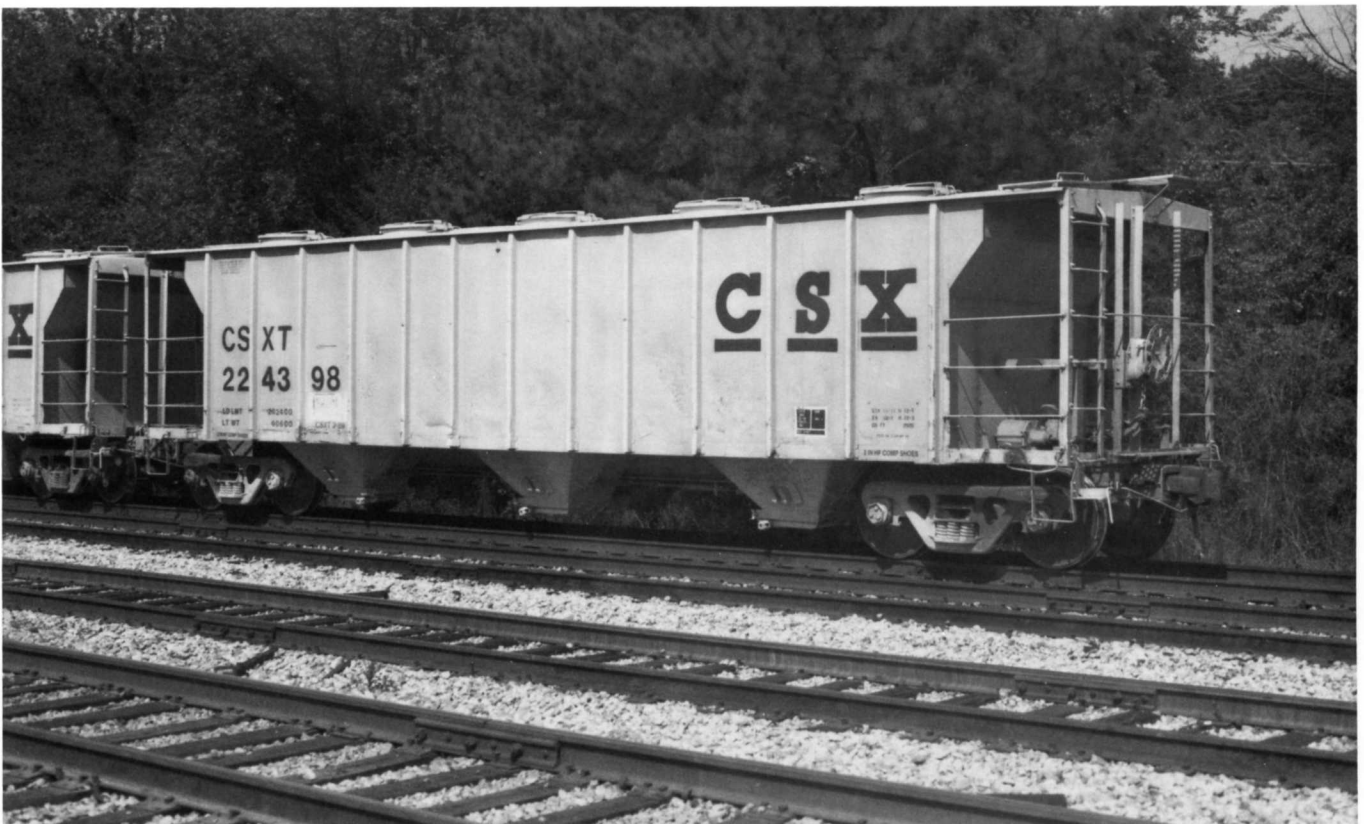
(Above) CSXT 223597. Former ACL 89427. Built in 1965. Painted 5-89 MRS. Capacity, 2929 cu.ft. Note riveted ribs. (Below) CSXT 224398. Former SCL 832078. Originally SAL 32078. Built in 1967. Painted 3-89 RA. Capacity, 2929 cu.ft.
