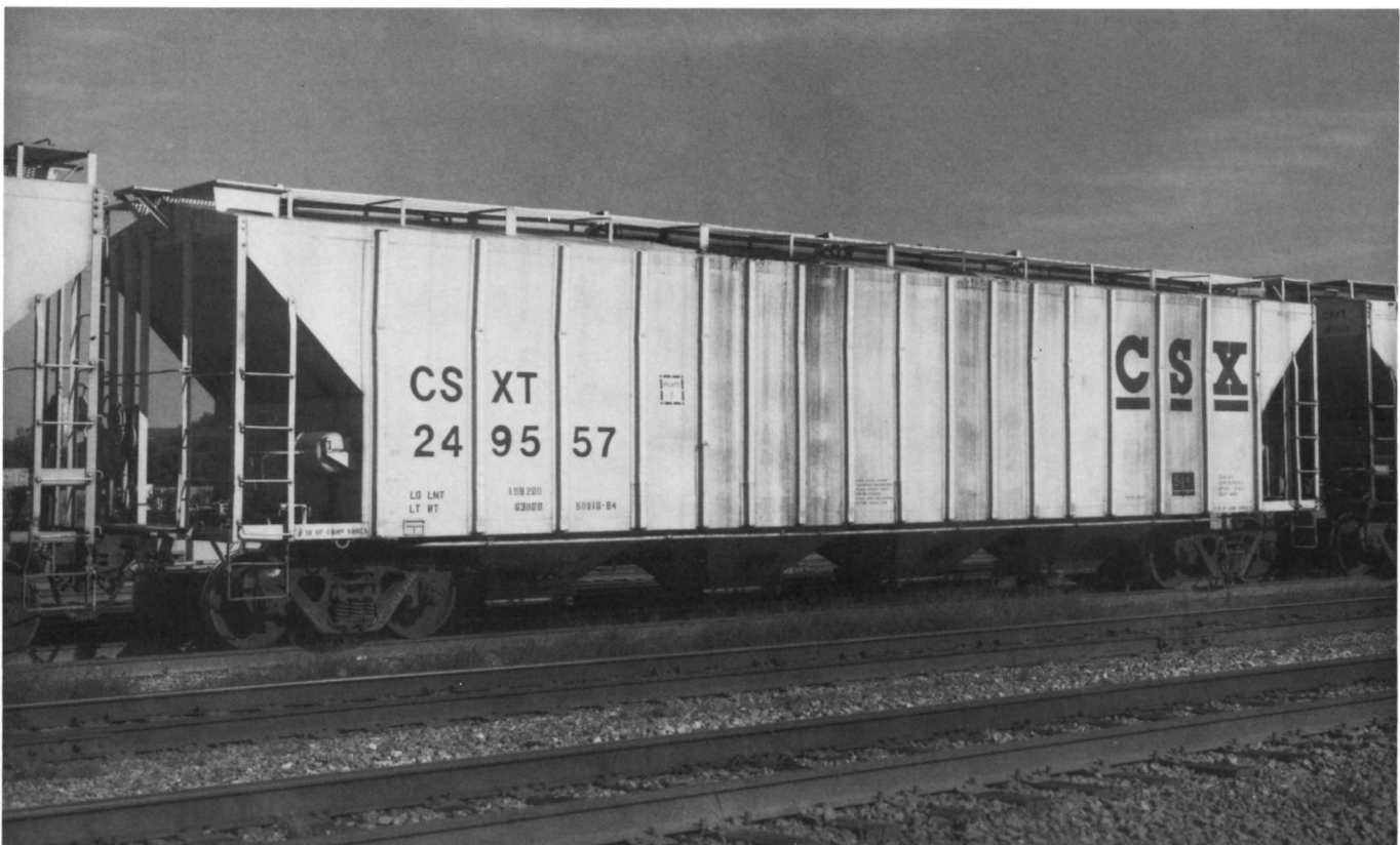
(Above) CSXT 249410. Former SCL 241220. Built in 1970 by Pullman-Standard. Capacity, 4740, cu ft. (incorrectly stencilled 4750 cu ft - note 16 ribs). (Below) CSXT 249557. Former L&N 240017. Built in 1969 by Pullman-Standard. Capacity, 4800 cu ft. Painted 2-89 DR.
