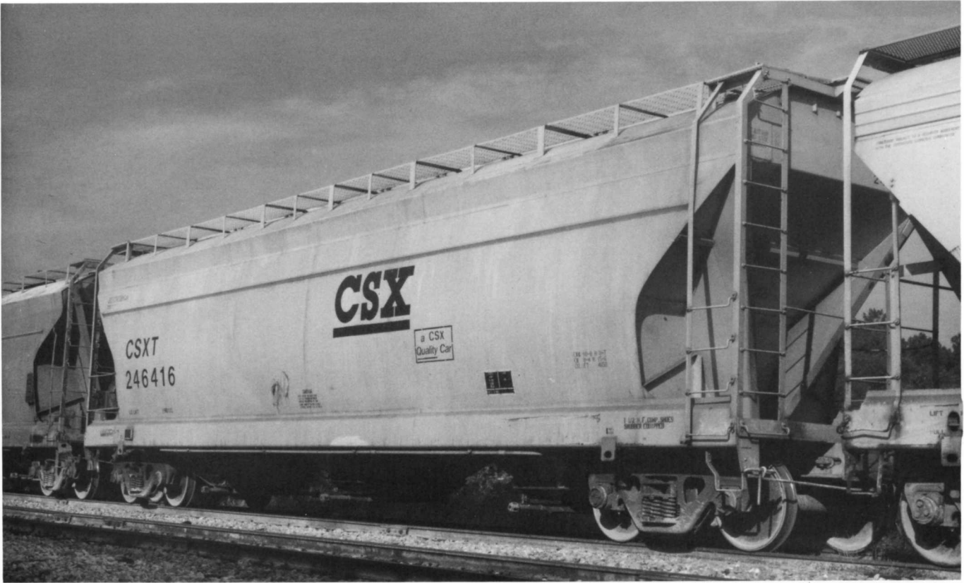
(Above) CSXT 246416. Former L&N 200304. Built in 1964 by ACF. Capacity, 4650 cu ft. Note the "Quality Car" slogan, rarely seen on covered hoppers in fertilizer service. (Below) CSXT 246740. Former L&N 240602. Built in 1971 by ACF. Capacity, 4600 cu ft. Originally restricted to grain service.
