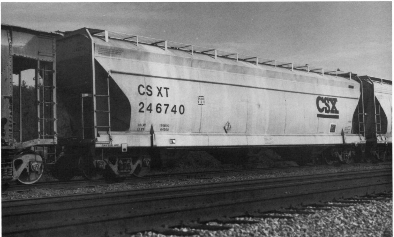
(Above) CSXT 246416. Former L&N 200304. Built in 1964 by ACF. Capacity, 4650 cu ft. Note the "Quality Car" slogan, rarely seen on covered hoppers in fertilizer service. (Below) CSXT 246740. Former L&N 240602. Built in 1971 by ACF. Capacity, 4600 cu ft. Originally restricted to grain service.
