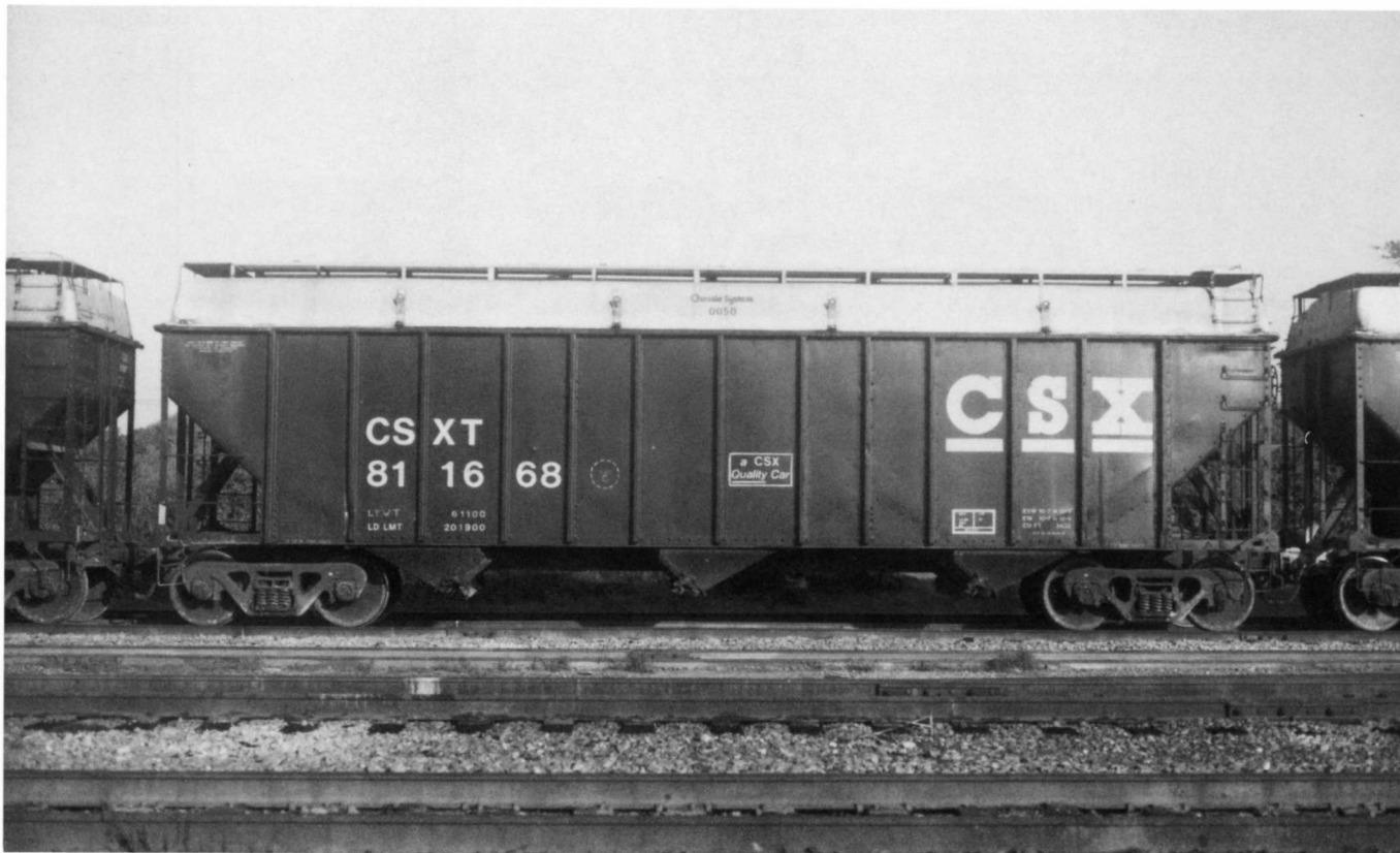
(Above) CSXT 811668. Former C&O 62435. Another example of the "hopper topper" use. (Below) Detail of logo as painted by the Raceland shops in 9-90. Note the drip ledge to the left under the logo.
