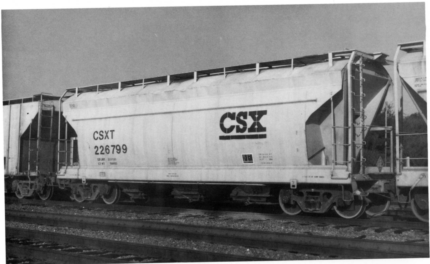
(Above) CSXT 226012. Former B&O 601076. Built in 1966 by ACF. Capacity, 3500 cu ft. (Below) CSXT 226799. Former C&O 601281. Built in 1970 by ACF. Capacity, 3560 cu ft.
