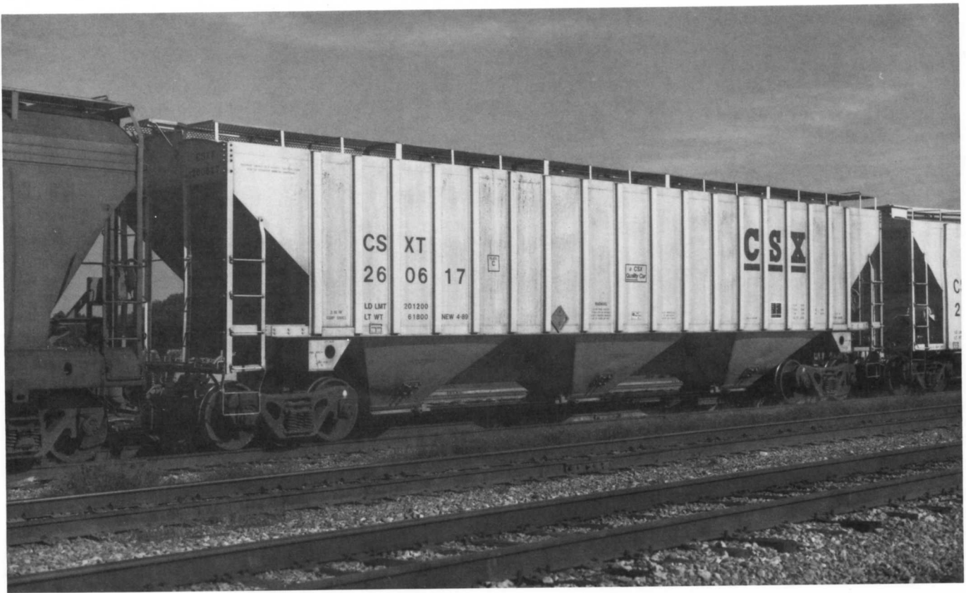
(Above) CSXT 260617. Built in 1989 by Trinity. (See also drawing on pp. 10-11 this issue). (Below) CSXT 805627. Former B&O 66684. Built in 1969 by the Raceland shops. Capacity 3418 cu ft. Often during peak season these coal hoppers with "hopper toppers" are cleaned and used for phosphate transport.
