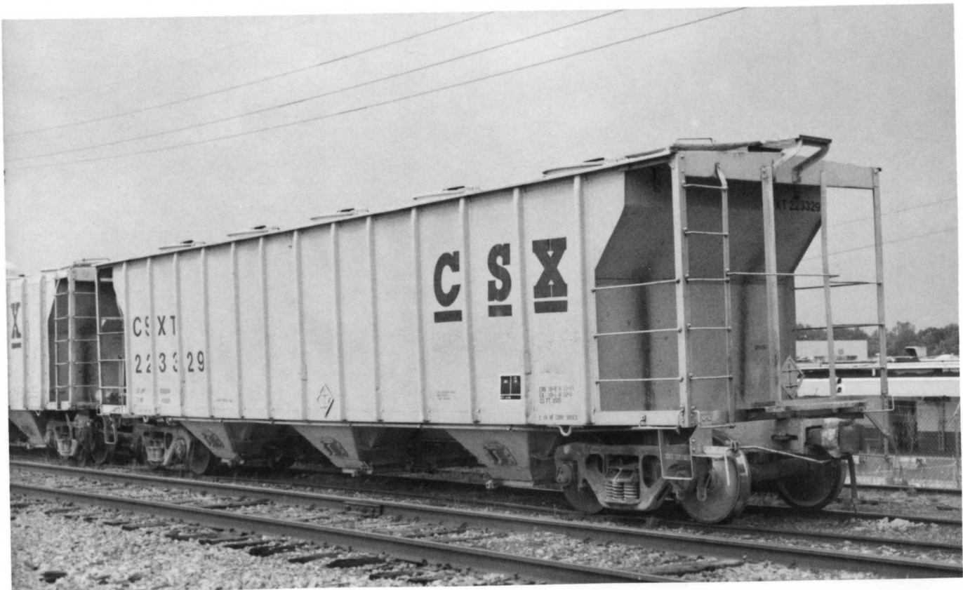
(Above) CSXT 222097. Former ACL 121127. Built by Pullman-Standard in 1966. Capacity, 2929 cu ft. (Below) CSXT 223329. Former ACL 122359. Built in 1966. Painted 5-89 HAR GRDN. Capacity, 2929 cu ft. Note welded ribs.
