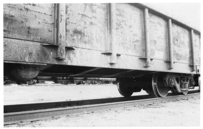
(Above) NSR 11107, close up on side. (Below) A nice view showing the gussets and the underside of the car. Note how the side posts are capped on the bottoms. Both photos by James Kinkaid.
