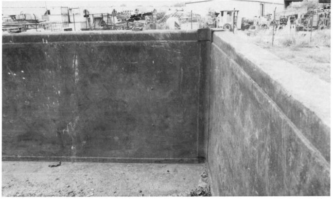
(Above) NSR 11107. This view was taken from the side ladder and looks across the car. The smooth side sheets and floor make for an exceptionally clean interior. (Below) This view should give you a better understanding of how the end beams were arranged with the stiffeners welded over them. The bases of the four-inch "I" beams are hidden by the stiffeners. Both photos by James Kinkaid.
