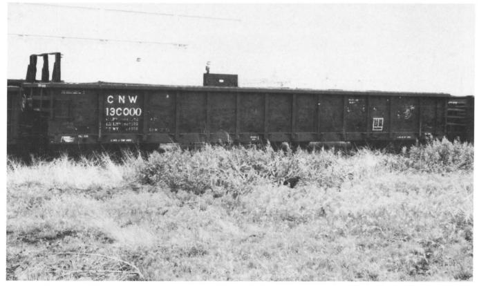
(Above) CNW 130000, the class car of the 130000-130299 series (SIECO ATL, 5-80). What's left of one of the bulkheads can be seen at the left end of the car. Note that the last two "00" digits have a different style than the rest. This car also has a continuous tie down rod (not used very often in scrap service). May 1991. (Below) CNW 340016. This car illustrates the height difference between the 2244 and the 2493 cuft cars (note CNW 130000, on right). May 1991. Both photos by James Kinkaid.
