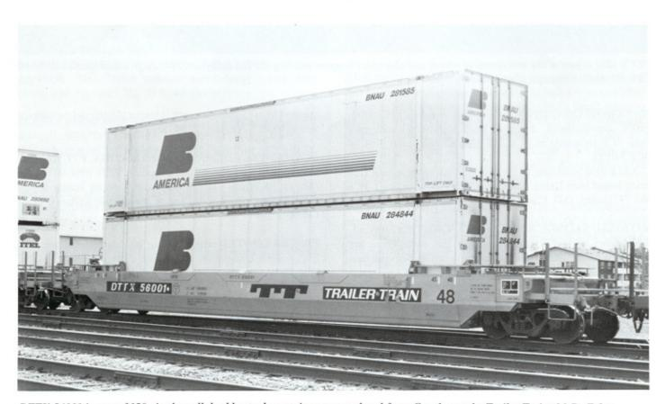
DTTX 56001 is one of 150 single-well double stack container cars ordered from Gunderson by Trailer Train. M.B. Foley.
