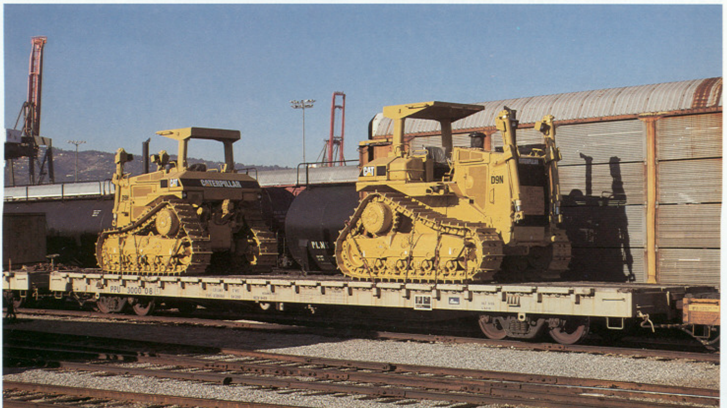
PPU 300008. Built 9-89 by Thrall Car. Tractor flat car (cf. FCJ 35:5). San Pedro, CA. December 1990. David G. Casdorff.
