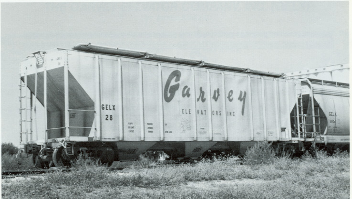
GELX 28. This car, one of the Pullman-Standard 4427 cu.ft. cars from the first P-S order, was destroyed 10-12-90. Photographed August 1990.
