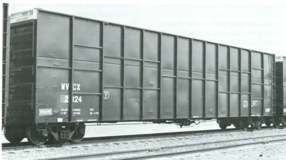
WVCX 2124. This car had just been renumbered from WVCX 20124. Former Southern Pacific woodchip gondola car class G-100-17. Colton, CA. David G. Casdorff.
