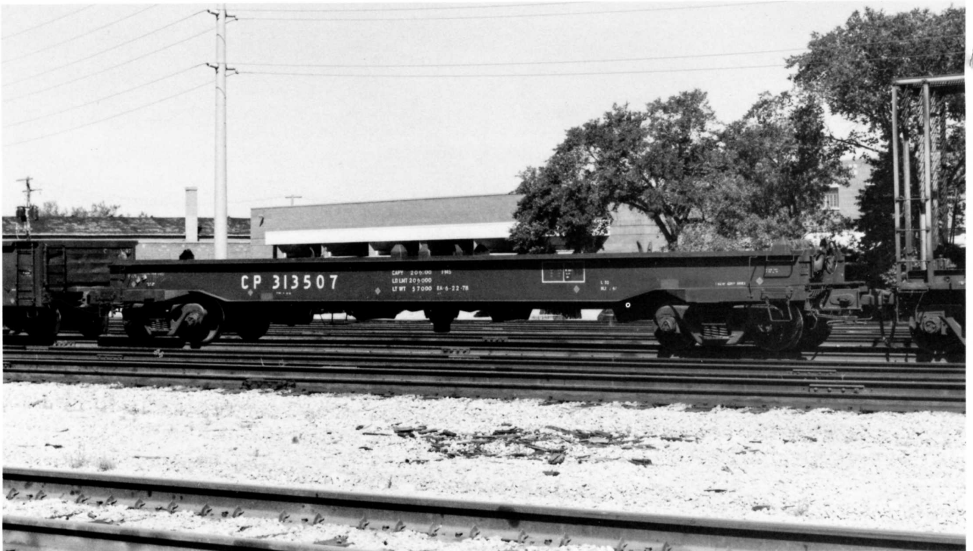
CP 313507. Built 2-67. AAR class FMS for steel coils. Regina, SASK. July 25, 1987.
