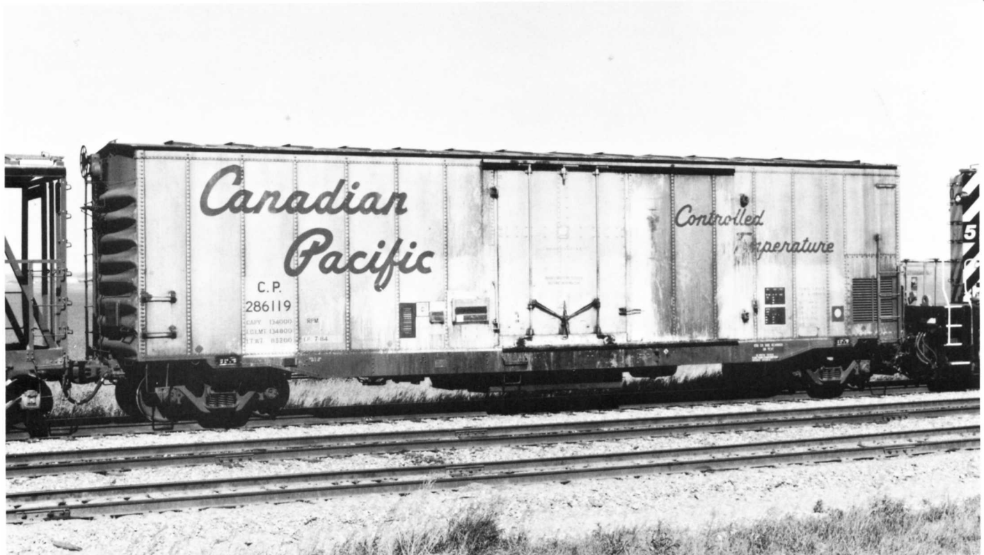
CP 286119. AAR class RP. 44'0" IL. Equipped with meat rails. June 13, 1987.
