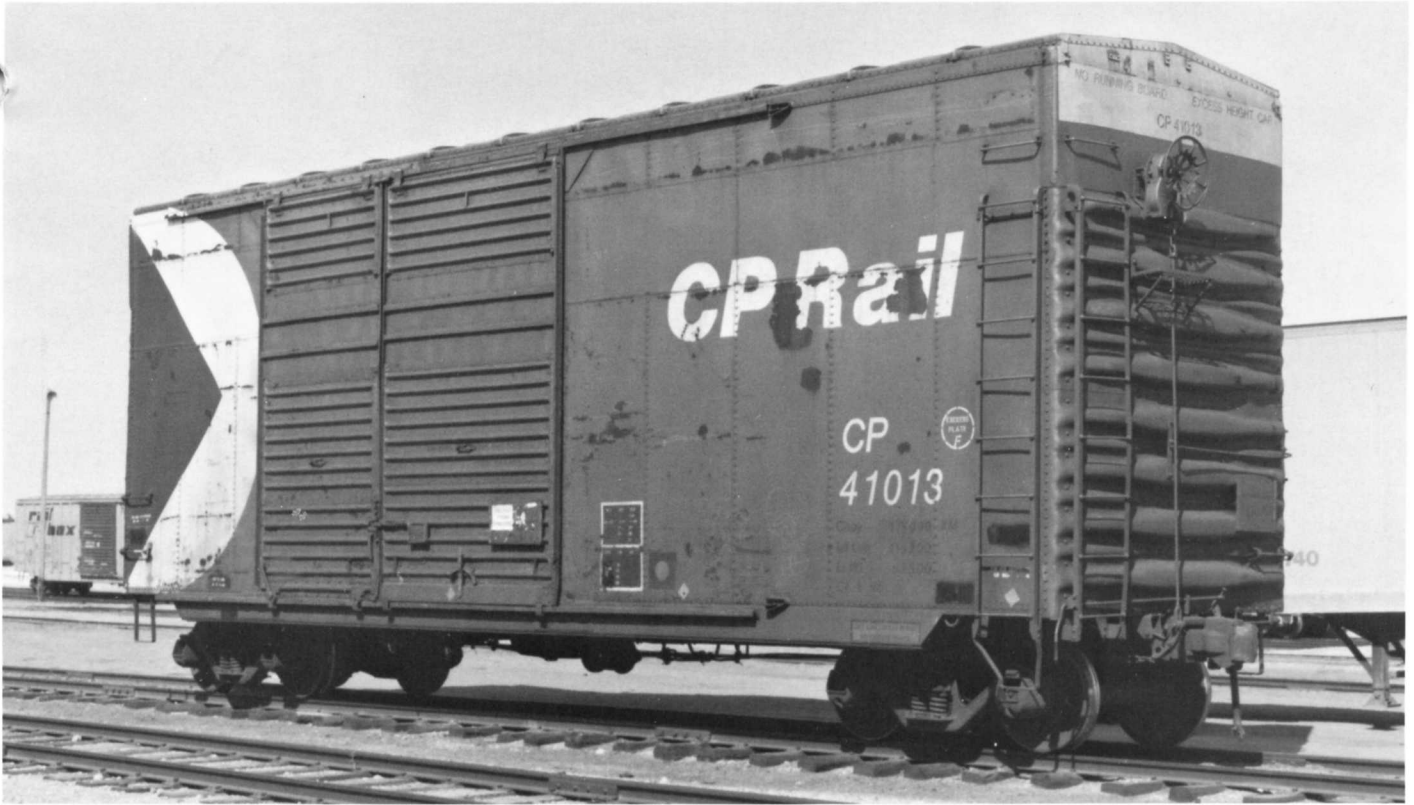
CP41013. Built 12-52. AAR class XM. 40'6" IL. Clearance plate F+. May 17, 1987.
