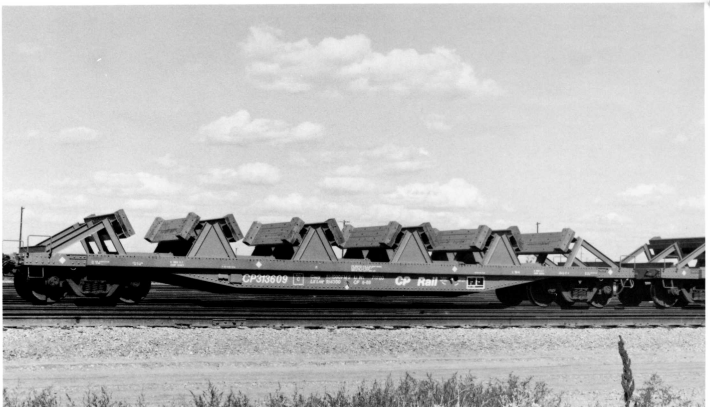
CP 313609. Built 1-52. AAR class FMS for steel coils. July 16, 1988.
