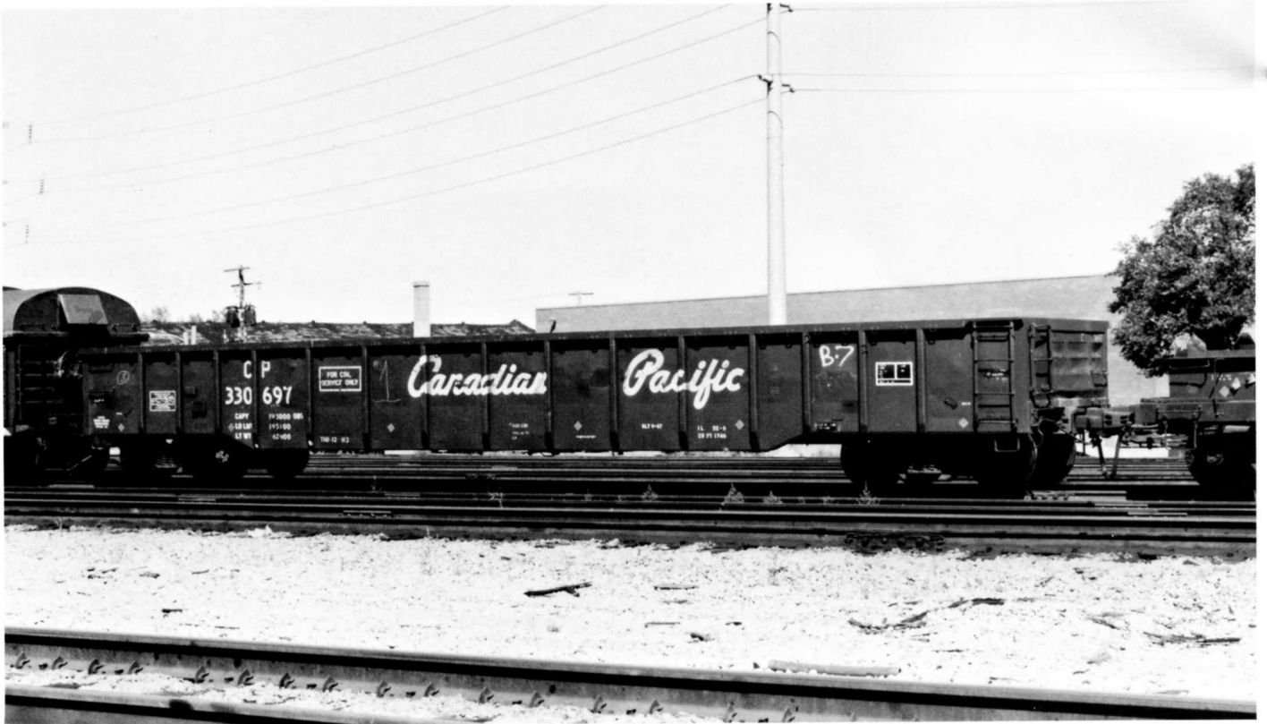
CP 330697. Built 9-67. AAR class GBS for coil steel. Regina, SASK. July 25, 1987.
