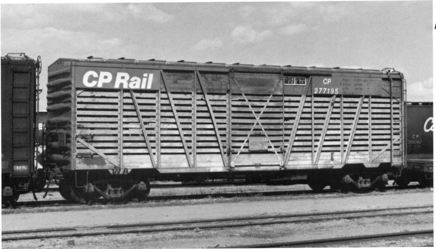
CP 277195. Built 4-58. Stock car. 40'6" IL. June 22, 1990.
