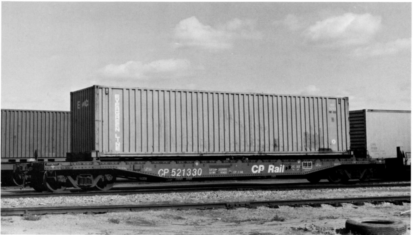
CP 521330. Built 1-52. AAR class FC. Container flat car. 50'6" IL. July 29, 1990.
