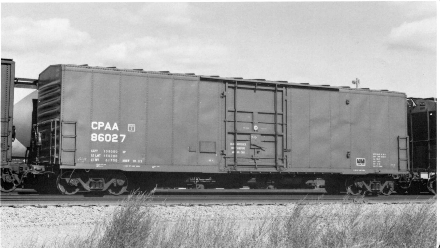
CPAA 86027. Built in 1969 by NSC. Ex-MDW. AAR class XP. 50'7" IL. August 27, 1988.
