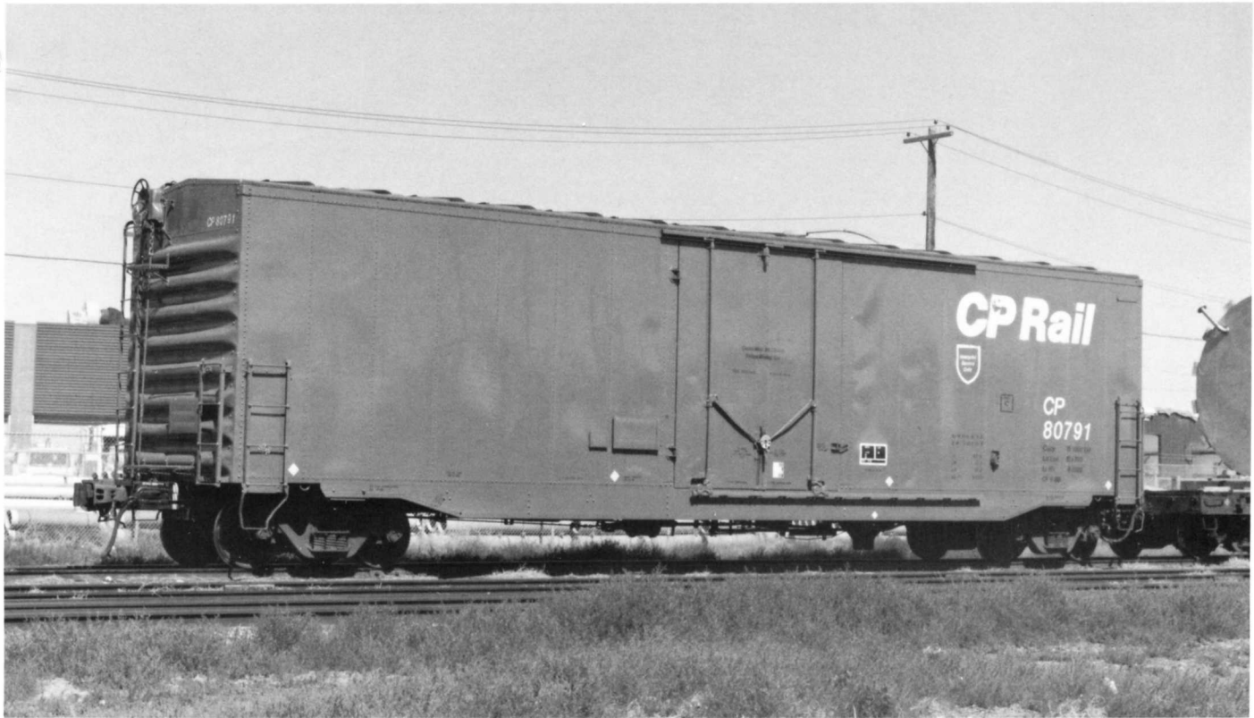
CP 80791. Built 4-65 by Hawker Siddeley. AAR class XM. 50'6" IL. Series: CP 80500-80999. Capacity: 5090 cu.ft. July 23, 1988.
