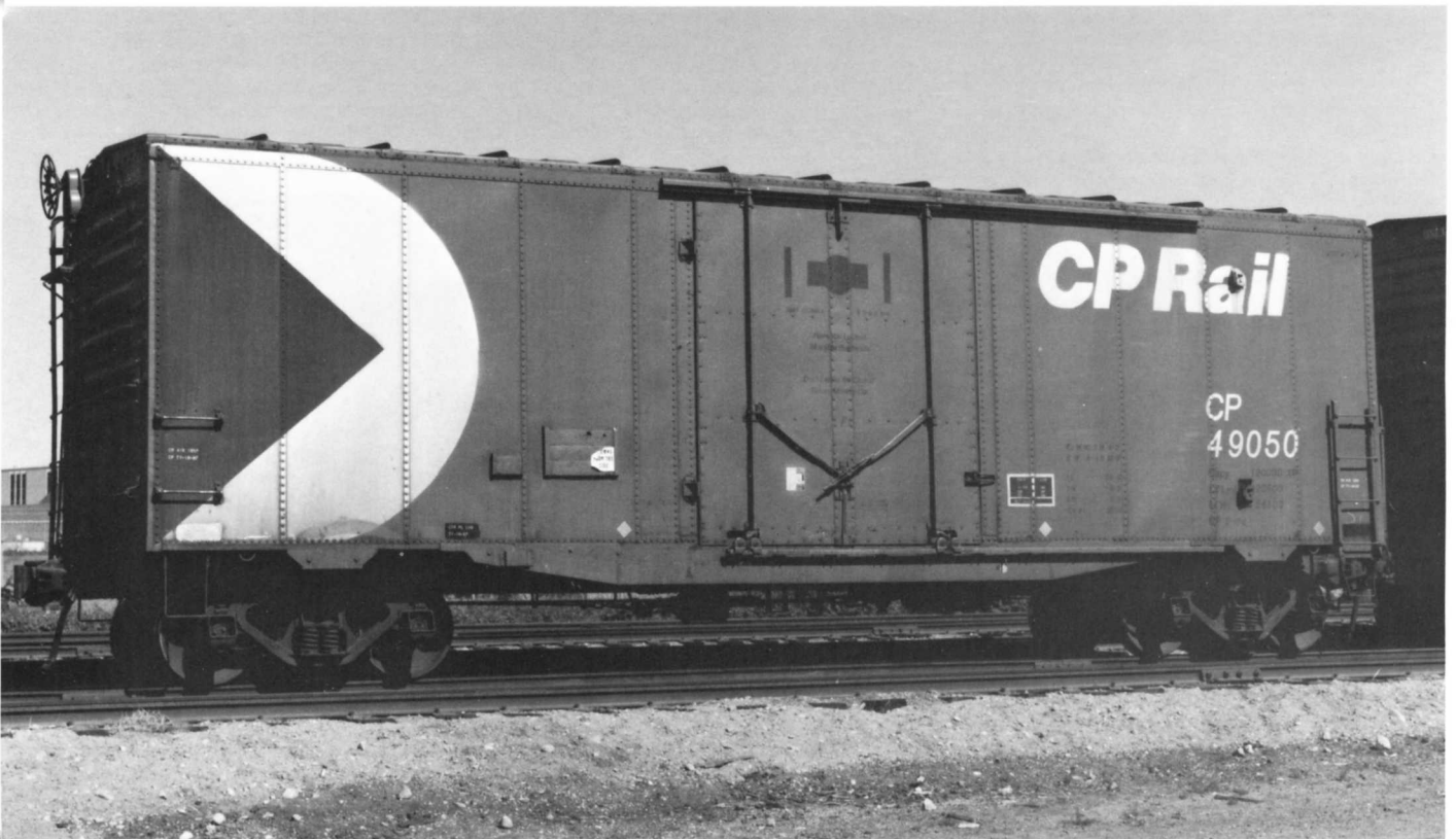
CP 49050. Built 11-55. AAR class XP for packaged petroleum products. Series: CP 49050-49074. June 19, 1988.
