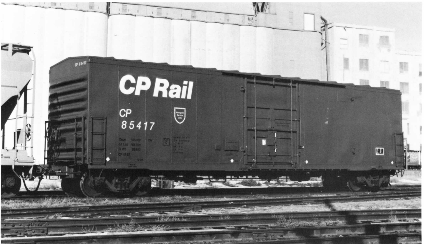
CP 85417. Built 7-69. AAR class XM. 50'7" IL. Series: CP 85000-85499. Feb. 27, 1988.
