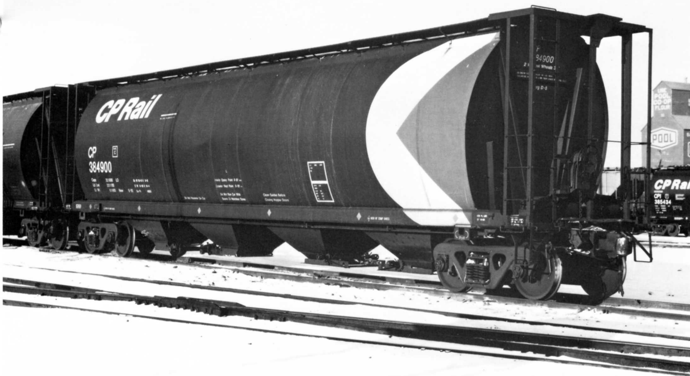
CP 384900. Built 1981 by HST. AAR class LO. Series: 384500-3848999. Capacity: 4550 cu.ft. January 17, 1987.
