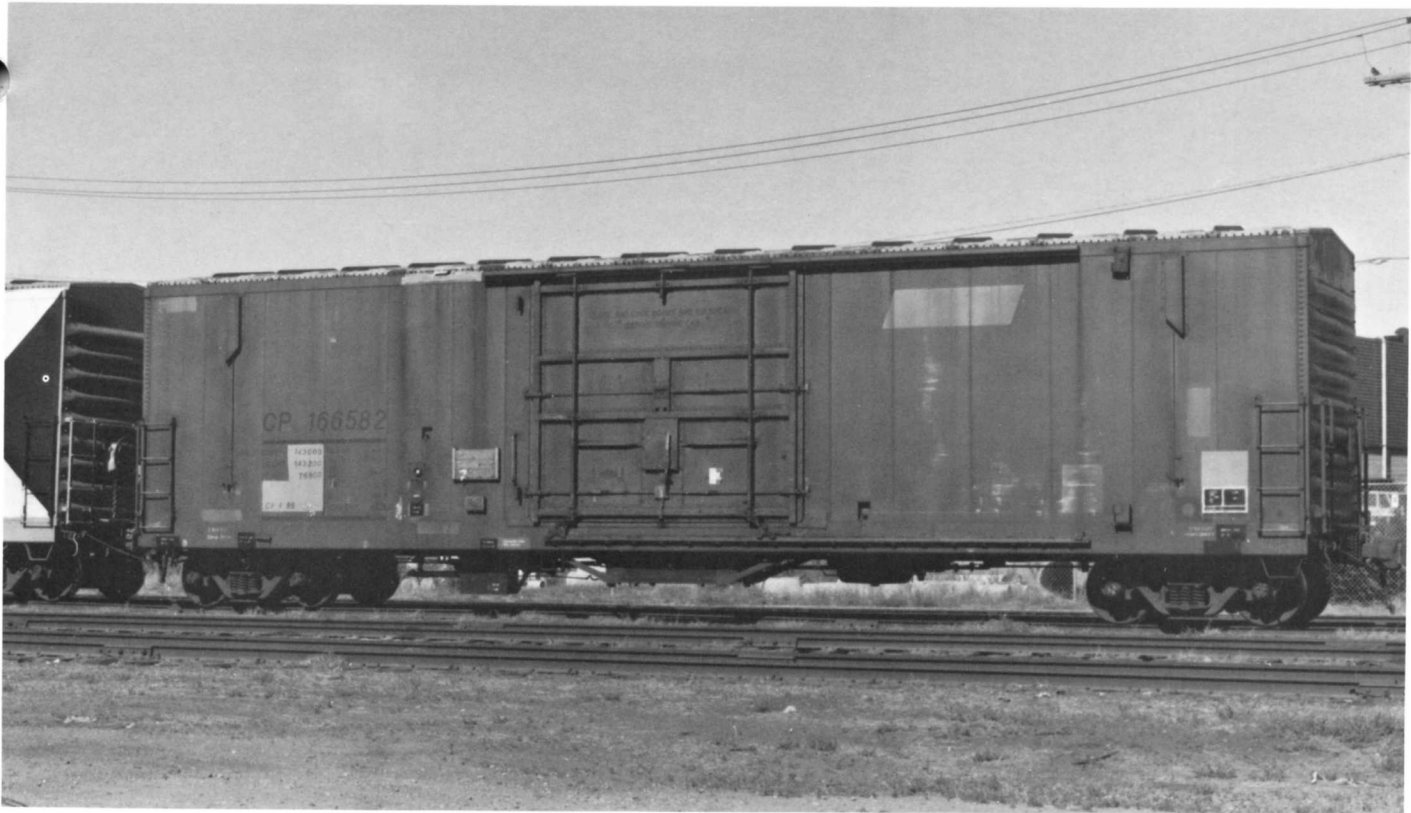
CP 166582. Built 3-72 by National Steel Car. AAR class XLI. 50'7" IL. Plate C. June 19, 1988.
