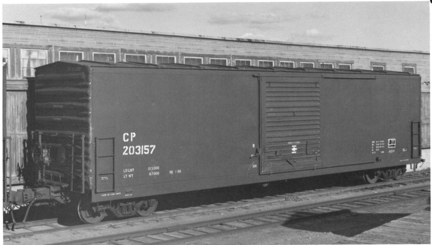
CP 203157. AAR class XL. 50'9" IL. Series 203000-203179. Built in 1971 by the Reading. Ex-RDG class XLj acquired in January 1988. July 19, 1988.
