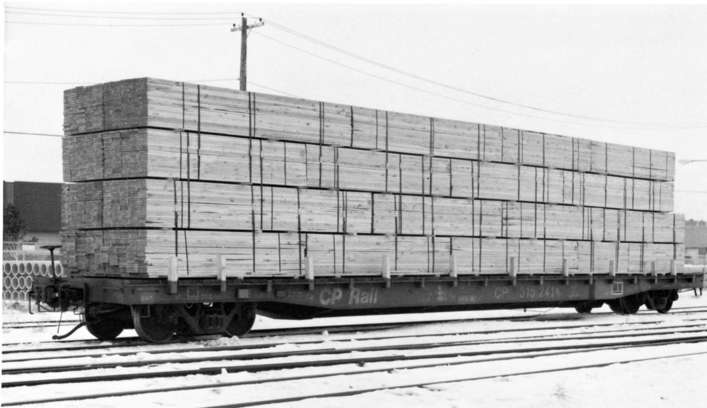
CP 315241. Built 11-74 by Marine Industries. AAR class FM. 65'0" IL. Series: CP 315200-315299. January 31, 1987.
