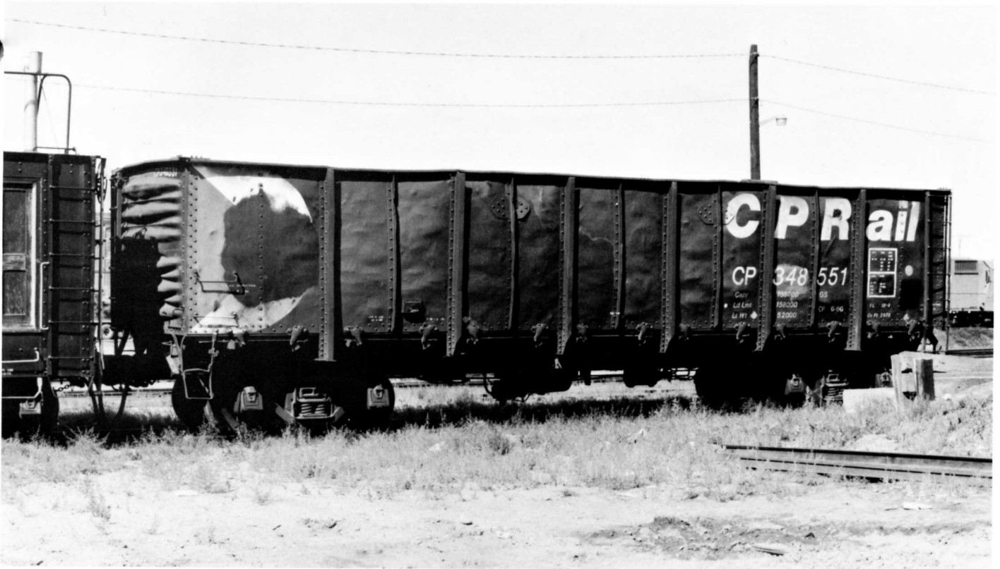
CP 348551. Built 10-48 by ECC. AAR class GS for coal. Series: 348000-348849. Regina, SASK. July 25, 1987.
