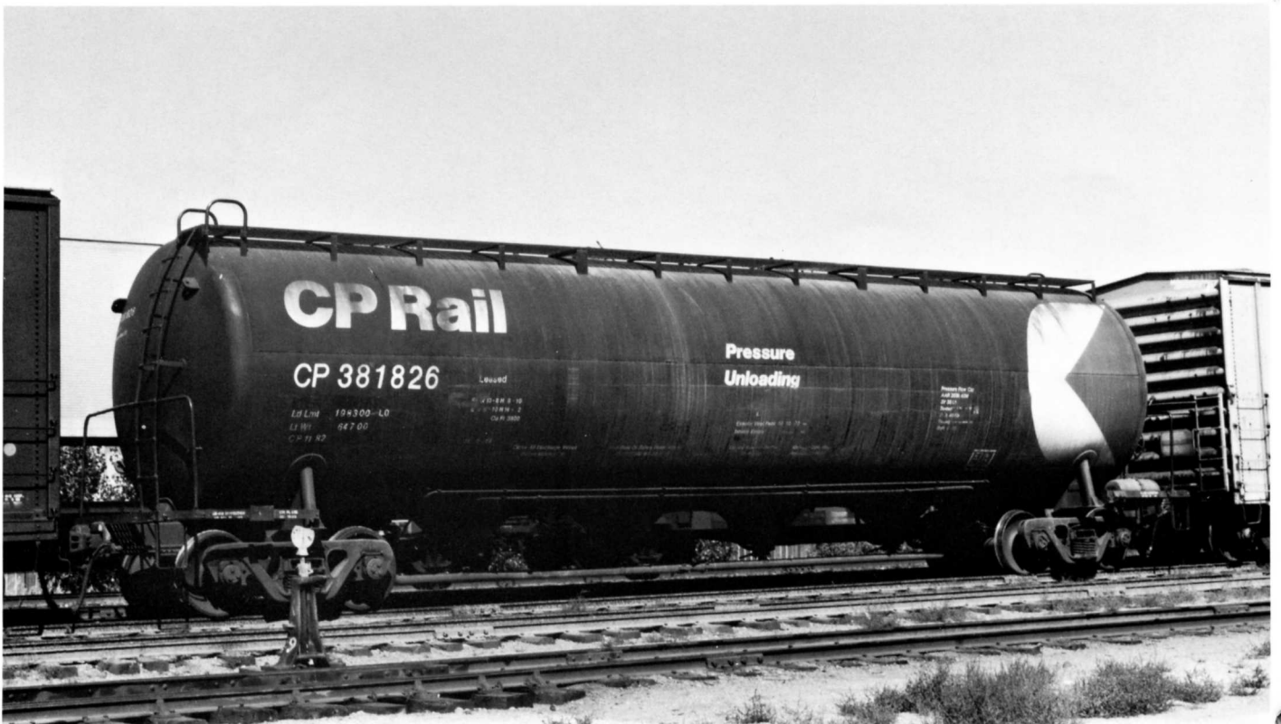
CP 381826. Built 6-69. AAR class LO. Pressure unloading. Sept. 1, 1990.
