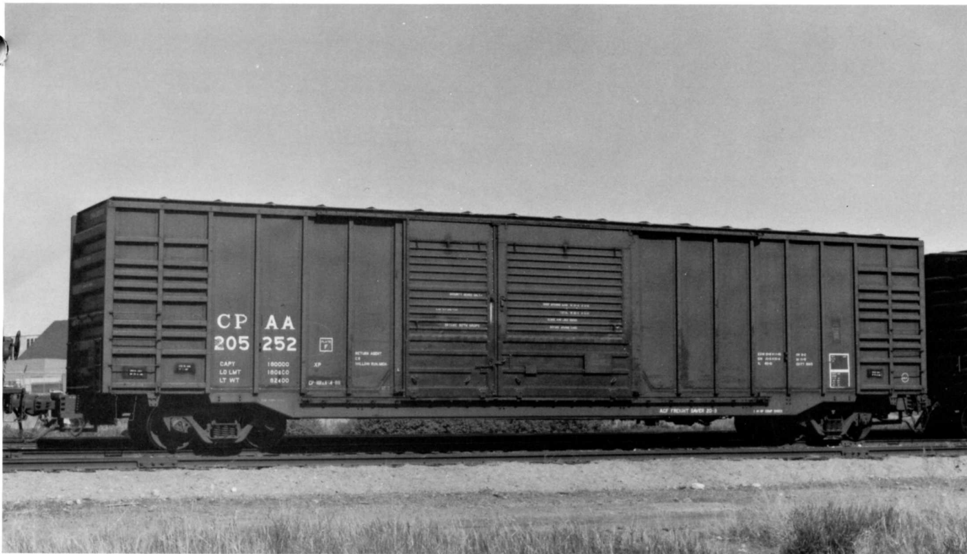
CPAA 205252. Built 3-77 by AC&F. Ex-Conrail. AAR class XP for auto parts. 60'9" IL. May 28, 1988.
