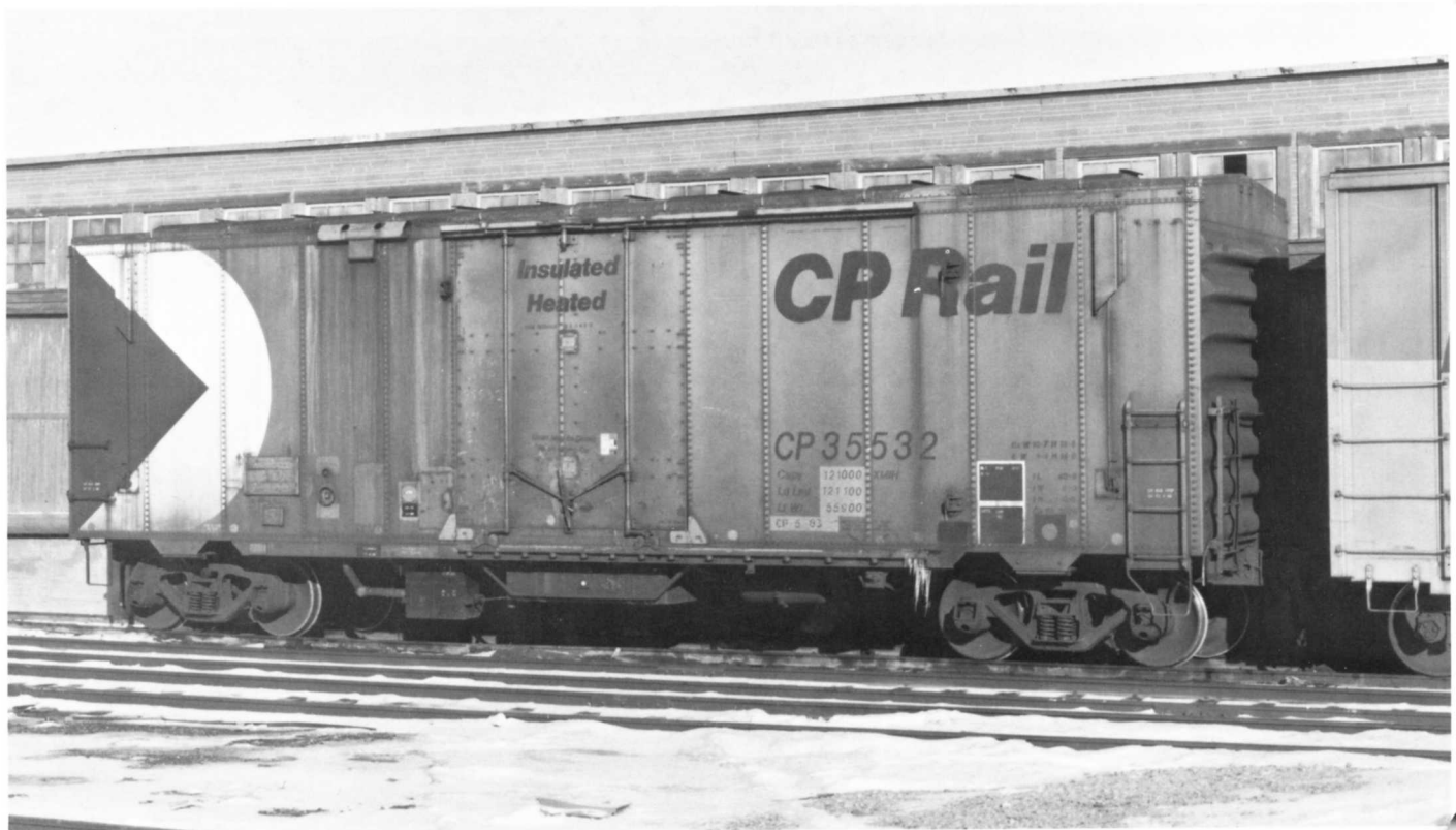
CP 35532. Built 10-61 by Eastern Car. AAR class XMI. 40'6" IL. Series: CP 35501-35800. March 8, 1987.
