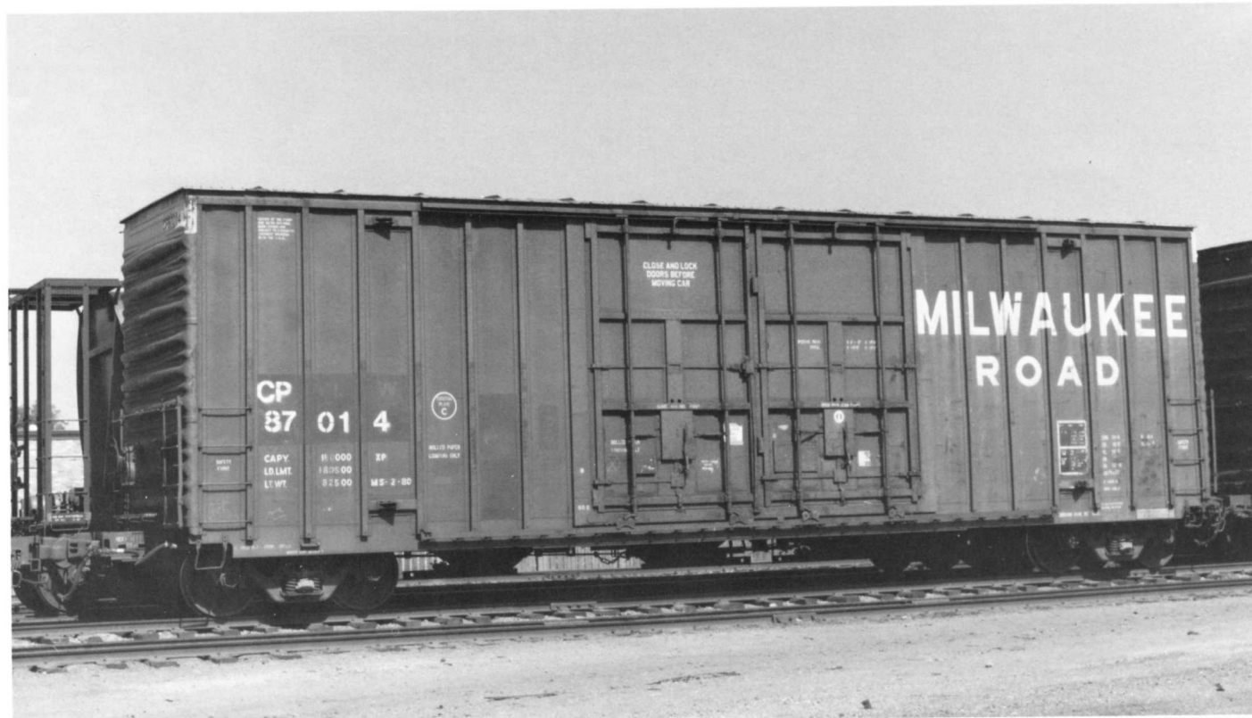
CP 87014. Built 7-72. AAR class XP. 50'6" IL. Clearance plate F. Series CP 87000-87024. May 28, 1988.
