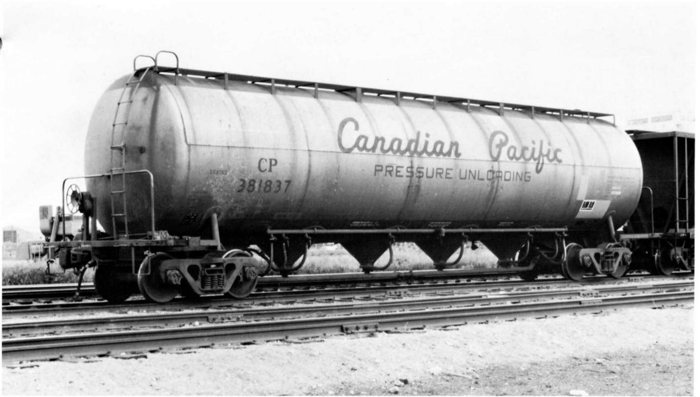
CP 381837. Built 6-69. AAR class LO. Pressure unloading. July 11, 1987.
