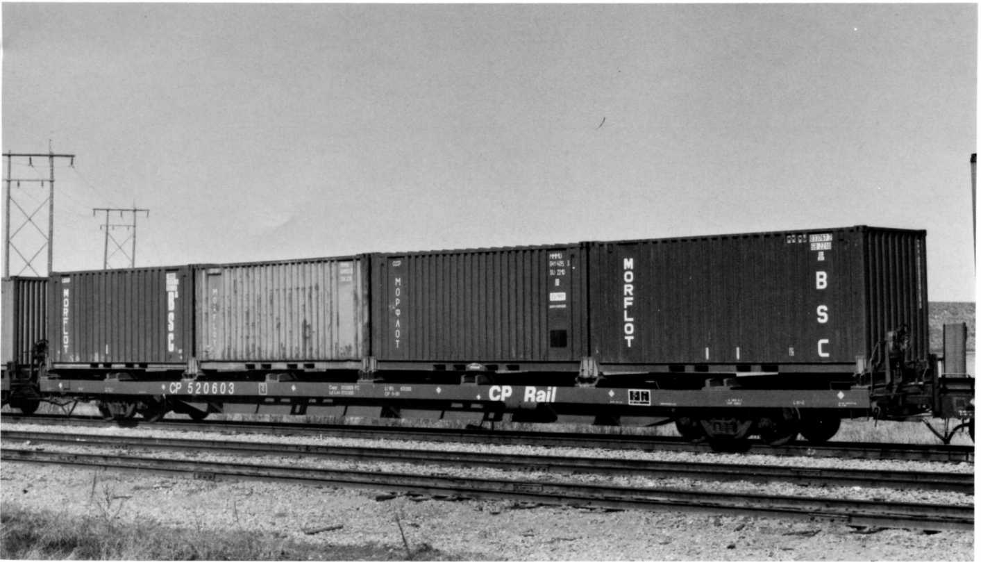
CP 520603. AAR class FC. Container flat car. Series: CP 520550-520649. 81'2" IL. April 4, 1987.
