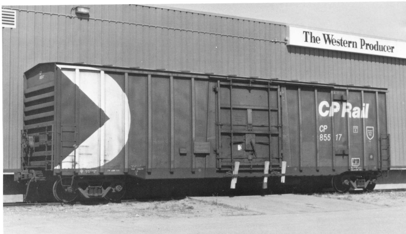
CP 85517. Built 4-75 by National Steel Car. AAR class XP. 50'6" IL. Plate C. Capacity: 5111 cu.ft. Series CP 85500-85634. May 29, 1988.
