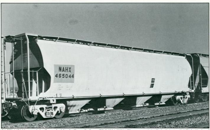
NAHX 465044 was originally marked for the Trona Railway (TRC 1226-1350). They were originally built in April 1979 by National Steel Car. Series NAHX 465000-465124. NSC 4650-cuft design.
