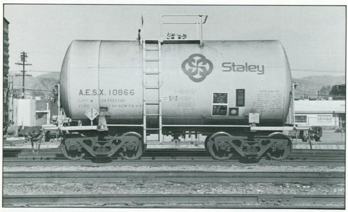
AESX 10866 was built in September 1977 for operator A.E. Staley. It is used for corn syrup transport to customers not needing large quantities.
