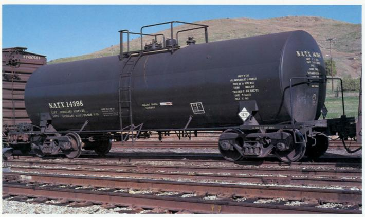
NATX 14398 was one of the last tank cars to come off the Texarkana assembly lines. Shown here on December 25, 1984 in San Luis Obispo, CA. It was built in May 1983 and is leased to Allied Chemical. It is a 100-ton, insulated, coiled, tank car. Pat Holden photo.
