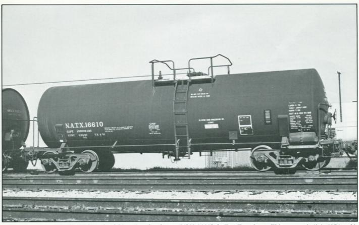
NATX 16610 shows the offset inlet style of this series of tank cars (16210-16665) built at Texarkana. This car was built in 1976 and is leased to Clinton Corn Processing Co. for corn syrup transport.
