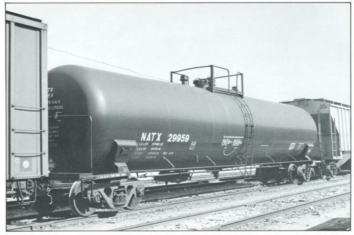
NATX 29959 was built in June 1969. It is a non-insulated, uncoiled, 100-ton, 30,000-gallon, general-service tank car.
