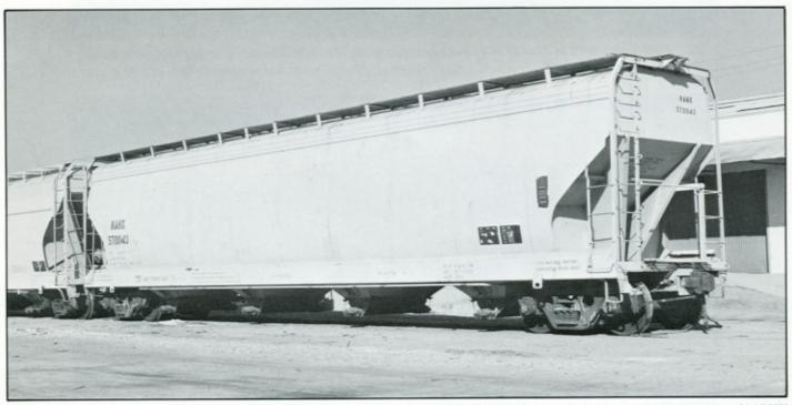
NAHX 570043 is an ACF 5701-cuft design (stencilled 5700) covered hopper. This one was built in February 1977 as part of MOHX 5750-5797. The cars were acquired by GERSCO in 1987. Series is NAHX 570000-570044.
