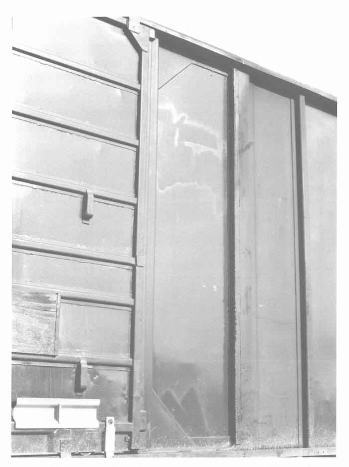
Close-up of the fill-in area to the right of the door. Note the angles at the top and bottom (reminds me of ACF's next-to-door panels).
