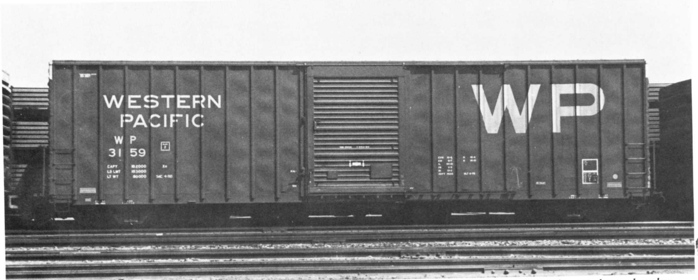
This large high cube box car, in series 3151-3167, was assigned to the GE appliance pool. This type of box car was designed to carry large volume low weight items.
