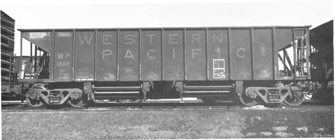
Darby Corp built 50 100 ton hoppers with selective ballast gates, used by WP in general service.
