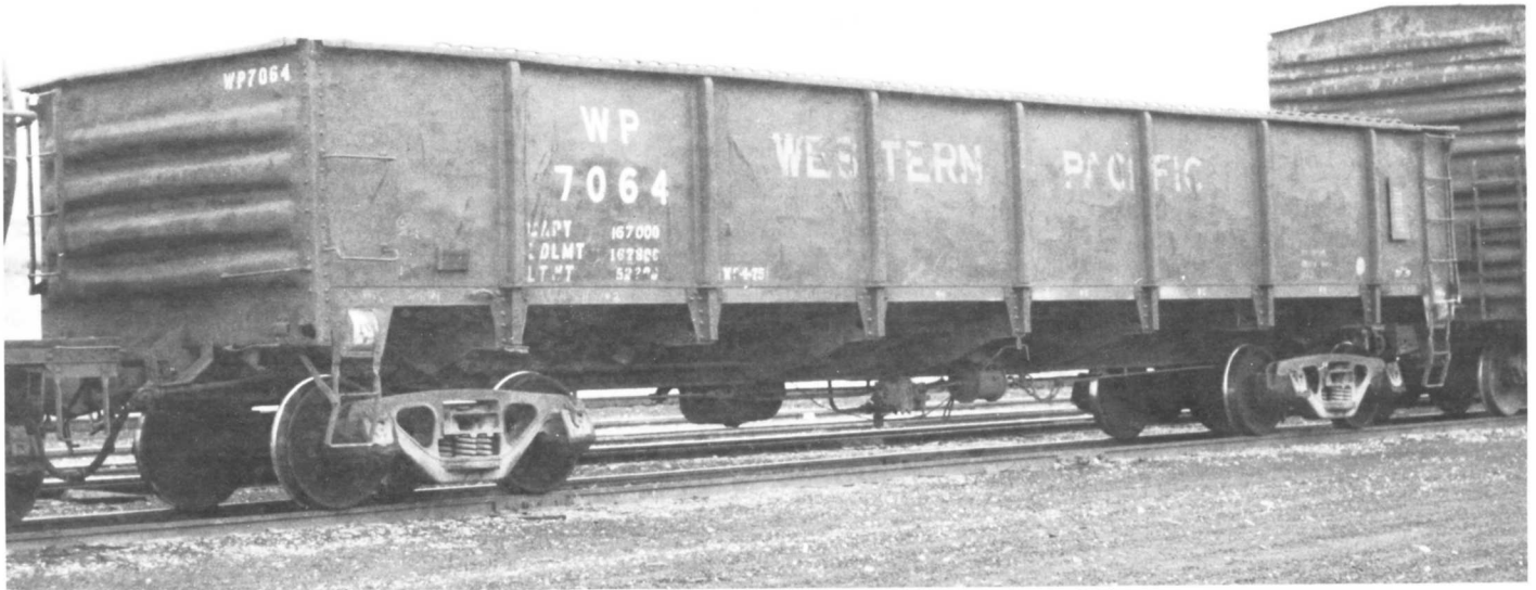
7064 was built by Pullman as a drop bottom GP gon and converted by WP into a solid bottom gon.
