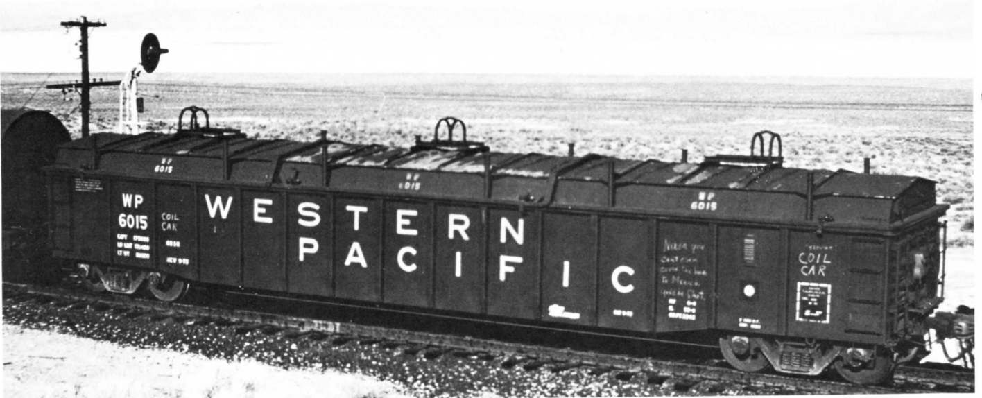
WP 6015 is one of 4 classes of covered gons used to transport coiled steel. The covered series were used for special shipments that needed weather protection.
