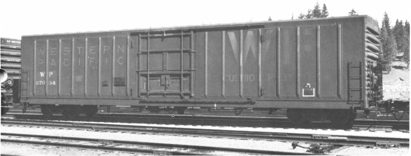
WP 67014 is one car in 4 classes of insulated 60' box cars assigned to COORS.
