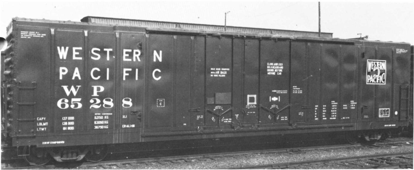
65288, a canned goods car, with dual air pak air bags at each end of the car to hold load tightly in place. This car has a one of a kind painted scheme applied in 1981.
