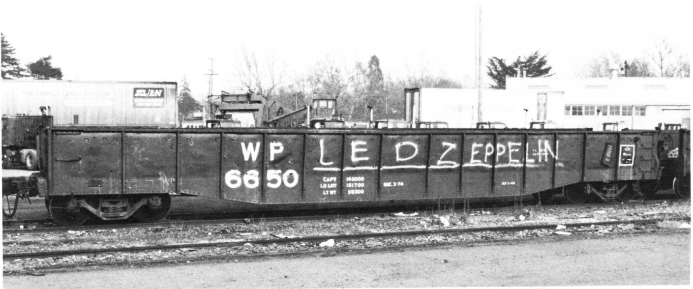
Three classes of 52' drop end gondolas from 3 builders totaling 325 cars, with only 144 left in 1983.
