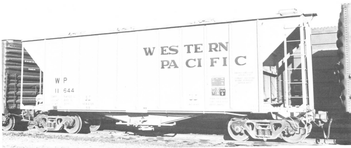
WP's fleet of General American Built Airslide® covered hoppers are used primarily for flour service.
