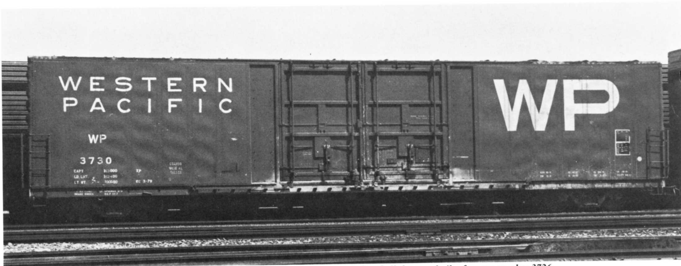
This style of 60' auto parts car built by Thrall is symbolic of all the cars built after car number 3726.
