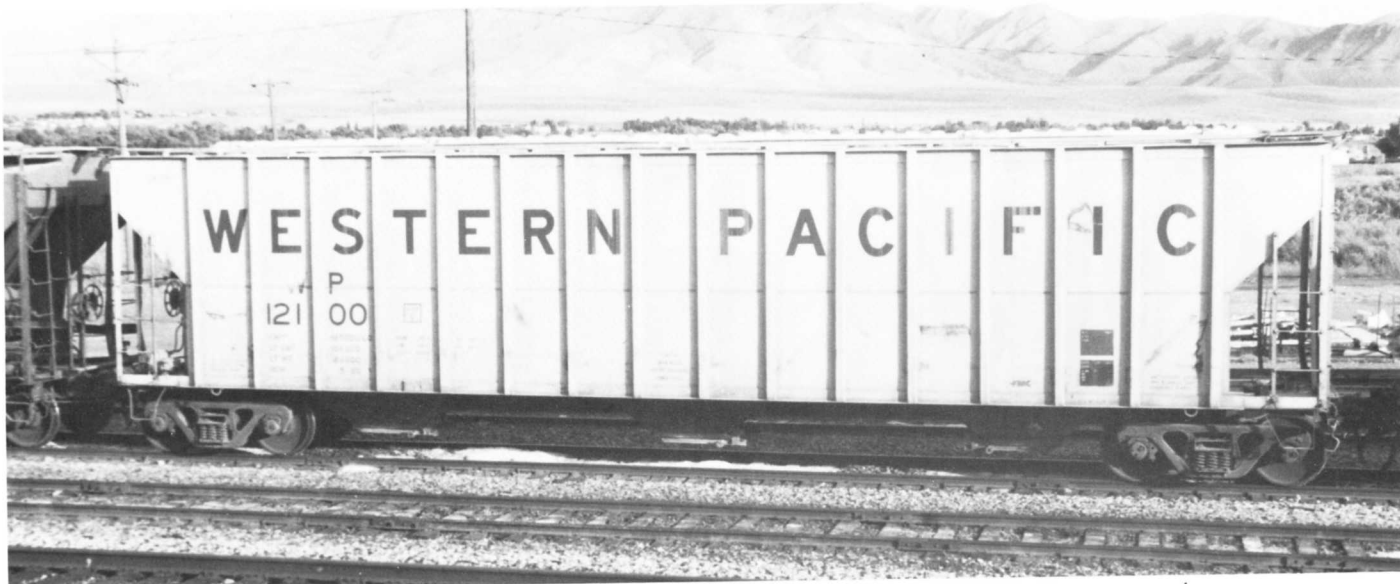
WP 12100 the last covered hopper, shown here in Winnemucca, NV., was built by FMC and used in gypsum service.
