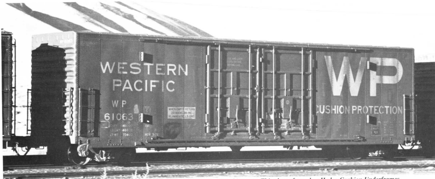
61063 is a double insulated box car used for temperature sensitive shipments. This class of cars has Hydro-Cushion Underframes.
