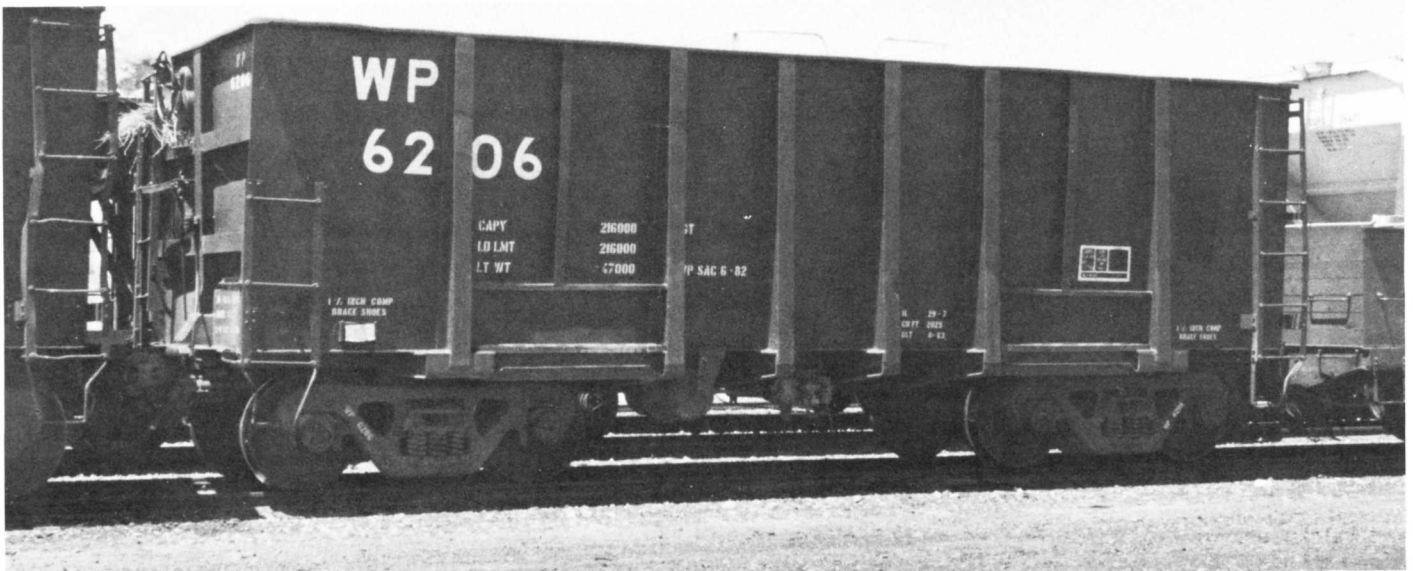
6206 was rebuilt in Sacramento 6-82 and repainted gloss black using the simplified lettering scheme. 10 of these cars were purchased by WP from the Oroville Dam Contractors after that large Northern California earthen Dam was completed.
