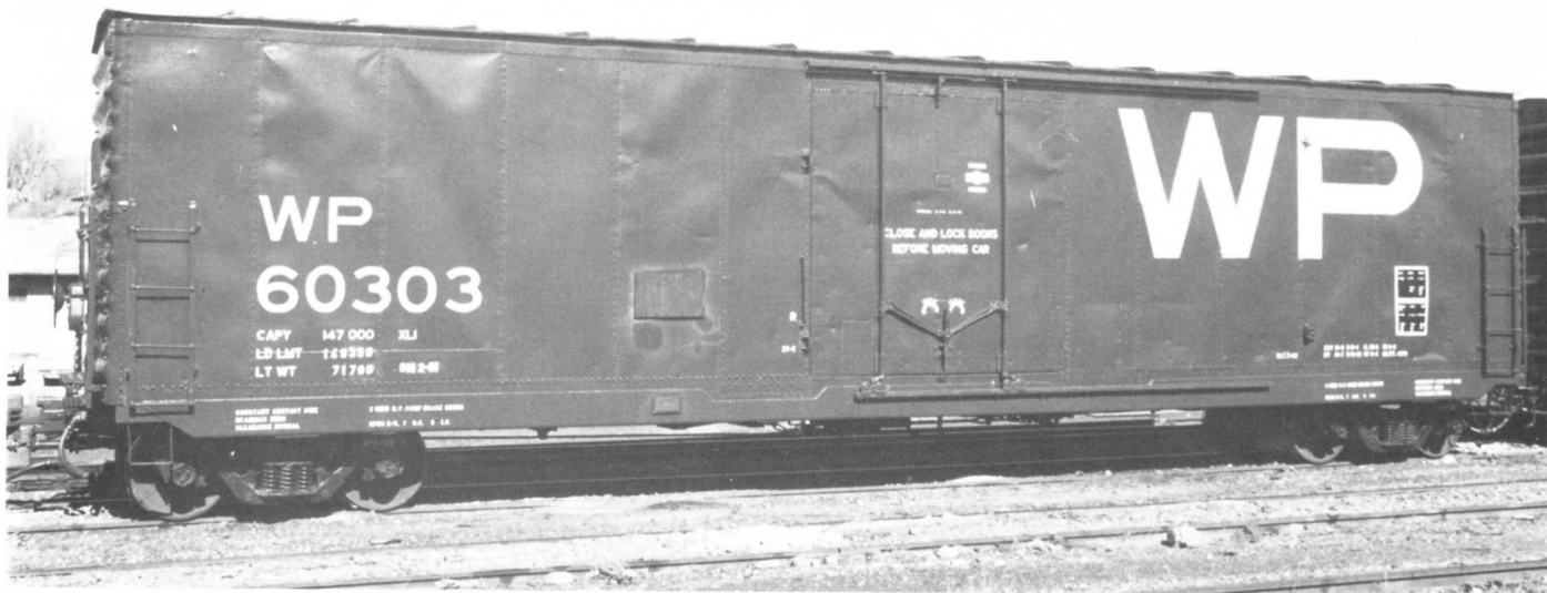
WP 60303 a rehabed, renumbered 60132 series, from RBL to XLI cars. Repainted at the same time into the simplified paint scheme.
