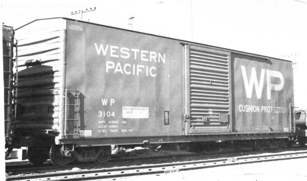
This 50' high cube box car in series 3101-3105 was assigned to paper service.
