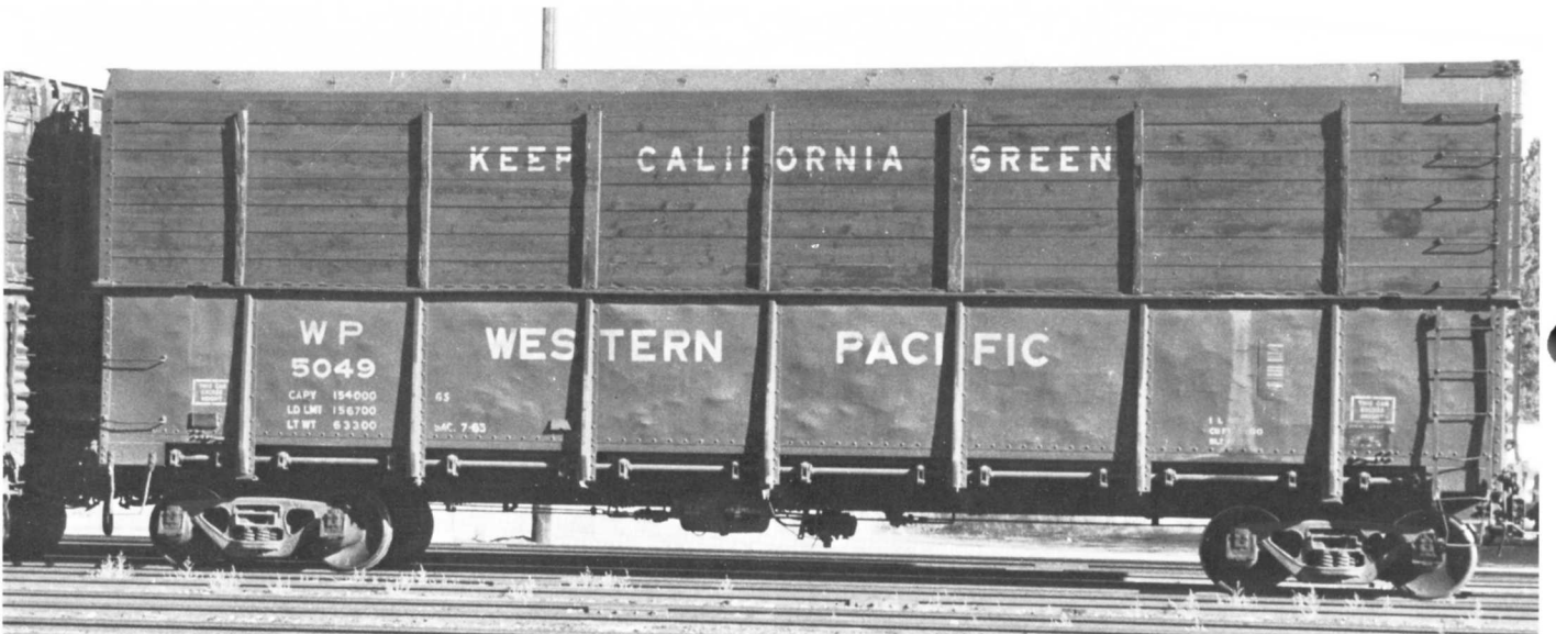
WP 5049 is one of WP's "Keep California Green" wood chip cars. WP built these wooden racks after SP's beet gons.
