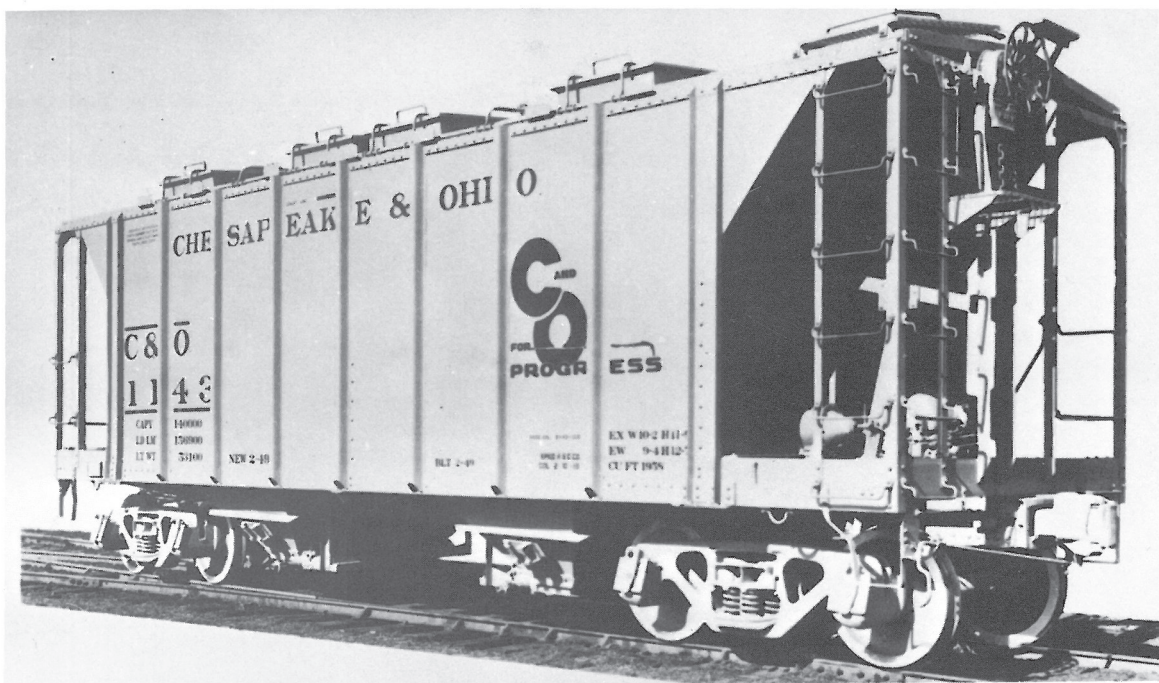
C&O 1143. Ralston Steel Car's version of the twin bay of the era. This photo is a little out of focus on the right side but most of the features are clear enough to define.
