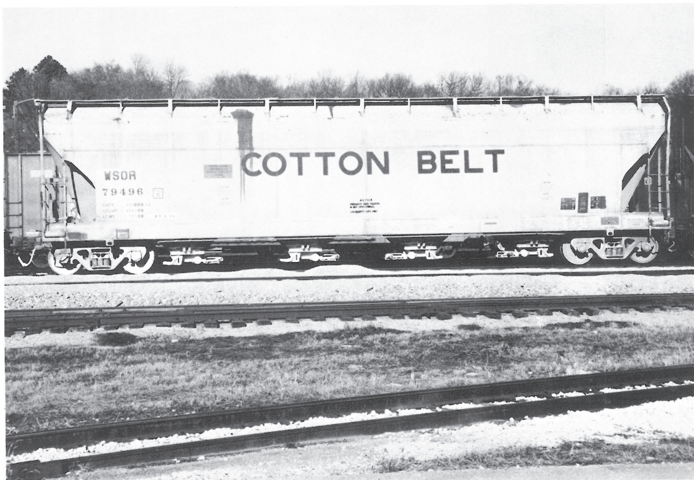
WSOR 79496. Wisconsin & Southern acquired a number of former SSW/SP covered hoppers without renumbering. The stencil under the "ON" in "Cotton Belt" says "Notice pneumatic gate feature is not operational use gravity gate only." (M.B. Foley photo)
