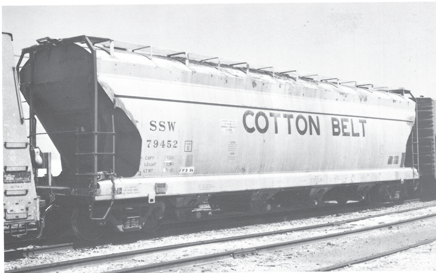
SSW 79452. Four bay ACF built "Center Flow." Note the pneumatic and gravity outlets.
