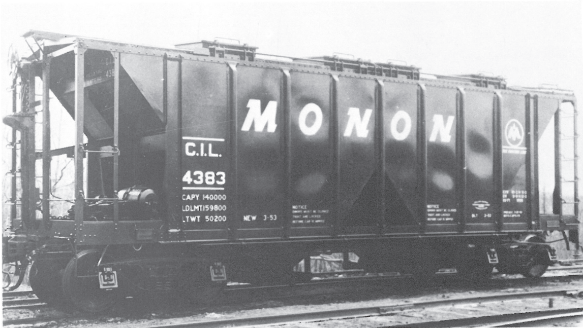
C.I.L. 4383. Series 4201-4390. Built by Pullman-Standard in 1953. A later built car than the CGW car. Note it still retains the welded side plates and this car does not have rivets on the first panel along the side sill.
