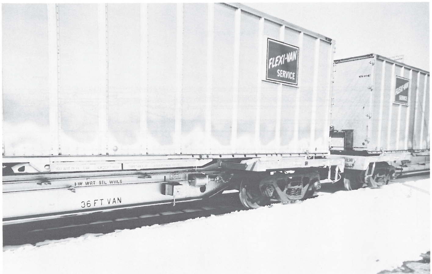
MILW 58020. The remaining brake rig detail is shown in this view of #58020. The box just to the left of the brake valve is the electrical plug-in that operated the hydraulic ram. The safety chain-down feature is also noticable. This would keep the trailer parallel with the flat car in case the turntable failed. (Milwaukee Road photo; Richard Yaremko Collection)
