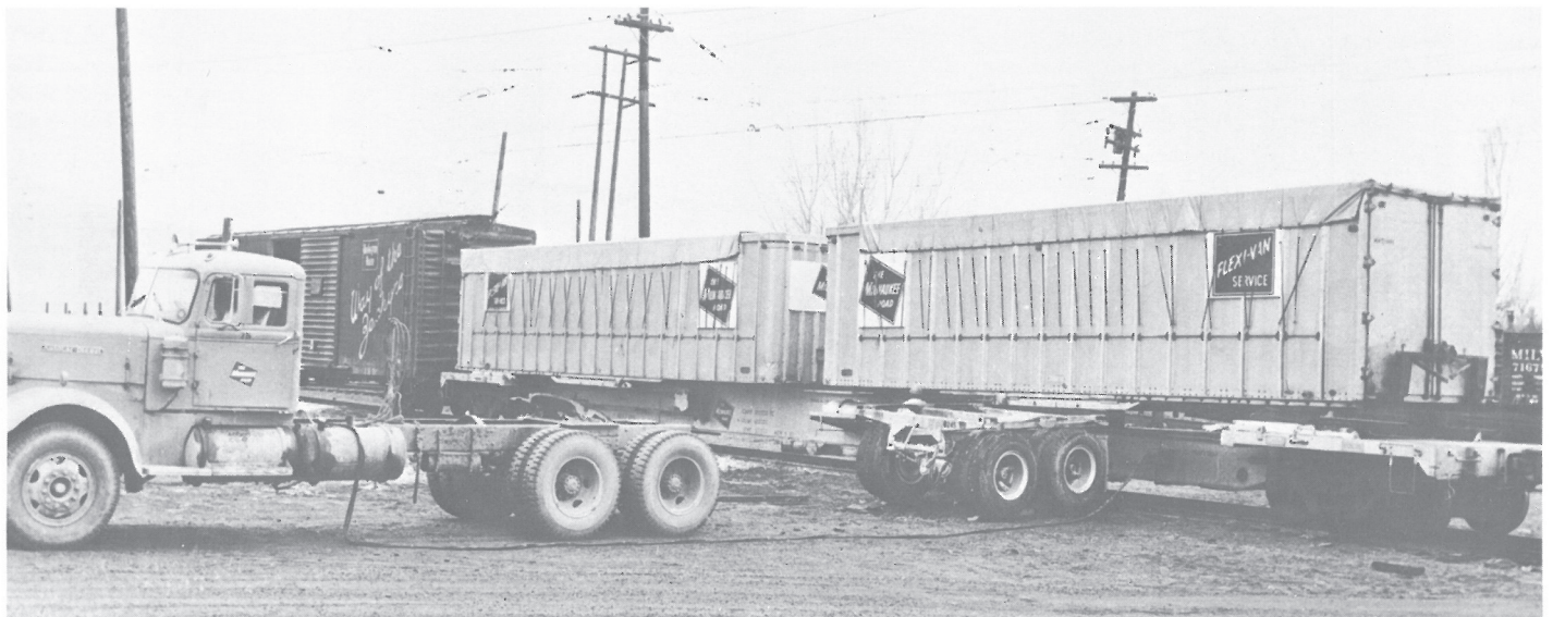
MILW Autocar Truck. This photo taken at Beverly, Washington shows two of the open top vans riding a Mark II flat. The "Ambiblical" cord which makes the whole thing work is plainly visible. We can presume that the cord traveled with the flat car in the box that is barely visible under the far trailer. The Autocar truck, painted solid orange is the only item easily modeled as it was offered as an HO scale kit, first by Lee Town and now by Alloy Forms. the flat and the vans will have to be scratch built. (Milwaukee Road photo; Richard Yaremko Collection)
