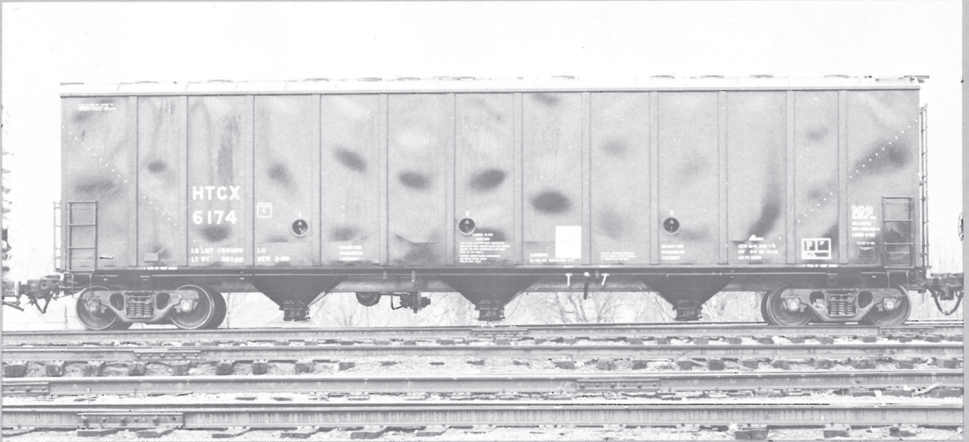
HTCX 6174 is a new carbon black covered hopper built in 3-89 by Thrall Car's Chicago Heights plant. (Dwight Jones)
