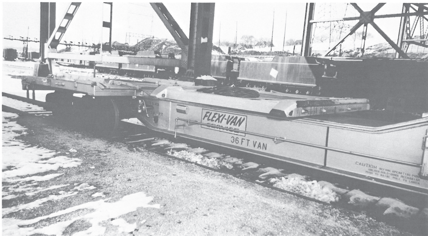
An empty Mark I flat with the turntable ready to accept a trailer. The brake wheel, also visible, was able to slide down until it was flush with the end sill. (Milwaukee Road photo; Richard Yaremko Collection)
