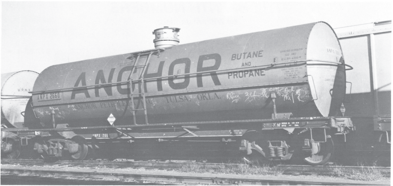
ANPX 2660. Anchor Petroleum Co. This car was built in April 1948 by ACF. Again it is a 50-ton, insulated, class 105A300W, 11,000 gallon LPG tank car. Compare the tank supports of this car to other ACF built car illustrated in this photo-essay. This may be an older type with a lack of the thin angle piece on the top of the support where it meets the tank. Photo c.1949.
