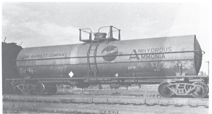
BMX 10083. The Barrett Company (later became a division of Allied Chemical) was built in July 1940 by General American Transportation. This particular car was assigned to Anhydrous Ammonia transport. Note the "full" platform which was not always present on all LPG/AA tank cars. Aluminum tank, black data and red emblem.
