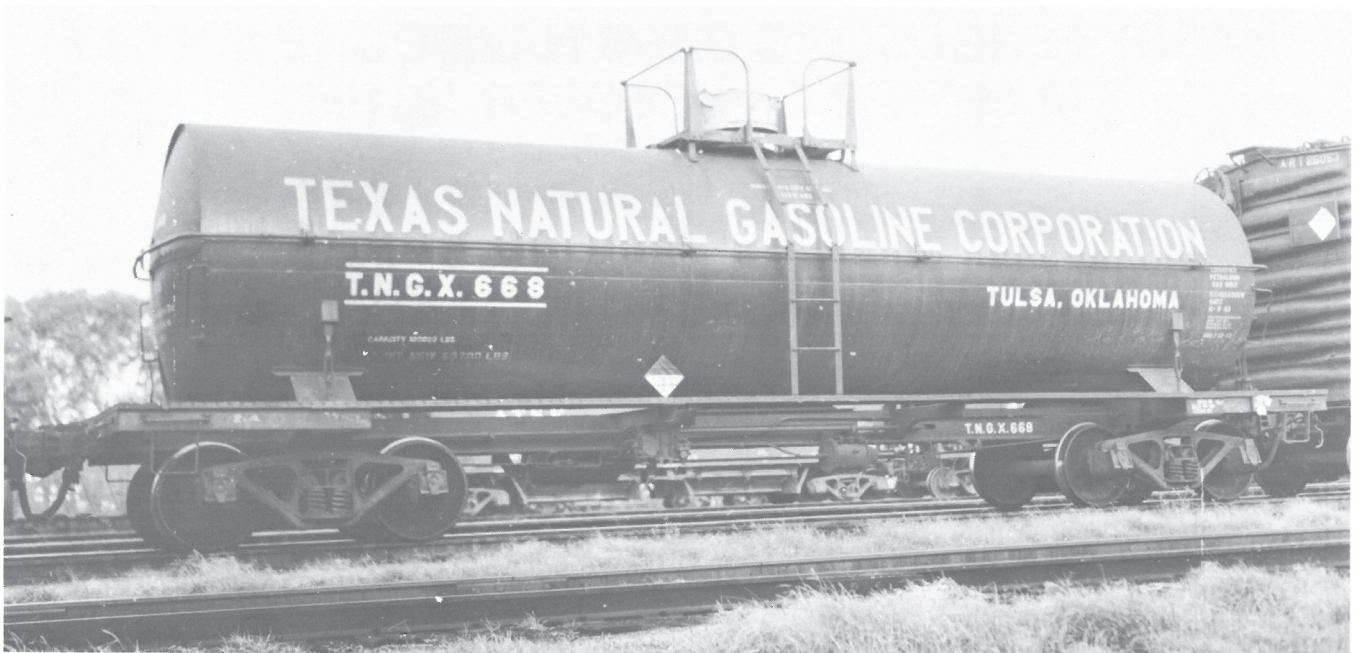
TNGX 668. This car was built in October 1953 by General American. Dual service LPG/AA tank cars. This tank is essentially very similar to TNGX 1076. However note the difference in ladders, "side sills", brake cylinder etc.
