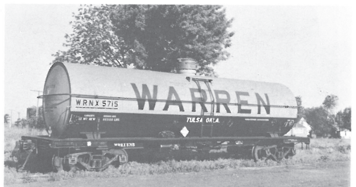
WRNX 5715. Warren Petroleum Corp. The back of the photo says it was built in March 1949. It was built by ACF as one can tell by their location and type of logo present on the center sill on the right side.
