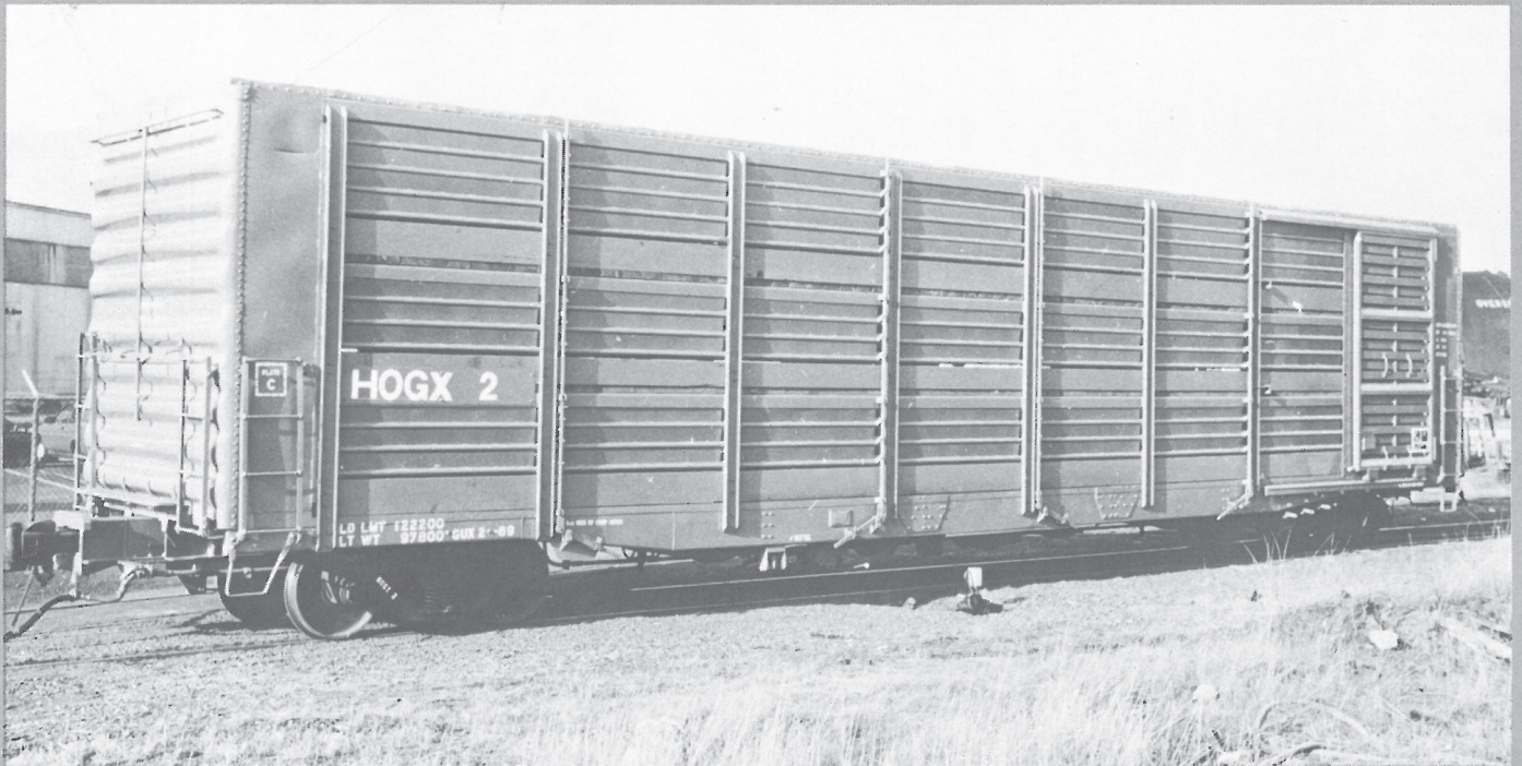
HOGX 2 was built in 1965 by Pullman-Standard and recently converted in 2-89 by Gunderson to this 60-foot stock car operated by Farmer John. Colors are green body with yellow lettering. (Ken Ardinger)
