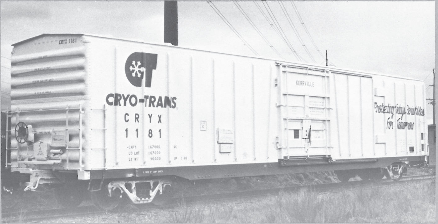
CRYX 1181 is part of the latest group of converted ATSF class Bx-131 XLI's to CO-2 refrigeration. The new series has a new slogan on the right "Protecting Today's Perishables For Tomorrow". (Ken Ardinger)
