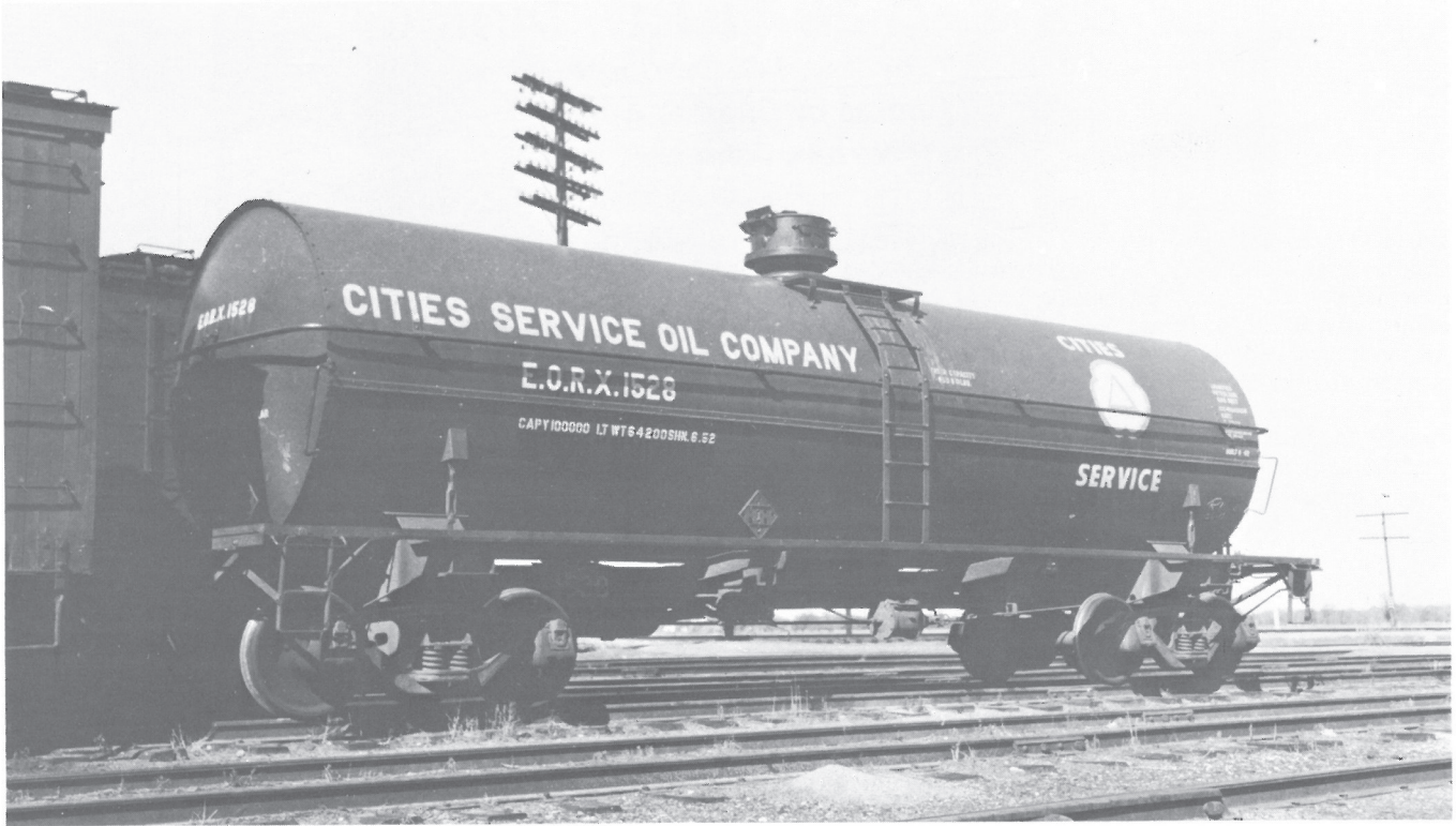
EORX 1528. EORX is one of the two reporting marks being used by Cities Service Oil Company in 1952 when this car was delivered by General American's Sharon, PA plant (see the abbreviation "SHN" and the date "6-52" which matches the "built" date of the car . . . this indicates it was built at Sharon; a practice that GATX Sharon continued until the plant closed in 1984). This 50-ton car is used for LPG and is black with white data and a green and white emblem.
