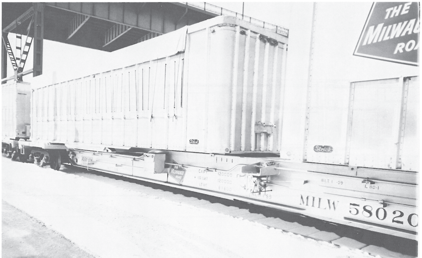
MILW 58020. This view highlights the brake rigging detail. Also note the tarpaulin tie down system on an open top van. These vans were frequently used for hauling pipe and other shipments that arrived by steamship and could be dropped into the waiting container. These early trailers also carried an older Strick logo. (Milwaukee Road photo; Richard Yaremko Collection)
