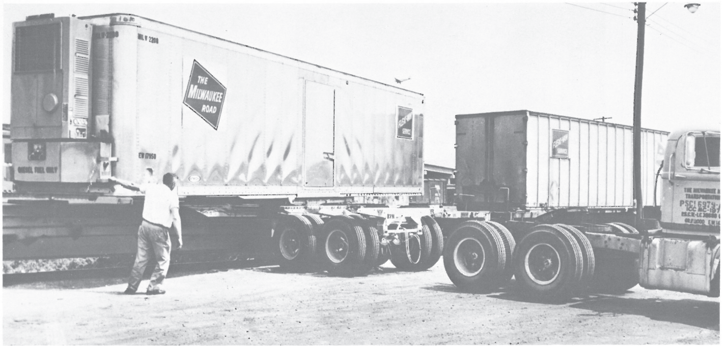
MILW Trailer 2208. Here a driver prepares to swing this refrigerated trailer over the bogies and off load the flat. Van 2208 is 39 feet in length with a diesel powered Thermo King refrigeration unit. (Milwaukee Road photo; Richard Yaremko Collection)
