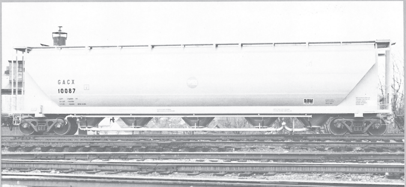
GACX 10087 was built in 12-88 and is part of a second batch of fifty cars being delivered to General American Transportation by Trinity. This is the new "Power Flo" design, a pressure differential covered hopper that appears to have been designed by Trinity despite similarities to the North American Car designs. (Dwight Jones)
