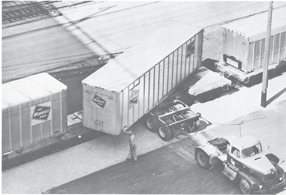
A hydraulic lift, powered by the cab unit's battery, raises the van free of the "bogie", or rear wheel and axle assembly, from which position it can be easily swung into place on the car, as demonstrated here by the driver. With the two vans locked securely in position on the flatcar, they are ready for fast rail movement to destination. The "bogie" from which the van was removed stands beside the car, ready to be taken away for picking up and delivering other vans from incoming trains. (Milwaukee Road photo; Ernest Lehmann Collection)
