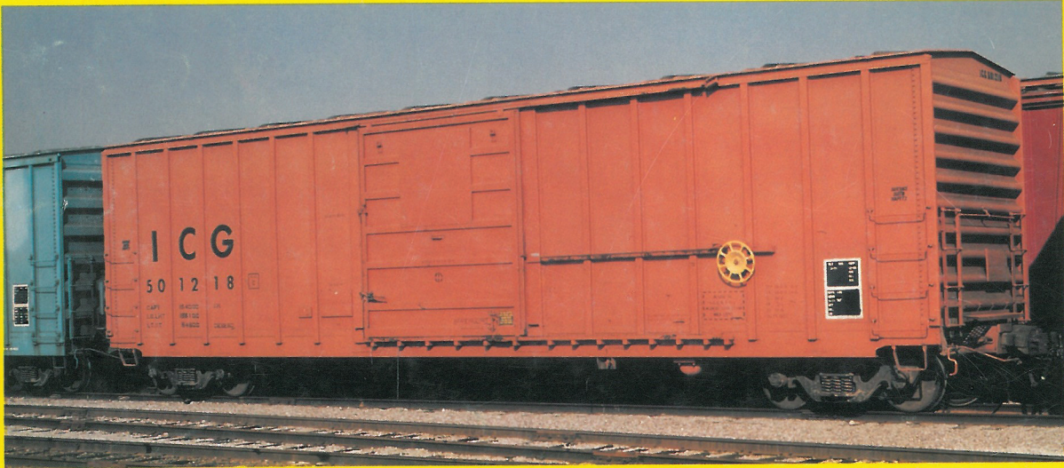
TYPE V. ICG 501218. Painted "CE 12.80". This is an ex NRUC road car built by Berwick. Note the location of the "when empty box" and the door assist wheel. (D. G. Casdorff)
