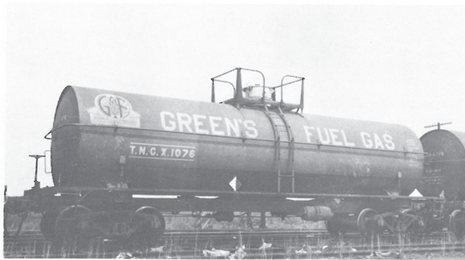
TNGX 1076. Cars in the general series TNGX 601-1100 were used in dual service for LPG and AA transport. This car appears to have been built in 12-55 by General American. These are "typical" LPG cars of the period — ICC 105A300W, 11,000 gallon insulated tank cars.
