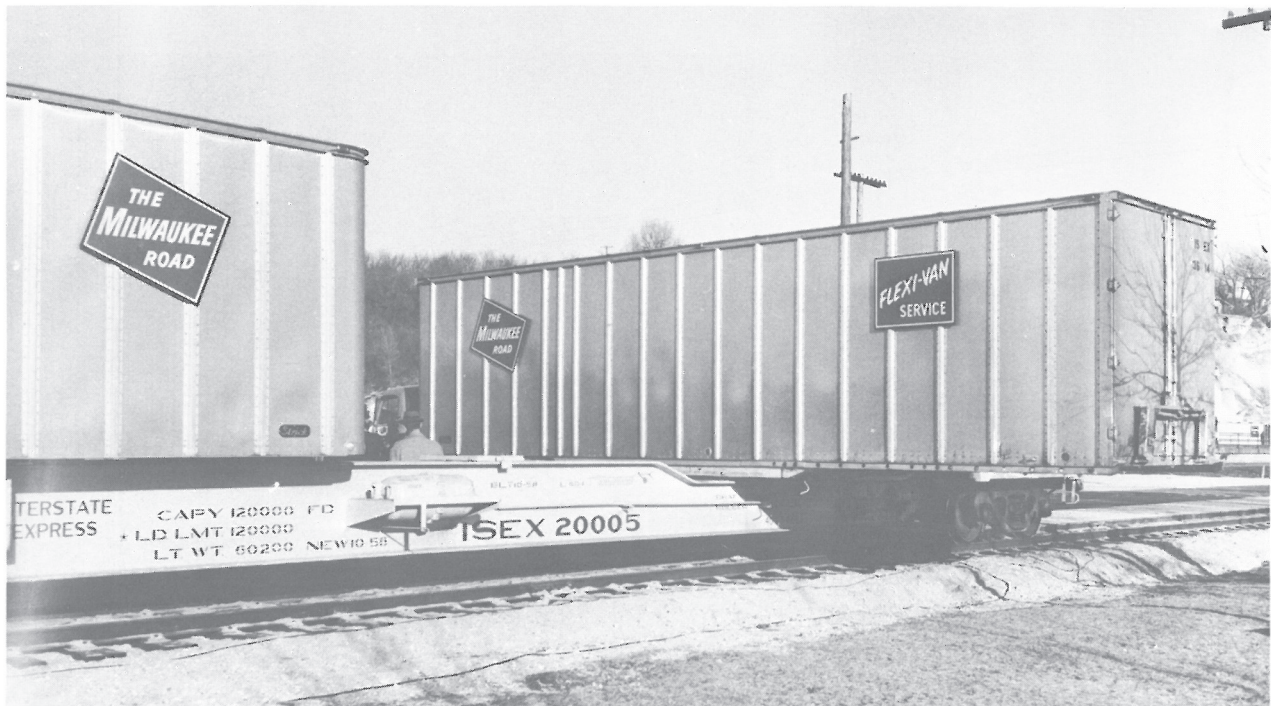
ISEX 20005. Interstate Express was running FLEXI-VAN in October 1958 several months before the MILWAUKEE obtained their first flat cars. Note that while the trailers have Milwaukee Road logos the van is numbered ISEX 3614. (Editor's note: The Official Railway Equipment Registers for July 1958 and April 1959 do not show any listing for ISEX or Interstate Express — anybody have any more information on these cars?) (Milwaukee Road photo; Ernest Lehmann Collection)
