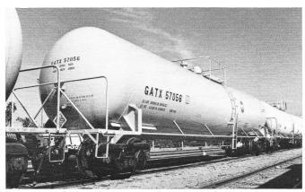
GATX 57056 is part of a new series of 26,500 gallon tank cars being leased by Dow Chemical. This car was built by Trinity in 9-88. The non insulated cars are being used for Aromatic hydrocarbon and styrene service. (David G. Casdorph)
