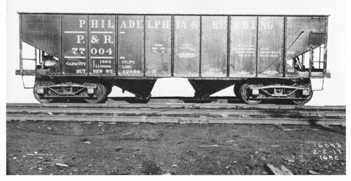
P&R 77004 is part of a series of 500 twin bay open hoppers built by the Standard Steel Car Co. 1916-1917. Note the 9 post construction of this car versus the 7 posts on the later Ralston Steel built car (see P&R 73790).
