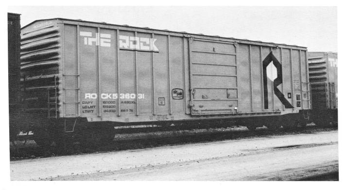
ROCK 536031, makes a good prototype for the recently released McKean 50-foot outside braced ACF boxcar model in H.O. scale. The car comes from a series originally built in 1972 by ACF STL as RI 36000-36299. These were 70-ton loader equipped cars with a cubic foot capacity of 5285. (Pete Arnold photo)
