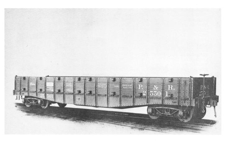
P&R 25501, a 41'10'' composite gondola was built by Standard Steel car in 1909.
