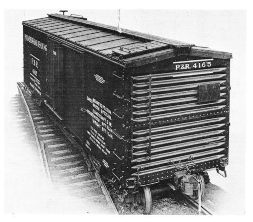
P&R 4165, class XMR was built by Pullman in 1918. Loading length is 36'2'' and loading height is 8'1-1/4''.
