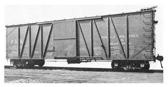
P&R 5539, class XMS was built by Pullman in 1919. The car has a 40'6'' loading length and 9'0'' loading height.
