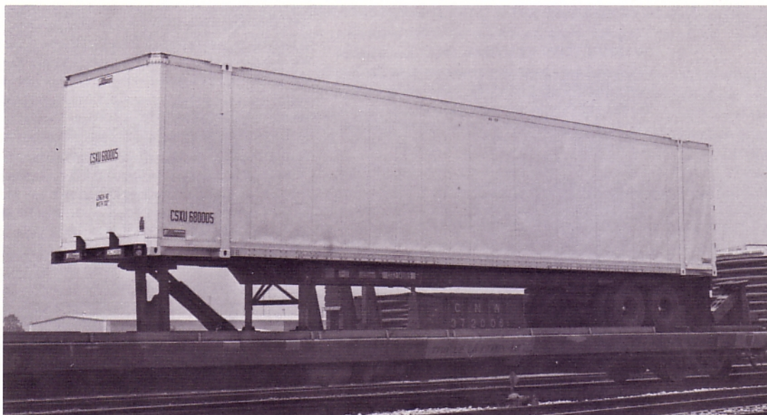
CSXU 680005 is one of the new built 48-foot domestic containers for CSXT. These, like other recent deliveries, were built by Monon. This is the typical livery on this container with no CSXT logos. Note also the CSXZ chassis, also built by Monon. (David G. Casdorph photo)
