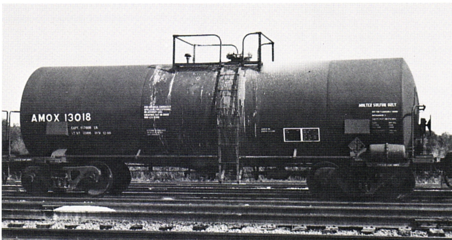
AMOX 13018 is a Trinity designed and built molten sulphur tank car. Typically molten sulphur cars are small 13,500 gallon, coiled and insulated 100-ton tank cars.
