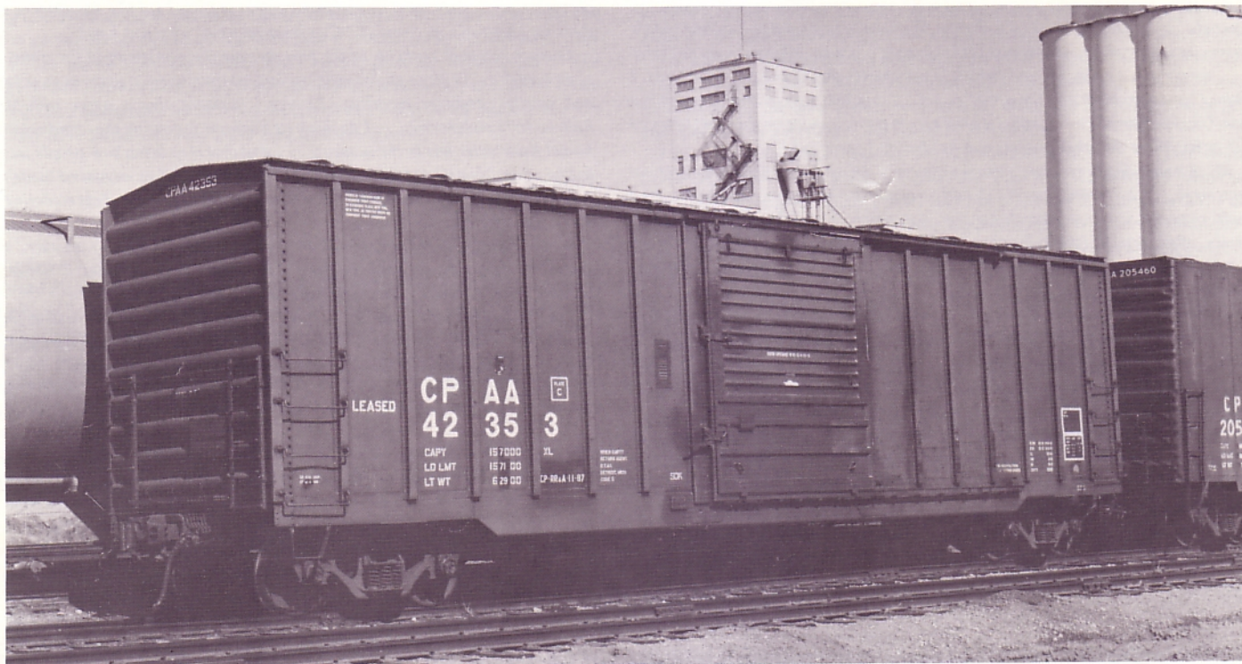
CPAA 42353 is a 70-ton 50'6" loader equipped auto parts boxcar assigned to the DT&I Detroit, Michigan (now GTW). Photographed in Saskatoon April 1988. (Mark Kindrachuk photo)
