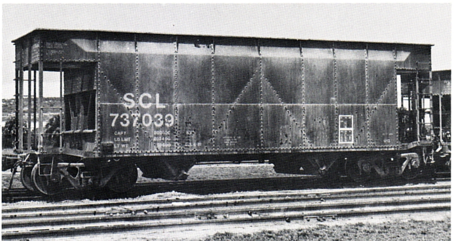
SCL 737039. A wet-rock phosphate hopper. Wet-rock cars are open hoppers. The cars of this series were originally the Atlantic Coast Line 7000-7402 series. Later became SCL 737000-737402 and finally became SBD/CSXT 630480-630850.
