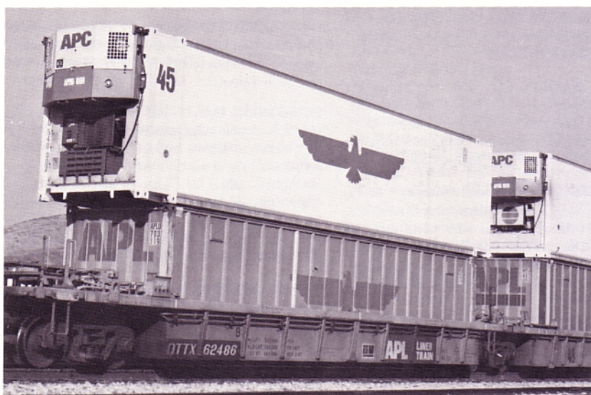
APLU 540007 is a new refrigerated 45-foot domestic container (first 45-foot reefer containers).
