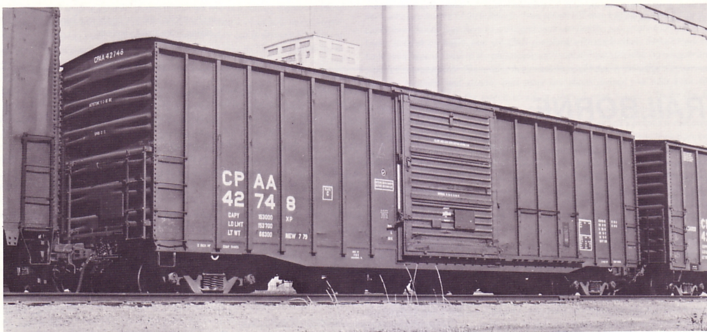
CPAA 42748, another 70-ton 50'6" auto parts boxcar was built by Fruit Growers Express at their Alexandria Shops in 1979. Note the "X" ends on this car. Saskatoon April 1988. (Mark Kindrachuk photo)
