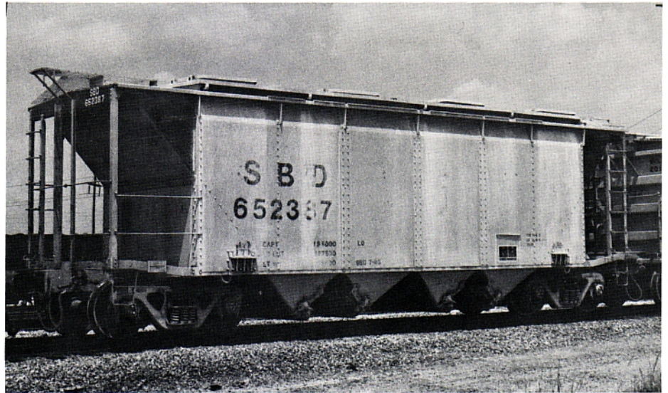
SBD 652387 was originally an Atlantic Coast Line class U-14. This is a covered hopper for the transportation of dry-rock phosphate. Built in 1966 by Bethlehem Steel.
