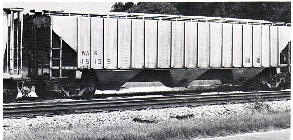
WAR 15135 is a standard sized (4750 cubic foot) modern grain hopper. This one built by Pullman-Standard in 1979.
