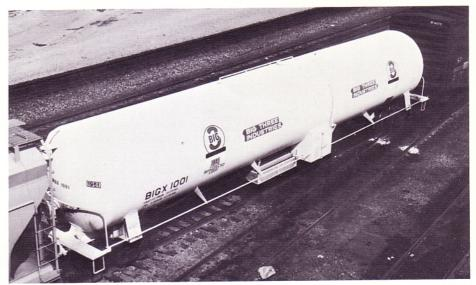
(RIGHT) BIGX 1001. Built in 1-69 has a 25,471 gallon capacity. All of the BIGX cars are used for refrigerated liquid argon. This top view shows the lack of typical tank car inlets. Only a small manway is barely visible near the center of the car on top.
