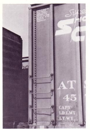
End-to-side joint of the **BFF 6196** design shows the riveted construction. Also note the shape of the posts.
