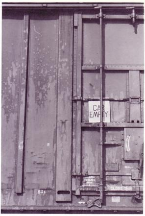
Door post (the post adjacent to the door) of the **BFF** 6196 design. Note the wider design and the oval opening at the bottom.
