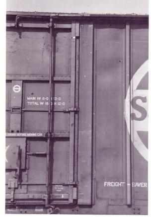
Door post of the **PS 6196** design. Note how it's similar to the other posts on the sides and narrower than the Berwick style.
