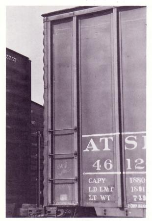
End-to-side joint of the ACF 6100 design showing the welded wrap-around construction. Note the thinner posts and wide flanges on this design versus the other two.
