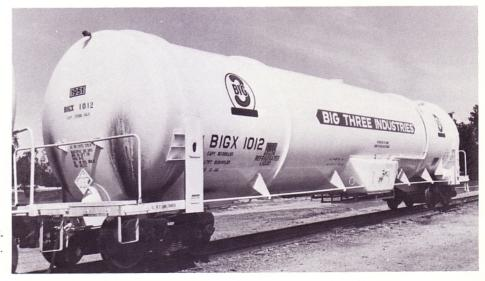
**BIGX 1012-1014.** Built in 11-80 by Process Engineering, Inc. in Plaistow, NH (abbrev: PEI NH). This series has a 25,840 gallon per car capacity.
