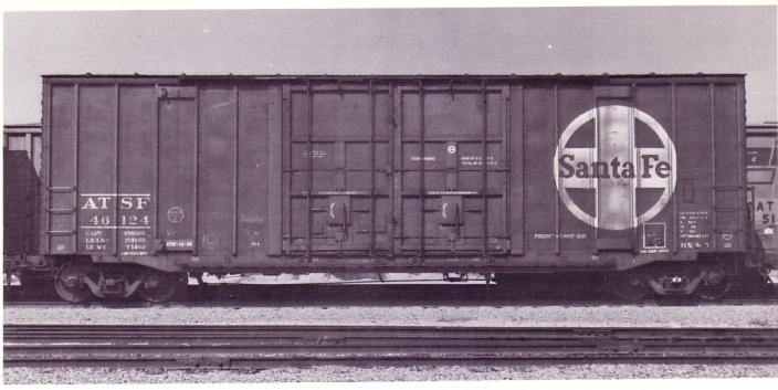
ACF 6100. ATSF 46124 as it appears in its delivery paint scheme. This car - exhibits the 10-post welded construction.
