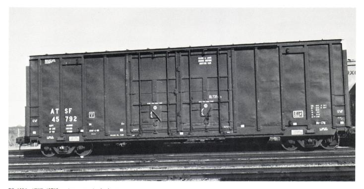
**PS 6196.** ATSF 45792 as it appears in the latest livery. Note the 8-post (referred to in the table under sides) welded construction.
