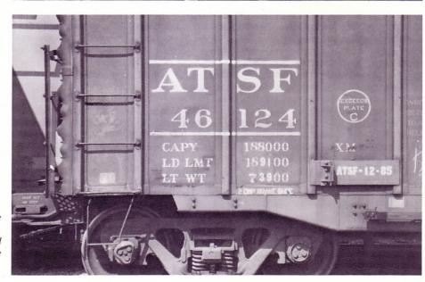
Side sill architecture of the ACF 6100 design. Note this style is very characteristic of ACF cars. In this case the first drop occurs in between the first and second post followed by a second drop in between the second and third posts.
