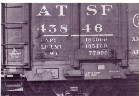
Side sill archicture of the **PS 6196** design. Note just the short line to almost the first post and then angled and dropped.
