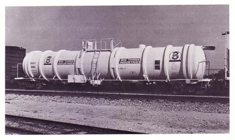
(RIGHT) BIGX 1006-1011. Built 8=9-62, 11-63. This series has a 16,293 gallon capacity. These 100-ton cars are the oldest still on the fleet.
