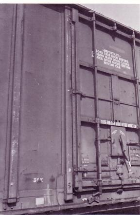
Door post of the ACF **6100** design. Note how it is similar in width to the Berwick design but lacks the oval opening at the bottom.
