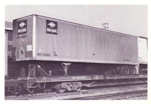
MPZ 250110. Trailmobile's 45-foot piggyback van. Note the use of two sets of reporting marks and numbers on the sides of the vans, an unusual practice for modern pig vans but common to later MP piggyback trailer liveries.
