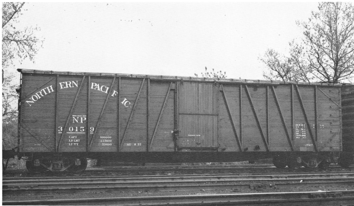
NP 30159, was built in 9-23 by General American as a 40-ton "door-and-a-half" auto boxcar in the 6000-series. It was later rebuilt into this single-door general-service boxcar. (Ed Mines Collection)
