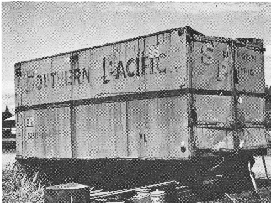
SPO-11, Albany, OR. July 28, 1987. While off its "dollies" this trailer is an excellent example of the first equipment Southern Pacific ran in Trailer Flatcar Service. (Richard Yaremko photo)
