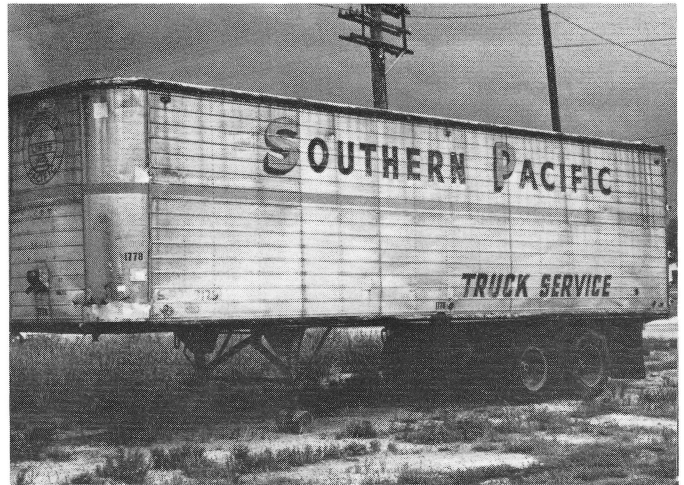
SPT 9129, Denison, TX. May 23, 1987. This photo illustrates the mid-to-late 1950's era trailers. Painted aluminum with orange bands, these trailers still haven't received the AAR TFC reporting marks. This Lufkin built trailer was assigned to service in Texas and Louisiana. (Richard Yaremko photo)
