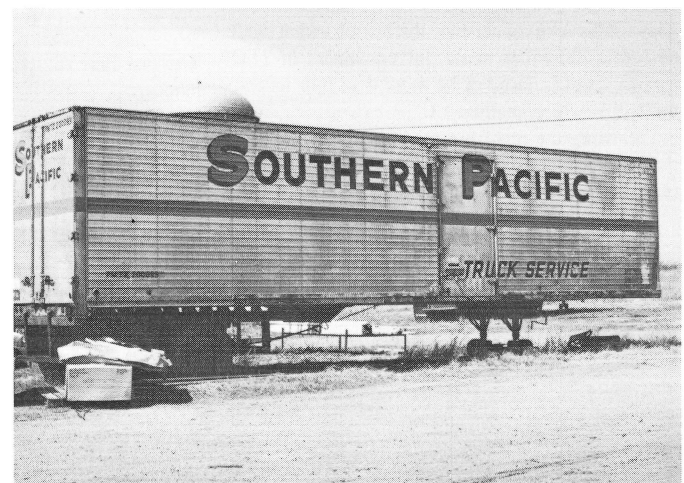
PMTZ 200093. Ennis, TX. March 15, 1980. Typical of the mid-to-late Sixties trailers, this Freuhauf 40-foot trailer was part of Pacific Motor Trucking but obviously spent time on the southeastern end of the Espee system. (Richard Yaremko photo)
