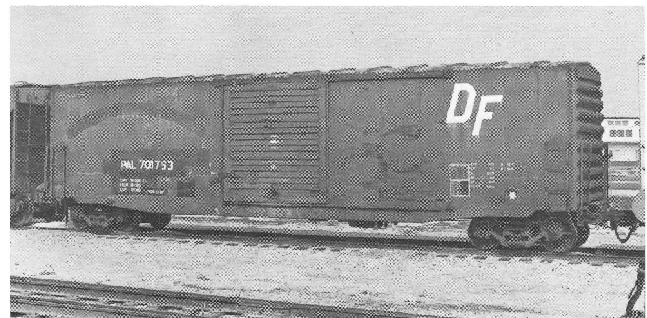
Paducah and Louisville's PAL 701753 is a Pullman-Standard built ex-ICG (Gulf, Mobile and Ohio) loader equipped 50' 6" boxcar. (David G. Casdorff photo)
