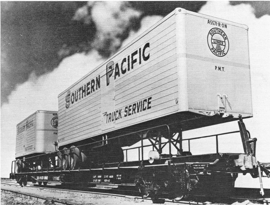
SP 510500. This flat car was built in April 1957. The trailer at the front of the photograph is PMT A5571-R a 35' insulated trailer. The trailer at the rear is a 26' trailer. (Richard Yaremko collection)
