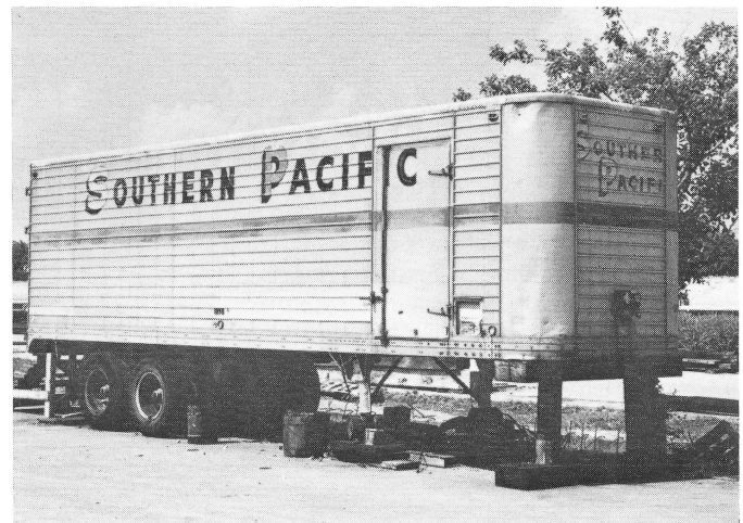
SPT 1898. Ennis, TX. May 17, 1987. Built by Brown Trailer of Spokane, Washington, this trailer came equipped with a side door. (Richard Yaremko photo)
