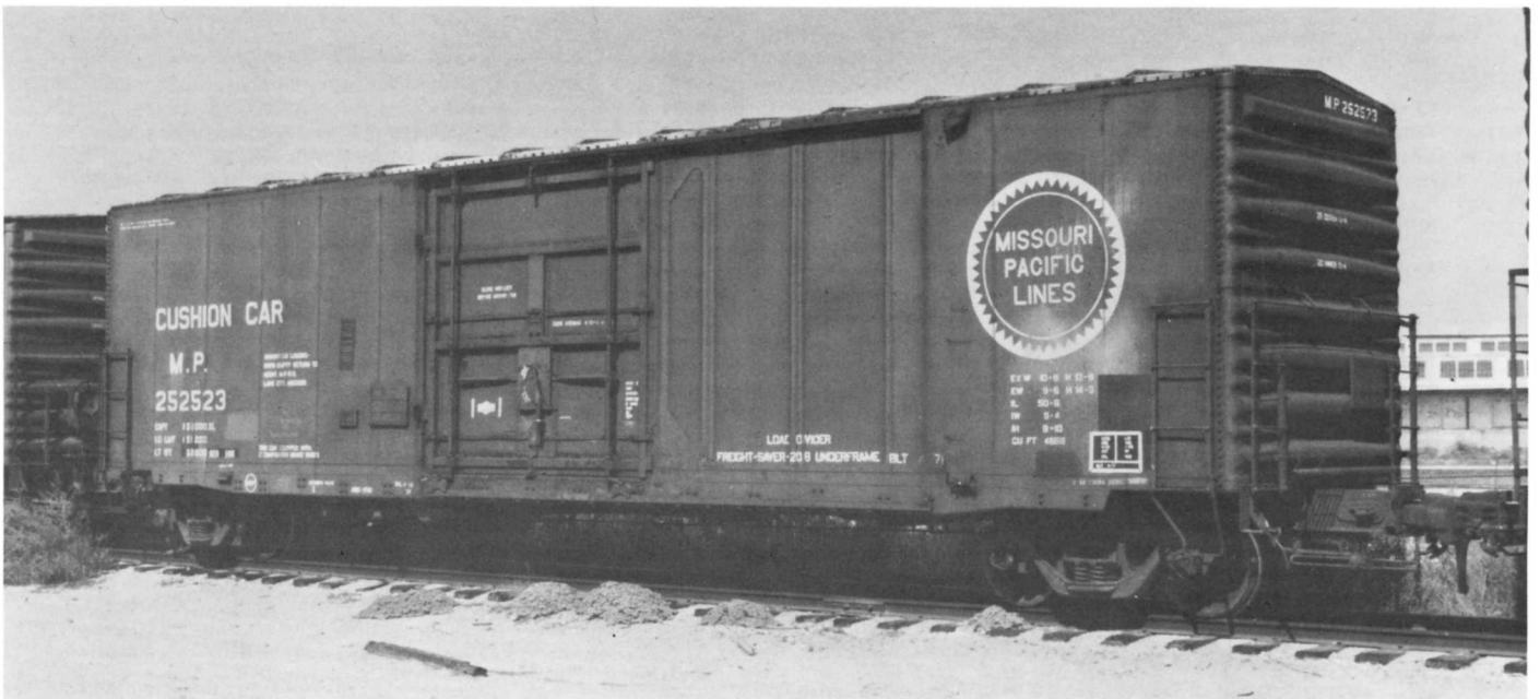
(ABOVE) MP 252523, with the very unique ACF "panels" (to the right of the door in this photo). The panels are a design feature to strengthen the door track area. The series of 150 cars were built in 1971 by ACF's St. Louis plant. This particular car was assigned to the M.P. Lake City, Missouri car pool. Notice the plug door and the side sill architecture compared to the car in the top photo on this page.
