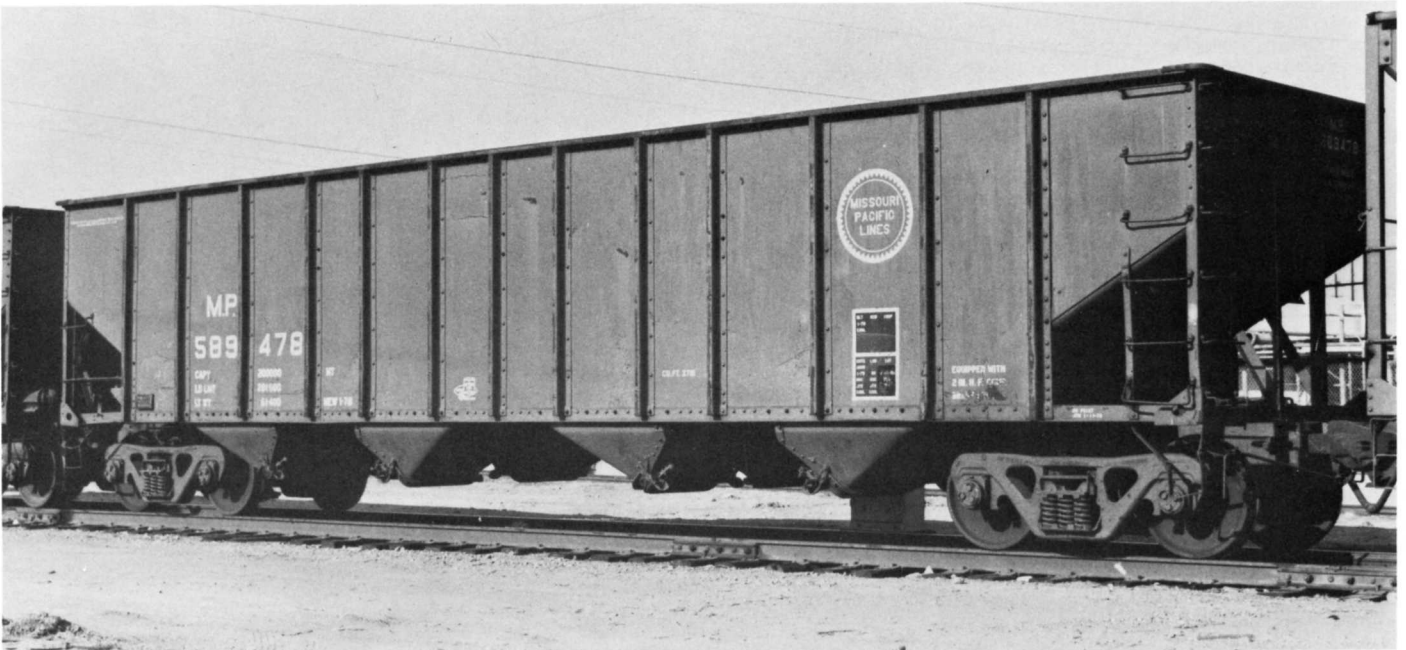
(ABOVE) MP 589478, another quad hopper displays the older "buzzsaw" logo. The series of 1000 cars were built in 1977 and 1978 by Bethlehem Steel Car.
