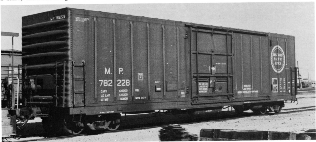
(BELOW) MP 782228 was built in 3-77 by Pacific Car and Foundry. Compare the similarities of this car and MP 780548 (illustrated before), built some 10 years apart. Both cars feature exterior post riveted construction, flat roofs, wrap-around ends, and side sills of nearly identical design.
