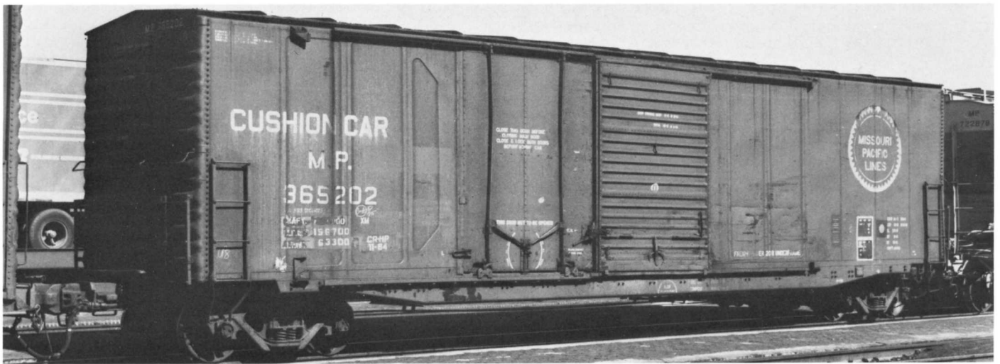
(ABOVE) MP 365202, part of a series of 75 cars built by ACF in 1969. Note the "ACF panels" on the plug side only (not always the case).
