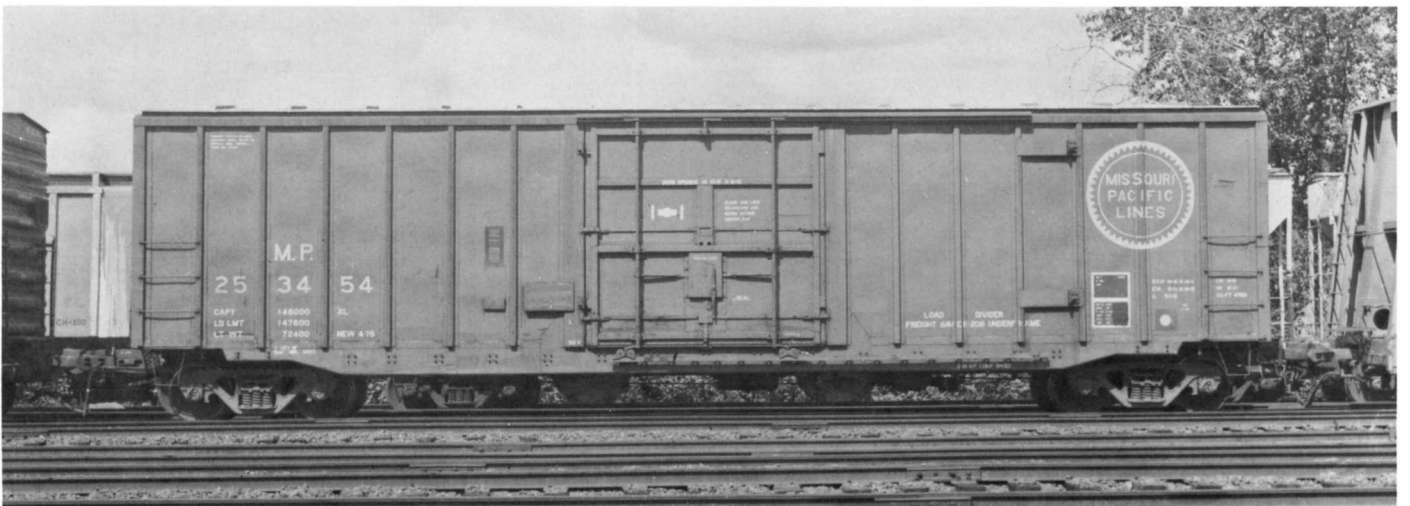
(BELOW) MP 253454, part of a series of 300 cars built by ACF in 1976. This car is shown here in its original markings. Notice how on this car (and others throughout this issue) the MP marks its cars to the right of the door with the type of loaders and cushioning the car is equipped with - in this case the Evans load dividers and ACF Freight Saver 20B.
