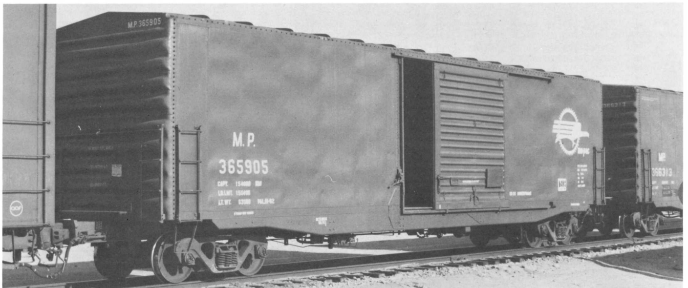
(BELOW) MP 367637, part of one of the largest series of boxcars on the modern MoPac roster. The series probably can also claim to be one of the (if not THE) largest series of purpose built "XF" boxcars (cars specially for food products). The 1000 cars of this series were delivered by Berwick in 1979. Notice the side sill design, offset combination doors, non-terminating ends with Pullman-Standard (-like) corrugations and peaked roof.
