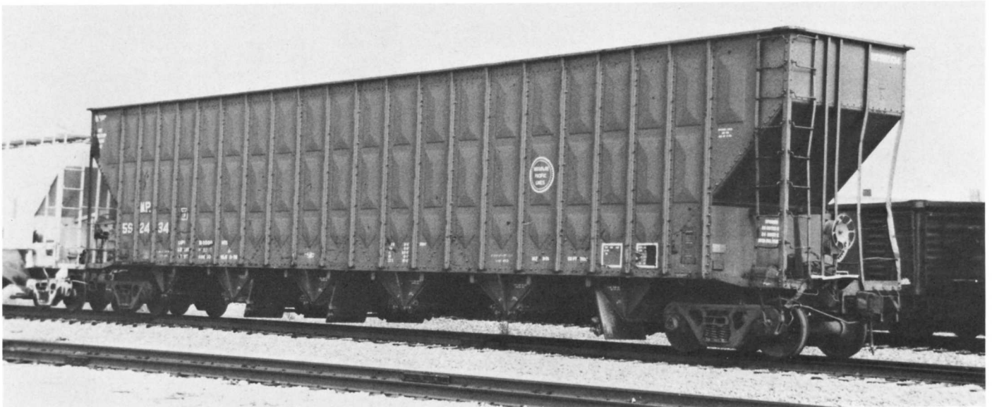
(BELOW) MP 641171, part of a series of 1,500 cars built in Mexico by CNCF. The Missouri Pacific is one of the few U.S. railroads known to have bought large numbers of freight cars built in Mexico (which included boxcars as well as gondolas).
