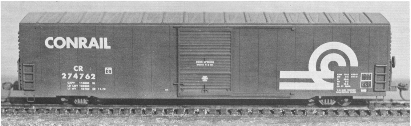
(Above) Conrail 274762 is another 60' Robin's Rails boxcar. This model is a similar conversion to the DRGW 63855 except the wheel base was left stock from the kit and the doors were made from two spliced Robin's Rails 50' PS-1 boxcar kit's doors. (Below) GTW 390250 again uses the Robin's Rails 60' boxcar. In a similar fashion as the other two cars on this page, this model has had its side sill replaced, wheel base extended, rivets removed and car side scribed. The doors were replaced with ones from an Athearn 50' "Railbox" kit. A-Line stirrups and Kadee couplers were added.
