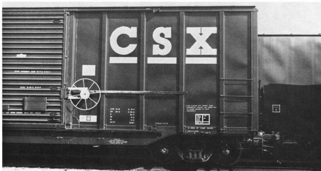
C&O 164243, part of a series of 50 auto parts boxcars delivered to the C&O just before its final merger into the CSX Transportation, Inc. system. These are the first boxcars to be new built in the United States since 1983. The cars are 51'7" (IL) double door boxcars. They feature a number of Pullman-Standard design boxcar parts and were made by Pullman Standard Mfg., Division of Trinity Industries in June 1 1987. Notice the cars are equipped with handwheels to assist in opening the doors. These are the new design Youngstown doors without the horizontal overlaps that separated the door into several distinct "panels." The cars have 15" End-of-Car cushioning made by Keystone. One other note, General Electric Railcar Services Corporation is the owner-lessor on these cars and most (if not all) are assigned to the DMSM Saginaw, MI pool. David G. Casdorff photos
