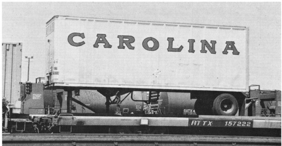
(Above) Carolina 27-2914 is an exterior-post Trailmobile built pup trailer. David G. Casdorff photo
