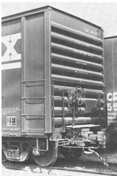
C&O 164243, part of a series of 50 auto parts boxcars delivered to the C&O just before its final merger into the CSX Transportation, Inc. system. These are the first boxcars to be new built in the United States since 1983. The cars are 51'7" (IL) double door boxcars. They feature a number of Pullman-Standard design boxcar parts and were made by Pullman Standard Mfg., Division of Trinity Industries in June 1 1987. Notice the cars are equipped with handwheels to assist in opening the doors. These are the new design Youngstown doors without the horizontal overlaps that separated the door into several distinct "panels." The cars have 15" End-of-Car cushioning made by Keystone. One other note, General Electric Railcar Services Corporation is the owner-lessor on these cars and most (if not all) are assigned to the DMSM Saginaw, MI pool. David G. Casdorff photos
