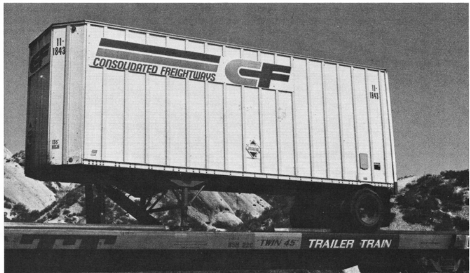
(Above) Consolidated Freightways 11-1843 is an exterior-post Road Systems built pup trailer. (Below) D-A Lubricant Co., Inc. is an example of a private-owner pup trailer riding the rails. David G. Casdorff photos
