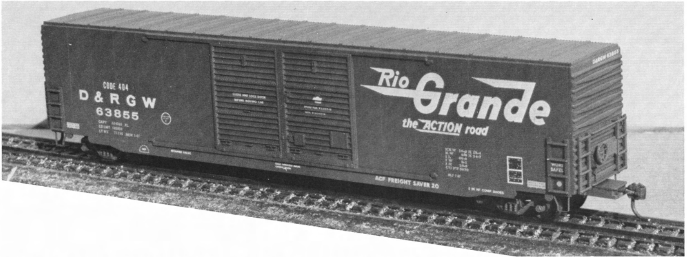
(Above) D&RGW 63855 started out with a 60' Robin's Rails Boxcar. The rivets were removed and car sides scribed to simulate the welded construction. The side sill was replaced and the wheel base was extended. The doors were replaced with doors from MDC's 50-foot double door boxcar. Kadee Couplers and A-Line stirrups were also used.
