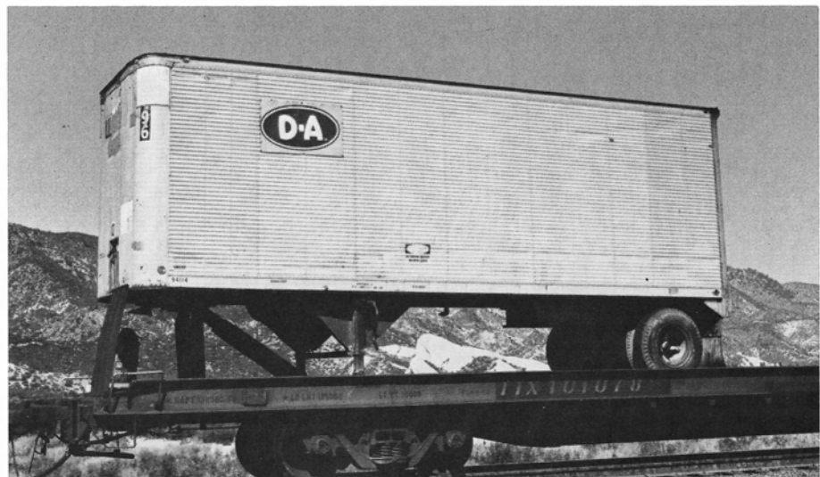
(Above) Consolidated Freightways 11-1843 is an exterior-post Road Systems built pup trailer. (Below) D-A Lubricant Co., Inc. is an example of a private-owner pup trailer riding the rails. David G. Casdorff photos
