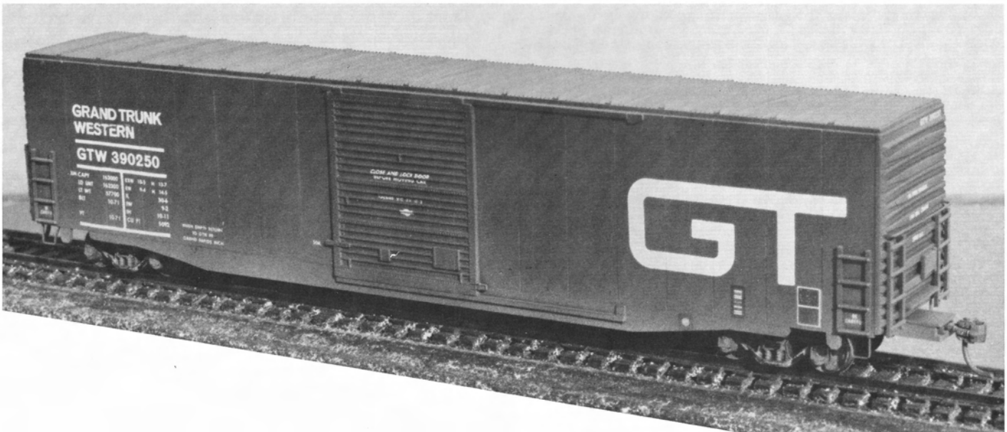
(Above) Conrail 274762 is another 60' Robin's Rails boxcar. This model is a similar conversion to the DRGW 63855 except the wheel base was left stock from the kit and the doors were made from two spliced Robin's Rails 50' PS-1 boxcar kit's doors. (Below) GTW 390250 again uses the Robin's Rails 60' boxcar. In a similar fashion as the other two cars on this page, this model has had its side sill replaced, wheel base extended, rivets removed and car side scribed. The doors were replaced with ones from an Athearn 50' "Railbox" kit. A-Line stirrups and Kadee couplers were added.
