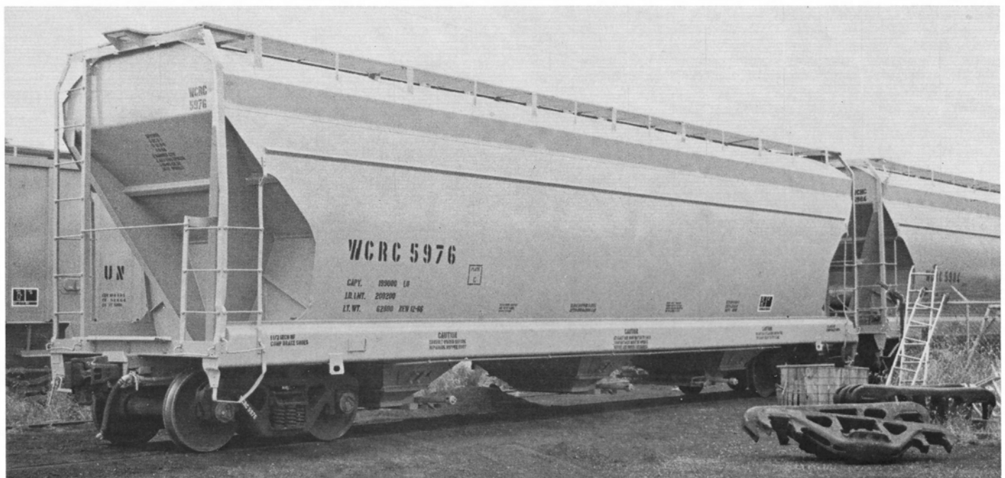
(Above) "Lake Huron," CRYX 1094 was rebuilt in June 1987 by CEECO, Tacoma, WA. The car was a former Santa Fe "XLI" Bx-132 class boxcar. Council Bluffs, IA, July 1987. (Below) Washington Central's WCRC 5976, former Conrail (nee-New York Central) ACF Center Flow covered hopper just after rebuilding by PLM's Sioux City, IA shops. Both photos by Mike Foley
