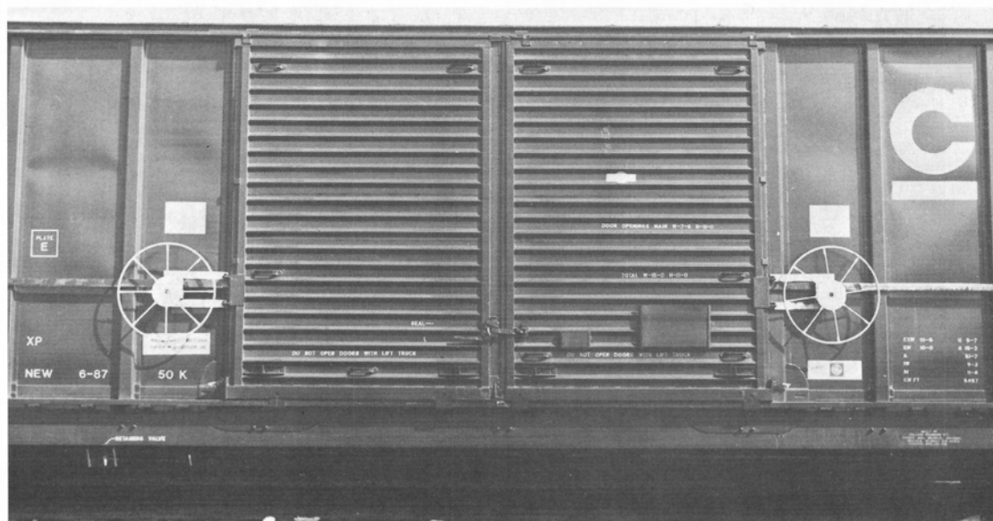
C&O 164243, part of a series of 50 auto parts boxcars delivered to the C&O just before its final merger into the CSX Transportation, Inc. system. These are the first boxcars to be new built in the United States since 1983. The cars are 51'7" (IL) double door boxcars. They feature a number of Pullman-Standard design boxcar parts and were made by Pullman Standard Mfg., Division of Trinity Industries in June 1 1987. Notice the cars are equipped with handwheels to assist in opening the doors. These are the new design Youngstown doors without the horizontal overlaps that separated the door into several distinct "panels." The cars have 15" End-of-Car cushioning made by Keystone. One other note, General Electric Railcar Services Corporation is the owner-lessor on these cars and most (if not all) are assigned to the DMSM Saginaw, MI pool. David G. Casdorff photos
