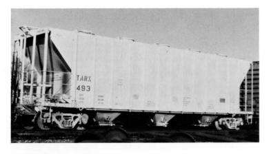
TARX 493, former SAN 493. TARX is the reporting marks for Sandersville Leasing, a subsidiary of the SAN. The cars were rebuilt in 1981 by the Safety Railway Service. Note the lack of the large Sandersville logo and large number used on SAN initialed cars. This car has the centered roofwalk, covered hoppers later received by the Sandersville had off-centered walks. Tony Hodun photo
