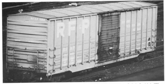
(Above) this photo of RF&P 5296 clearly shows the "X" end corrugations used on this series. Built by Berwick in 1976. S. Maher photo. (Below) RF&P 2145, also a waffle-sided car. This one built by Berwick in 1973. Ends on this car are of the Pullman-Standard 5/5 corrugated design. J.R. Quinn
